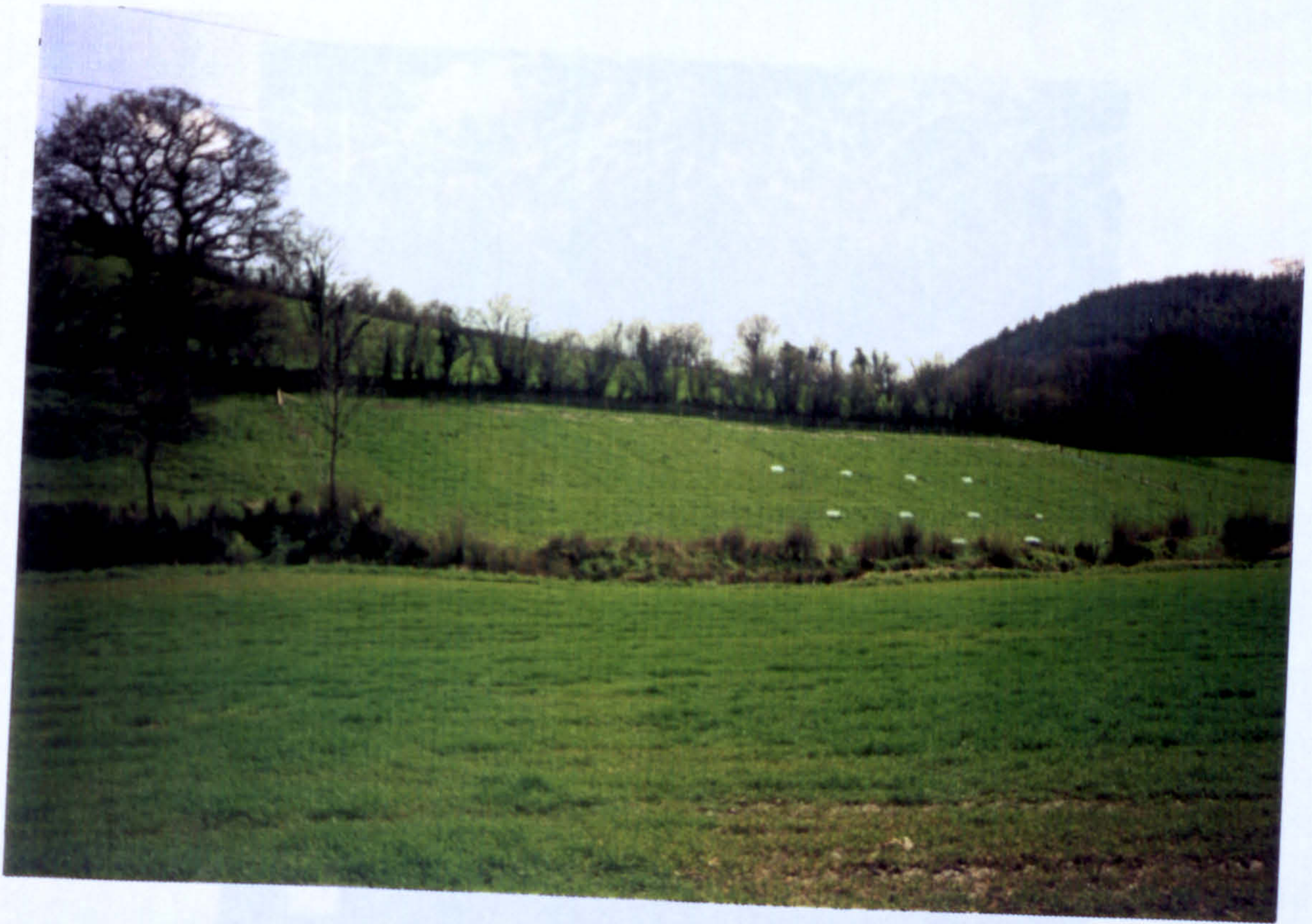
Fig. 3.1. The plots at Sidney Meadow in March 1992. The light squares are the covers of surface runoff collection troughs.
