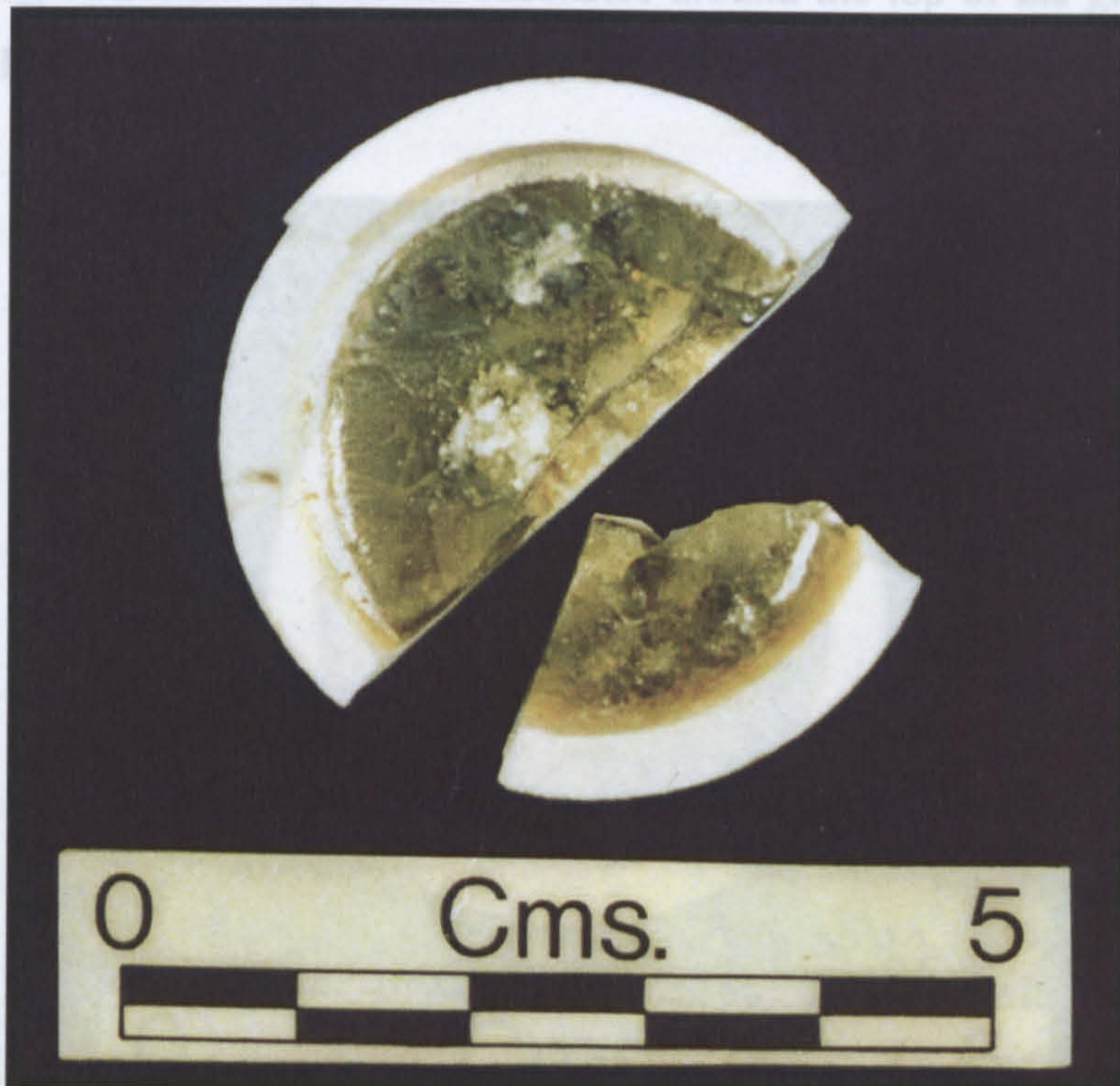
Plate 4:7 An unmixed, fritted bracken ash batch heated at 1300°C for 1 hour (Br6, Table IV:12)
