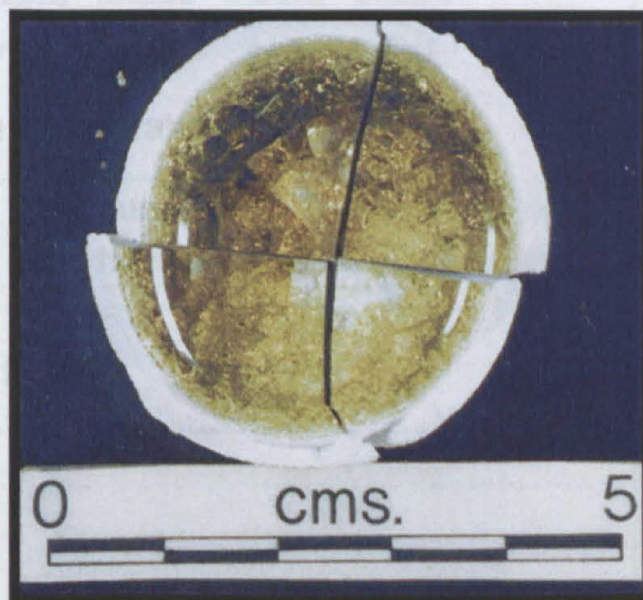
Frit 800°C 1 hour Visually homogeneous glass (Br132)
