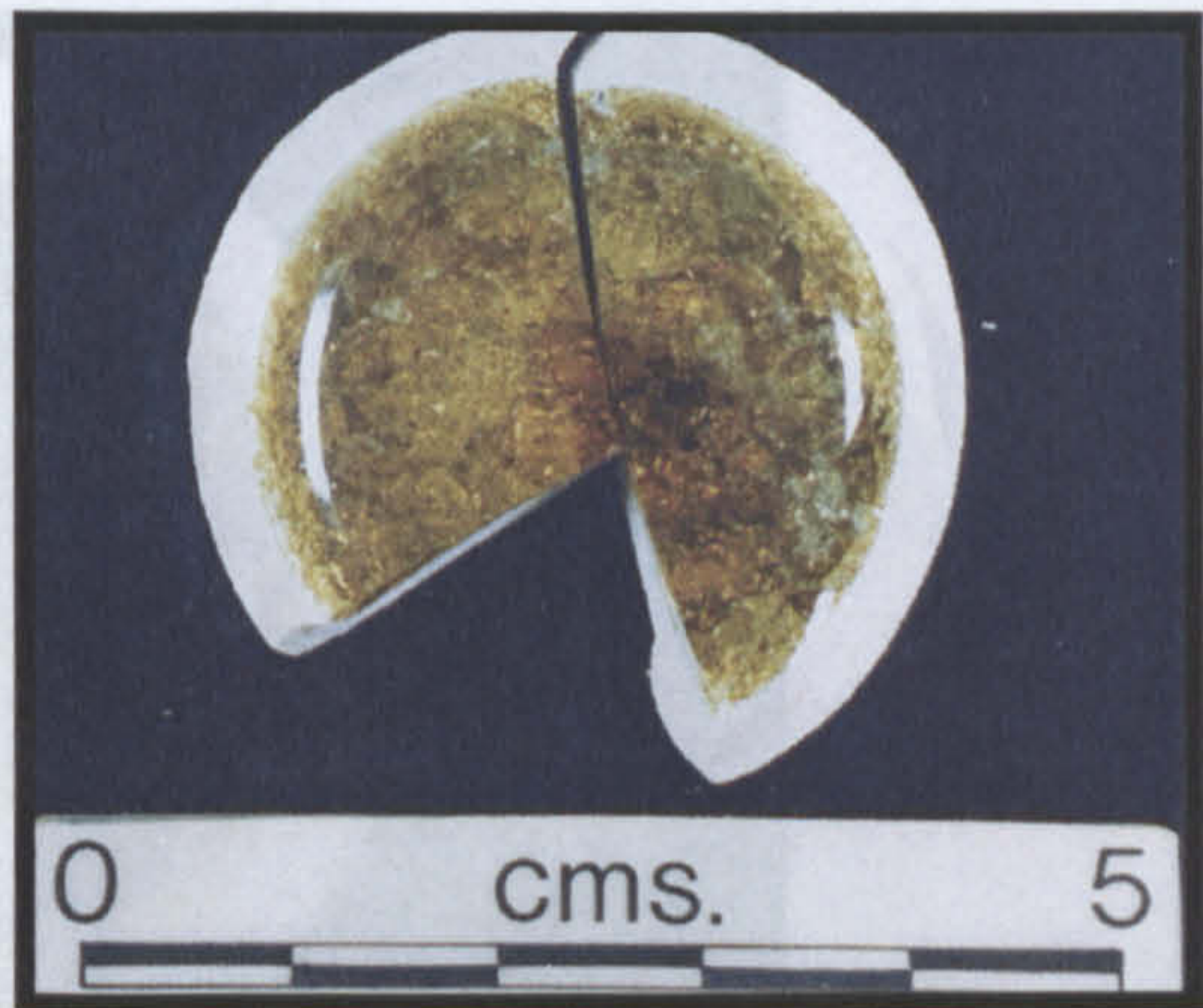
Frit 600°C 1 hour Low levels of batch relics (Br102)
