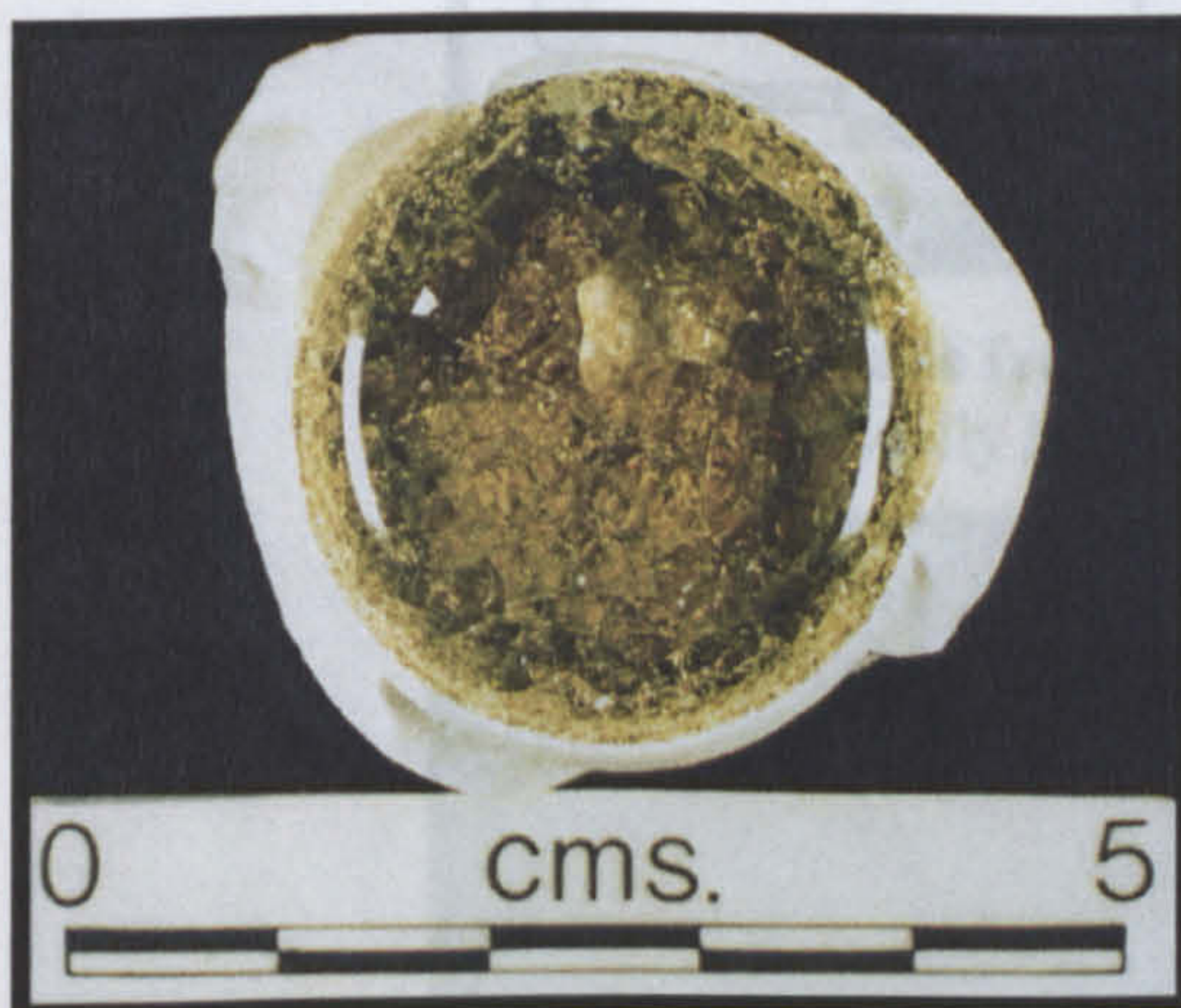
Frit 900°C 1 hour Visually homogeneous glass (Br98)
