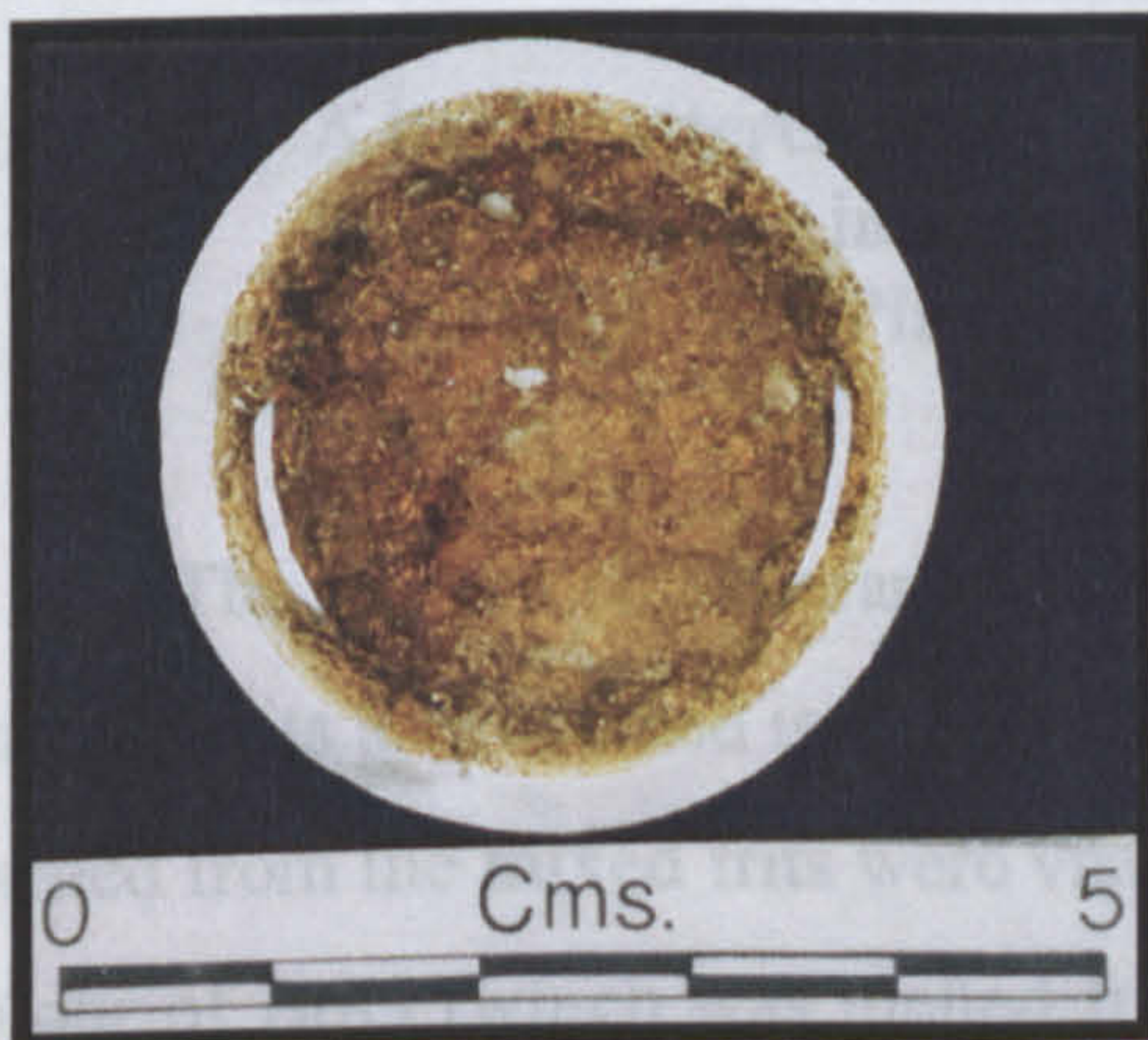
Frit 900°C 24 hours Medium levels of batch relics and low opacity (Br70)
