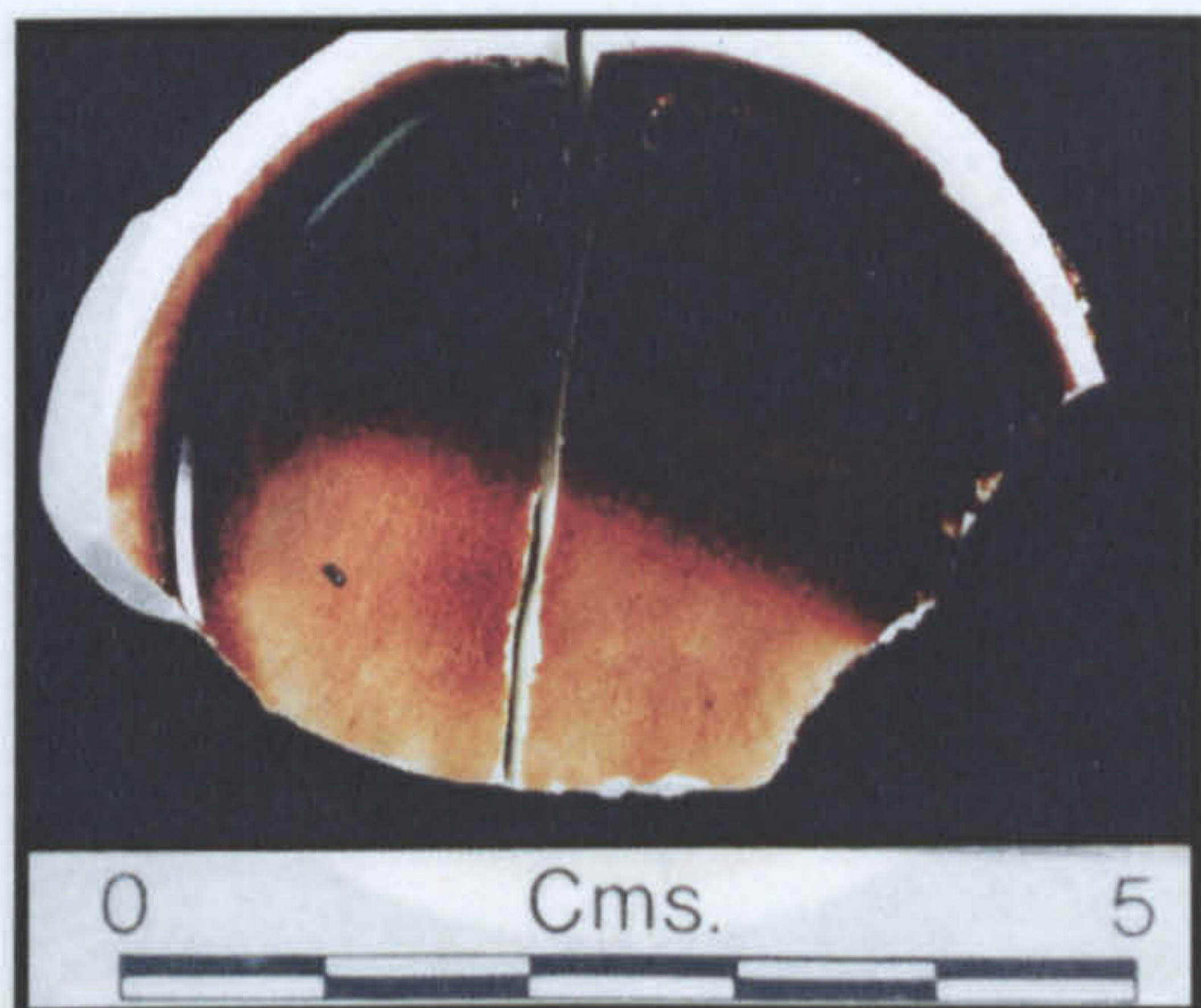
Beech Glass CON7 Crucible Visually Homogeneous Glass (Be146)
