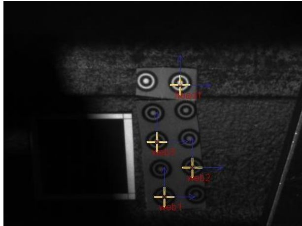
Figure 88: Targets on the web of the rail as seen by the video camera
