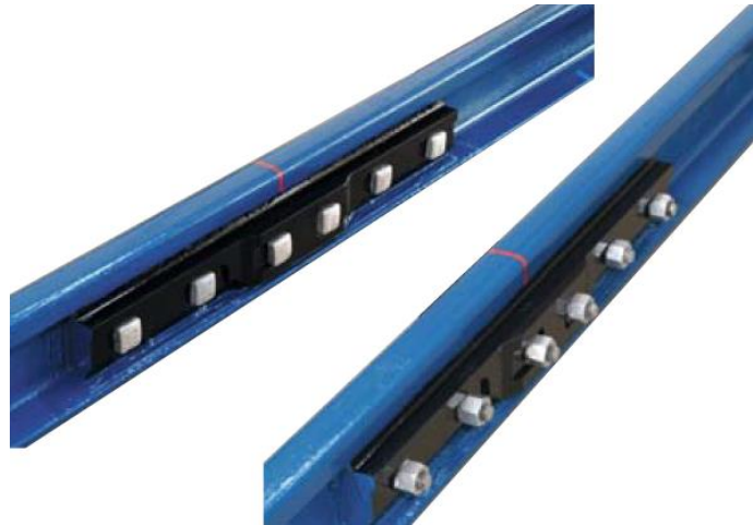
Figure 10: Fishplate strengthened in the centre to give higher modulus and reduced deflection (9)
