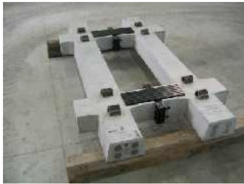
Figure 14: A joint supporting sleeper arrangement where two adjacent sleepers are fastened together (20)
