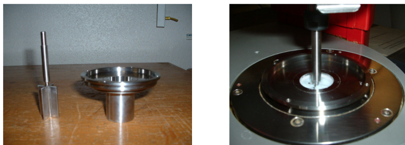
Figure 5.5: Vane geometry used by Gaiani et al. (2006) for “rheological approach.”
