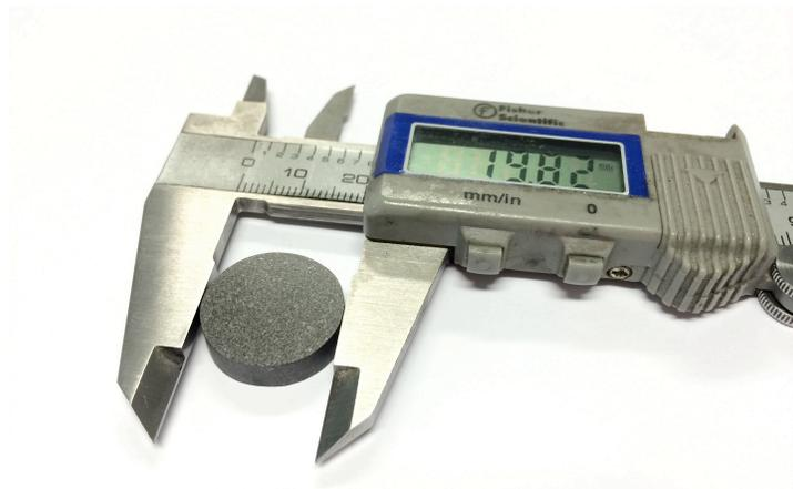
Figure 6-5: A CAS30G sample sintered at 890C for 20 min using SPS.
