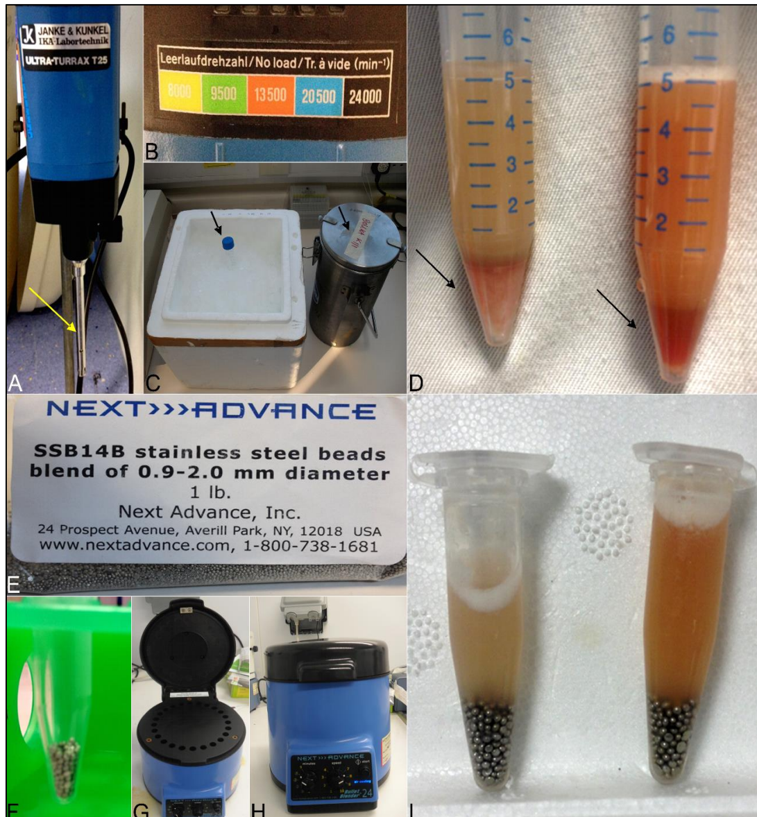
Figure 2.20: Equipment and process of tissue homogenization
