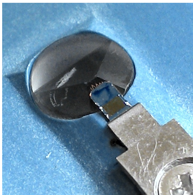
Figure 3.13: Galactose glycopolymer-coated MLCT cantilever chip in position in the AFM cantilever holder. The chip appears to have a coating and all 5 cantilevers (1 rectangular and 4 triangular, with different lengths and spring constants) are undamaged. This cantilever is the one shown in the left-hand image of Figure 3.12, above.
