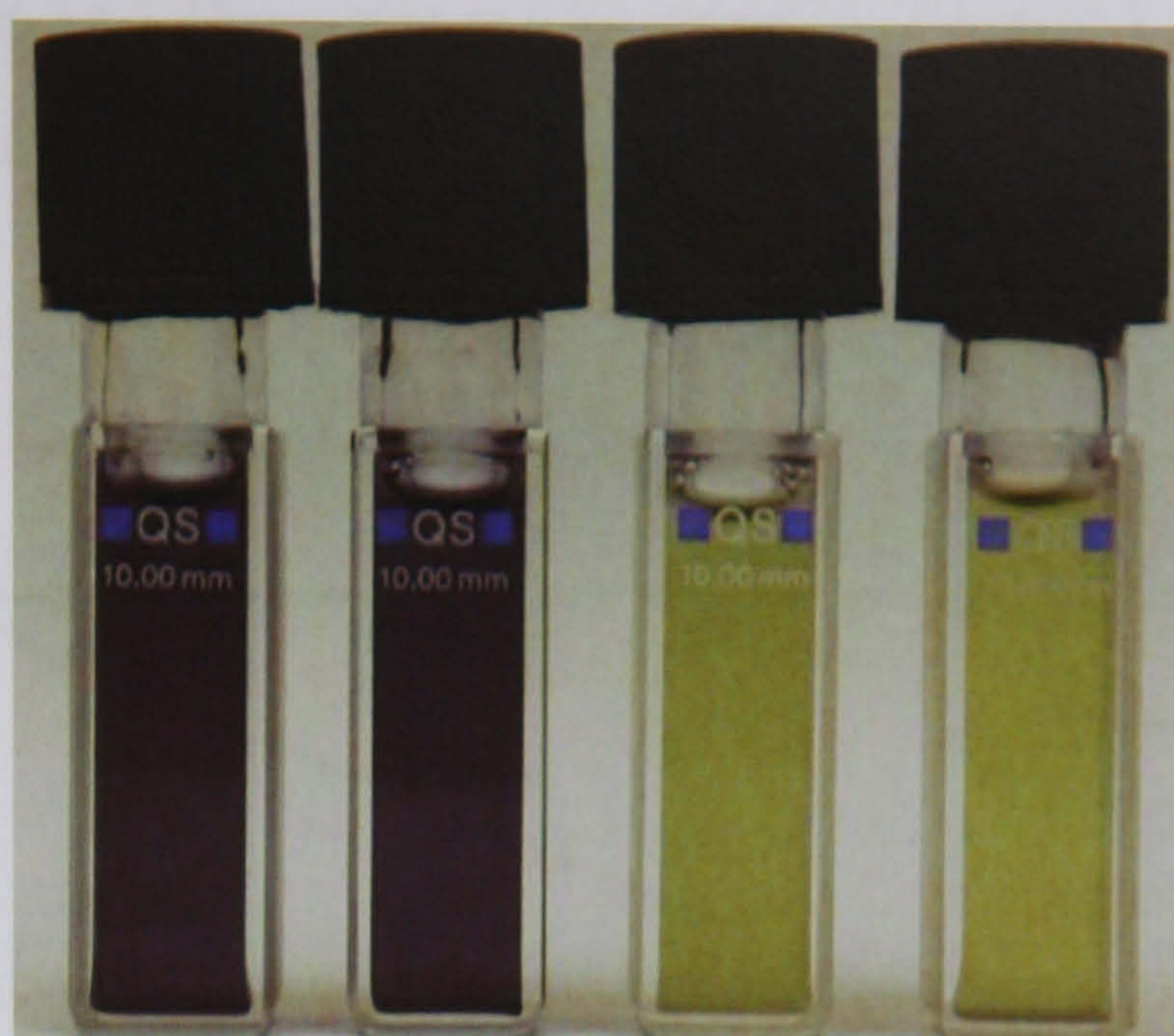
Figure 3.3.11 Photographs of Standard Dye Solutions of Irgalan Black RBLN and Reduction of the Dye Solutions using Shewanella Strain J18 143 after 18 Hours of Incubation, at 30°C
