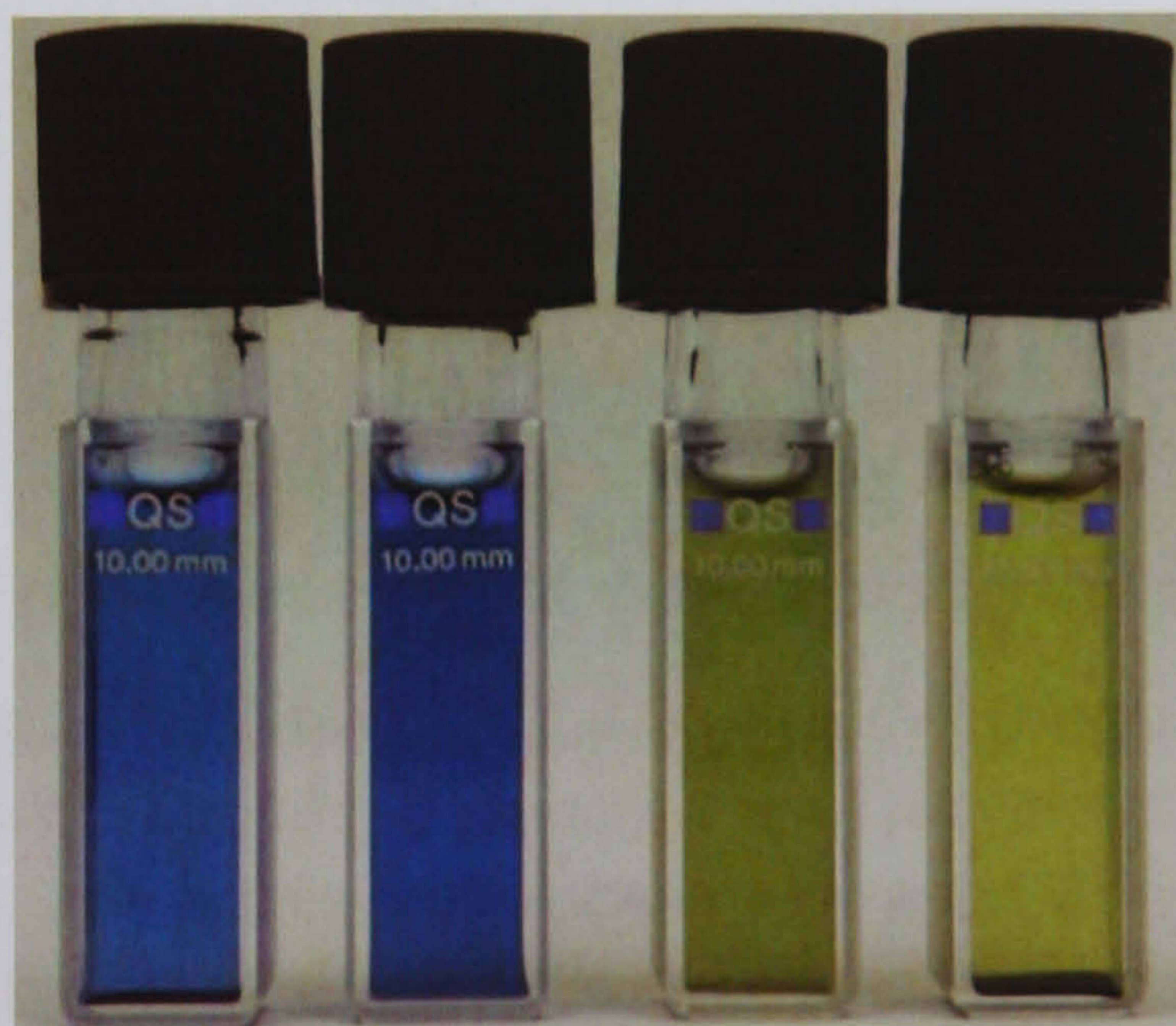
Figure 3.3.16 Photographs of Standard Solutions of Irgalan Blue 3GL and Reduction of the Dye Solutions using Shewanella Strain J18 143 after 18 Hours' Incubation, at 30°C pH 7
