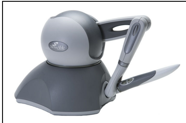
Figure 50 The Omni Haptic handwriting device
