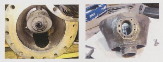
**Figure 7.3**: a) The cylindrical casing that houses the liner. b) A common Olympus diffuser and the place where the fuel injector mounts.
