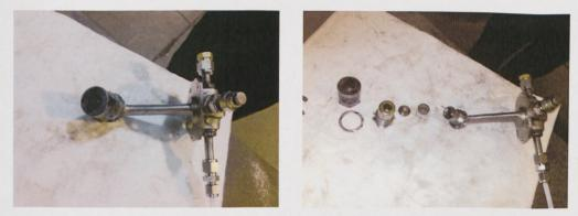
Figure 7.4: a) The fuel atomiser. b) cleaning of the fuel atomiser's parts.
