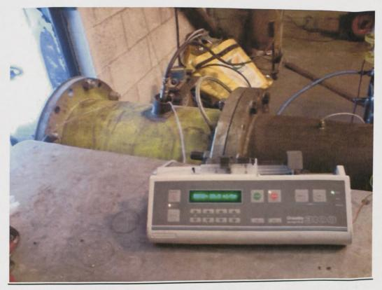
**Figure 7.7**: The Graseby 3100 syringe driver with the 25ml BD plastic syringe containing the hydrogen peroxide installed. The supply pipe that attaches to the igniter is also visible.
