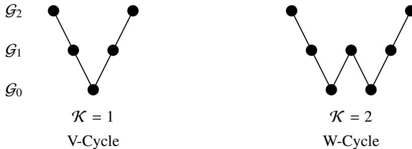
Figure 3.4: Structure of one multigrid cycle for  $\mathcal{K} = 1$  and  $\mathcal{K} = 2$ .
