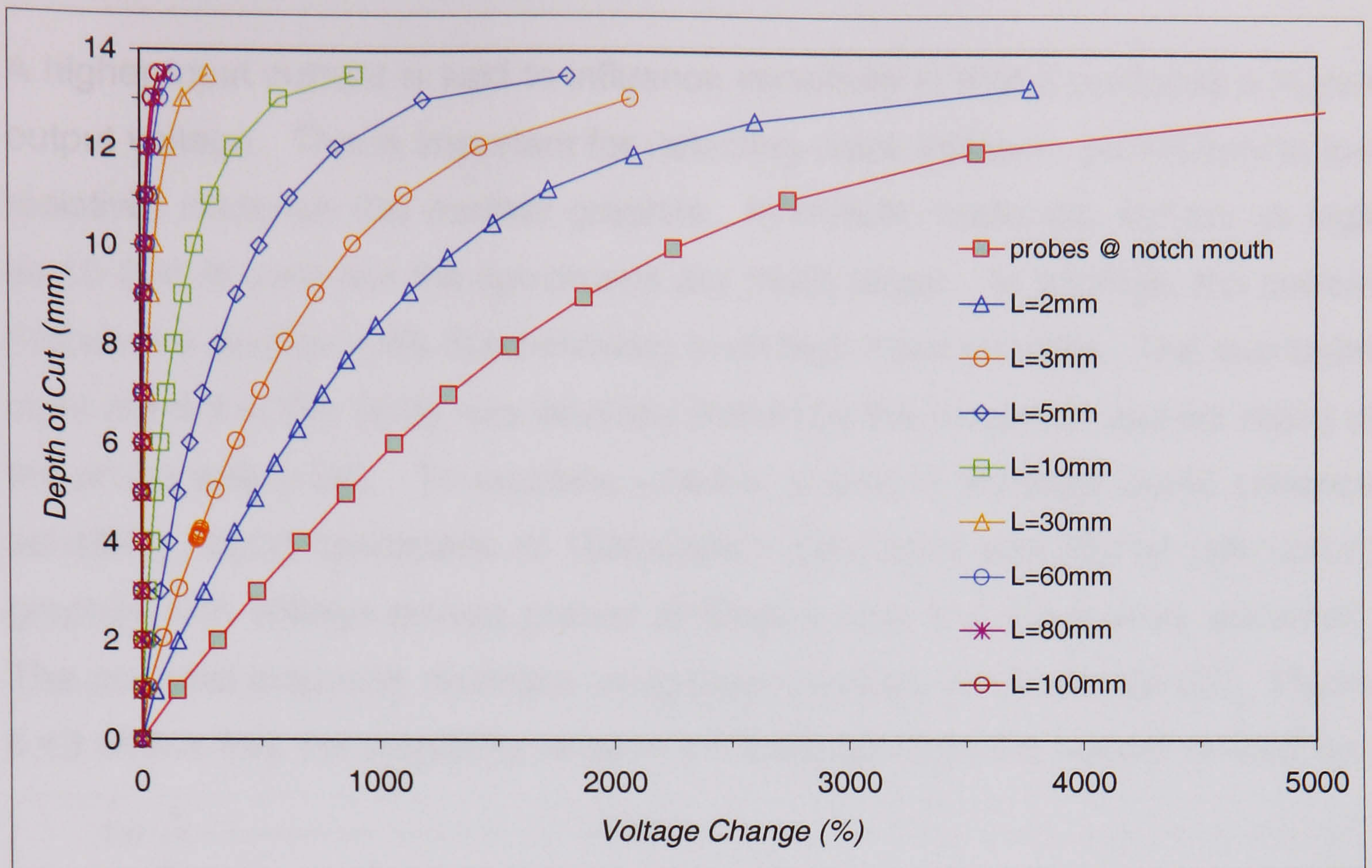
Figure 5.11. Change in sensitivity with different voltage probe spacing: Gilsocarbon bend specimen, W=14\text{mm} , i=1\text{A DC} .
