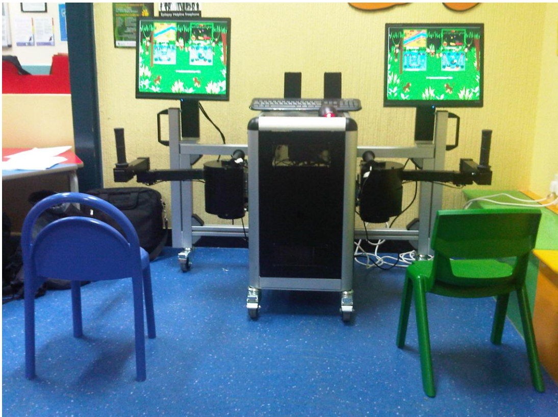
Figure 6. K005 robotic device designed for children with cerebral palsy
