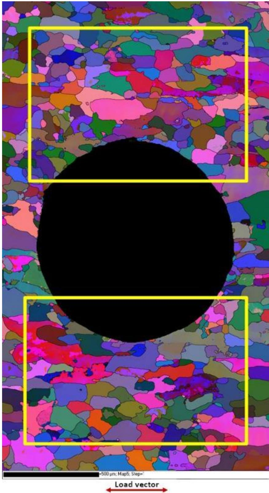
Figure 6-43. EBSD map of the regions around the hole selected for in situ observations during micro-bending.
