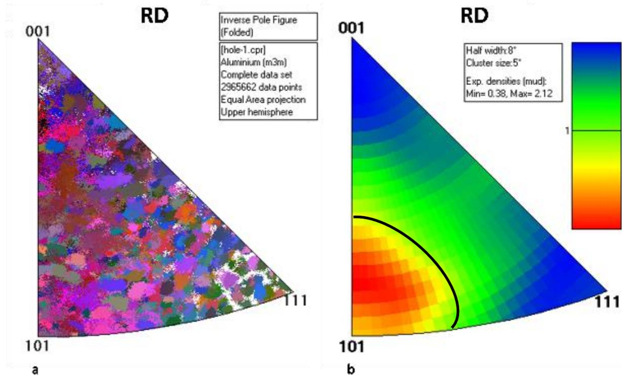
Figure 6-60. Inverse pole figures (IPF) for the EBSD map of figure 6.43 with respect to RD. a) Data points of each grain within the IPF, and b) Density contours showing the effect of rolling.
