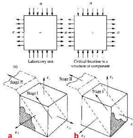
Figure 2-3. The importance of orientation of the applied stress-strain field with respect a) to the defect and b) the surface plane [2].
