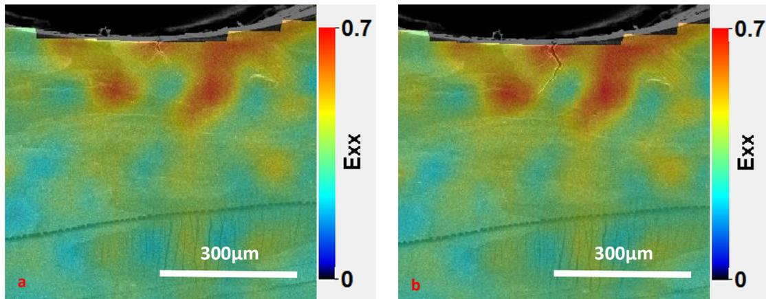
Figure 6-41. DIC strain maps at the region of cracking.
