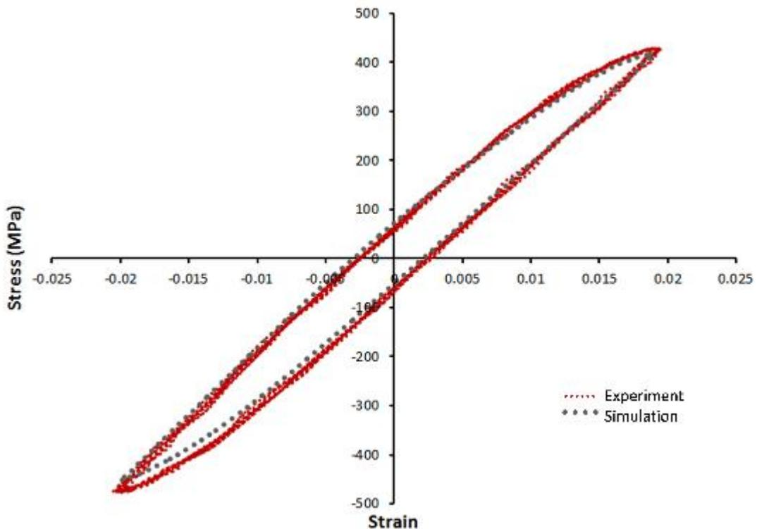
Figure 7-7. Comparison between the experimentally obtained stabilised stress-strain curve and the simulated one for  $R=-1$  and strain amplitude of 0.02.
