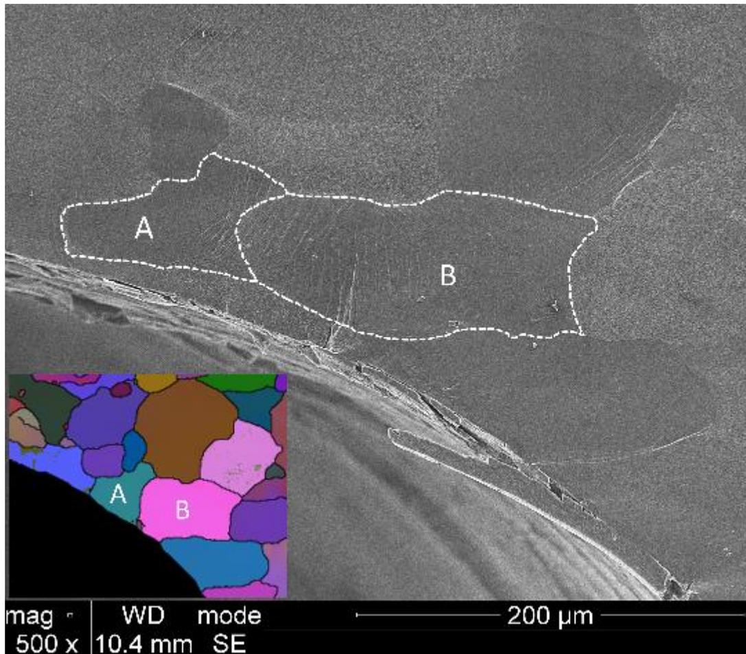
Figure 6-64. Two grains close to the edge of the hole showing strong slip banding mechanisms.
