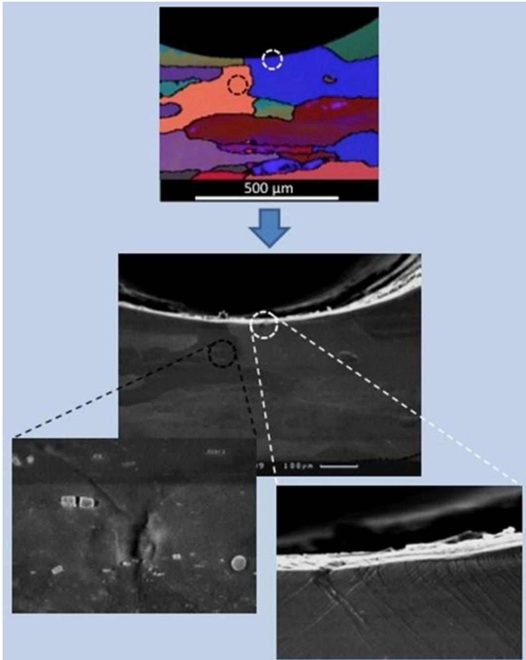
Figure 6-28. EBSD map and SEM images of the triangular region highlighted in figure 6.27b for the fully loaded condition of the specimen after 1 cycle.
