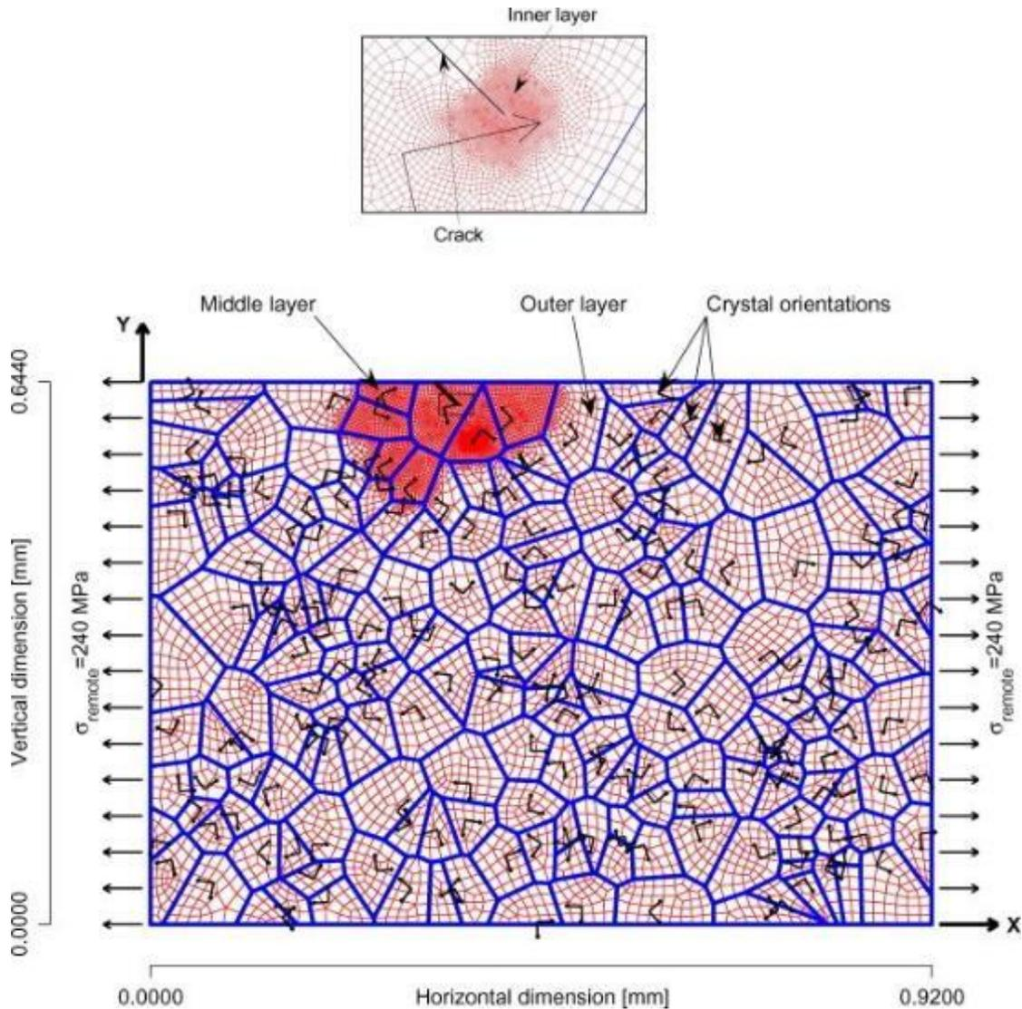
Figure 2-40. The finite element model. Details of the crack tip mesh are shown in the insert [32].
