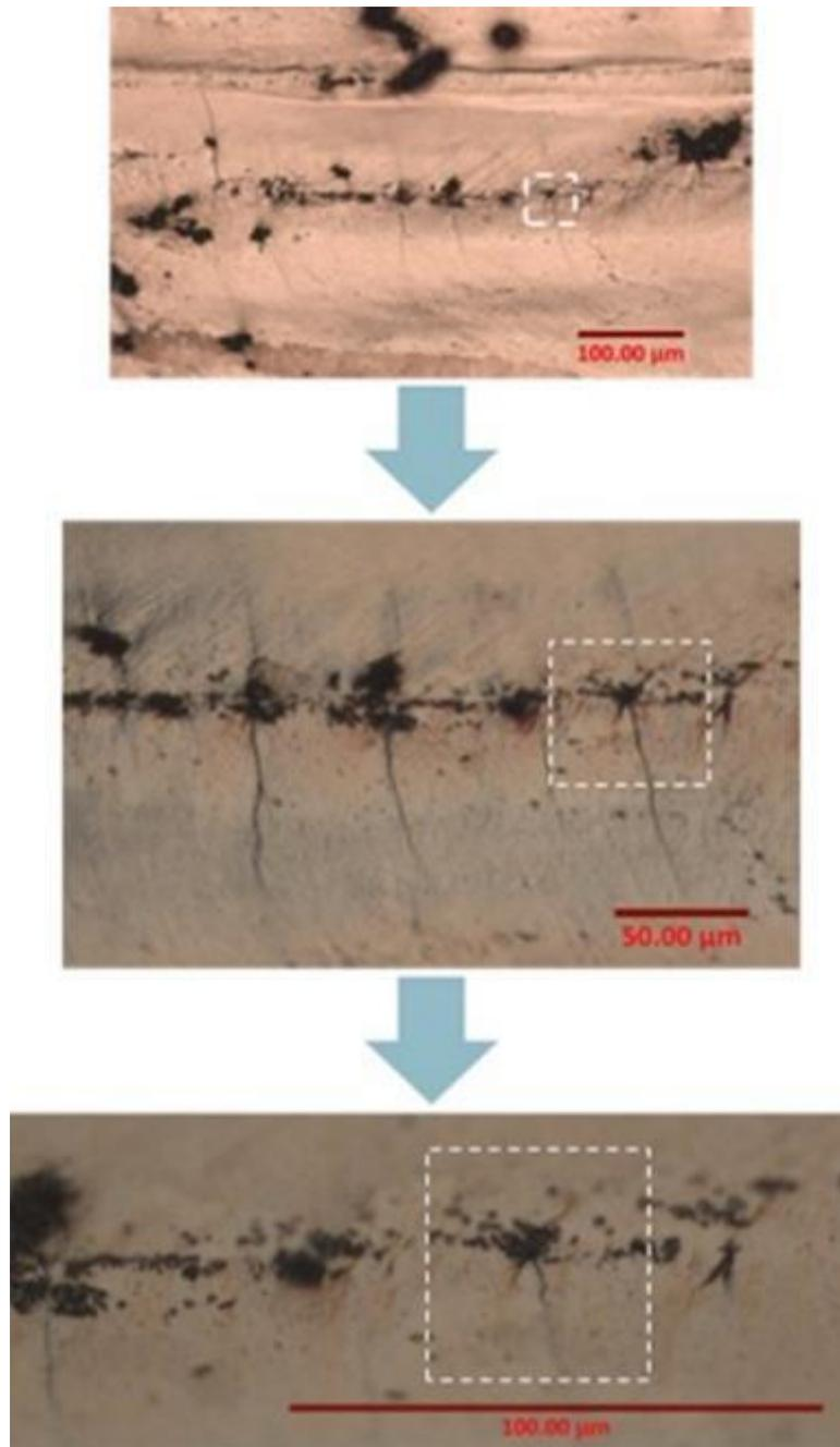
Figure 6-19. Different magnifications of a region where deformation localisations were observed. Strain localisations occurred at the neighborhood of particles lying along a GB.
