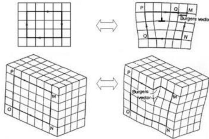
Figure 4-8. The two basic types of dislocation within a lattice: edge and screw dislocation.
