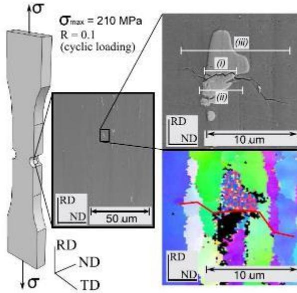
Figure 2-43. The geometry of the samples, showing also the 3 stages of MSFC phase [45].
