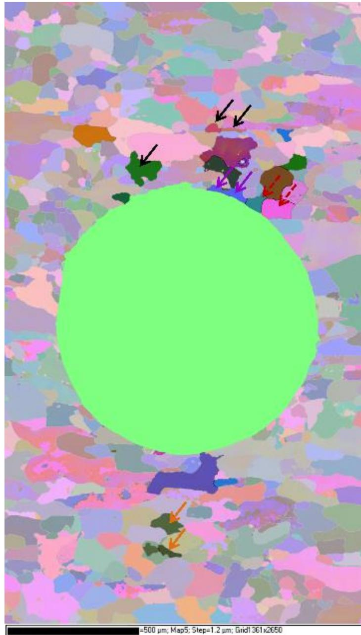
Figure 6-61. Soft grains, showing non uniform matrix deformation with slip bands observed.
