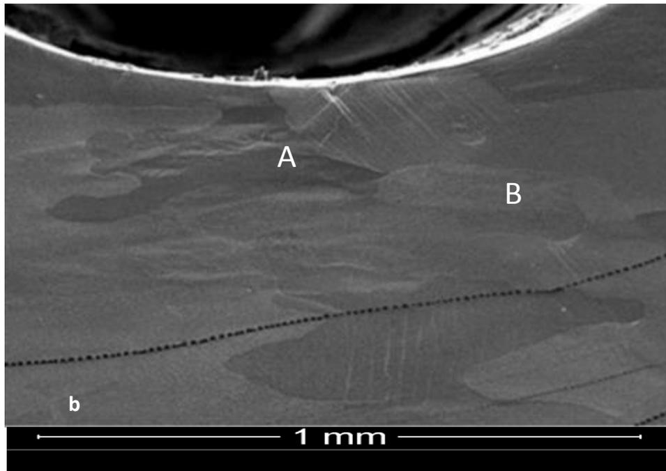
Figure 6-39. a) 'Weak' grain A facilitating a crack path towards its matrix, b) Overview image at the location of cracking, together with grain A and B.
