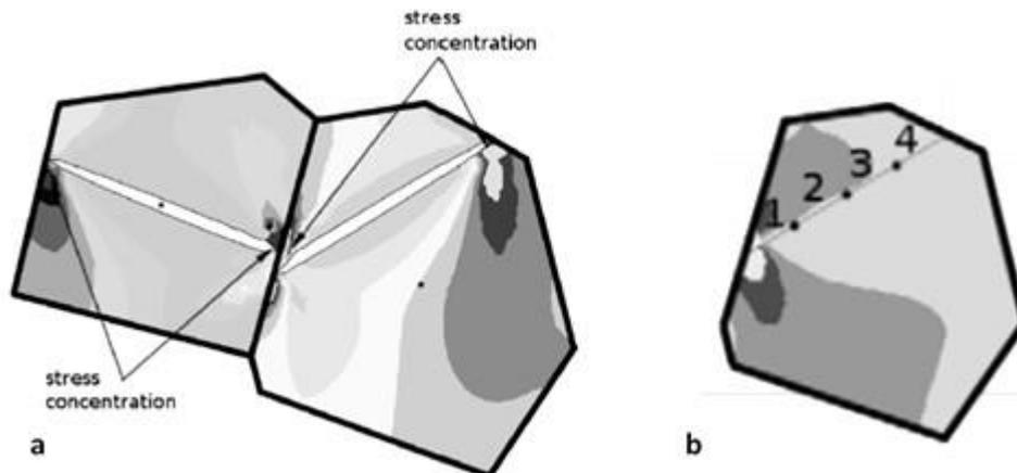
Figure 2-14. a) Nucleated crack in two grains, b) Segmented crack inside a grain [12].
