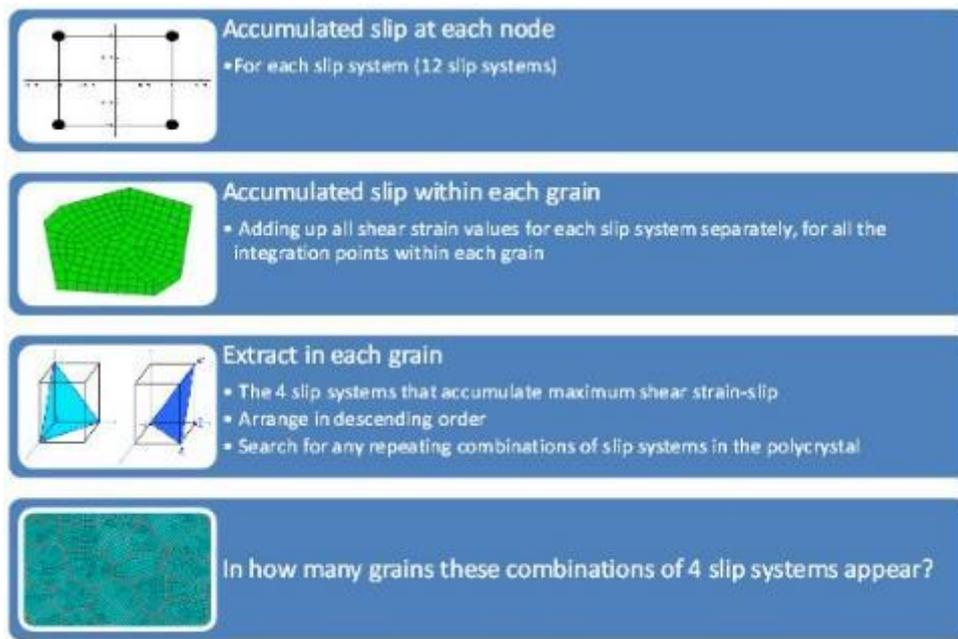
Figure 7-6. Process for identifying the slip systems with maximum shear strain values within the 2D RVE polycrystal of figure 7.5a.
