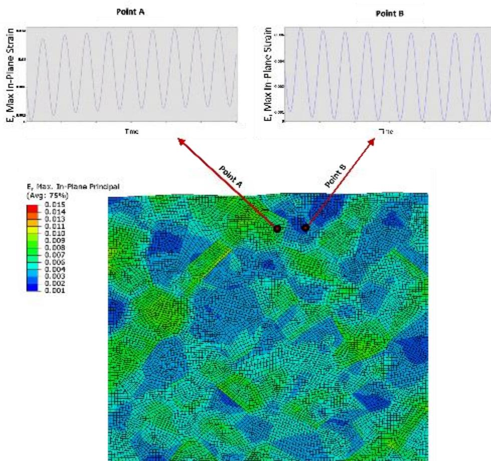
Figure 7-8. Maximum in plane strain deformation for the RVE of figure 7.5, under cyclic loading conditions, at maximum displacement and after 10 cycles. The two points show the corresponding hardening and softening that occurs at the highlighted points (A & B).
