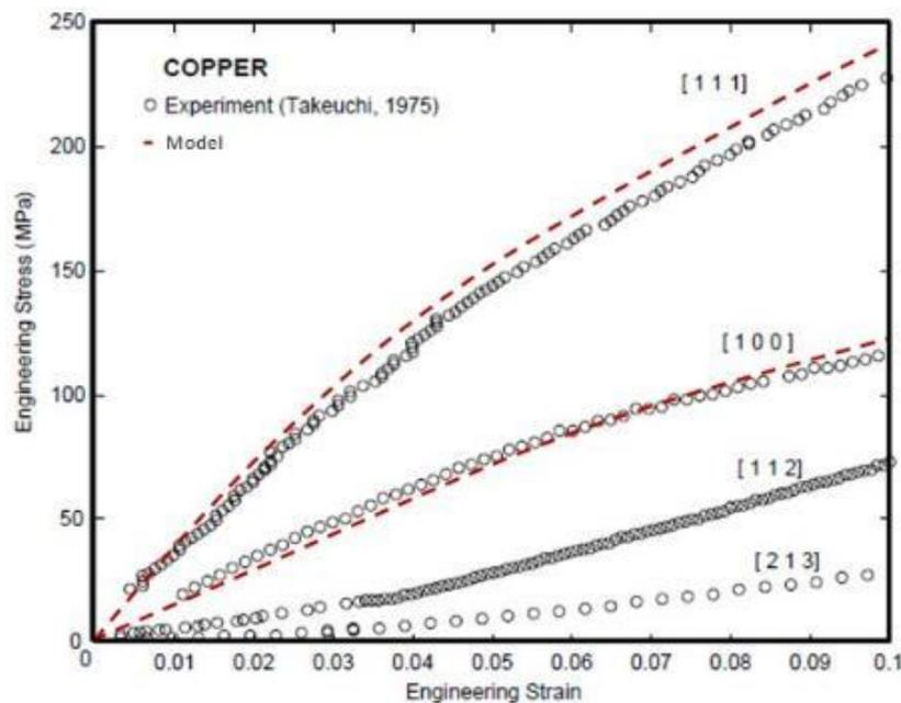
Figure 7-1. The influence of orientation for a Copper single crystal on the stress-strain curve. The open circles correspond to the experimental results; and the red lines obtained by using the UMAT code.
