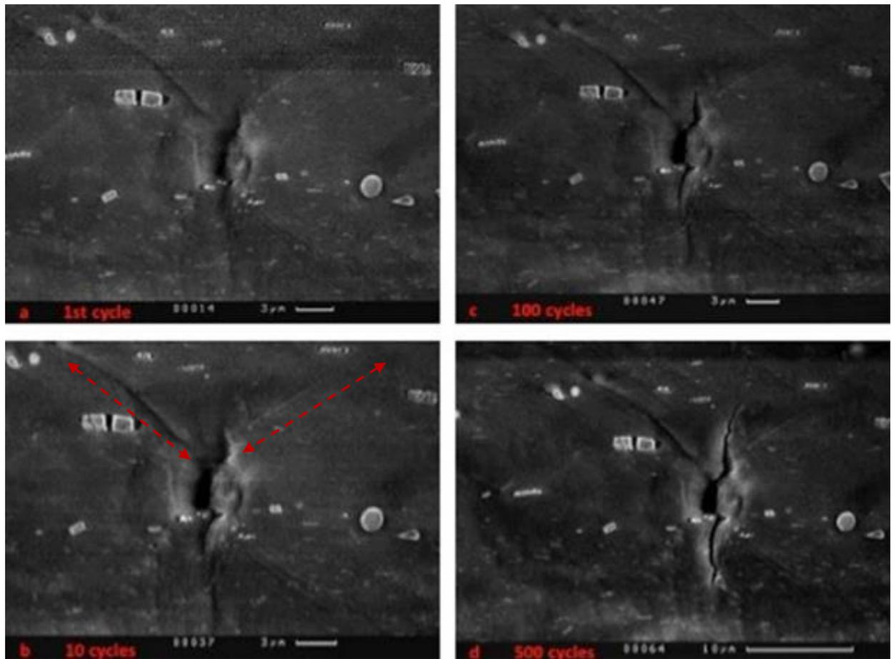
Figure 6-31. SEM images of the region of the EBSD map in figure 6-28 highlighted by a black circle for the fully loaded condition of the specimen after: a) 1 cycle, b) 10 cycles, c) 100 cycles and c) 500 cycles.
