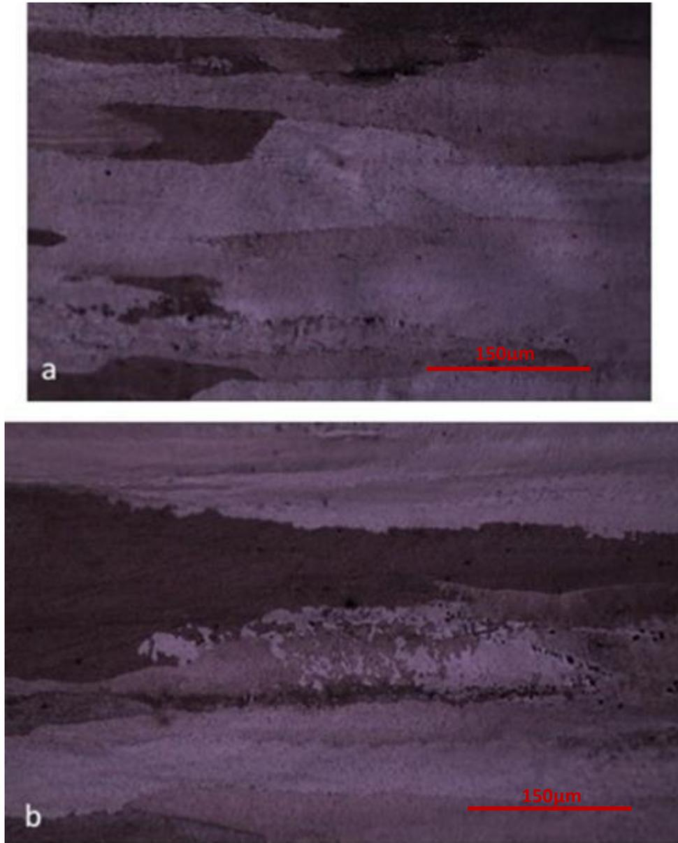
Figure 6-7. High magnification optical microscopy image from area L in Figure 6.3a. Images indicate the absence of slip bands and any significant out of plane deformation.
