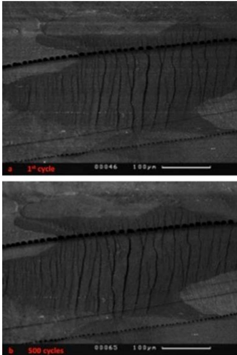
Figure 6-33. SEM images grain highlighted in figure 6-27a for the fully loaded condition of the specimen after: a) 1 cycles and b) 500 cycles.
