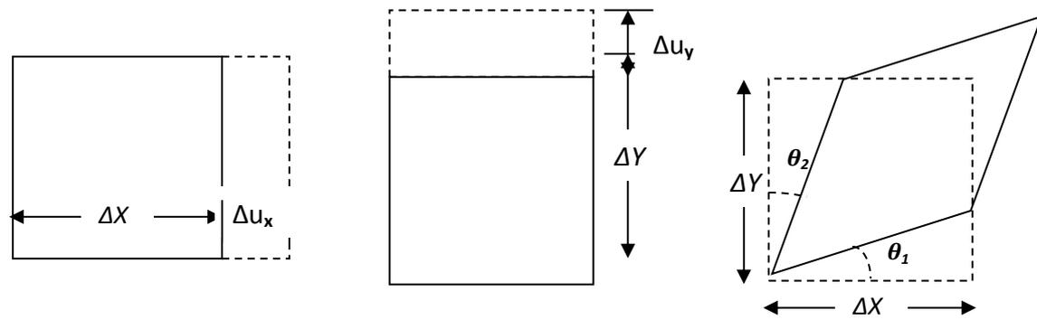
Figure 4-2. a) Uniaxial extension in the x-direction, b) Uniaxial extension in the y-direction and c) Pure shear without rotation ( $\theta_1 = \theta_2$ ).
