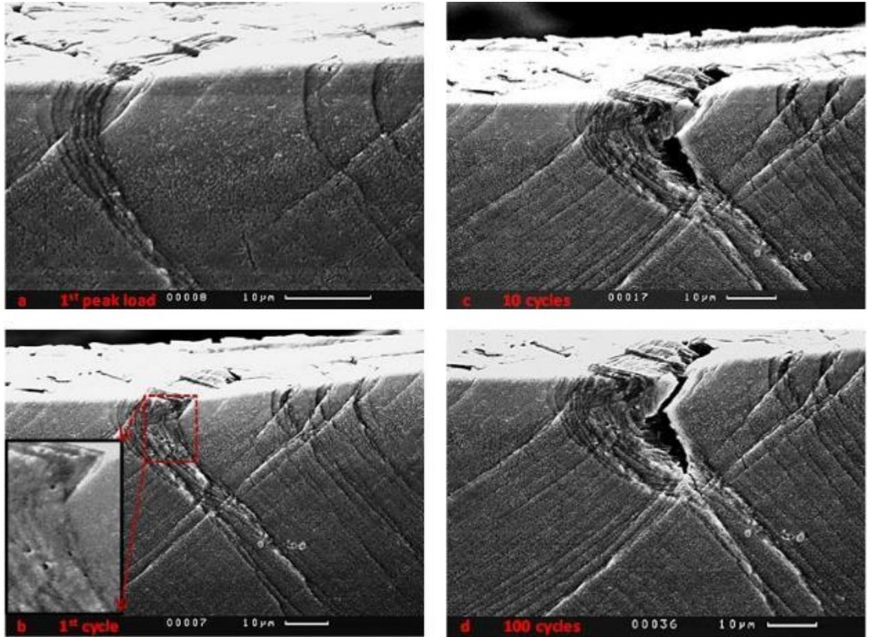
Figure 6-29. SEM images of the white-highlighted region of the EBSD map in figure 6.28 for the fully loaded condition of the specimen after: a) 1<sup>st</sup> peak load, b) 1 cycle, c) 10 cycles and d) 100 cycles.
