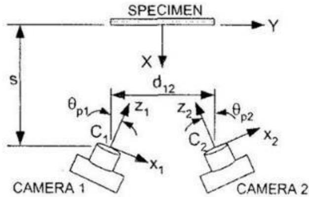
Figure 3-14. System set-up for 3D DIC.
