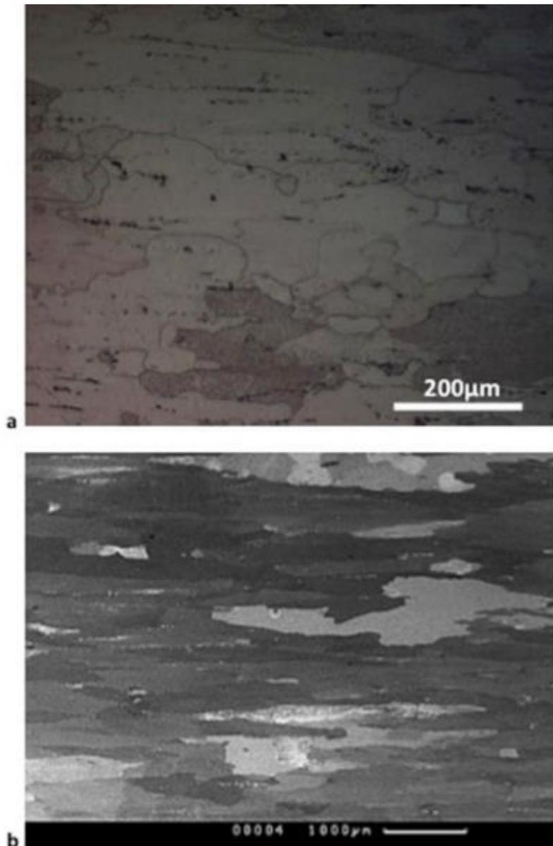
Figure 5-2. a) Optical microscopy image of the microstructure of Al2024 T3 alloy, b) low magnification SEM image for the same alloy (Al2024 T3).
