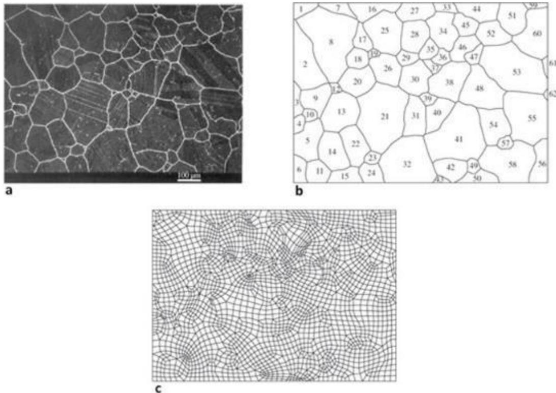
Figure 2-18 (a) A typical microstructure of the standard heat-treated C263; (b) the grain boundaries simulated; (c) a finite-element mesh for the corresponding microstructure [14].
