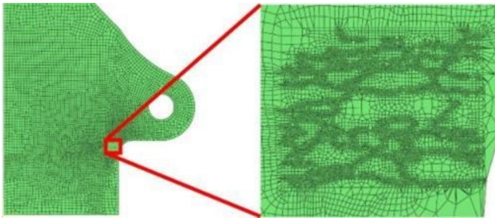
Figure 2-28. Finite element mesh of lug joint [18].
