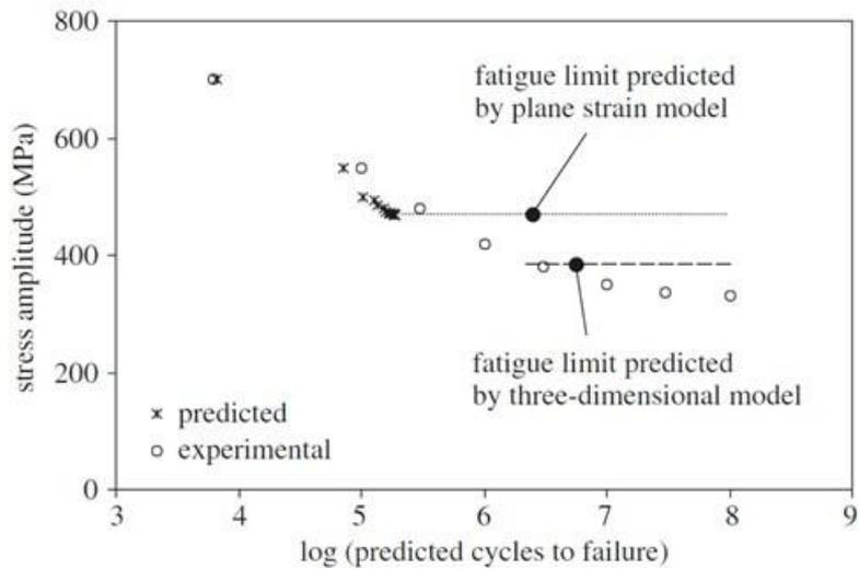
Figure 2-20. Predicted and experimental S-N curves [14].
