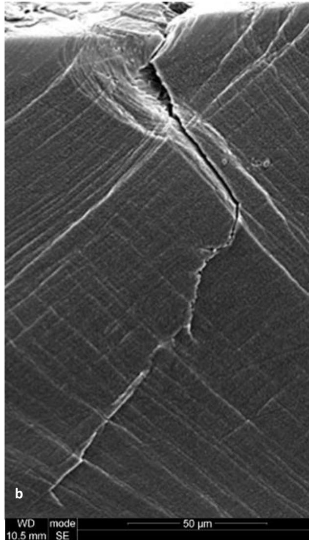
Figure 6-38. a) High magnification imaging at the location where crack initiation occurred, b) Image of the whole cracked area.
