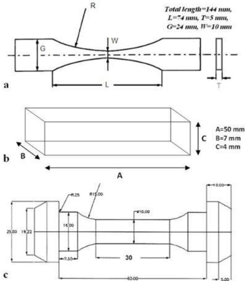
Figure 3-1. a) Specimen geometry for tensile and fatigue (tension-tension) experiments, b) for 4-point bending, and c) for fully reversed fatigue loading.
