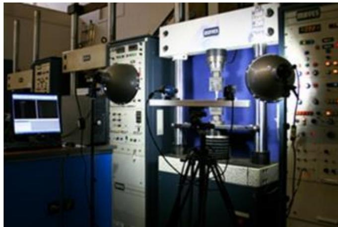
Figure 3-15. 3D DIC set-up with 2 cameras.
