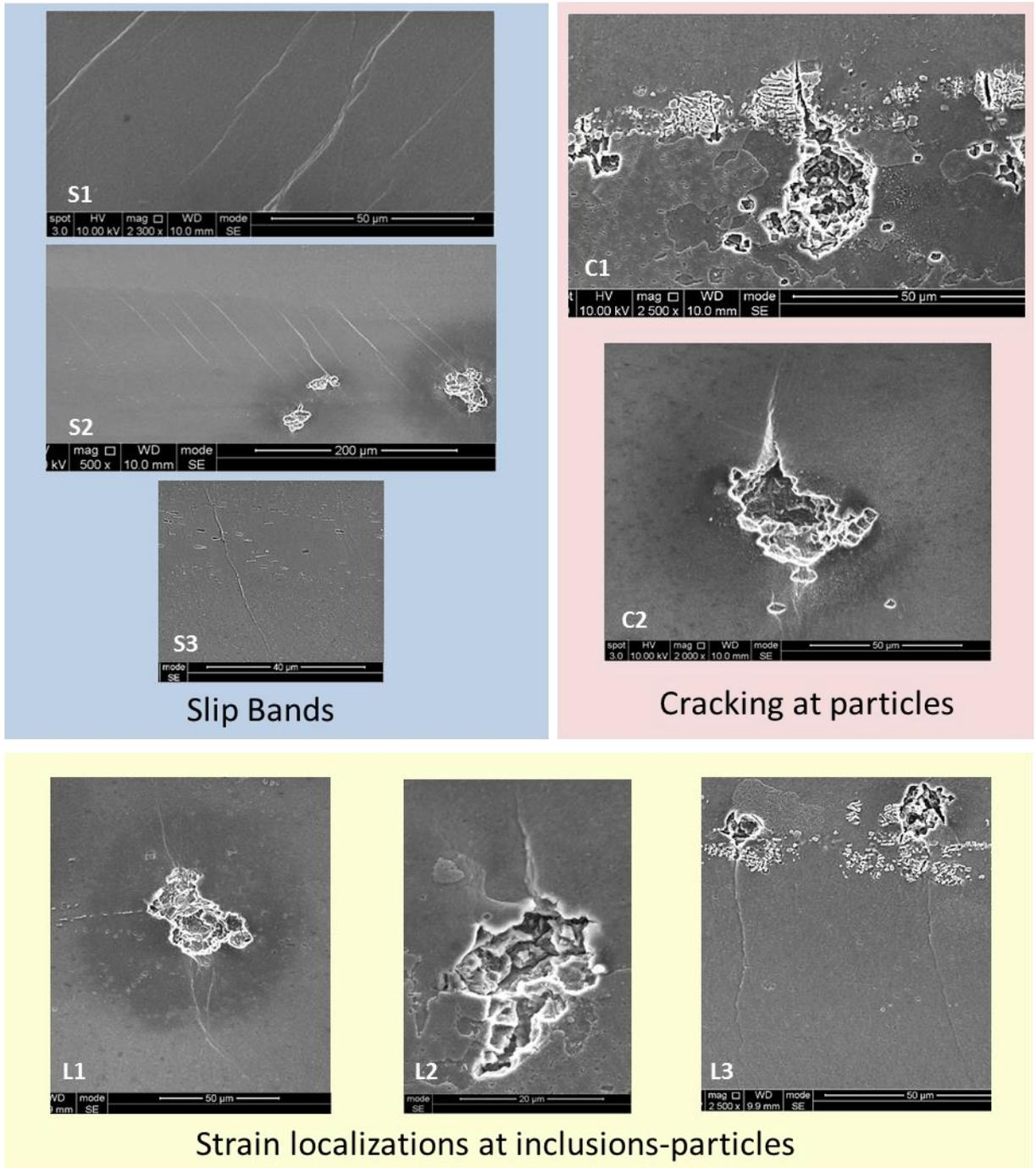
Figure 6-14. Regions where microstructural deformation was observed. S1-S3, C1-C2, and L1-L3 images correspond to the respective boxed areas in Figure 6.12b.
