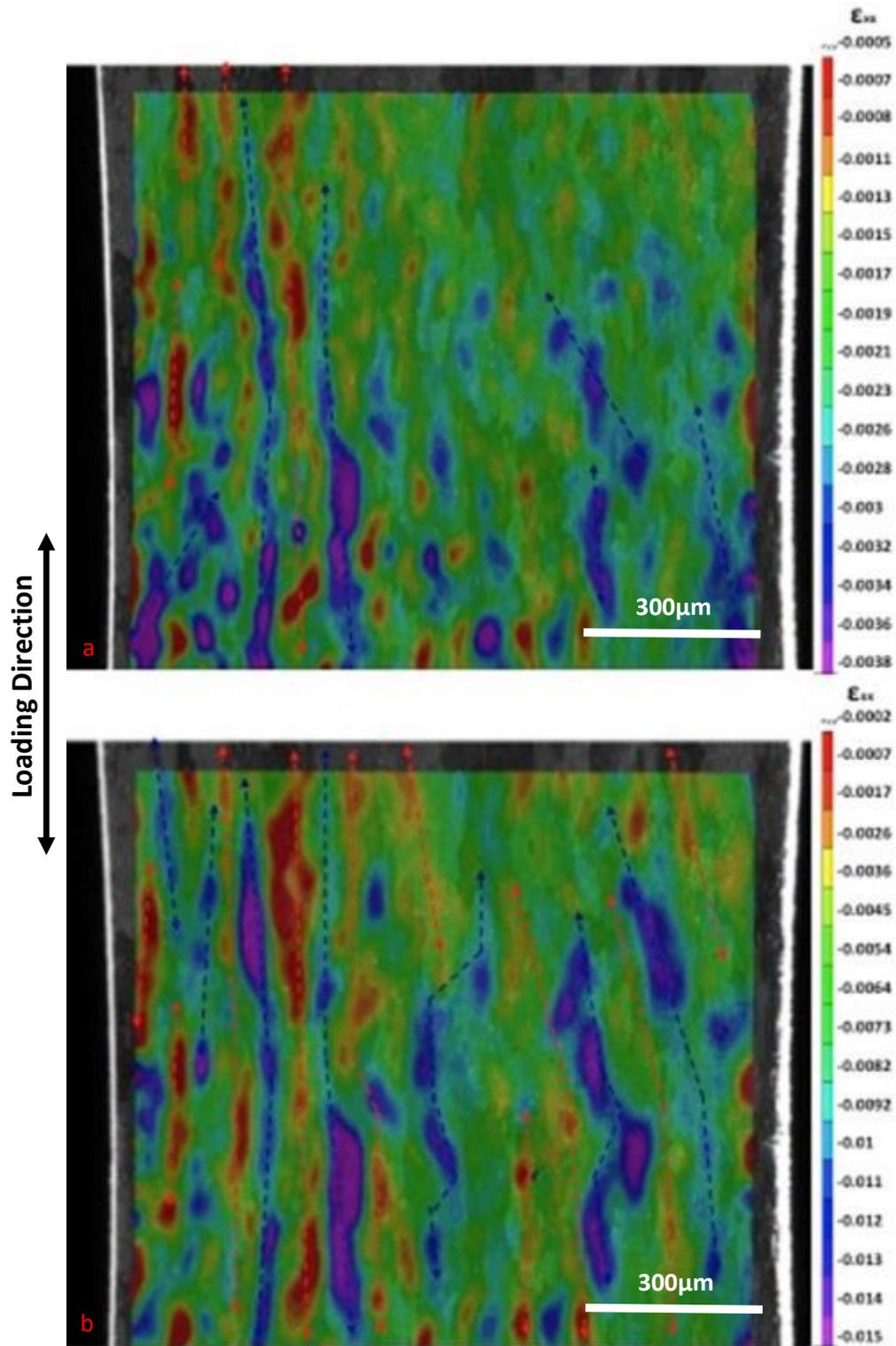
Figure 5-22. Strain distributions on the x-direction for the fully loaded sample after: a) 1 cycle, and b) 5000 cycles.
