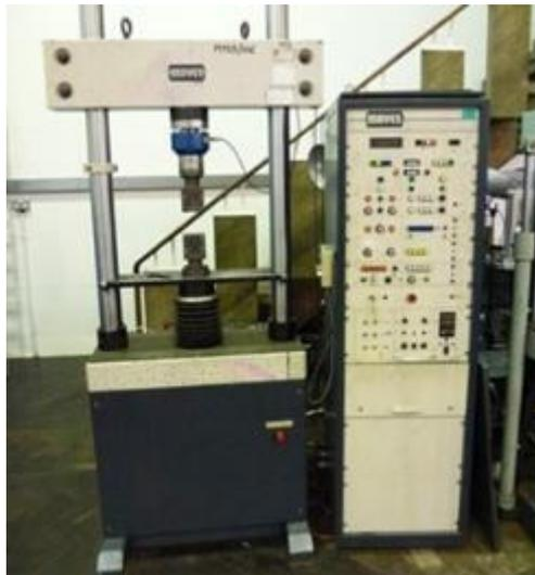
Figure 3-5. Electromechanical Mayes DM 100 tensile testing equipment.
