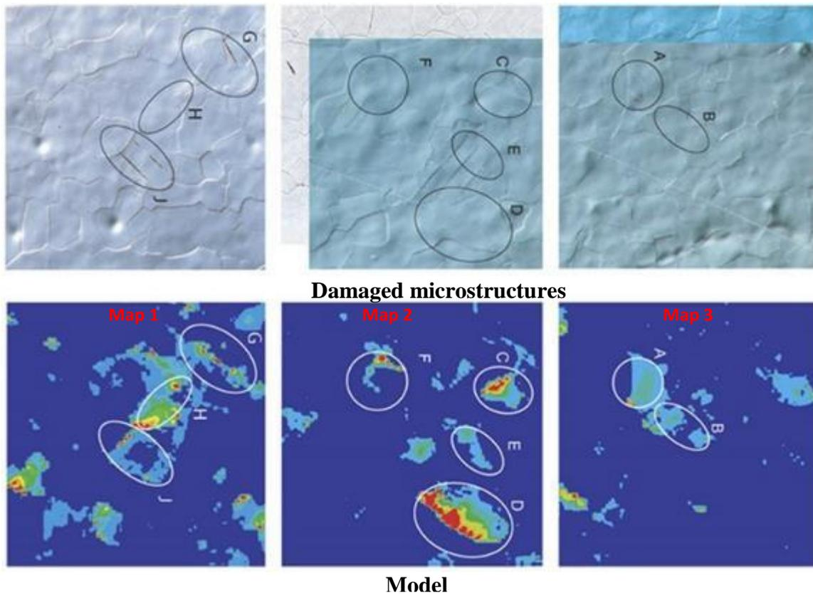
Figure 2-17. Contour plots of local energy dissipation  $E_p$  predicted in Maps 1, 2 and 3 after 143 cycles, compared with corresponding images taken after  $5 \times 10^5$  load cycles [13].
