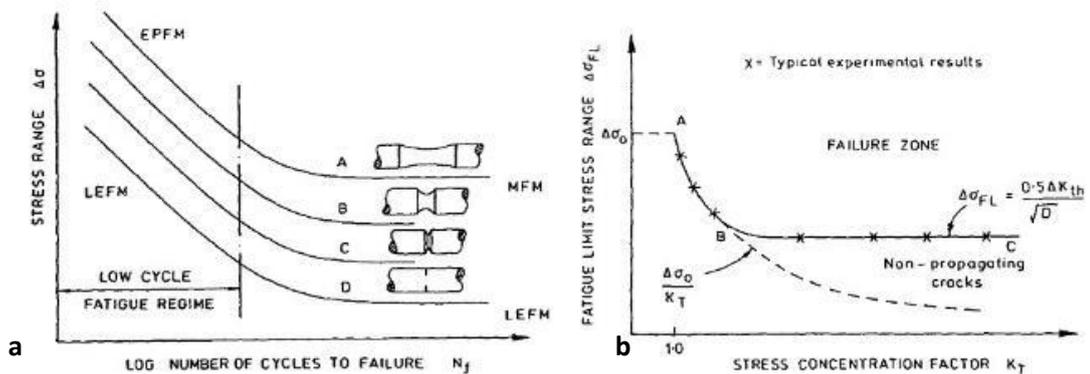
Figure 2-2. a) S-N curves for the same ferrous material but four different geometries of specimen, b) The boundary conditions between failure and non-failure of variously notched specimens A-B: the material threshold condition. B-C: the mechanical threshold condition [2].
