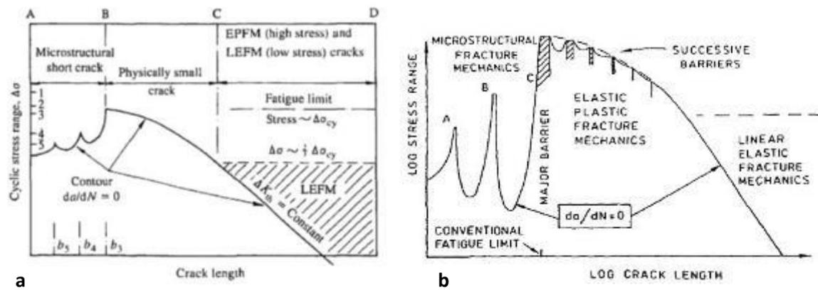
Figure 2-1. a) Regimes of fatigue life during crack formation and growth, b) highlighting the effect of grain boundaries upon crack growth [2].
