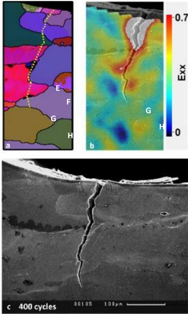
Figure 6-57. a) EBSD map of the undeformed sample with the crack path shown with yellow dotted line, b) DIC strain map at the cracked region, and c) SEM image at the cracked area, for the fully loaded condition of the specimen after 400 cycles.
