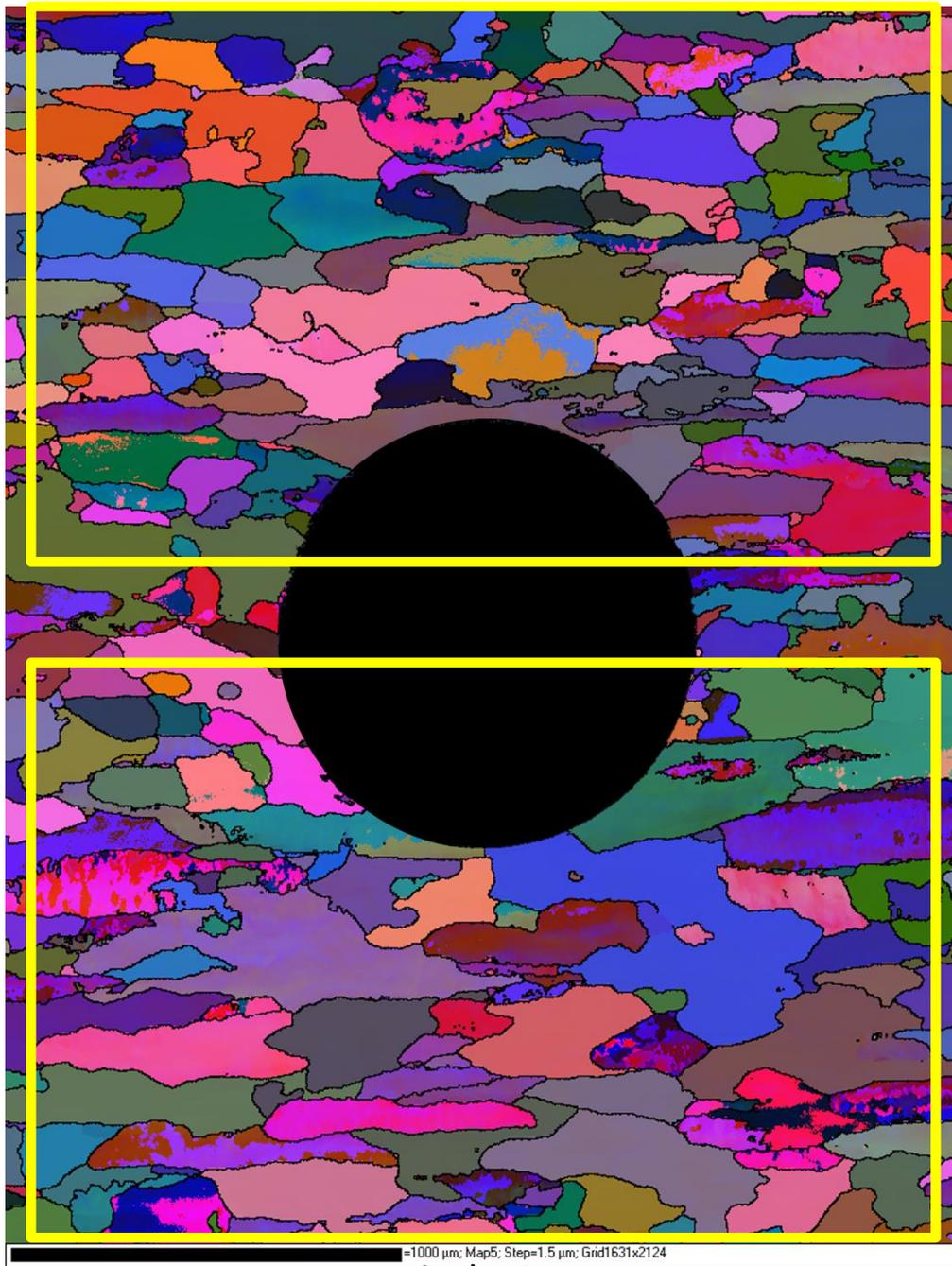
Figure 6-21. EBSD map at the region around the hole. Two highlighted regions were selected and in situ observations were made during micro-bending.
