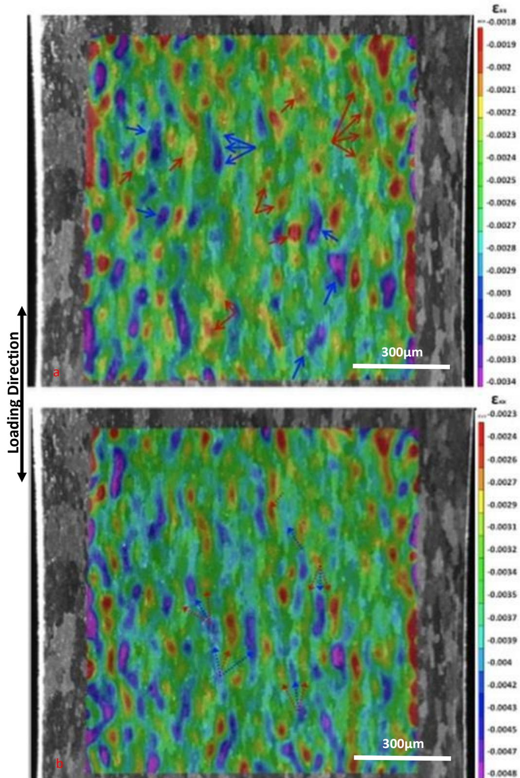
Figure 5-18. Strain distributions on the x-direction for the fully loaded sample after: a) 1 cycle, and b) 30000 cycles.
