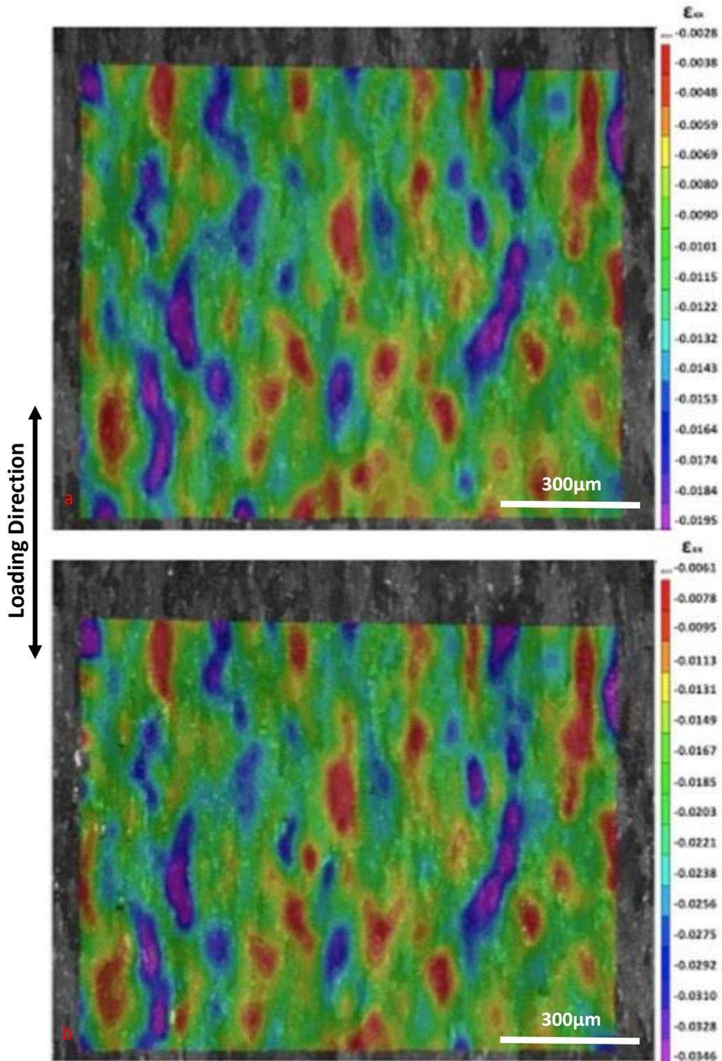
Figure 5-26. Strain distributions on the x-direction for the fully loaded sample after: a) 1 cycle, and b) 5000 cycles.
