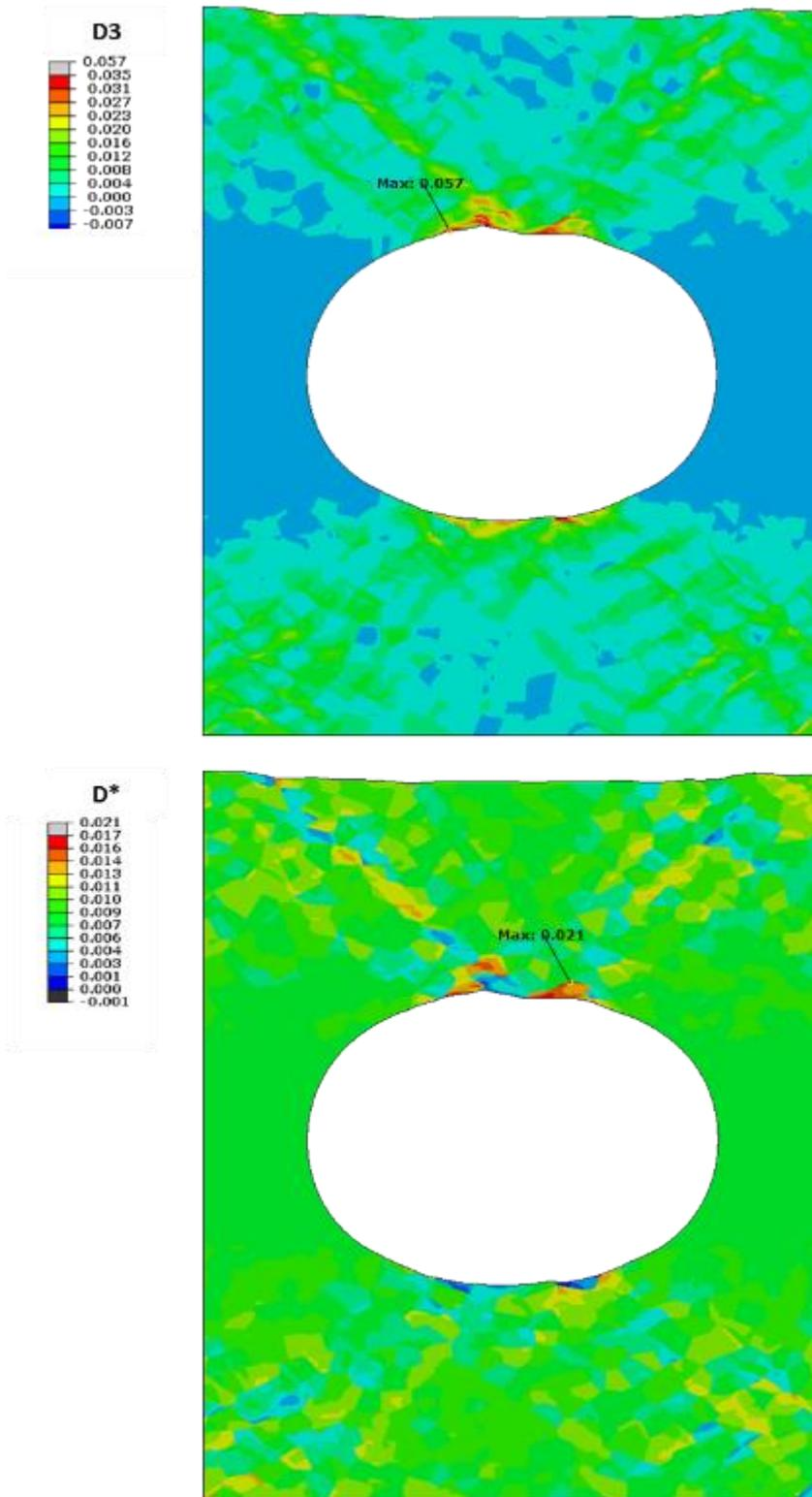
Figure 7-11. Deformed microstructure after 1 cycle for an applied strain of 0.01. a) The contours show the variations of the: a) D3 metric and b) the FIP introduced.
