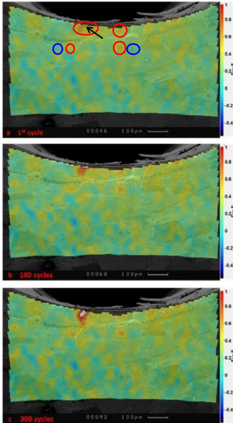
Figure 6-52. Strain distributions for the fully loaded sample after: a) 1, b) 100 and c) 300 cycles.
