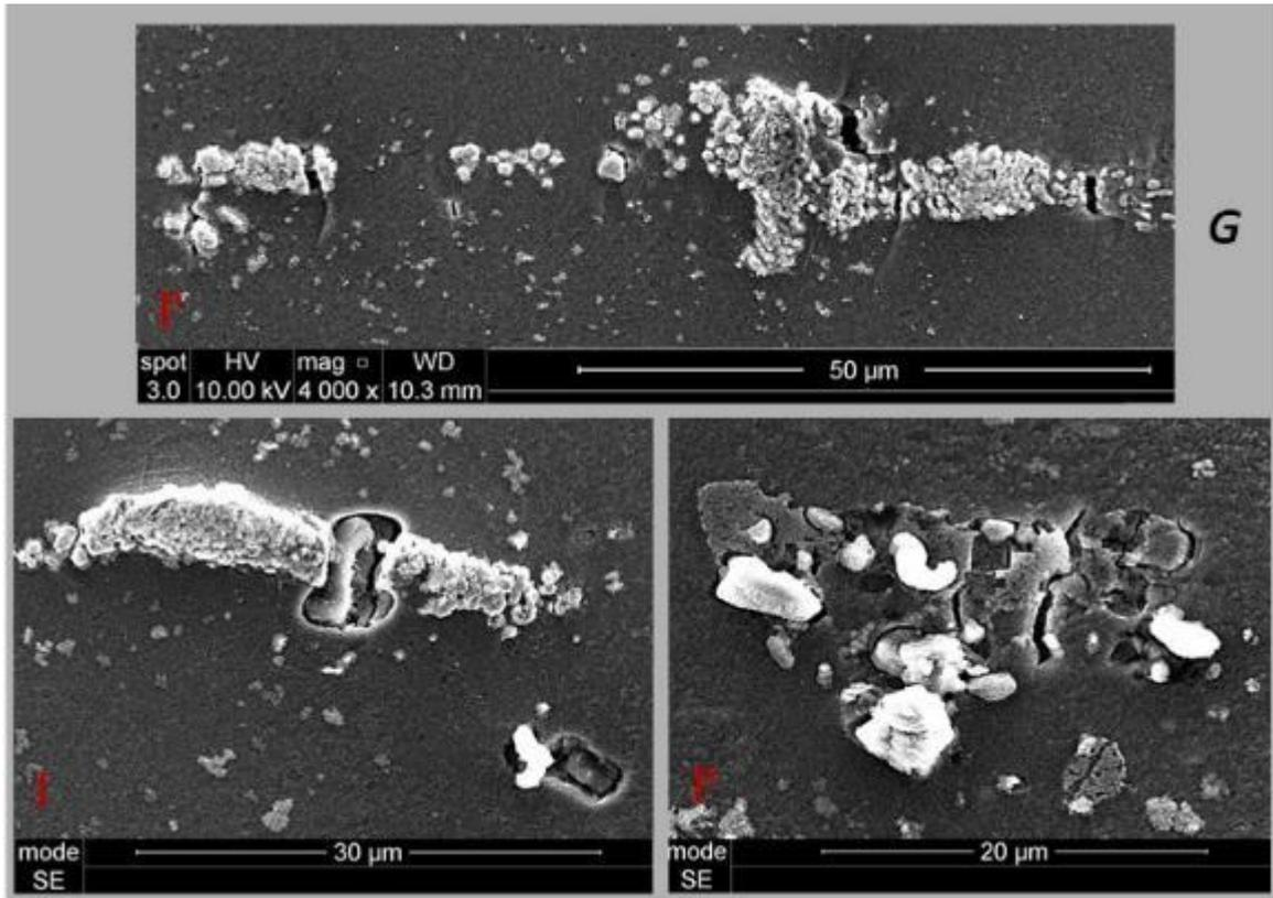
Figure 6-8. a - g) SEM images at the corresponding regions of figure 6.3a. The regions show plastic localisations as well as damage in the neighbourhood of particles and inclusions.
