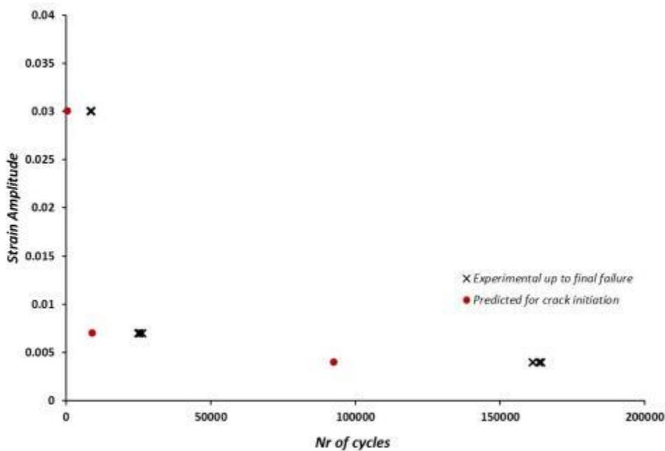
Figure 7-16. S-N curve for the material studies. Comparison between the total fatigue lifetime experimental results (number of cycles up to failure) and the modelling predicted values for the FCI period (number of cycles up to the point where FCI occurs).
