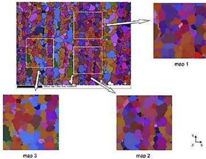
Figure 2-16. Digitally constructed microstructures, labelled Maps 1, 2 and 3, using 100x100 finite-elements for sub-modelling, based on the experimentally derived EBSD image [13].
