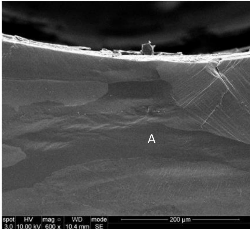
Figure A2. A 'weak' grain deflecting the crack towards its' matrix.
