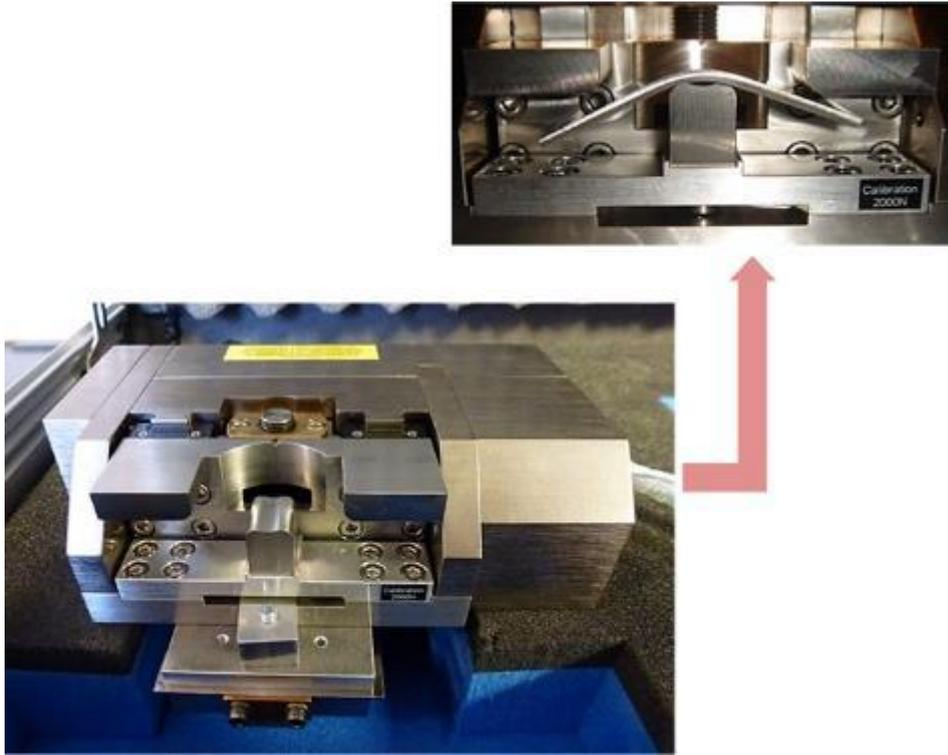
Figure 3-7. Deben vertical bending equipment
