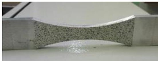
Figure 3-13. The sample after spraying with white and black paints.
