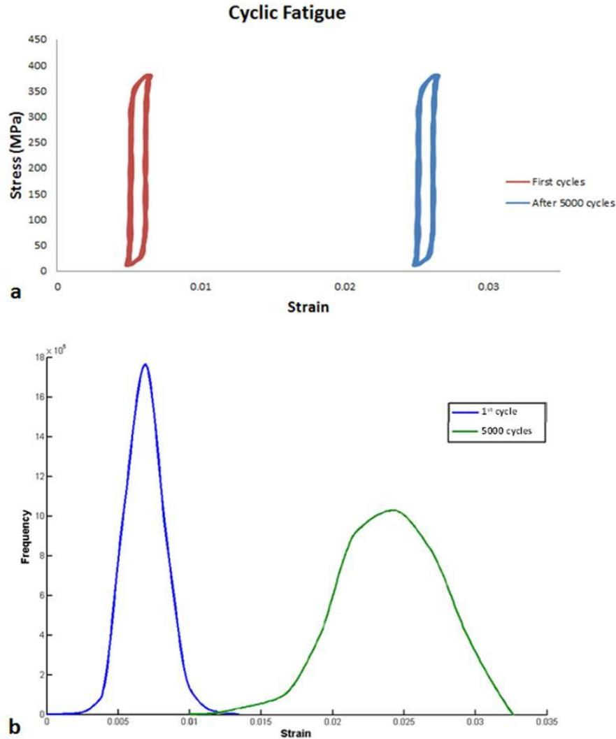
Figure 5-21. a) Stress-strain curves output from the testing machine, b) Strain distributions measured by means of DIC at maximum displacement ( $1.02\sigma_y$  and initial applied strain 0.007) after 1, and 5000 cycles.
