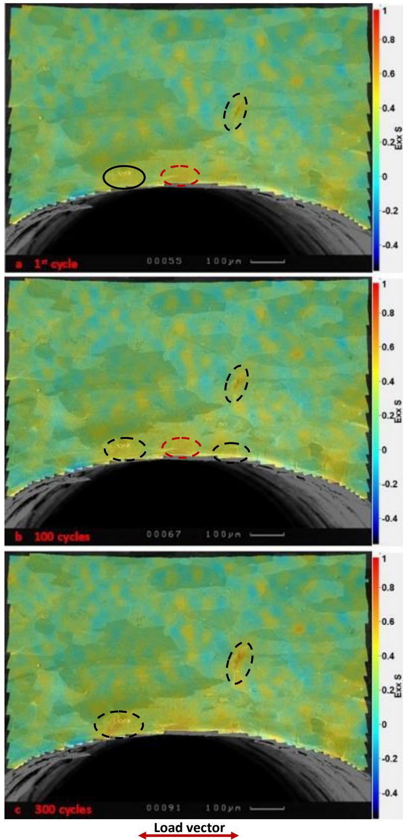
Figure 6-45. Strain distributions for the fully loaded sample after: a) 1, b) 100 and c) 300 cycles. No macroscopic strain accumulation was observed.
