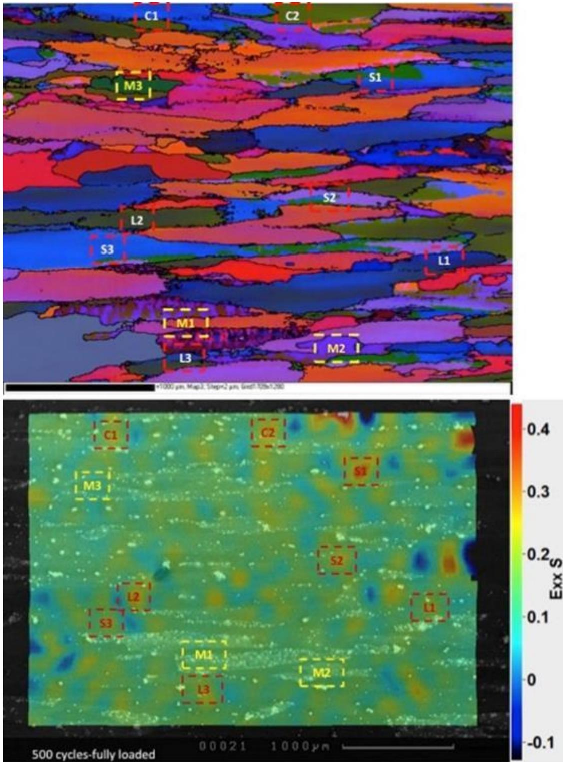
Figure 6-12. a) EBSD measurements and b) strain distributions of the same area after 500 cycles. The boxed areas were inspected with high resolution SEM to check for the occurring microstructural deformation.
