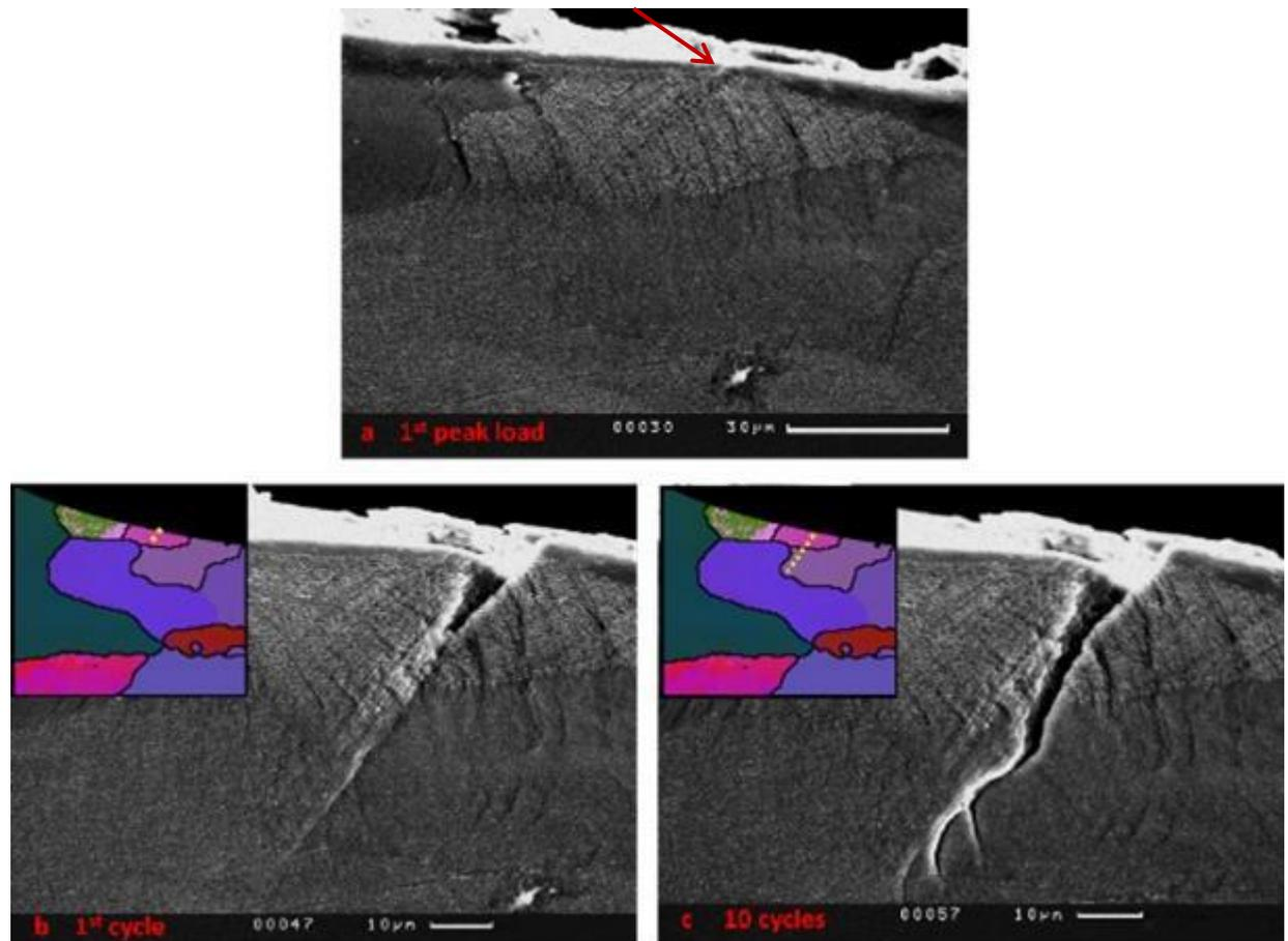
Figure 6-54. SEM images at the black arrowed region of figure 6.52a, for the fully loaded condition of the specimen after: a) 1<sup>st</sup> peak load, b) 1 cycle and c) 10 cycles.
