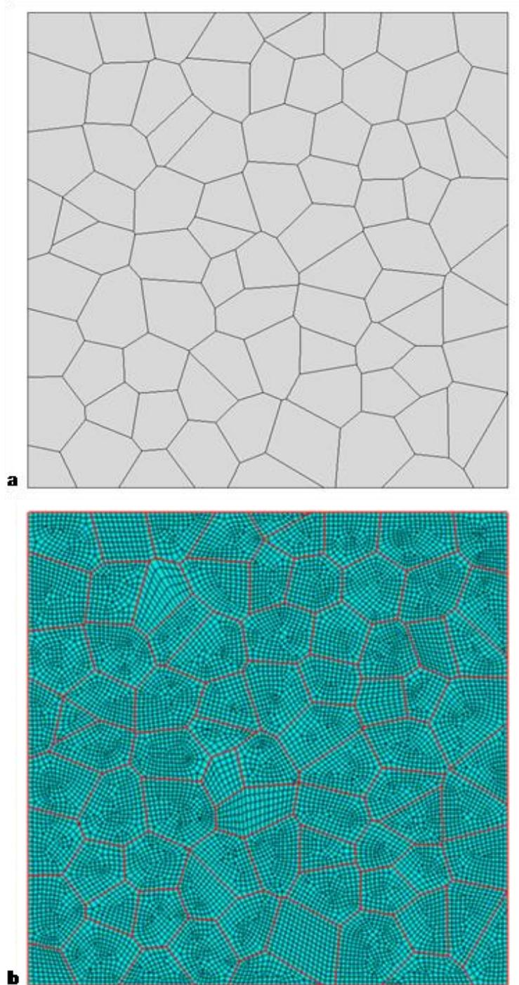
Figure 7-4. a) The created geometry for the 2-D RVE, and b) the meshed part.
