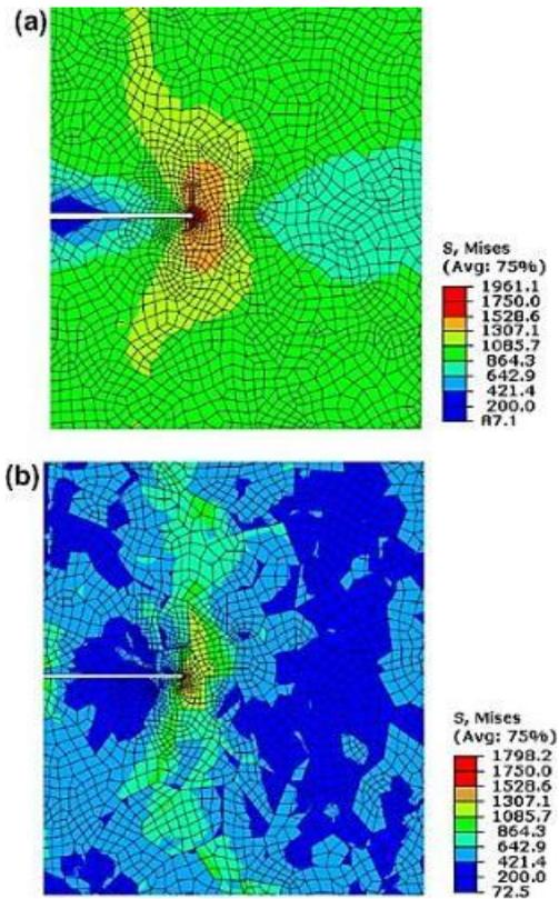
Figure 2-37. Contour plots of the von Mises stress obtained from the FE analyses using (a) crystal plasticity and (b) viscoplasticity model [28].
