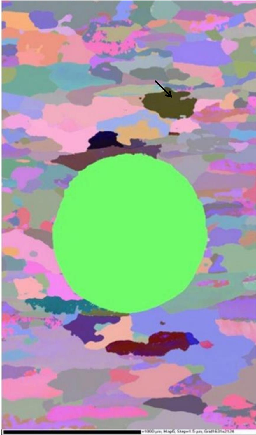
Figure 6-35. The highlighted grains correspond to 'hard' grains, showing uniform matrix deformation without slip bands observed. While the arrowed grain correspond to the grain circled in figure 6-37.
