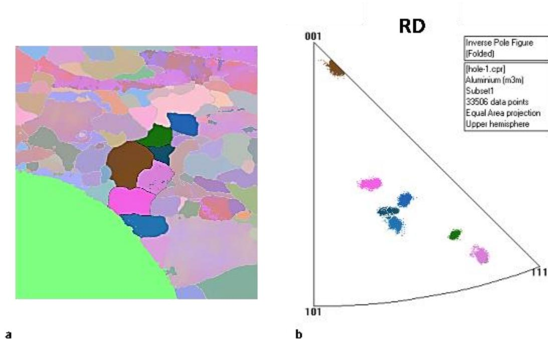
Figure 6-65. Texture components at the location where the deformation band formed in figures 6.45 and 6.46.
