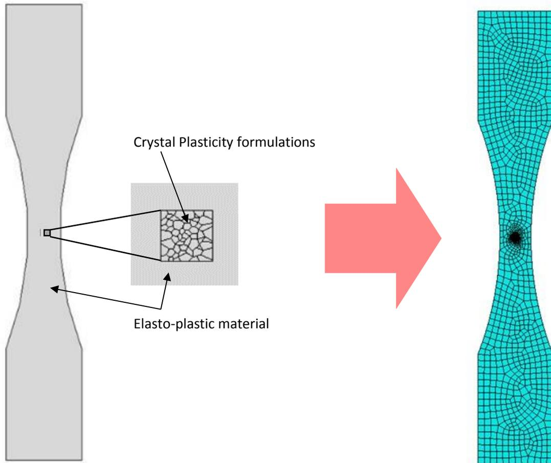
Figure 7-17. Multiscale approach for a tensile specimen
