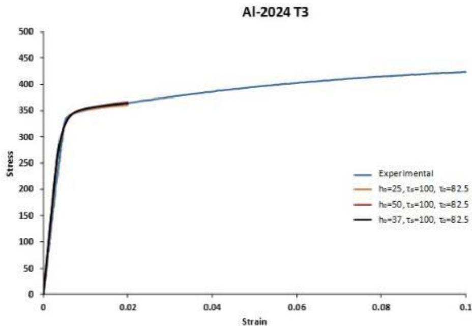
Figure 7-5. Comparison between modelling and experimental results for Al2024 for strain up to 0.02.
