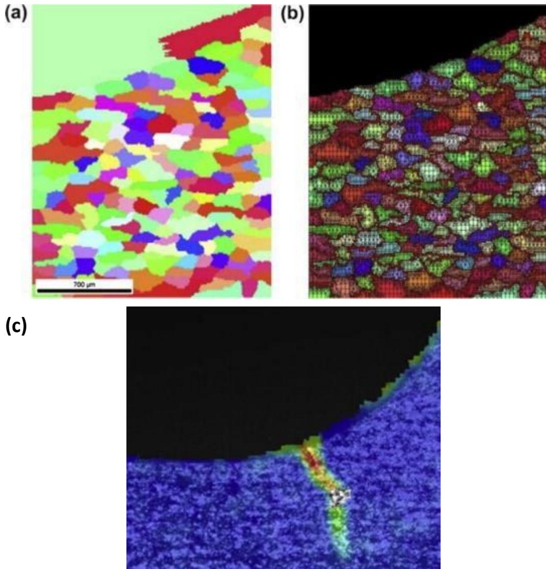
Figure 2-32. a) EBSD scan directly at the lug joint, b) Meshed geometry, and c) experimentally observed crack propagation for the same geometry as in a and b [18].
