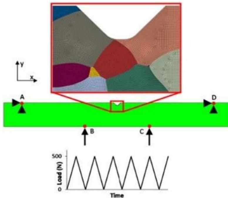
Figure 2-22. The BCs are shown on the sample, the loading conditions, and the meshed geometry at the edge of the notch [15].
