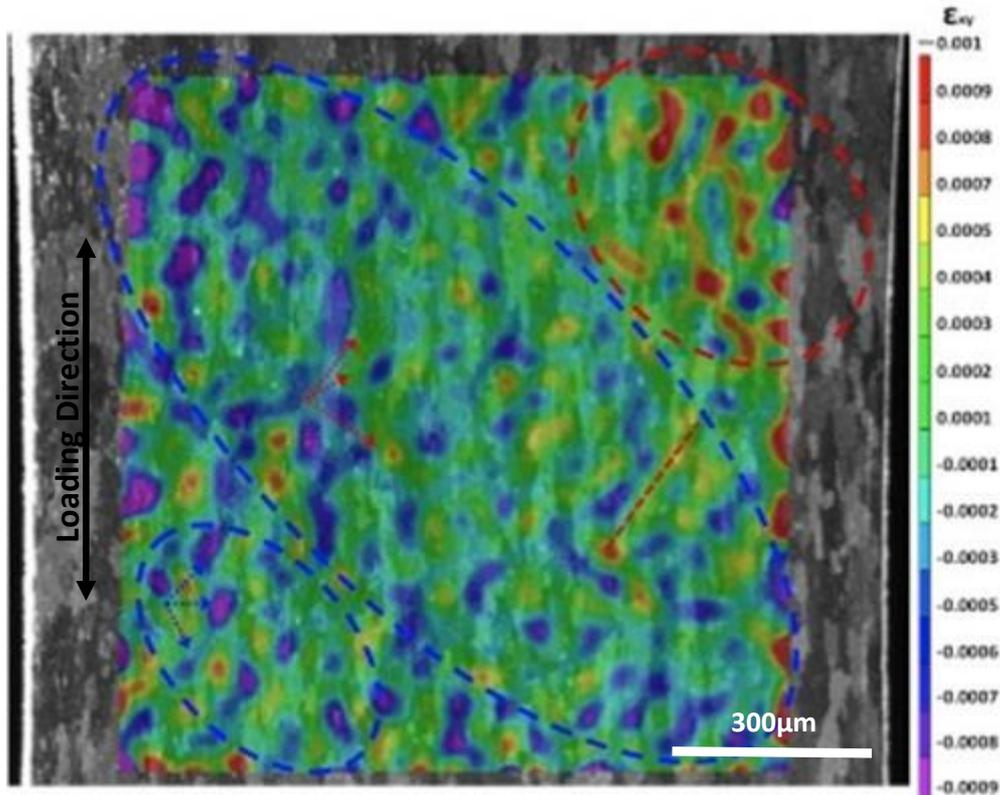
Figure 5-19. Shear strain distribution for the fully loaded sample after 30000 cycles.
