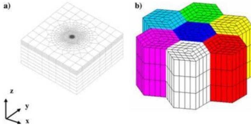
Figure 2-11. a) The global mesh and b) the mesh of the surface aggregate containing seven prismatic grains.
