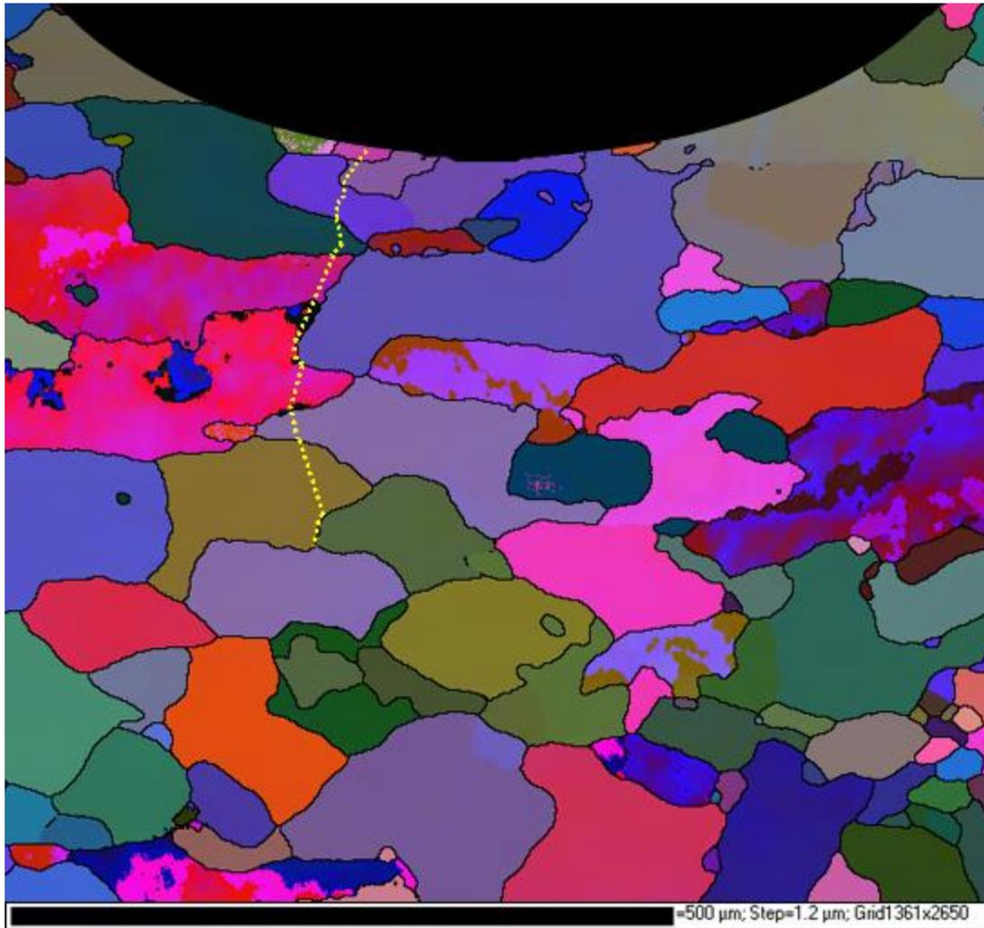
Figure 6-59. EBSD map of the lower part of the map shown in figure 6.43, with the crack path shown with yellow dotted line. The crack corresponds to the failure that occurred after 700 cycles.
