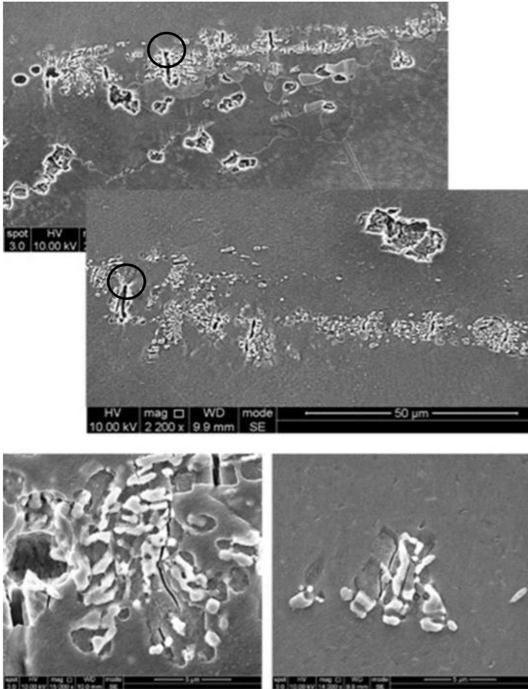
Figure 6-17. Cracks within clusters of particles.
