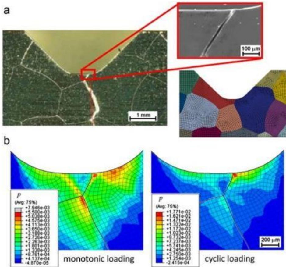
Figure 2-23. (a) Images of crack path for specimen 1 along with the FE mesh in the notch region, together with predicted field variations for specimen 1 of (b) effective plastic strain,  $p$ . Plots are provided for full load after monotonic loading and full load after cyclic loading as indicated [15].
