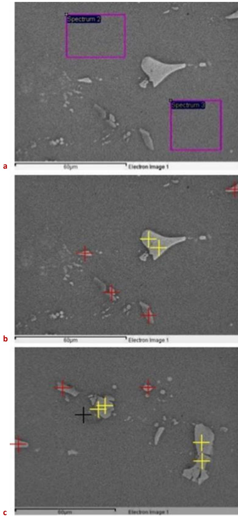
Figure 5-8. a-c) Chemical composition spectrums and spot analysis at various locations highlighted with crosses and boxes.
