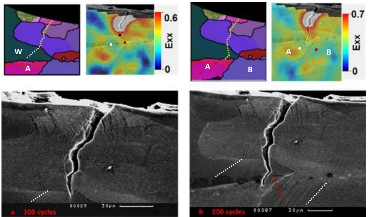
Figure 6-55. SEM images at the black arrowed region of figure 6.52a, for the fully loaded condition of the specimen after: a) 100 cycles and c) 200 cycles.
