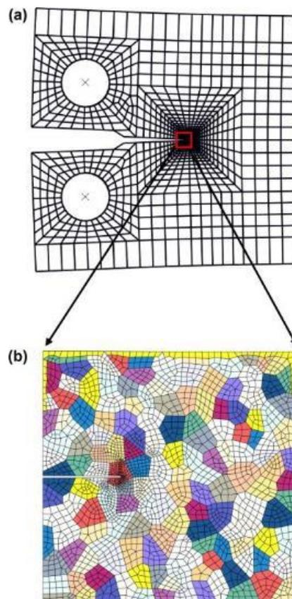
Figure 2-36. Global finite element model for the CT specimen; (b) a 150-grain submodel with crack introduced across a couple of grains (mesh size near the crack tip is  $\sim 0.20 \mu\text{m}$ ) [28].
