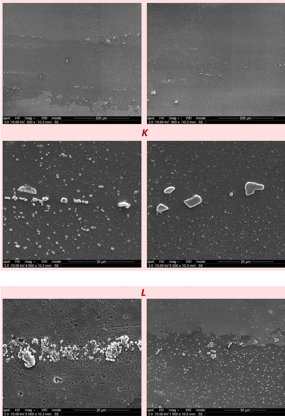
Figure 6-9. h, i, j, k and l) SEM images at the corresponding regions of figure 6.8a. The regions show minimum matrix deformation, absence of plastic localizations, and intact particles.
