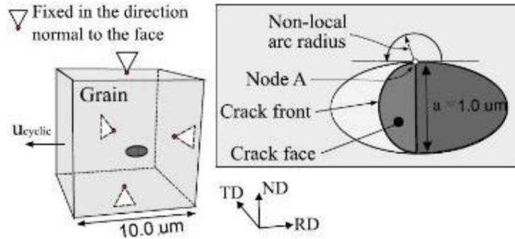
Figure 2-44 Single grain with embedded particle baseline model configuration [45].
