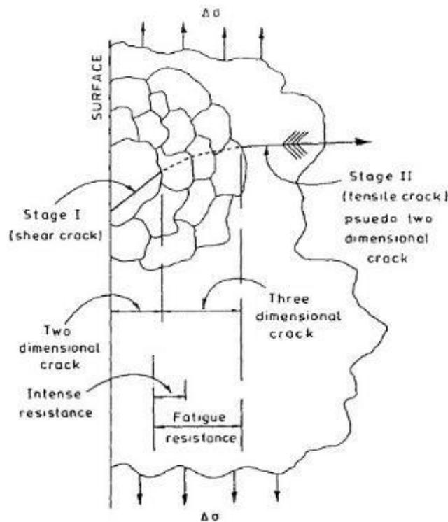
Figure 2-5. Fatigue resistance indicated in terms of the difficulty of an initial Stage I shear crack becoming a Stage II tensile crack [3].
