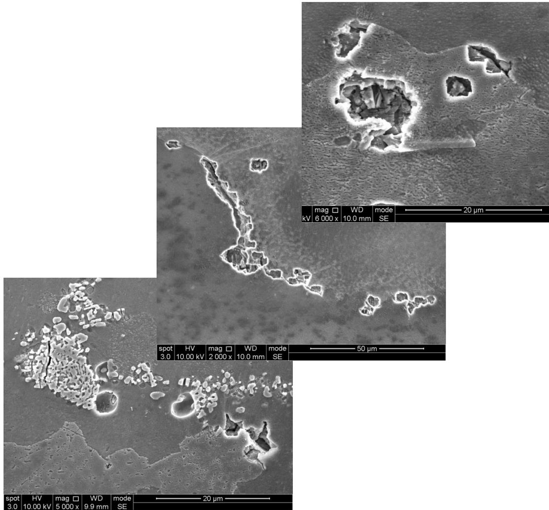
Figure 6-15. Grain boundary decohesions due to segregation of impurities in the vicinity of GBs.
