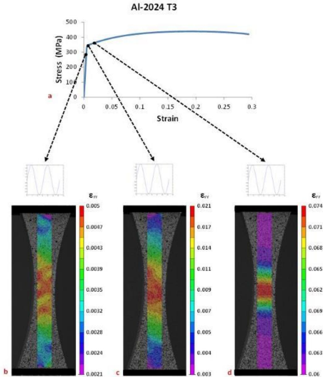
Figure 5-13. a) The stress-strain curve obtained by tensile testing. The  $\epsilon_{yy}$  strain distributions for 3 samples cyclically loaded ( $R=0$ ) at different stress amplitudes: b) 0.75 $\sigma_y$  and after 30000 cycles, c) 1.02 $\sigma_y$  and after 5000 cycles and d) 1.11 $\sigma_y$  and after 5000 cycles. The sinusoidal graphs are shown just schematically.
