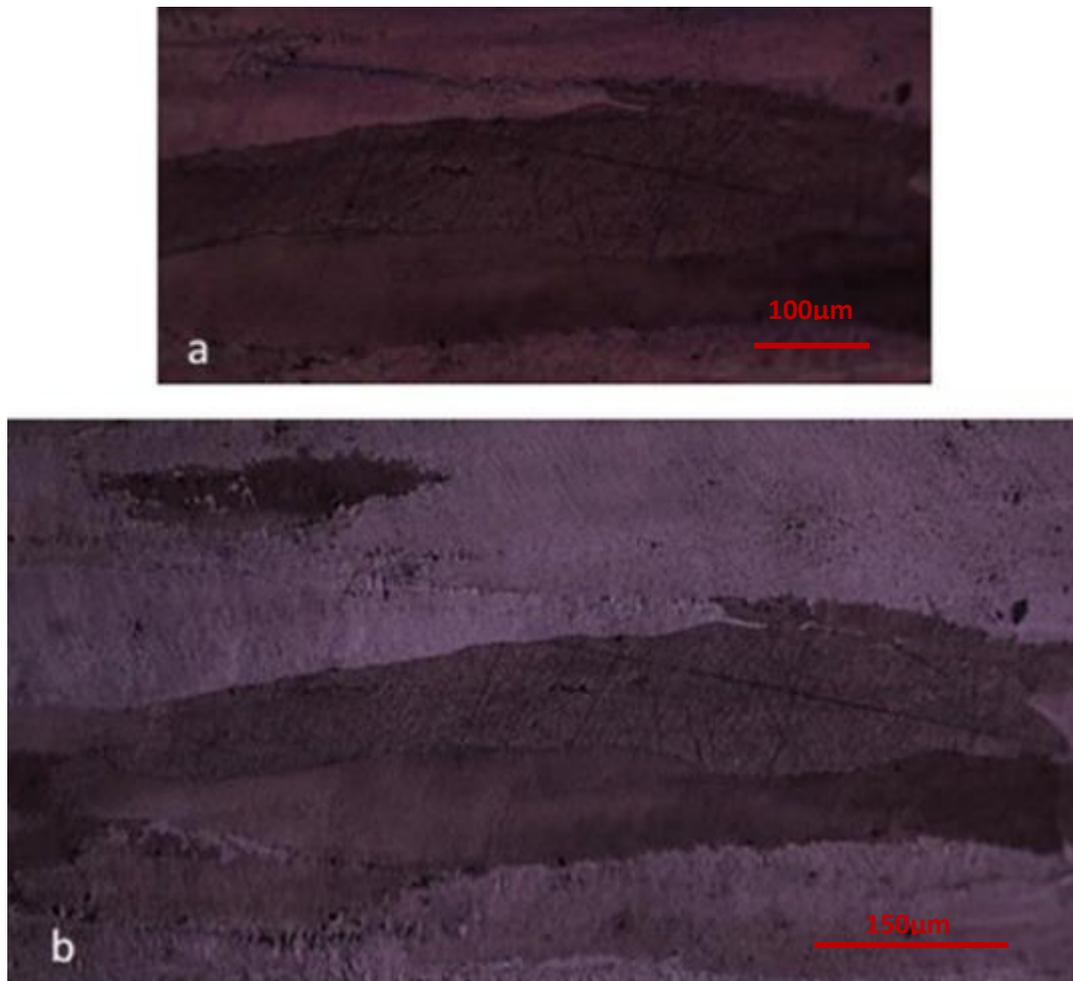
Figure 6-6. High magnification optical microscopy images from area J in Figure 6.3a. a) DIC (Differential Interference Contrast) microscopy image to indicate the presence of negligible out of plane deformation, and b) Optical microscopy image at the same area.
