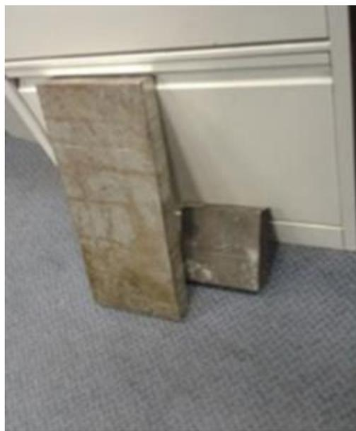
Figure 5-1. Slab of Al2024 T3, provided by ALCAN.
