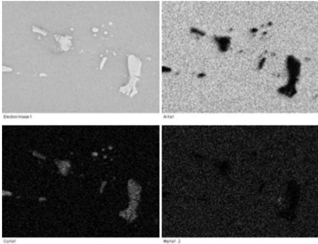
Figure 5-7. Chemical composition map at a location of containing large particles. The spot size was 3nm with the particle size varying from 2 micron up to 50 micron.
