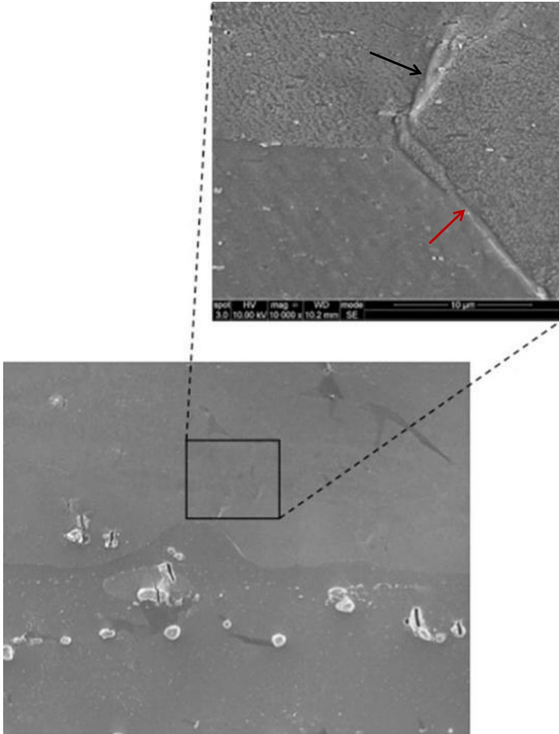
Figure 6-16. Grain boundary sliding and slip band formation in the matrix.
