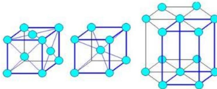
Figure 4-7. Three basic crystal structures; FCC, BCC, HCP.
