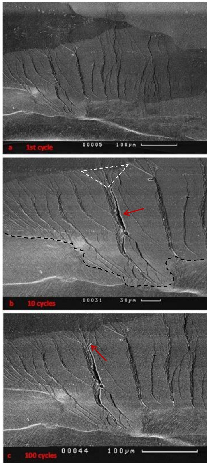
Figure 6-24. SEM images of the highlighted grain of figure 6.23a for the fully loaded condition of the specimen after: a) 1 cycles, b) 10 cycles and c) 100 cycles.
