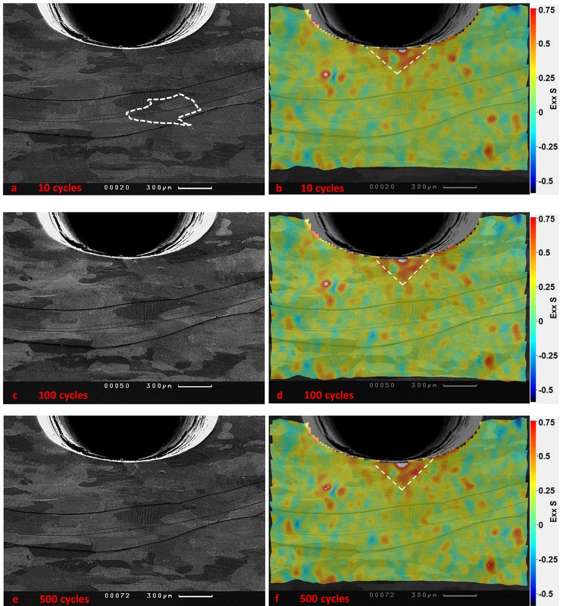
Figure 6-27. SEM images at the same region of the sample with figure 6.26 for the fully loaded condition of the specimen after: a) 10 cycles, c) 100 cycles and e) 500 cycles. Strain distributions for the fully loaded sample after: b) 10 cycles, d) 100 cycles and f) 500 cycles.
