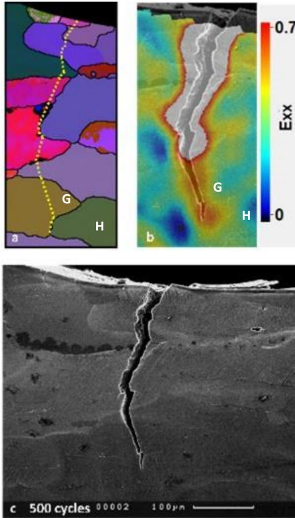
Figure 6-58. a) EBSD map of the undeformed sample with the crack path shown with yellow dotted line, b) DIC strain map at the cracked region, and c) SEM image at the cracked area, for the fully loaded condition of the specimen after 500 cycles.
