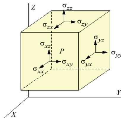
Figure 4-1. Definition of stress components on an infinitesimal volume element.
