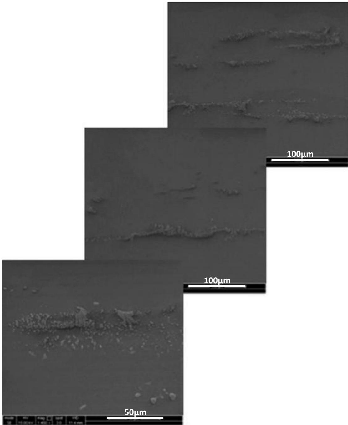
Figure 5-5. Clusters of particles in un-etched Al2024 T3 sample. The length scale in figure 5-5 is 100µm, 100µm and 50µm.
