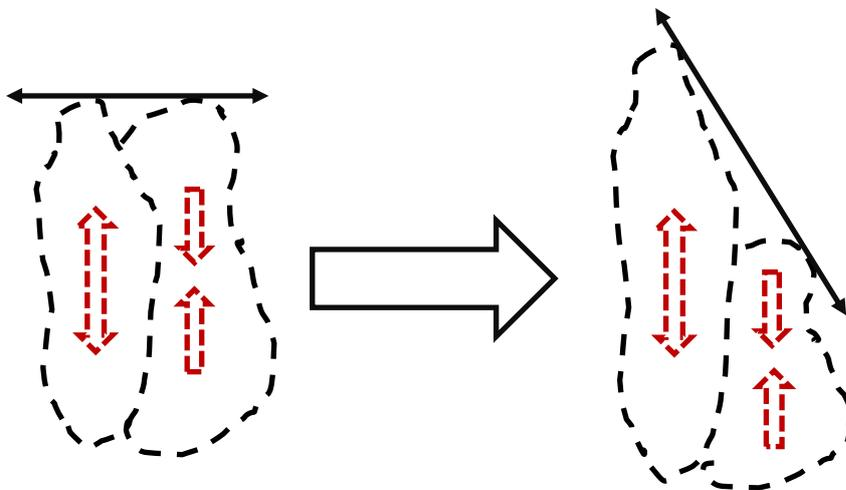
Figure 5-28. Schematic representation of shape changes in two grains for which one of them is under tension and the other under compression.
