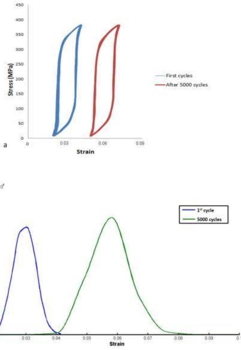
Figure 5-25. a) Stress-strain curves output from the testing machine, b) Strain distributions measured by means of DIC at maximum displacement ( $1.11\sigma$ , and initial applied strain 0.03) after 1 cycle (blue line), and after 5000 cycles (green line).
