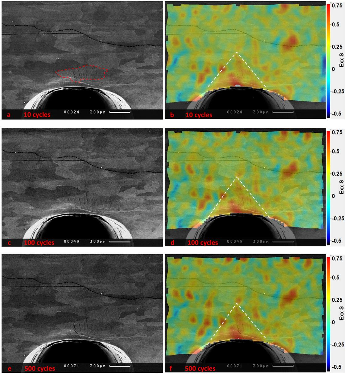
Figure 6-23. SEM images of the same region of the sample as in figure 6.22 for the fully loaded condition of the specimen after: a) 10 cycles, c) 100 cycles and e) 500 cycles. Strain distributions for the fully loaded sample after: b) 10 cycles, d) 100 cycles and f) 500 cycles.
