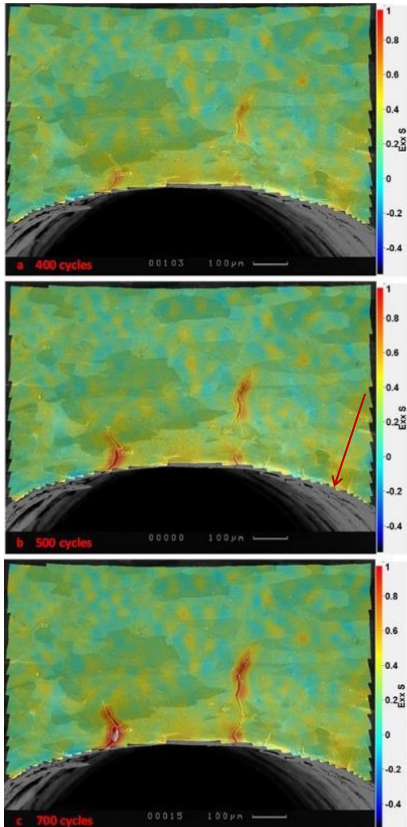
Figure 6-46. Strain distributions for the fully loaded sample after: a) 400, b) 500 and c) 700 cycles.
