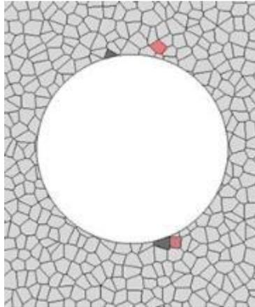
Figure 7-12. Predicted location for damage initiation by using the D3 metric (grey grains), and by using the FIP criterion (light red coloured grains).
