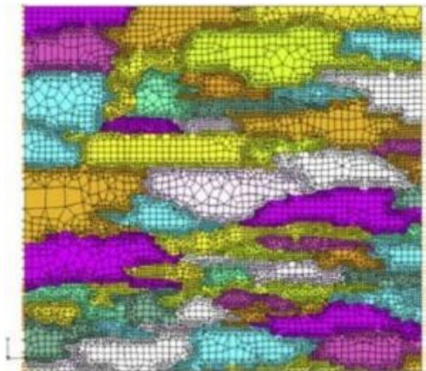
Figure 2-27. Meso RVE containing different oriented grains [18].
