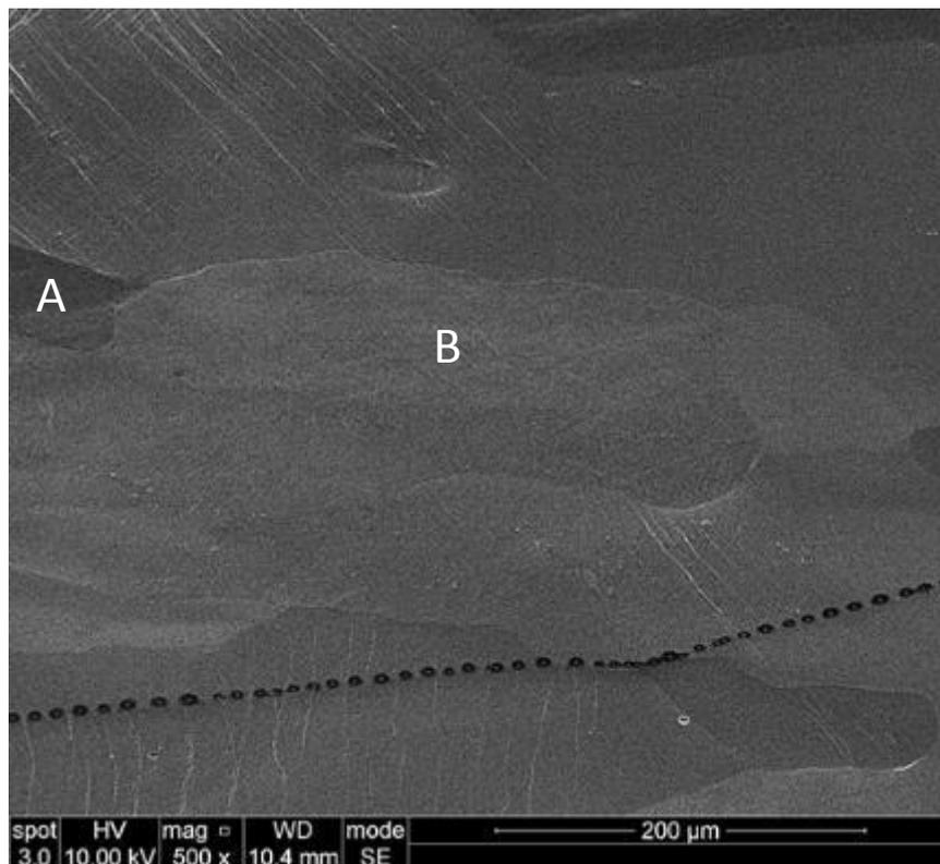
Figure A1. A hard grain in between highly deformed 'weak' grains.
