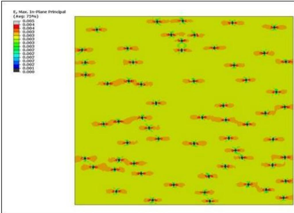
Figure 7-14. Deformed body after a 3% displacement. The contours show the variations of Von Mises stresses.
