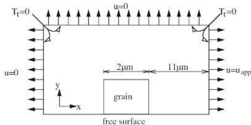
Figure 2.7. a) Boundary conditions and model, b) The single grain inside of which dislocation dynamics is applied; the surrounding material is elastic. The grain has three slip systems [7].
