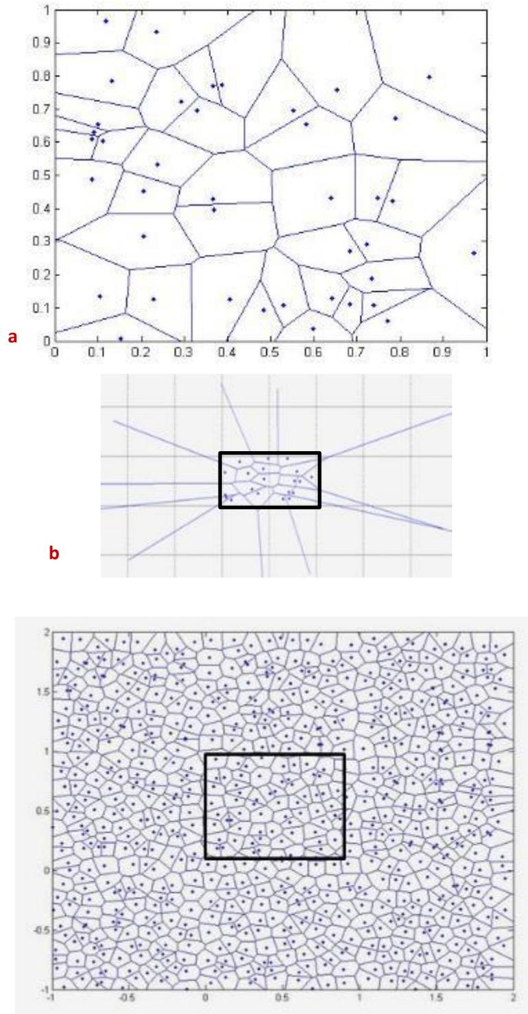
Figure 4-14. a) Simple case of a 2D Voronoi diagram for the case of 20 randomly centred polyhedra, b) clarifying the unclosed polygons and the problem with some vertices extending to infinity, and c) creating a square domain within a region.
