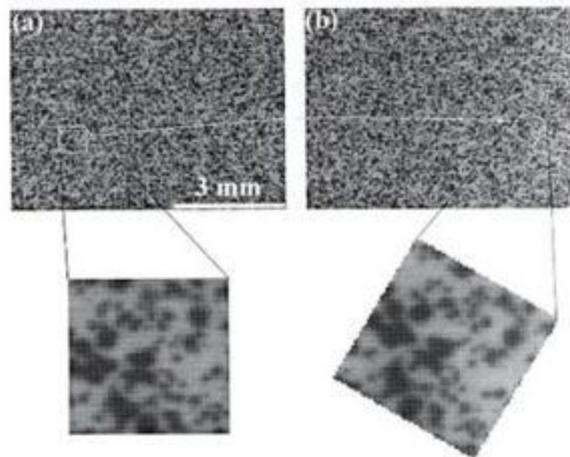
Figure 3-12. Speckle patterns for DIC image processing.
