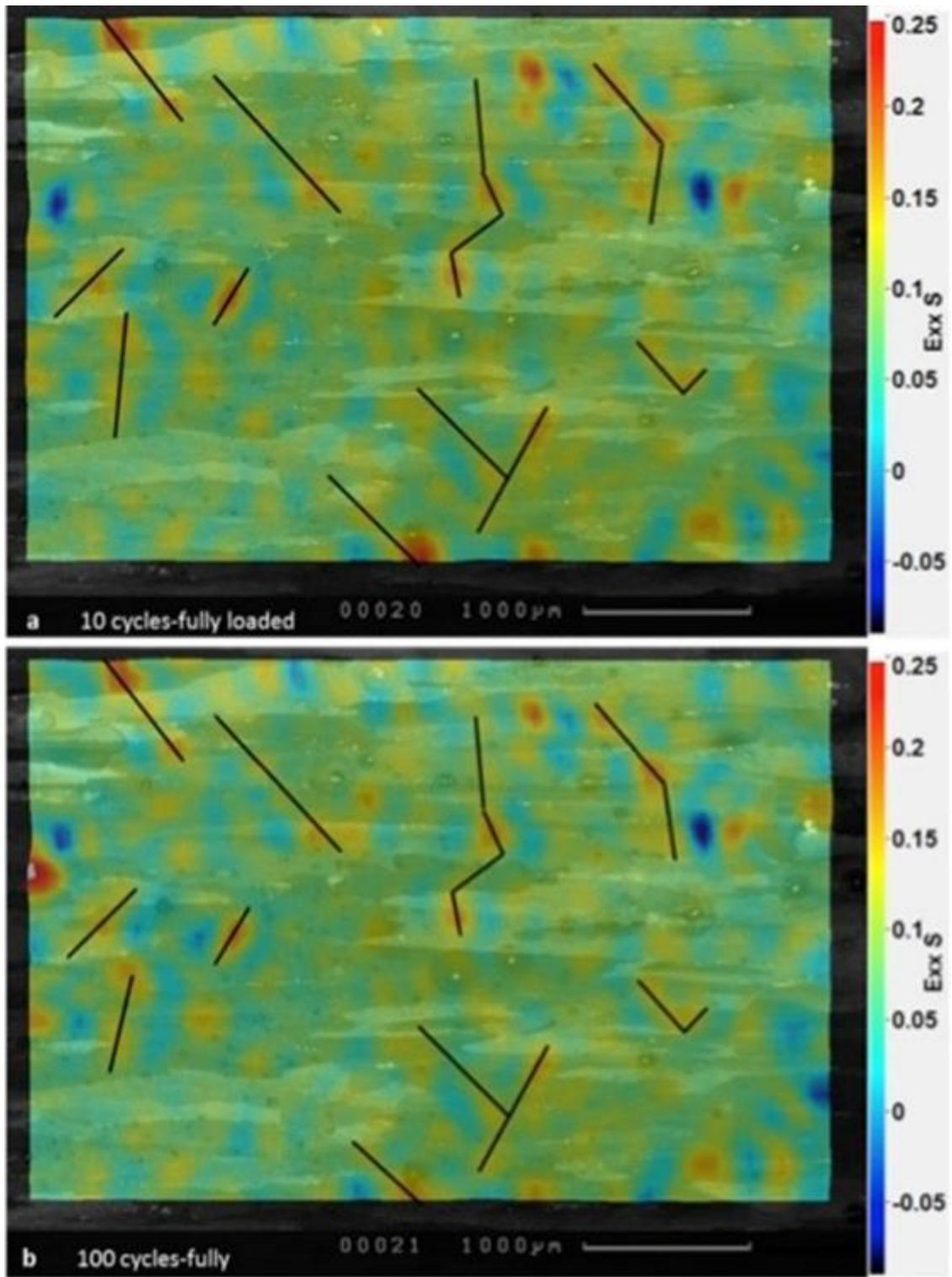
Figure 6-2. a) Strain distribution for the fully loaded sample after a) 10 cycles and b) 100 cycles. No macroscopic strain accumulation was observed.
