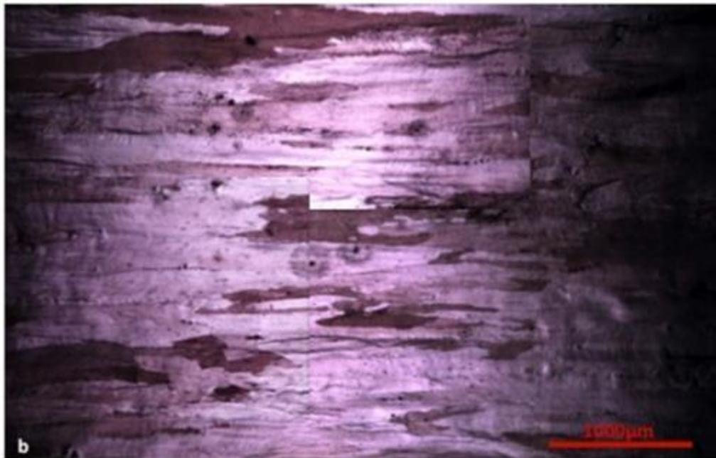
Figure 6-3. a) Strain distribution for the fully loaded sample after 500 cycles, b) optical microscopy image at the same region after 500 cycles (unloaded condition).
