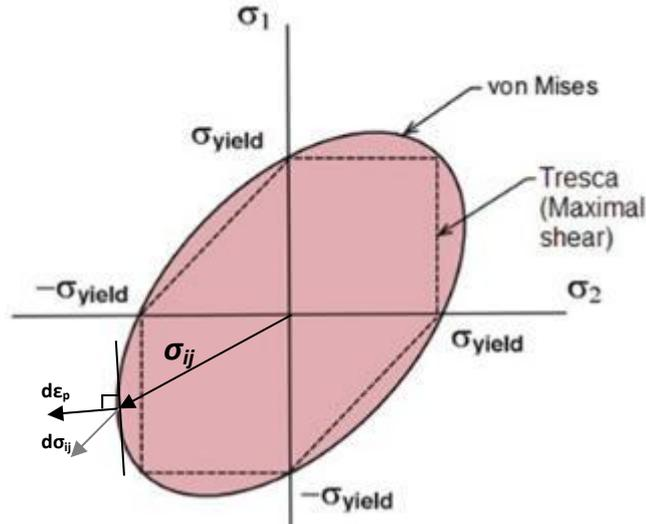
Figure 4-4. Von Mises and Tresca criteria for a 2-D stress state.
