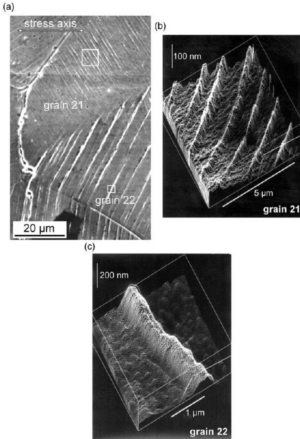
Figure 2-6. Surface relief within the grains nr 21 and 22 of 316L stainless steel cycled with constant plastic strain amplitude of  $1 \times 10^{-3}$  for 30.000 cycles. a) SEM micrograph at the area of the two grains at low magnification. b-c) Three-dimensional AFM images showing the detail of the occurring surface relief within grain nr 21 and 22 respectively. The areas scanned by atom force microscopy are marked in (a) with white boxes [5].
