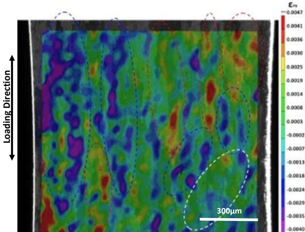
Figure 5-23. Shear strain distribution for the fully loaded sample after 5000 cycles.
