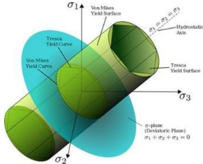
Figure 4-5. 3-D image of the yield surface for a 3-D stress state.
