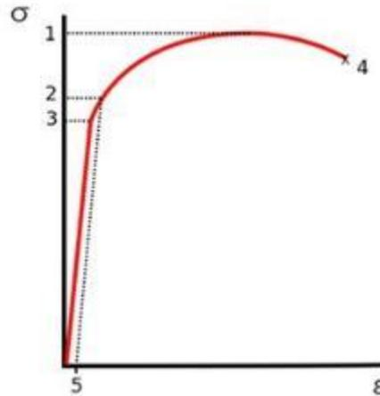
Figure 4-3. Stress-strain curve obtain from a typical tensile experiment.
