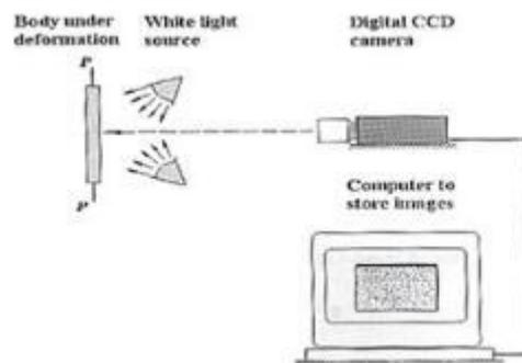
Figure 3-9. DIC set-up system for one camera.
