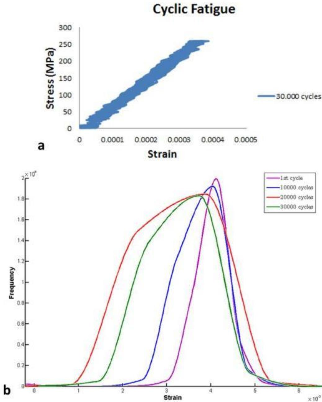
Figure 5-17. a) Stress-strain curves output from the testing machine, b) Strain distributions measured by means of DIC at maximum load ( $0.75\sigma_y$  and initial applied strain 0.004) after 1, 10000, 20000, and 30000 cycles.
