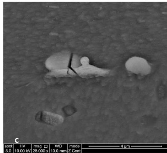
Figure 6-18. Nanoparticles broken, with no strain localizations in the matrix.
