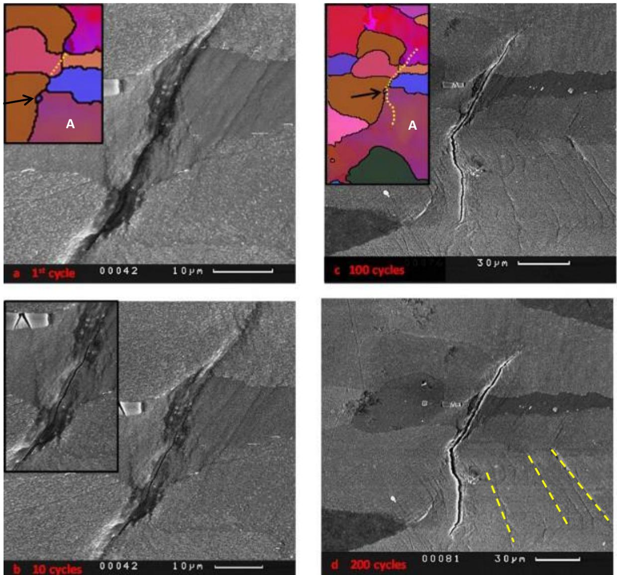
Figure 6-47. SEM images at the black (dotted) circled region of figure 6.45a, for the fully loaded condition of the specimen after: a) 1, b) 10, c) 100 and d) 200 cycles.
