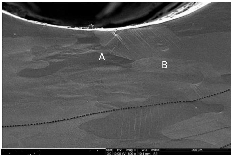
Figure A3. Overview image at the location of cracking, together with grain A and B
