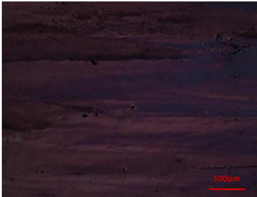
Figure 6-5. High magnification optical microscopy image from area B in Figure 6.3a. Differential Interference Contrast microscopy image indicates the presence of out of plane deformation, and the formation of deformation ripples on the surface.
