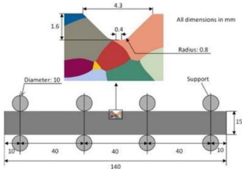
Figure 2-21. 4 point bending set-up and the grain geometry at the edge of the notch [15].
