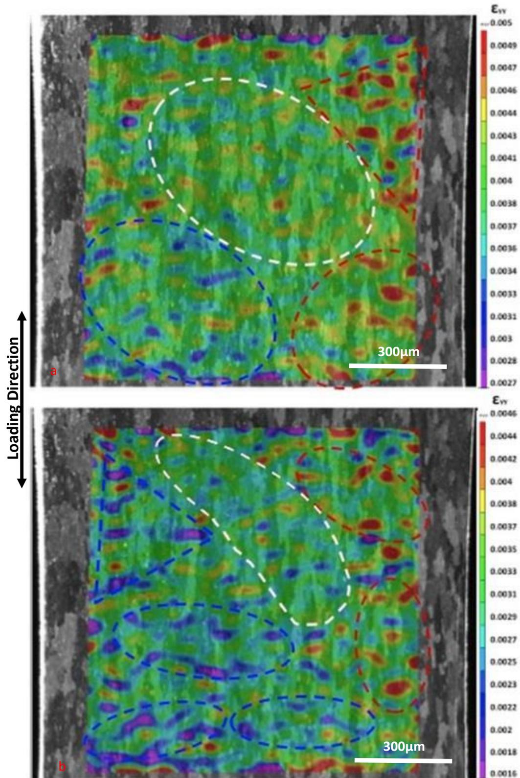
Figure 5-16. Strain distributions (on the principal direction,  $\epsilon_{yy}$ ) for the fully loaded sample after: a) 1 cycle, and b) 30000 cycles.
