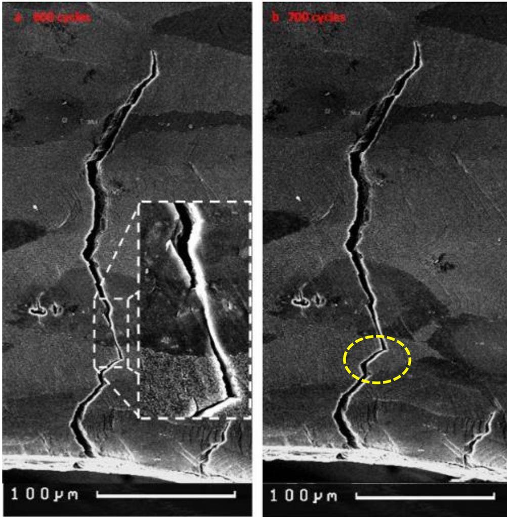
Figure 6-49. SEM images at the black (dotted) circled region of figure 6.45a, for the fully loaded condition of the specimen after: a) 600 and b) 700 cycles. The two crack meet due to the local stress fields.
