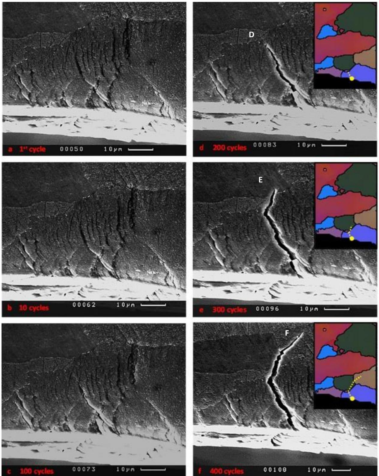
Figure 6-50. SEM images at the location of crack C2, for the fully loaded condition of the specimen after: a) 1, b) 10, c) 100, d) 200, e) 300 and f) 400 cycles.
