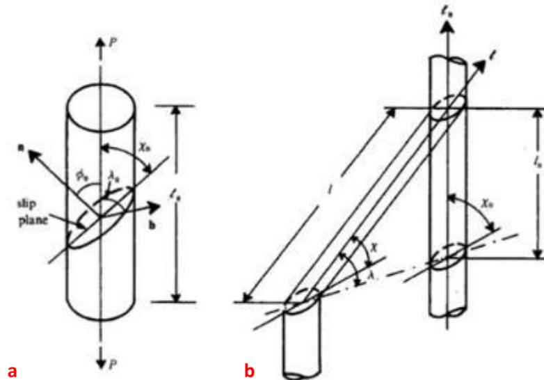
Figure 4-10. a) A single crystal with the associated slip plane and direction. b) Change of the shape of the single crystal due to slip [8].
