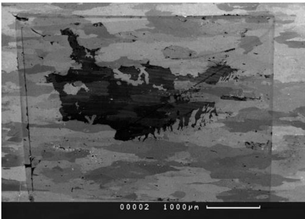
Figure B1. HC deposition. Imaging at the location where EBSD measurements were previously taken, for the after etched condition for the sample.
