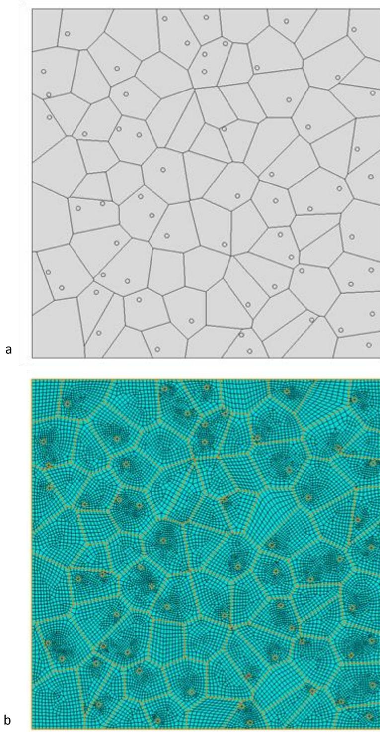
Figure 7-13. a) Polycrystal geometry created containing a user-defined distribution of particles. b) Meshed part
