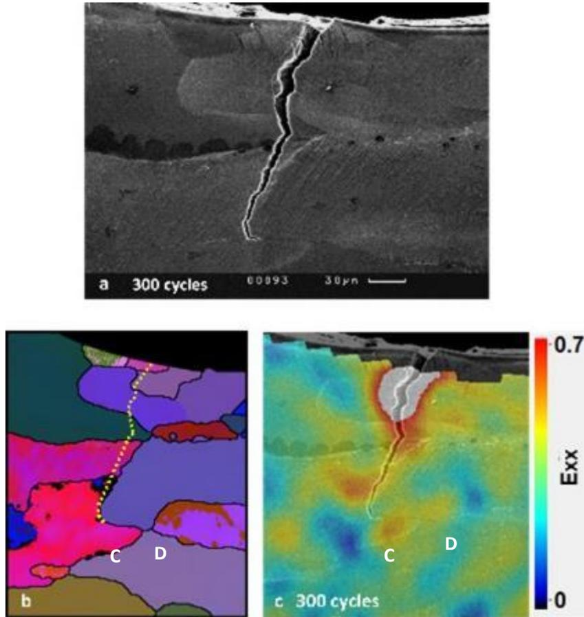
Figure 6-56. a) SEM image after 300 cycles, at maximum displacement, b) EBSD measurements of the corresponding location and c) DIC map at the same region after 300 cycles, at maximum displacement.
