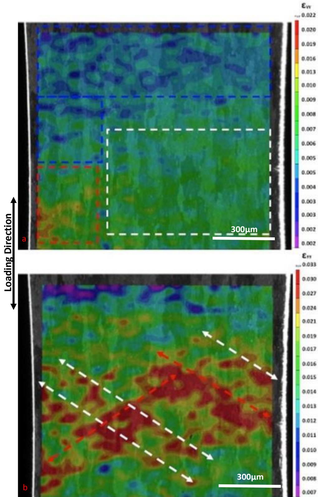
Figure 5-20. Strain distributions (on the principal direction:  $\epsilon_{yy}$ ) for the fully loaded sample after: a) 1 cycle, and b) 5000 cycles.
