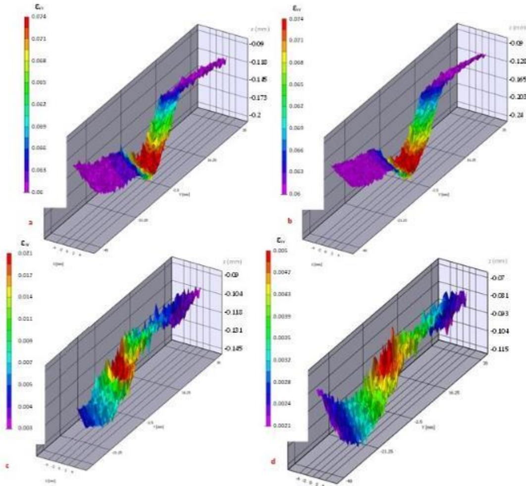
Figure 5-14.  $\epsilon_{yy}$  strain contours and surface profile for: a) tensile loading at 0.065 strain, b) the same accumulated strain 0.065 after 5000 cycles and  $1.11\sigma_y$  stress amplitude, c) after 5000 cycles and at a stress amplitude  $1.02\sigma_y$  and d) after 30000 cycles and at a stress amplitude  $0.75\sigma_y$ .
