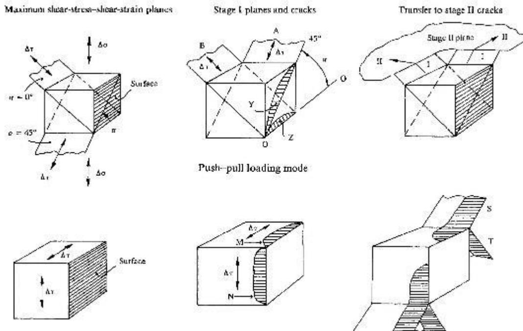
Figure 2-4. The effects of loading mode on the development of stage I and II cracks. Y, Z, M and N are stage I cracks while S and T are stage II cracks [2].
