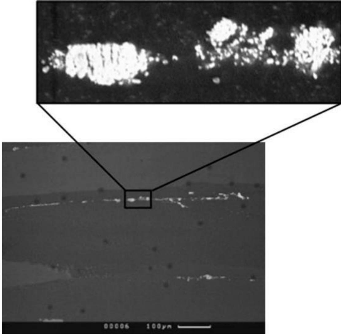
Figure 5-4. Particles in Al2024, in an etched sample.
