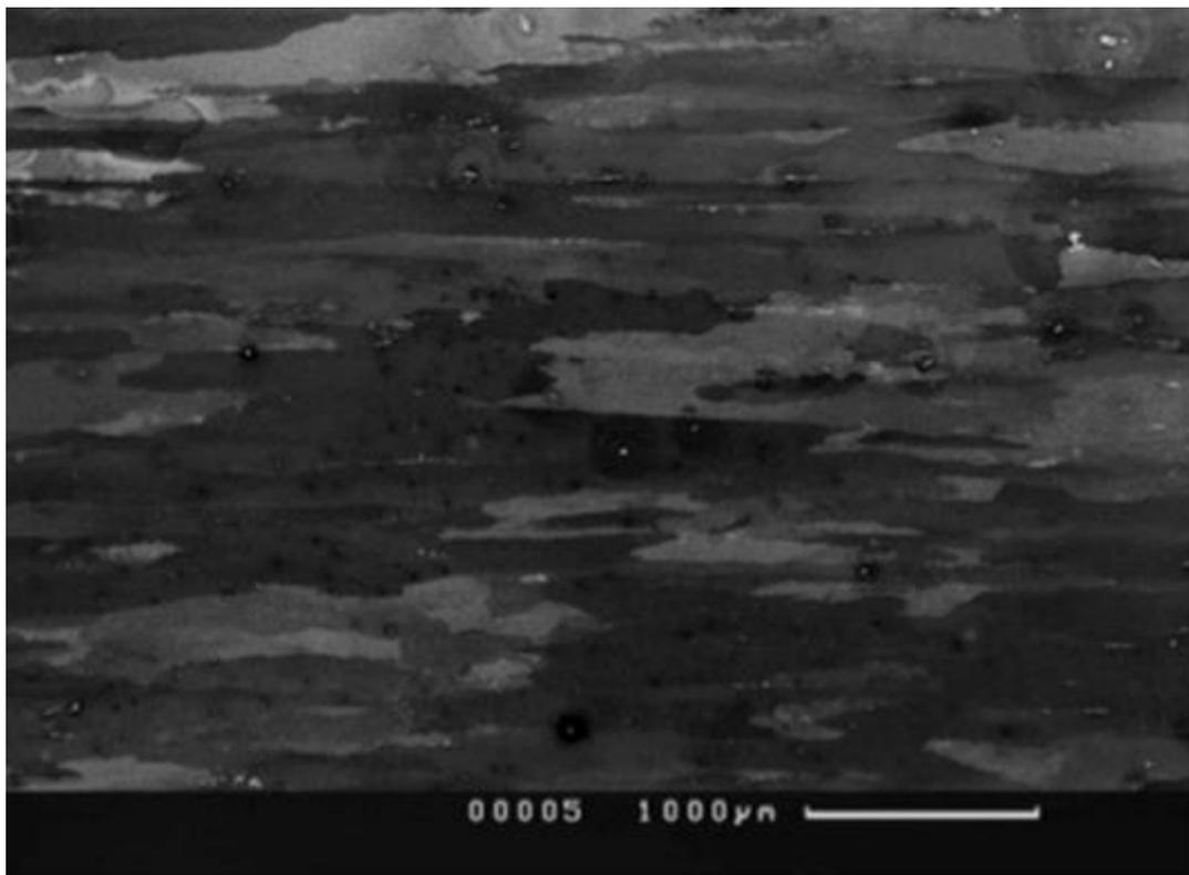
Figure 6-1. SEM image of the region selected for observing in situ strain development within the grains.
