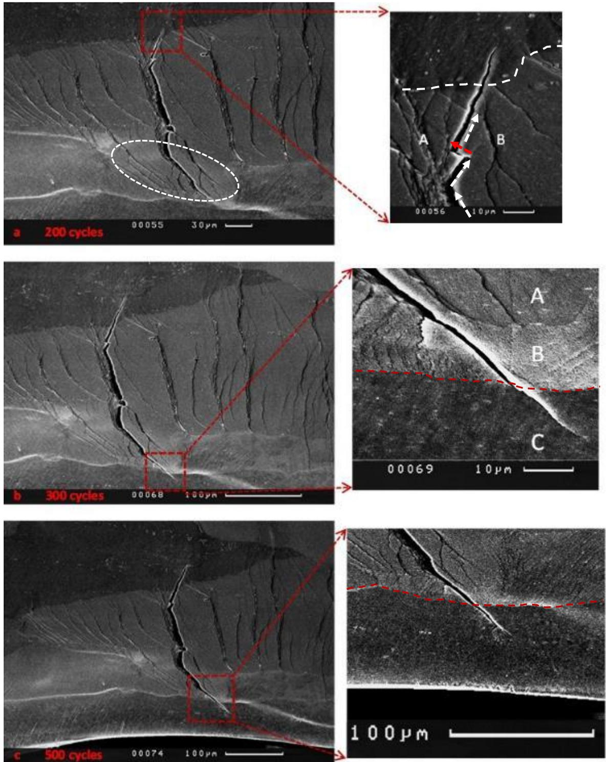
Figure 6-25. SEM images of the highlighted grain of figure 6.23a for the fully loaded condition of the specimen after: a) 200 cycles, b) 300 cycles and c) 500 cycles.
