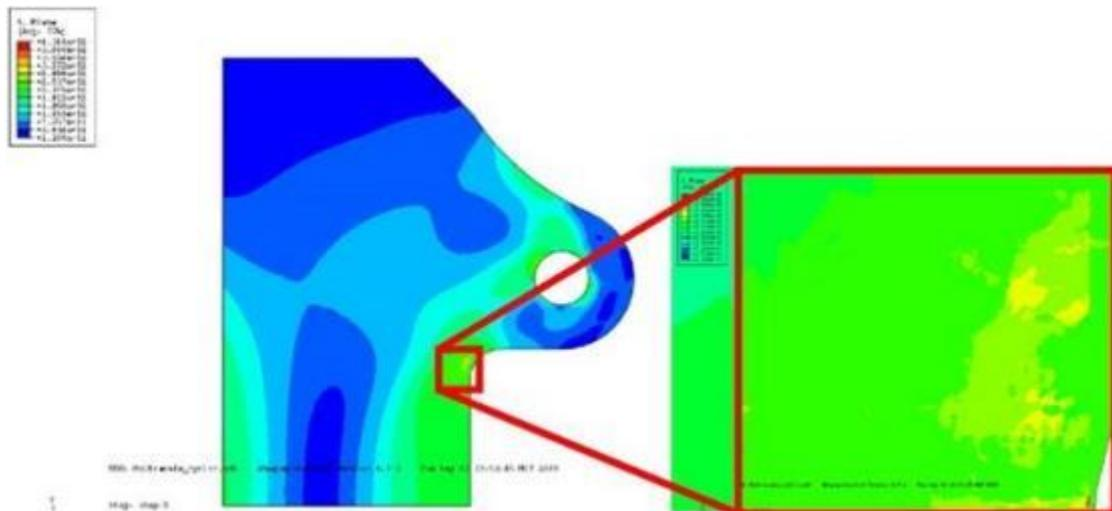
Figure 2-29. Mises stress distribution of lug joint [18].
