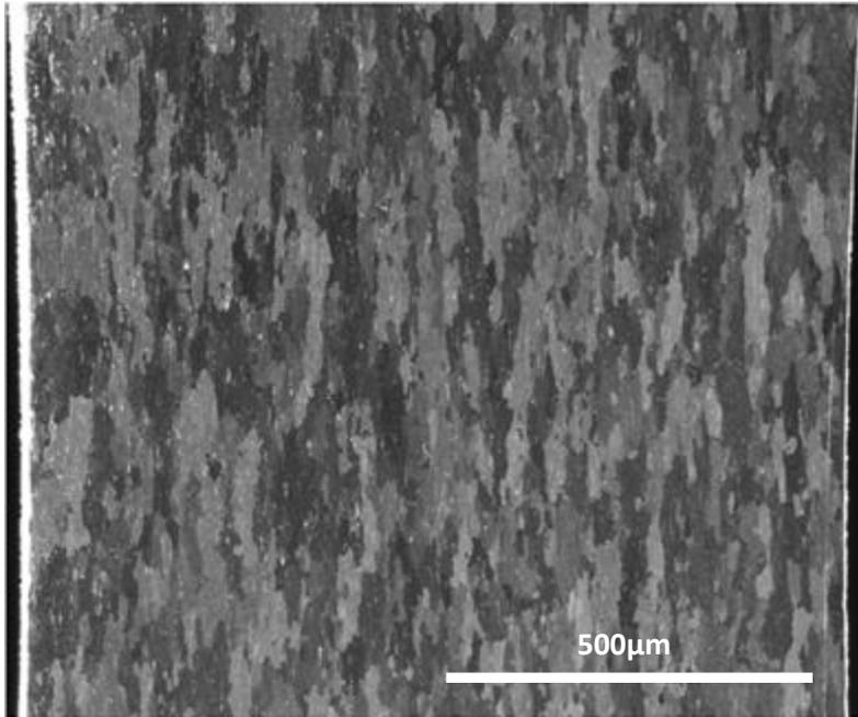
Figure 3-2. Etched microstructure of Al2024.
