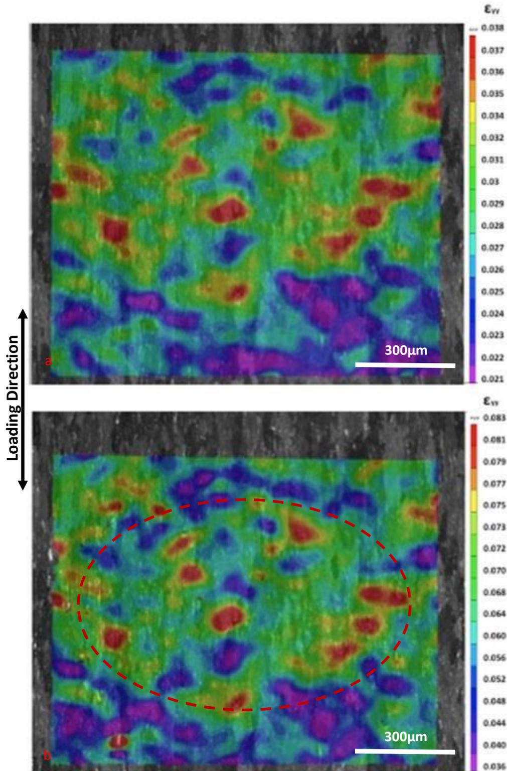
Figure 5-24. Strain distributions (on the principal direction:  $\epsilon_{yy}$ ) for the fully loaded sample after: a) 1 cycle, and b) 5000 cycles.
