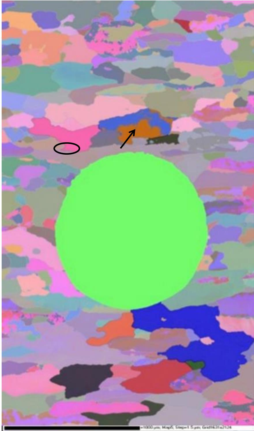
Figure 6-36. Soft grains, with slip bands and non-uniform highly localised plastic deformation.
