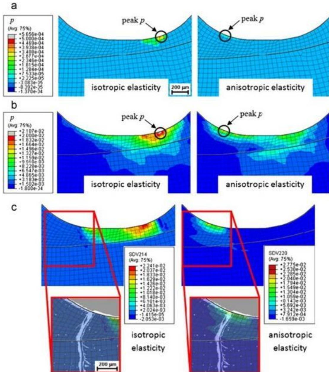
Figure 2-24. Field variations for specimen 2 from crystal FE models with isotropic and anisotropic elasticity of (a) effective plastic strain,  $p$ , initially after yielding, (b) effective plastic strain,  $p$ , at full load after cyclic loading and (c) accumulated plastic slip,  $\gamma_\alpha$ , on the slip system with the highest slip for each model at full load after cyclic loading [15].
