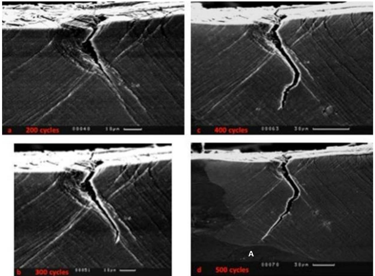
Figure 6-30. SEM images of the white-highlighted region of the EBSD map in figure 6-28 for the fully loaded condition of the specimen after: a) 200 cycles, b) 300 cycles, c) 400 cycles and c) 500 cycles.
