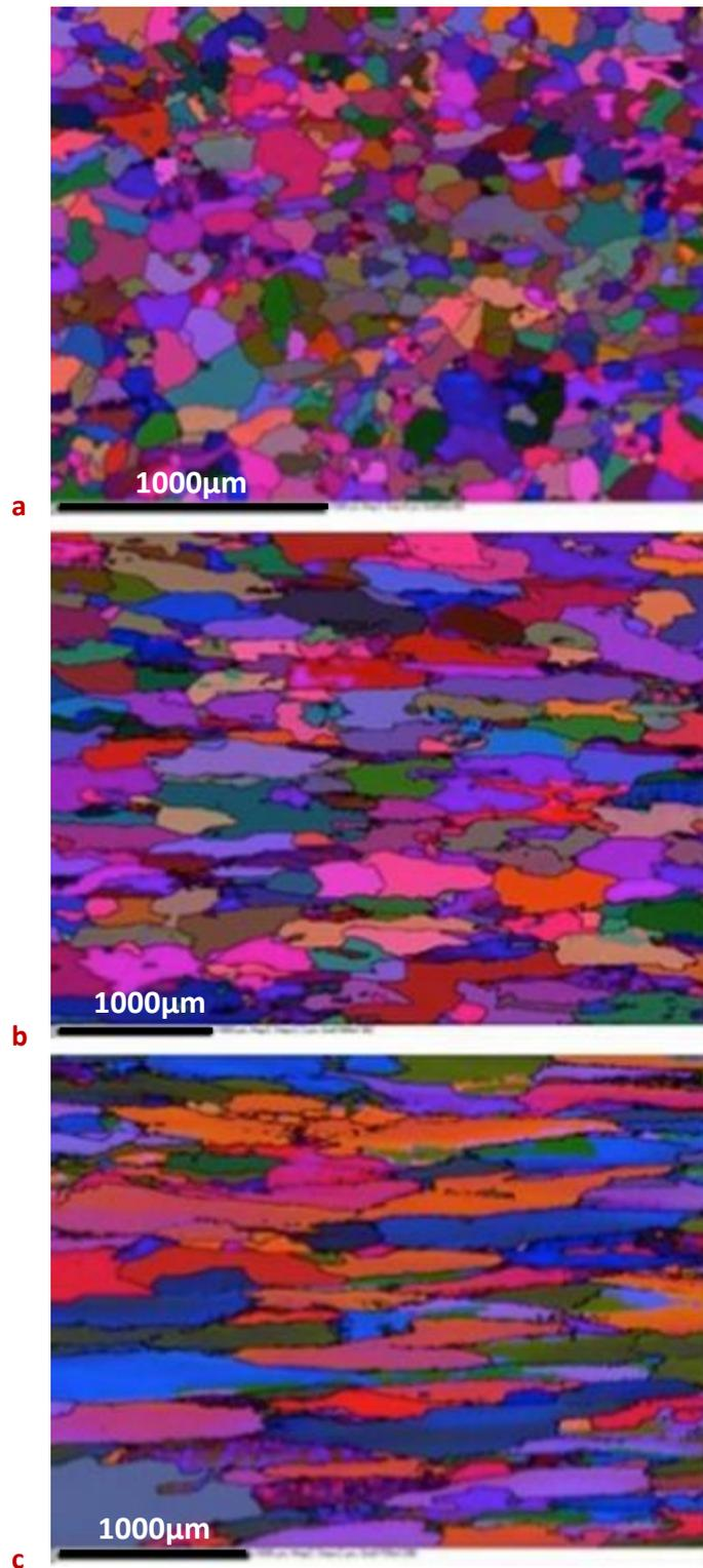
Figure 5-3. EBSD maps at various locations of the aluminium slab. a) From surface ( $\sim 200$  micron from the slab surface), b) moving towards the slab centre (approximately 1 cm from the slab surface) and c) at the centre of the slab.
