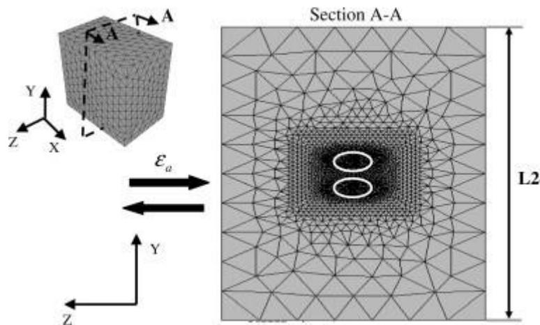
Figure 2-42. Cross-section of FE mesh through the center of inclusion with refinement close to the inclusion [43].
