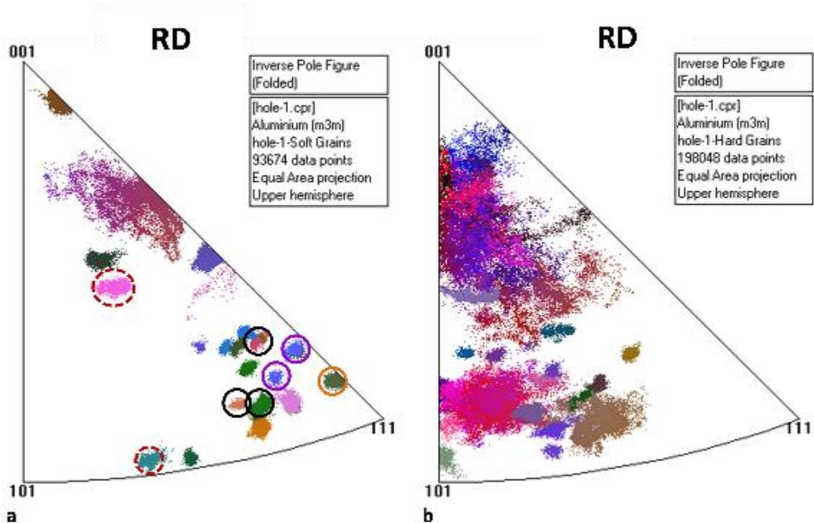
Figure 6-63. Inverse pole figures (IPF) for the highlighted grains of a) figure 6.61 and b) 6.62.
