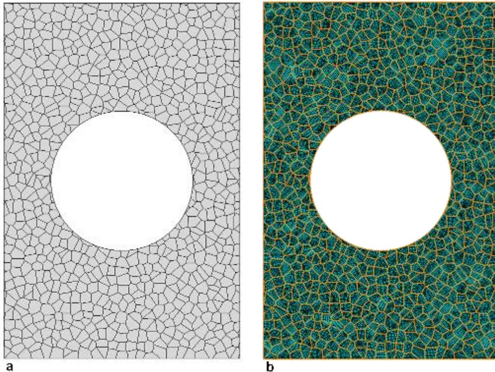
Figure 7-10. a) The geometry used in Abaqus modeller. The Voronoi grains had random orientations, while grain boundaries were modelled explicitly, b) Meshed part.
