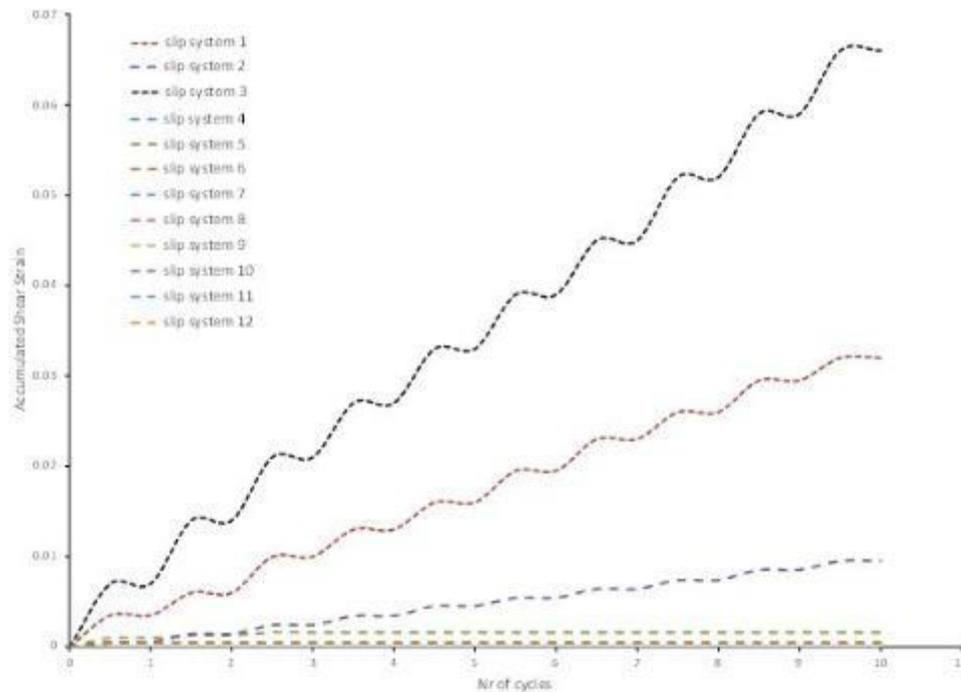
Figure 7-9. Accumulated shear strain for each slip system against the number of cycles at location A in figure 7.8.
