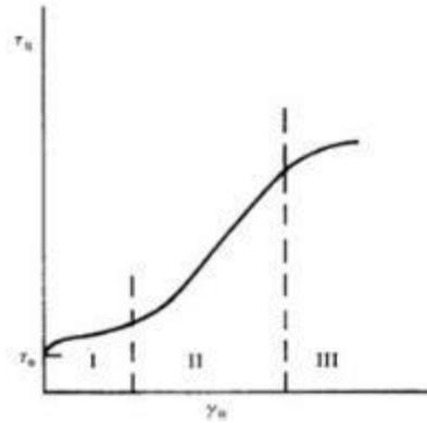
Figure 4-11. A stress - strain curve for an FCC single-crystal, and the 3 regimes of deformation [8].
