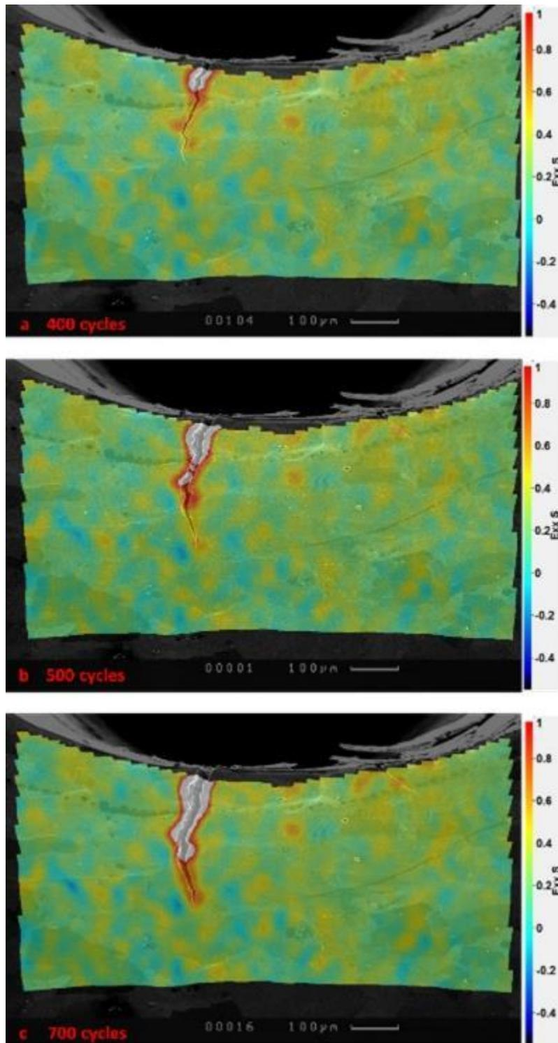
Figure 6-53. Strain distributions for the fully loaded sample after: a) 400, b) 500 and c) 700 cycles.
