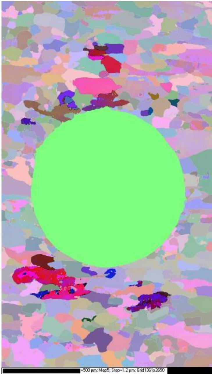
Figure 6-62. Hard grains, with no slip bands and uniform plastic deformation.
