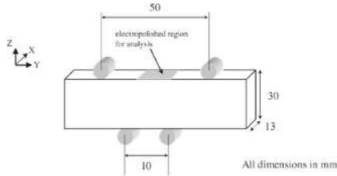
Figure 2-15. Schematic representation of the four-point bend test specimen geometry for high cycle fatigue testing [13].
