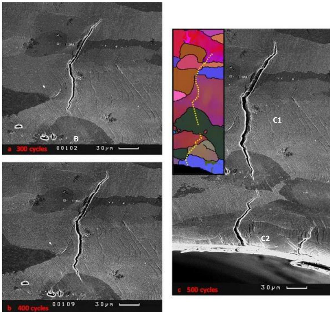
Figure 6-48. SEM images at the black (dotted) circled region of figure 6.45a, for the fully loaded condition of the specimen after: a) 300, b) 400 and c) 500 cycles.
