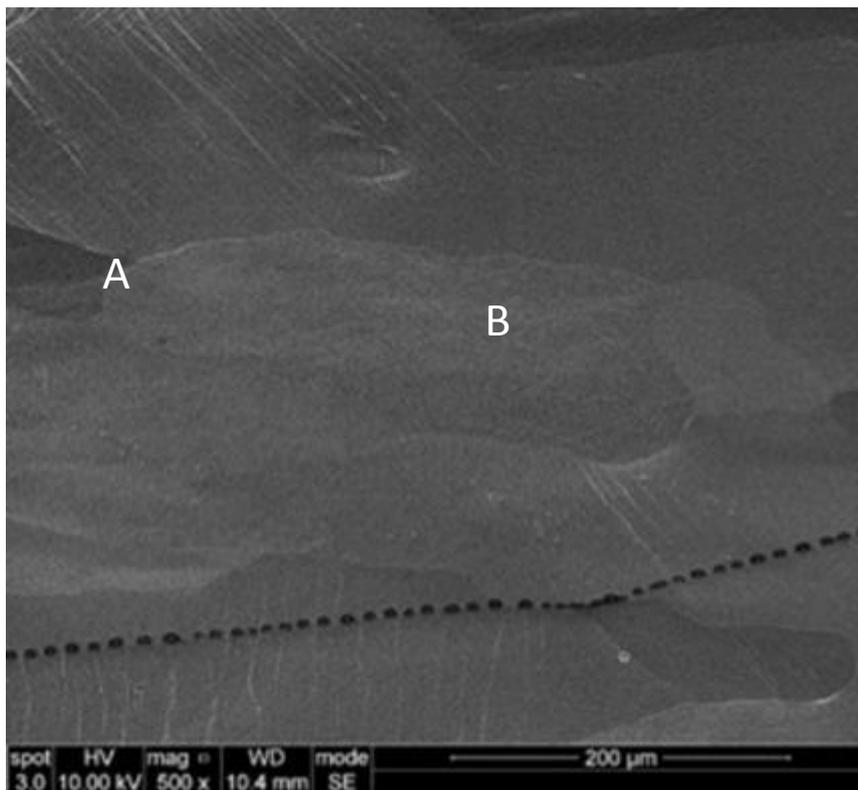
Figure 6-39. 'Hard' grain B in between highly deformed 'weak' grains.
