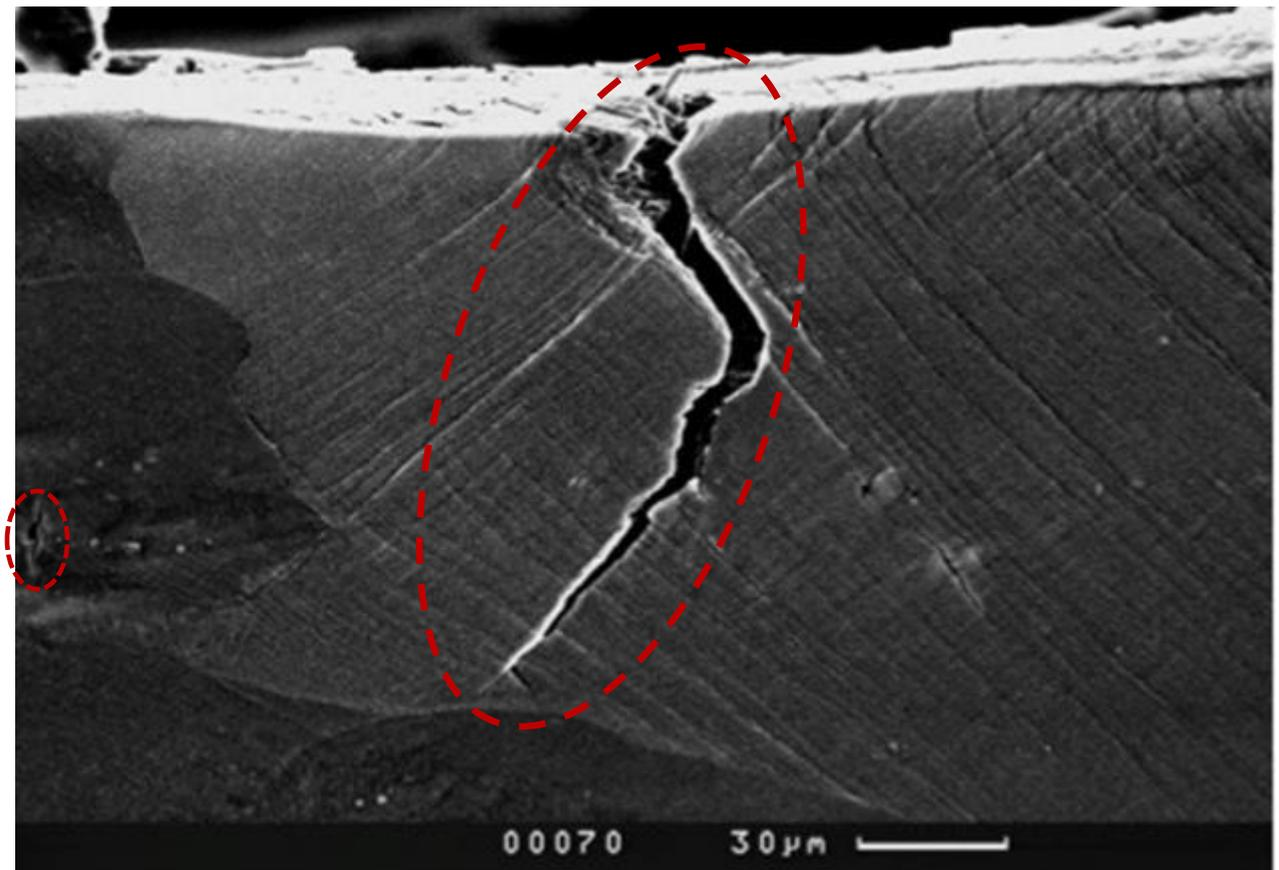
Figure 6-32. SEM images of the region of the EBSD map highlighted by the white and black circles in figure 6-28 for the fully loaded condition of the specimen after 500 cycles.
