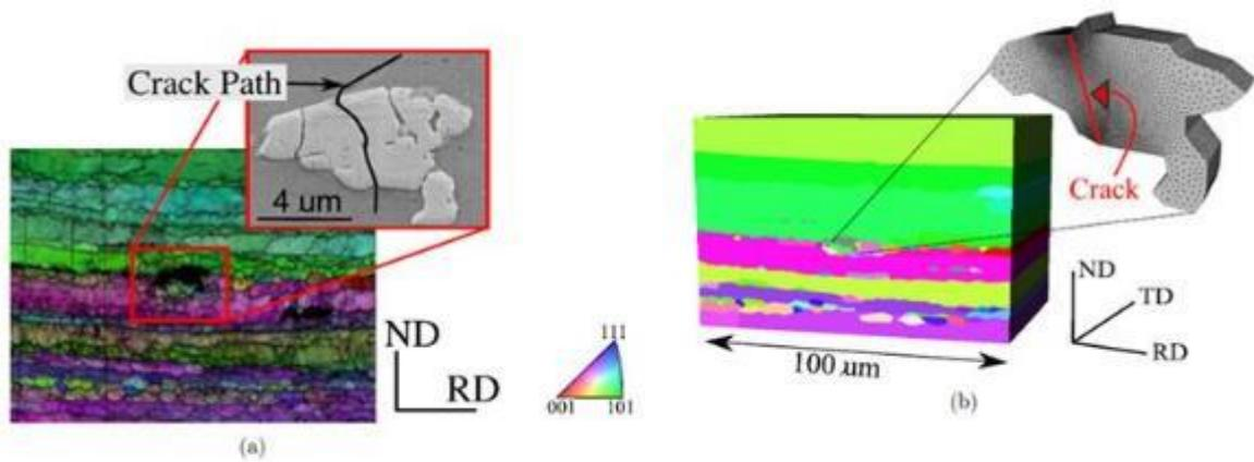
Figure 2-50. Finite Element Model generated from experimental data [45].
