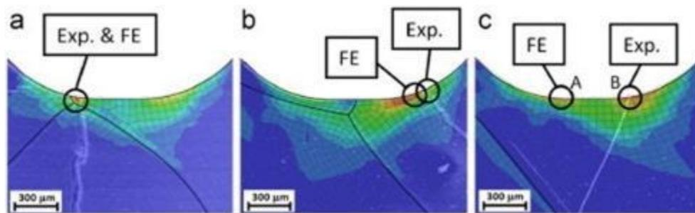
Figure 2-25. Field variations of effective plastic strain,  $p$ , with superimposed images of experimentally observed crack nucleation and growth for (a) specimen 7, (b) specimen 8 and (c) specimen 6. Experimental and crystal FE predicted sites of fatigue crack nucleation are highlighted [17].
