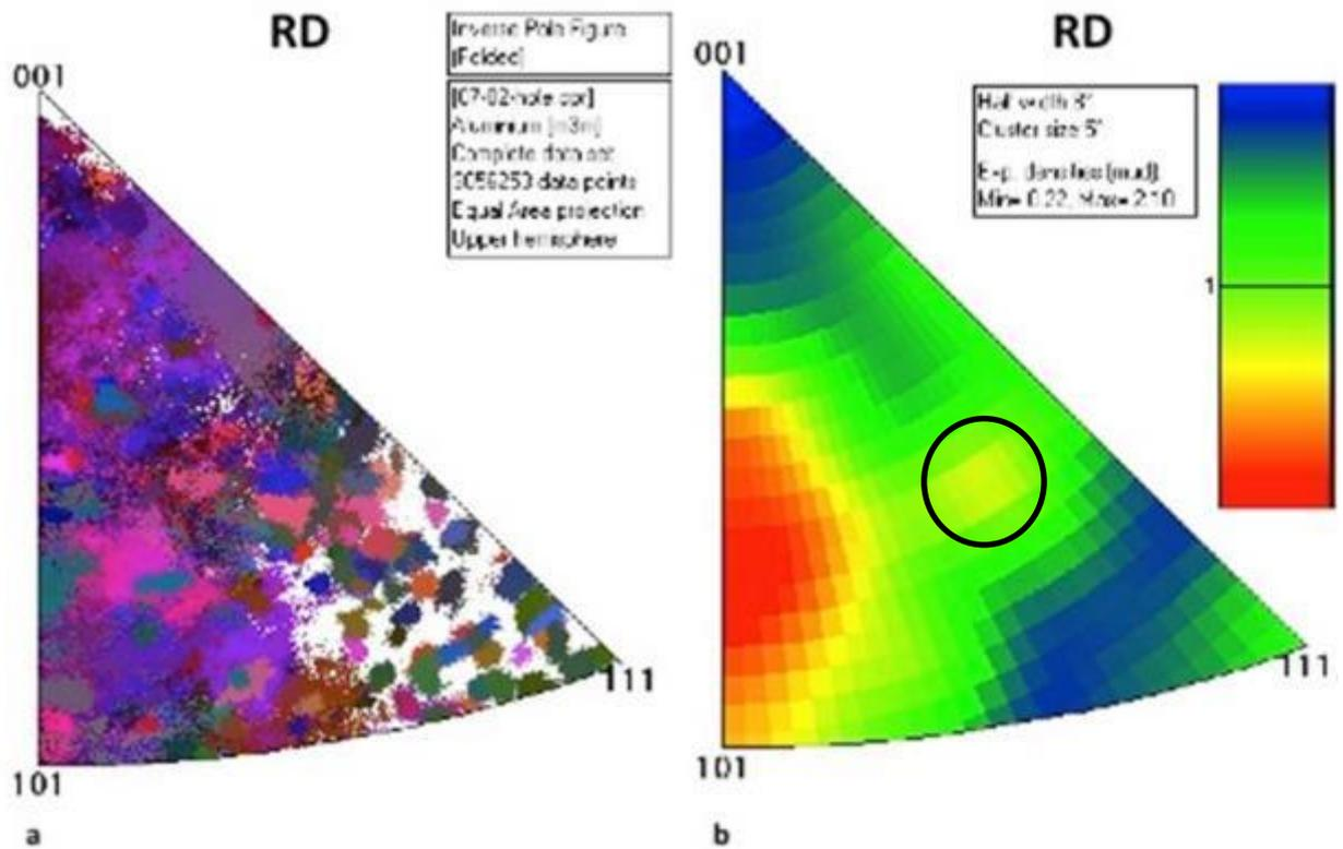
Figure 6-34. Inverse pole figures (IPF) for the EBSD map of figure 6.21 with respect to RD. a) Data points of each grain within the IPF, and b) Density contours showing the effect of rolling.
