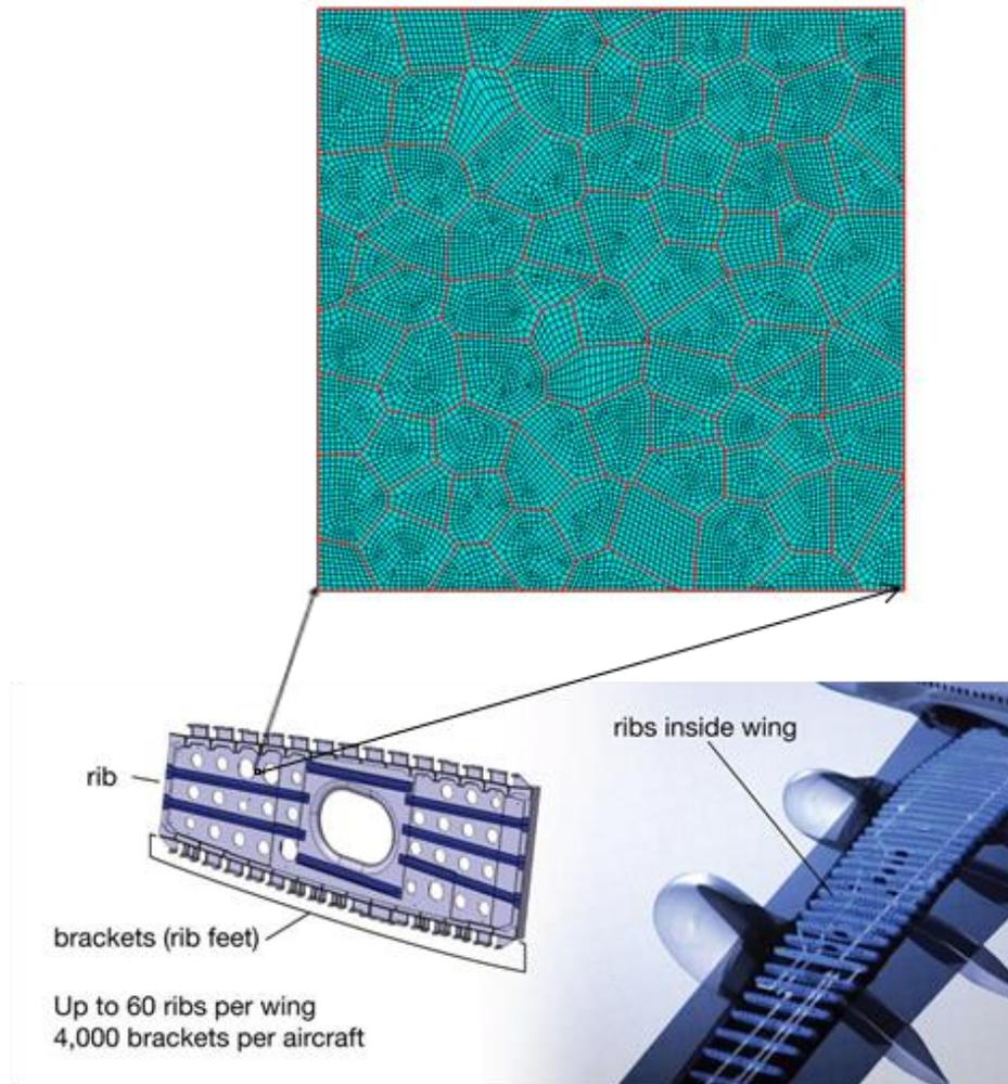
Figure 7-18. Multiscale approach for a more complex geometry.
