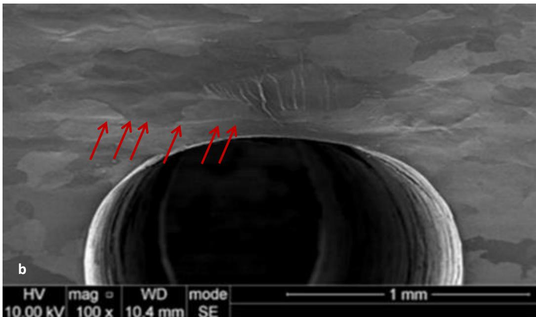
Figure 6-42. a) Slip band formation at the location circled in figure 6-36, b) low magnification imaging at the same area.
