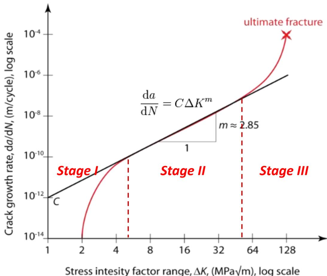
Figure 1-2. Fatigue lifetime: the 3 fatigue lifetime regimes-stages and the Paris law relation describing stage II cracks.
