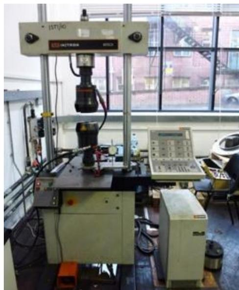
Figure 3-6. Instron 8501 hydraulic machine.
