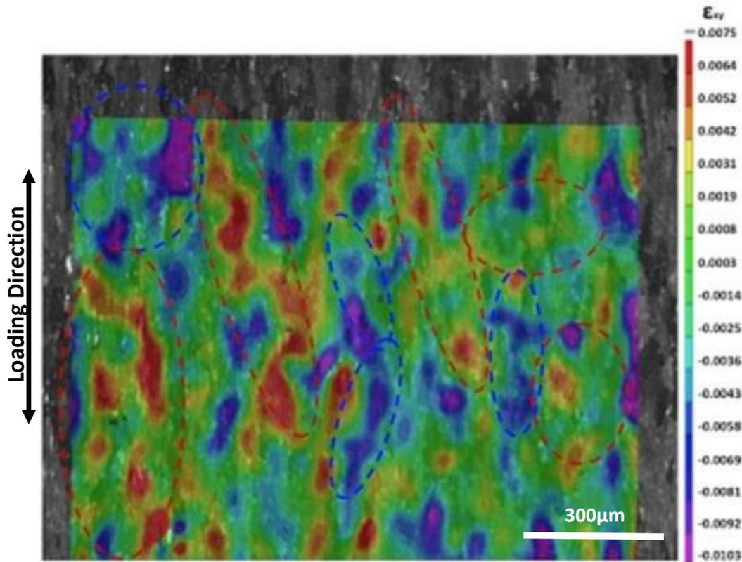
Figure 5-27. Shear strain distribution for the fully loaded sample after 5000 cycles.
