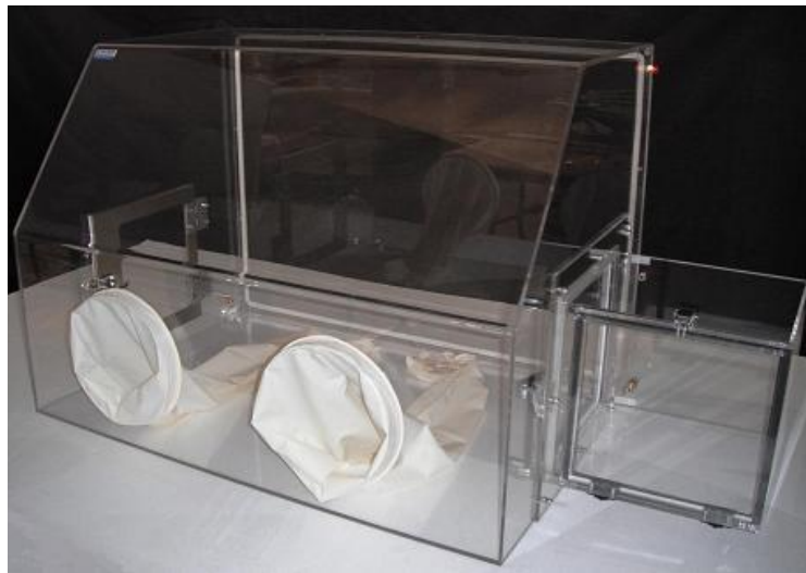
Figure 57. Image of a glove box that could be placed around a Raman microscope the direct acquisition of Raman spectra from sterile cells. Image from http://www.laboratory-supply.net/gloveboxes/isolation_glovebox.html
