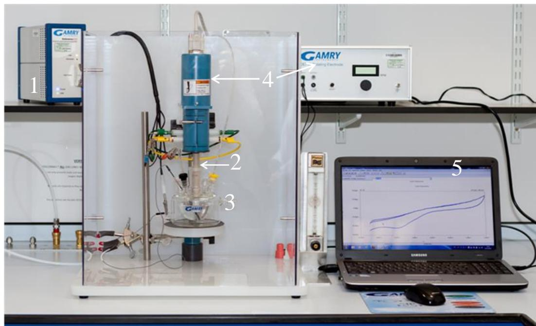
**Figure 6.15** Photograph of the RRDE equipment: (1) potentiostat, (2) rotating ring disk electrode, (3) test cell, (4) electrode rotator, and (5) computer.
