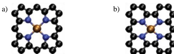
**Figure 2.13** Transition metal macrocycle active sites based on the structures of a) porphyrine, and b) tetraazaannulene [104]. The carbon, nitrogen and transition metal atoms are designated by the black, blue and brown colours, respectively.
