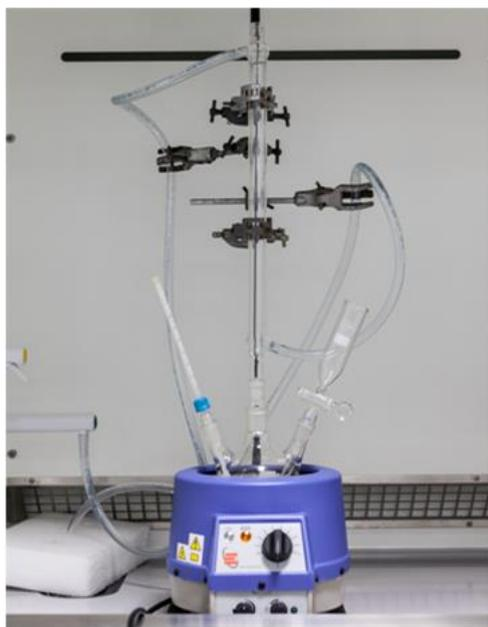
**Figure 6.12** Photograph of the reflux condenser.
