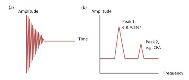
**Figure 6.2** Diagrammatic representation of the (a) FID signal collected following an NMR run and (b) data following Fourier transformation. Adapted from Newton (1998).
