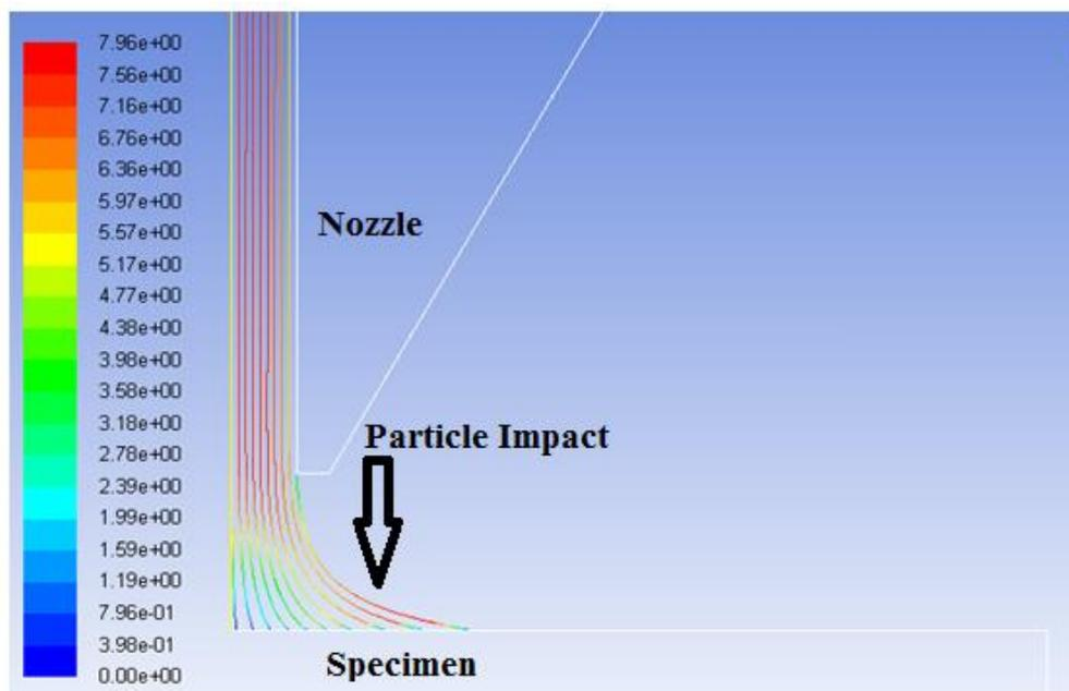
**Figure 7.20: Illustration of sand particle motion within the impingement jet and subsequent impact on the specimen surface as predicted by CFD.**
