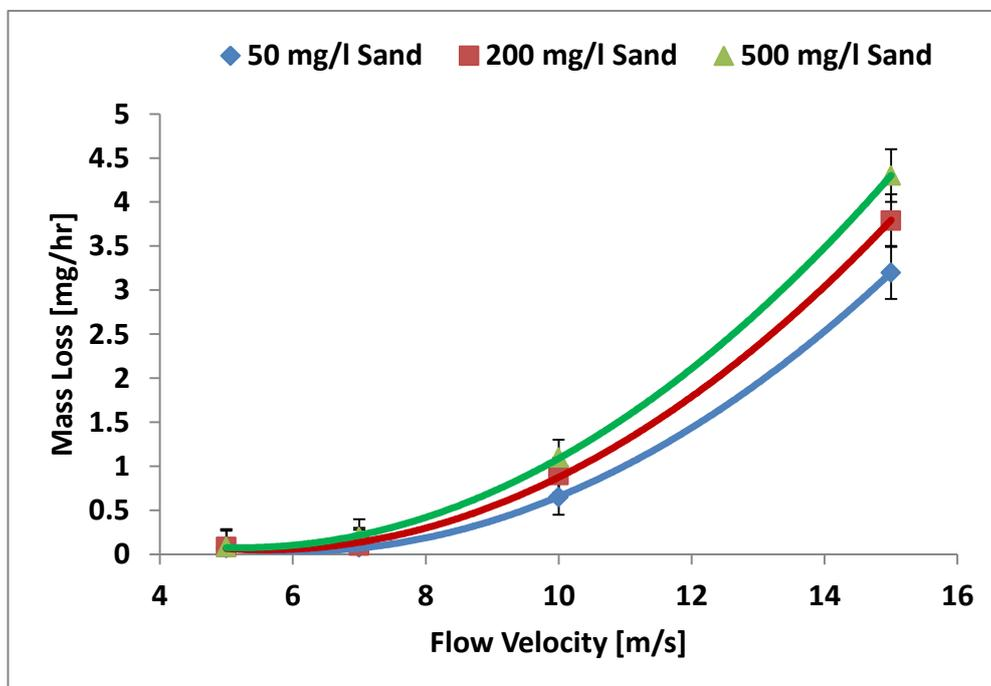
**Figure 6.9: Variation of mass loss with flow velocity test with tap-water saturated with  $N_2$  ( $pH \approx 7.0$ ) at  $90^\circ$  impingement angle and  $50^\circ C$  temperature.**
