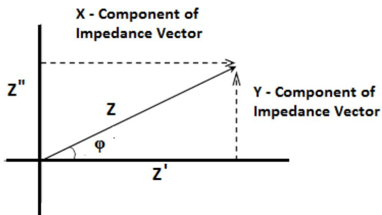
**Figure 2.9: An impedance vector resolved into X-Y components [43].**
