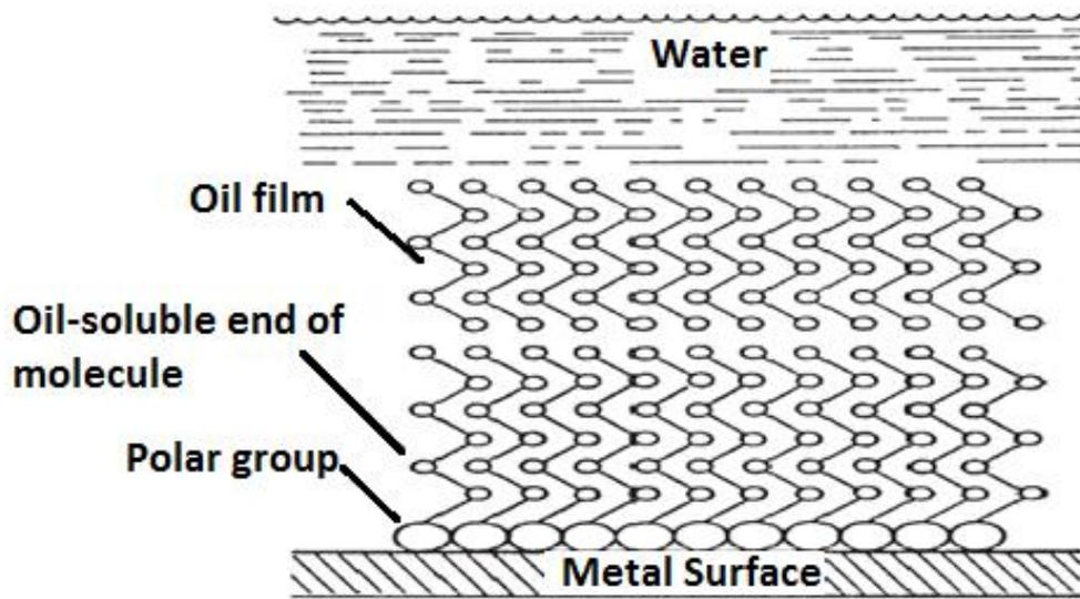
**Figure 3.20: Illustration of basic principles of inhibitor film-forming [147].**
