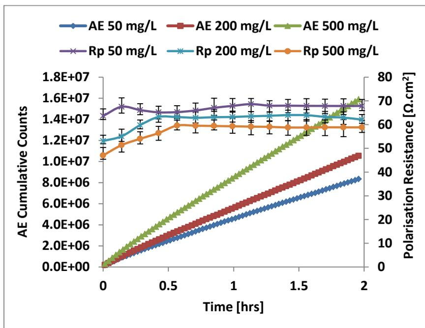
Figure 8.11: Results for erosion-corrosion test showing polarisation resistance variation with AE cumulative counts for 10 m/s in  $\text{CO}_2$  saturated brine (pH 5.5) at  $50^\circ\text{C}$ .
