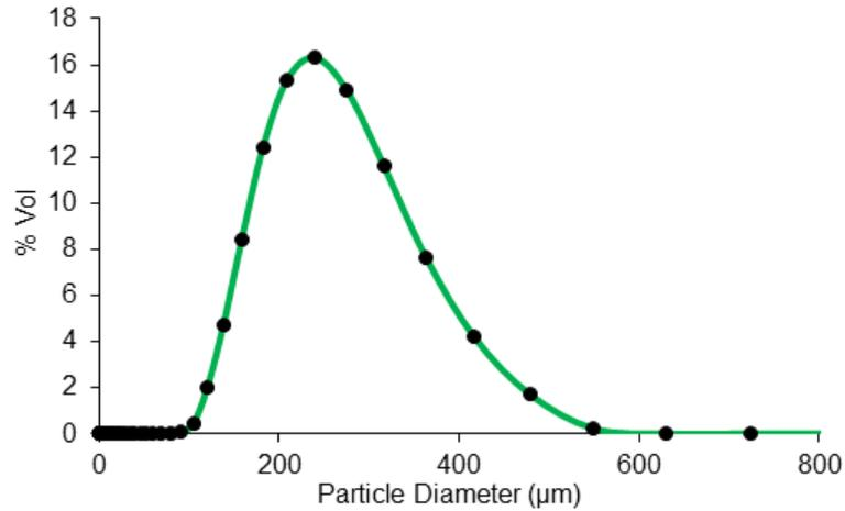
Figure 5.4: Sand particles' size distribution from sieve experiment.
