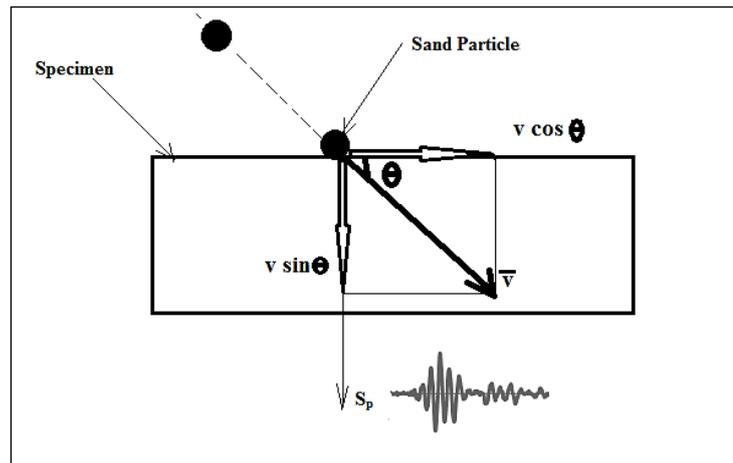
**Figure 7.2: Illustration of generation of AE signal from single sand impact [201].**
