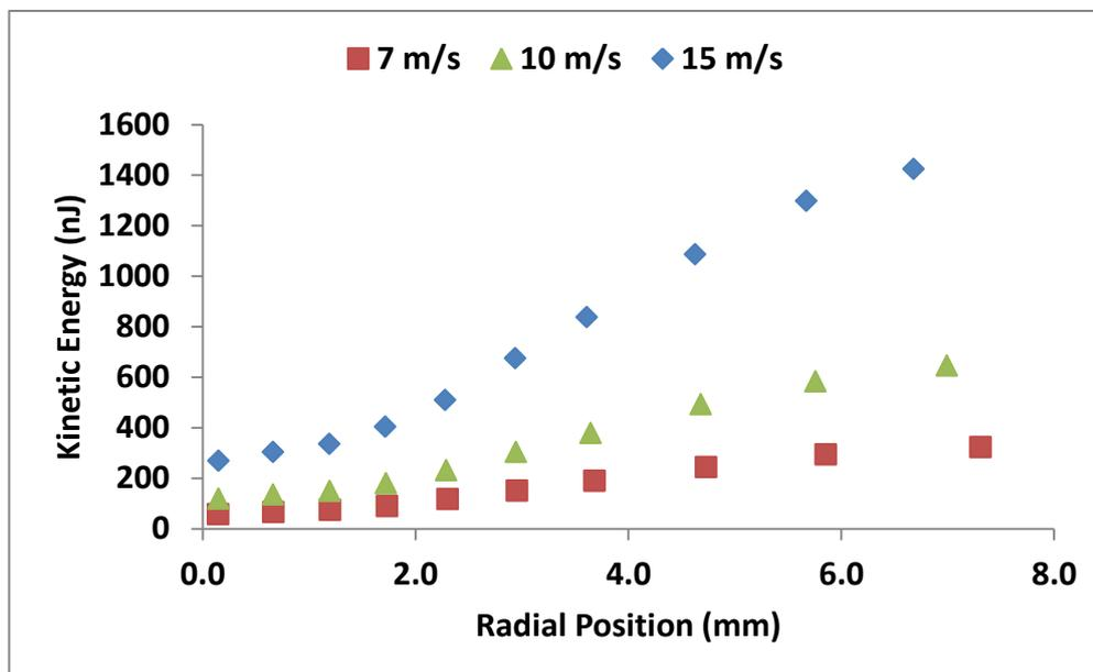
**Figure 7.23: Predicted variation of particle impact energy with radial distance.**
