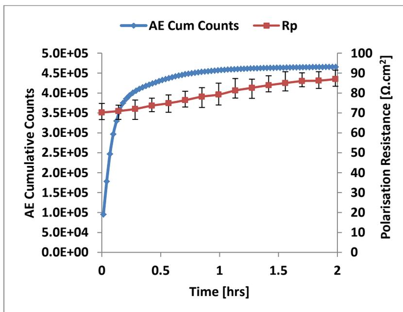
Figure 8.2: Polarisation resistance variation with AE cumulative counts for 7 m/s flow in CO<sub>2</sub> saturated brine (pH 5.5) at 50°C.
