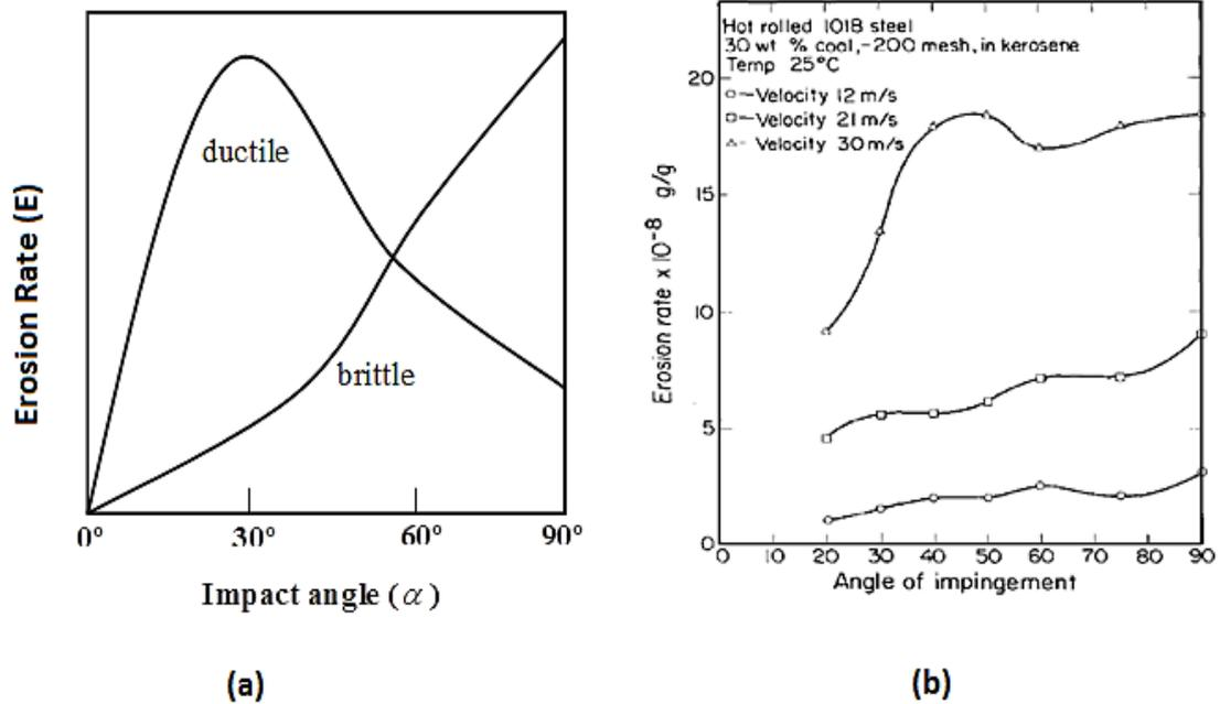
**Figure 3.14: Effect of impact angle on erosion (a) Hutchings [83], (b) Levy and Yau [86].**
