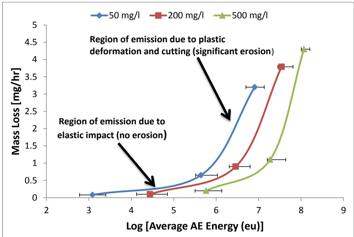
Figure 6.21: Relationship between mass loss and average AE energy for the flow velocities and sand loading investigated with tap-water saturated with N<sub>2</sub>.
