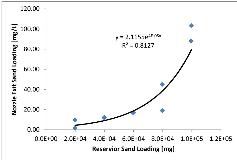
Figure 5.7: Plot of nozzle exit sand concentration variation with sand loading added to the reservoir during the sand loading calibration for 7 m/s flow velocity.
