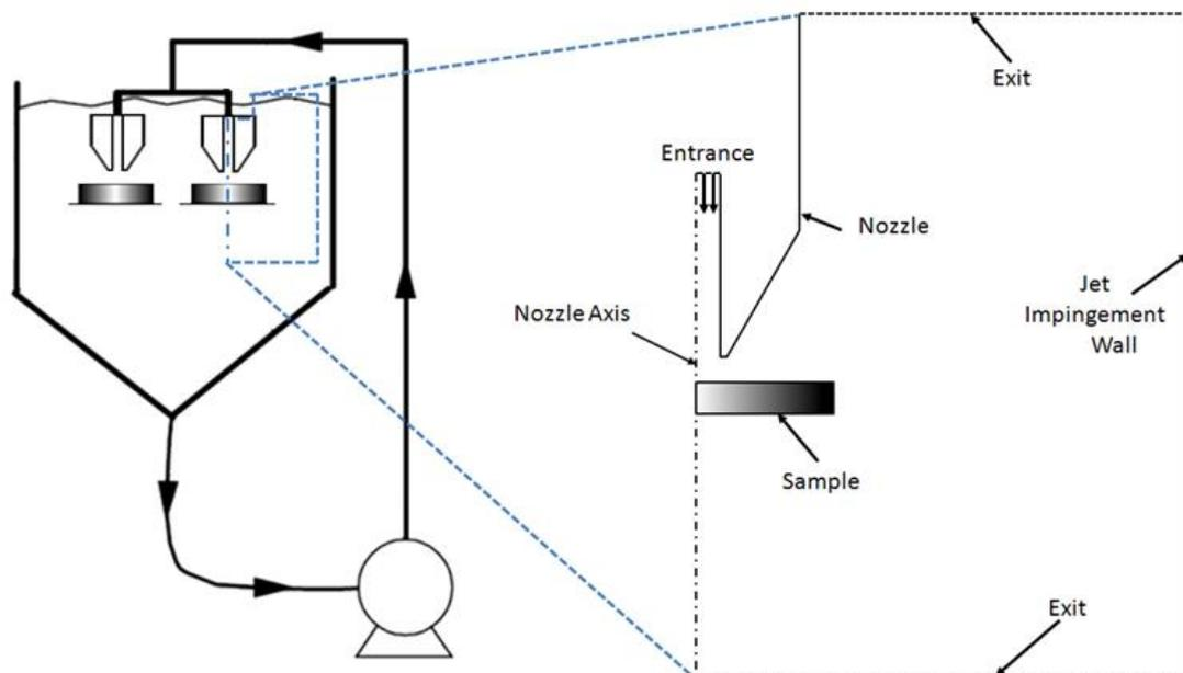
**Figure 7.16: Schematic illustration of the physical domain (left) and computational domain (right) of the submerged impinging jet.**
