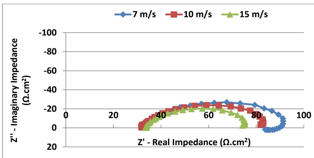
**Figure 9.4: Summary of the Nyquist plots of all the flow velocities after 120 minutes with process brine without sand, 50°C and CO<sub>2</sub> saturated at 1 bar.**
