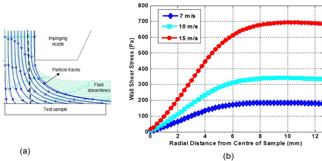
**Figure 5.2: (a) Fluid streamlines with the particle tracks in the SIJ system and (b) wall shear stresses across the surface for 7, 10 and 15 m/s flow velocities [110].**
