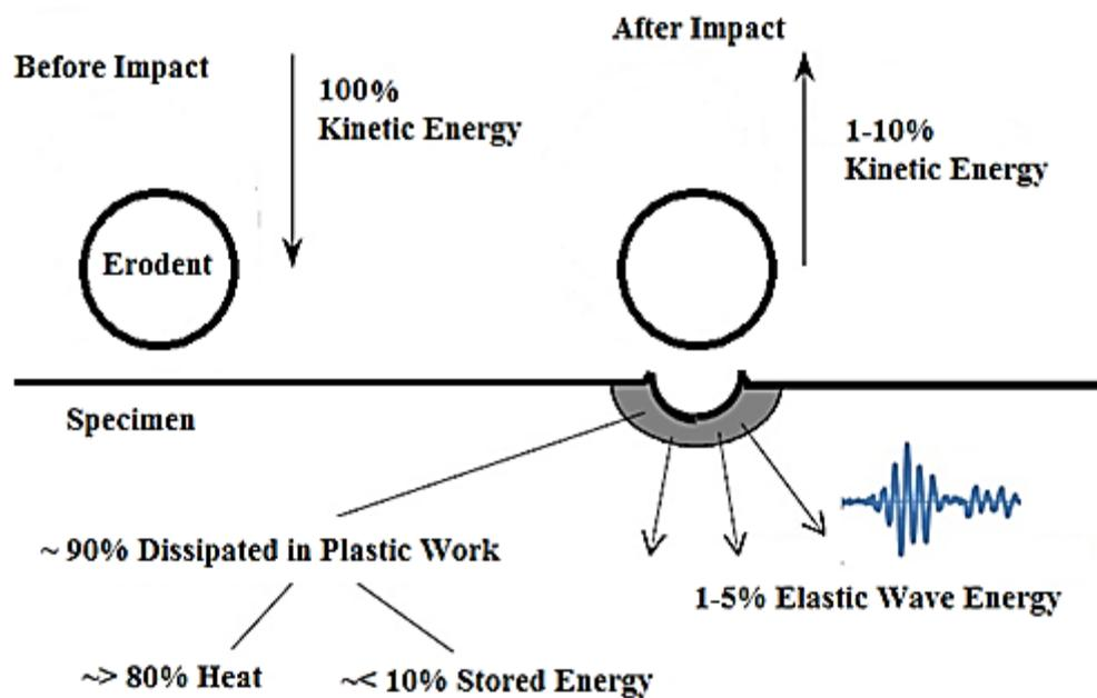
**Figure 4.8: Illustration of AE release from solid particle impact [101, 176].**
