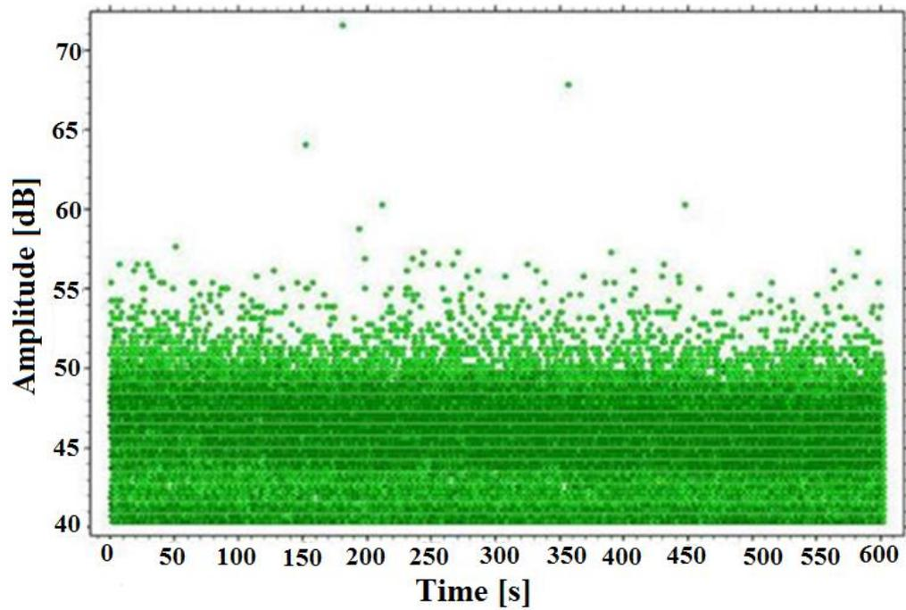
Figure 5.14: Raw data of noise test with pump running at 7 m/s flow velocity and threshold set at 40 dB.
