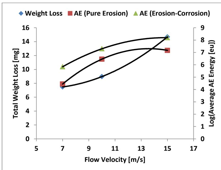
Figure 8.19: Results of the total weight loss with measured average AE energy in energy units ([eu],  $1\text{eu}=1\text{E}-18\text{J}$ ) in the presence and absence of corrosion for 200 mg/L sand concentration.
