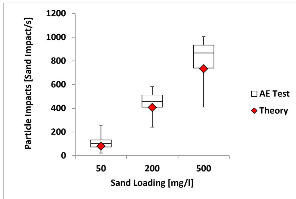
Figure 7.14: Comparison of measured particle impacts with theory for 10 m/s flow velocity.
