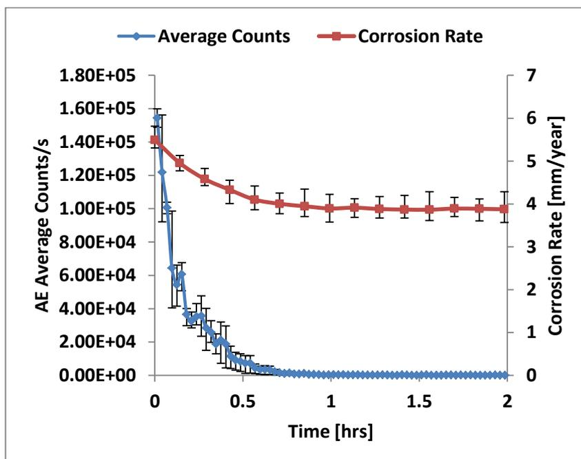
Figure 8.3: Flow-induced corrosion rate with AE count rate for 10 m/s flow in CO<sub>2</sub> saturated brine (pH 5.5) at 50°C. Corrosion rates were obtained from LPR measurement using Stern-Geary Coefficient of 26 mV.
