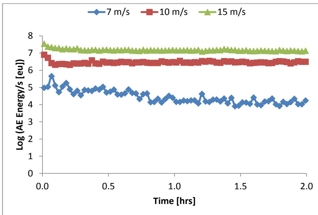
Figure 6.7: Variation of average AE energy with time for different flow velocities and fixed sand loading of 200 mg/L at 90° impingement angle and 50°C temperature in tap-water saturated with N<sub>2</sub> (pH ≈ 7.0).
