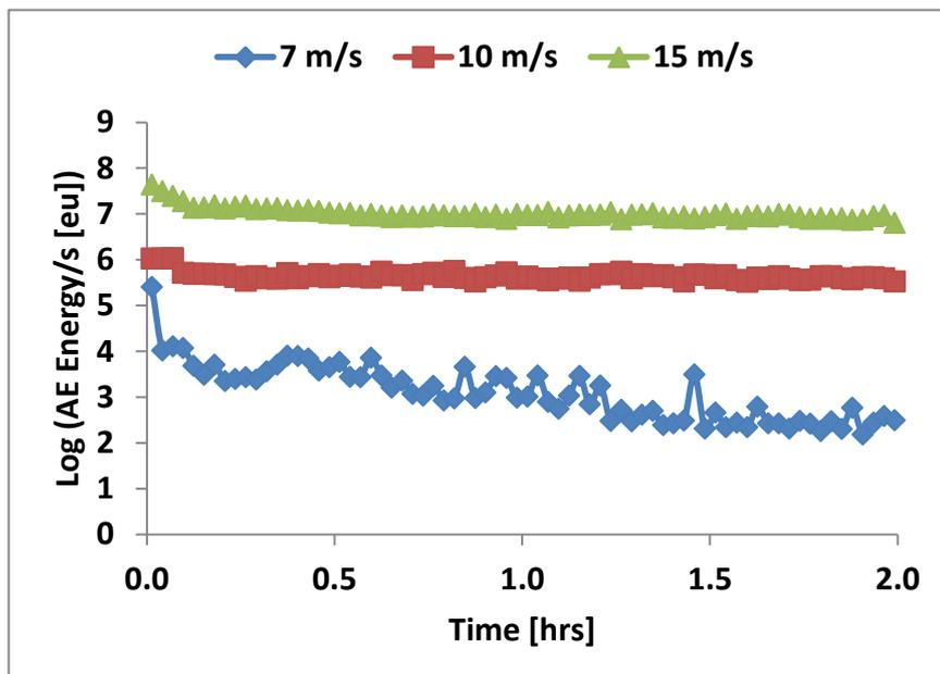
Figure 6.6: Variation of average AE energy with time for different flow velocities and fixed sand loading of 50 mg/L at 90° impingement angle and 50°C temperature in tap-water saturated with N<sub>2</sub> (pH ≈ 7.0).
