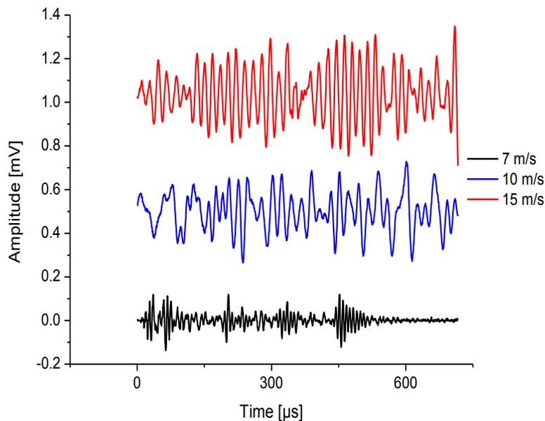
**Figure 6.24: Measured time-domain (waveforms) without sand for 7, 10 and 15 m/s at 90° impingement angle and 50°C temperature in tap-water saturated with N<sub>2</sub> (pH ≈ 7.0).**
