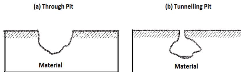
**Figure 2.12: Two types of pitting corrosion attack (a) through pit and (b) tunnelling pit [58].**
