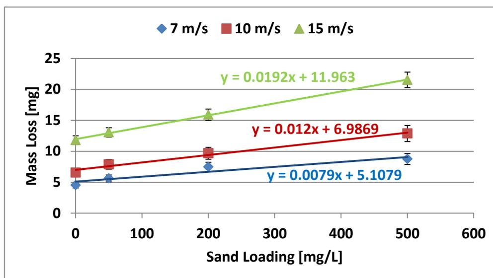
Figure 9.21: Total mass loss vs. sand loading from gravimetric technique.
