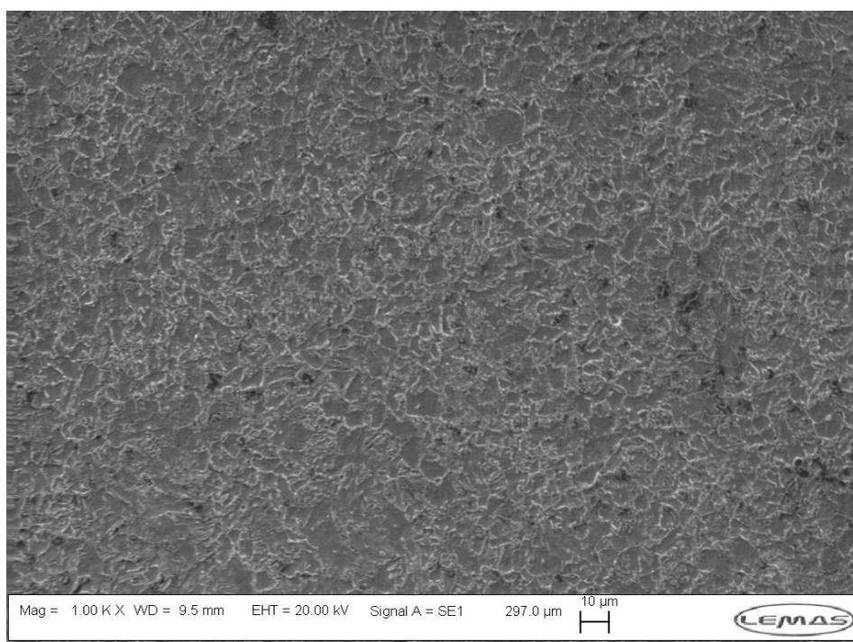
**Figure 9.17: SEM image of X65 carbon steel sample after test for 7 m/s flow velocity without sand revealing  $\text{Fe}_3\text{C}$  on the sample's surface**
