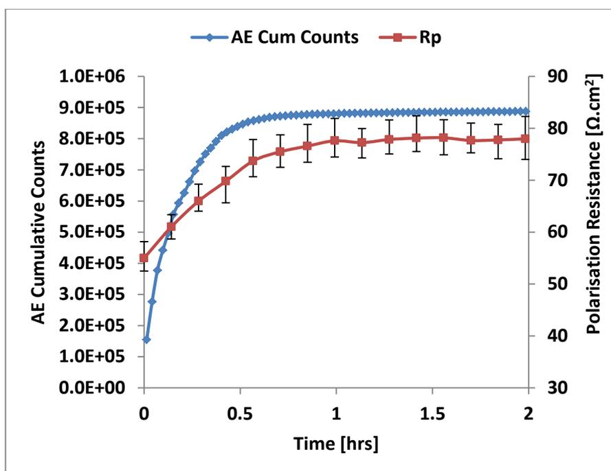
Figure 8.4: Polarisation resistance variation with AE cumulative counts for 10 m/s flow in CO<sub>2</sub> saturated brine (pH 5.5) at 50°C.
