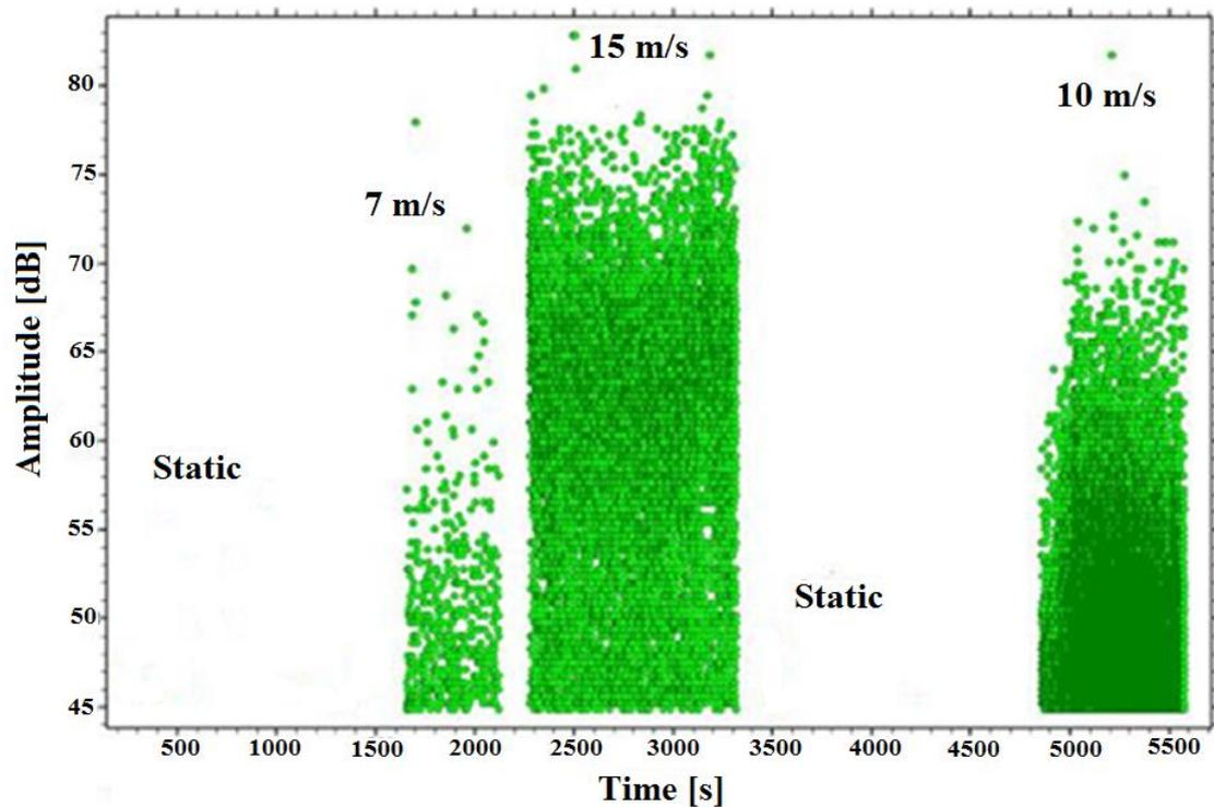
**Figure 5.16: Raw Data of AE test with sand loading for static condition and 7, 10 and 15 m/s flow velocities.**
