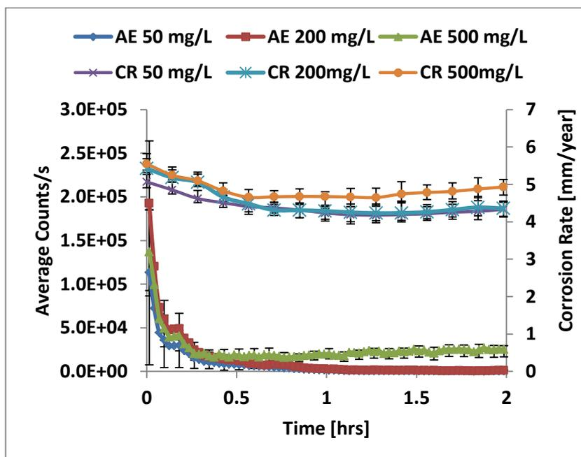
Figure 8.8: Results for erosion-corrosion test showing corrosion rate with AE count rate for 7 m/s in CO<sub>2</sub> saturated brine (pH 5.5) at 50°C. Corrosion rates were obtained from LPR measurement using Stern-Geary coefficient of 26 mV.
