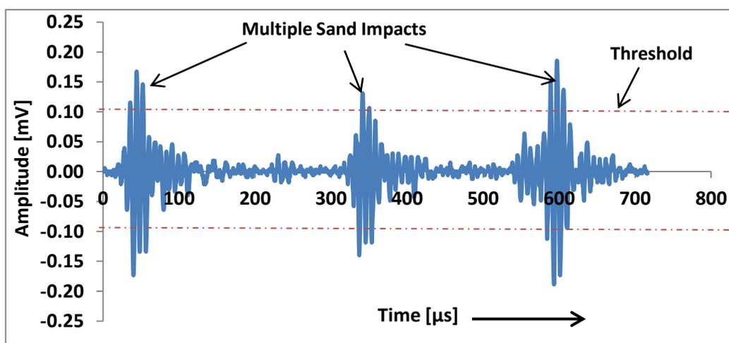
**Figure 6.4: Measured AE signal waveform due to multiple sand impacts at 7m/s flow velocity, 90° impingement angle and 50°C temperature with tap-water saturated with N<sub>2</sub> (pH ≈ 7.0).**
