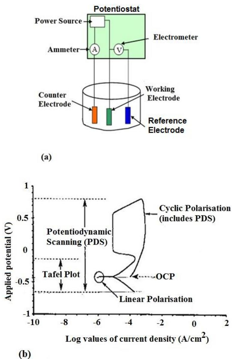
Figure 2.5: (a) Set-up for corrosion test and (b) summary of DC methods.
