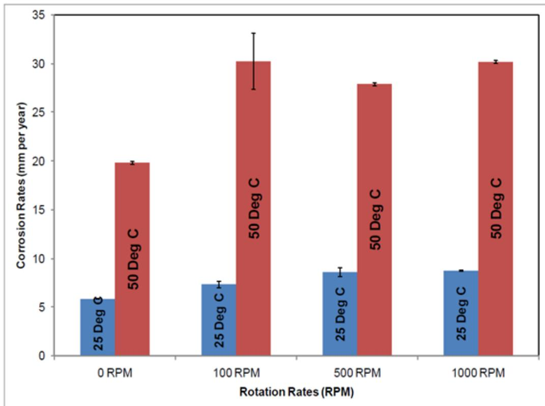
**Figure 3.7: Variation of corrosion rate with flow velocity flow velocity and  $\text{pCO}_2 = 10$  bar at 25°C and 50°C and pH 3 [70].**
