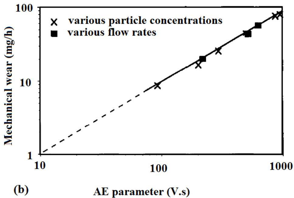
Figure 4.9: (a) AE (RMS) vs. particle K.E and (b) Erosion vs. AE (RMS) [186].
