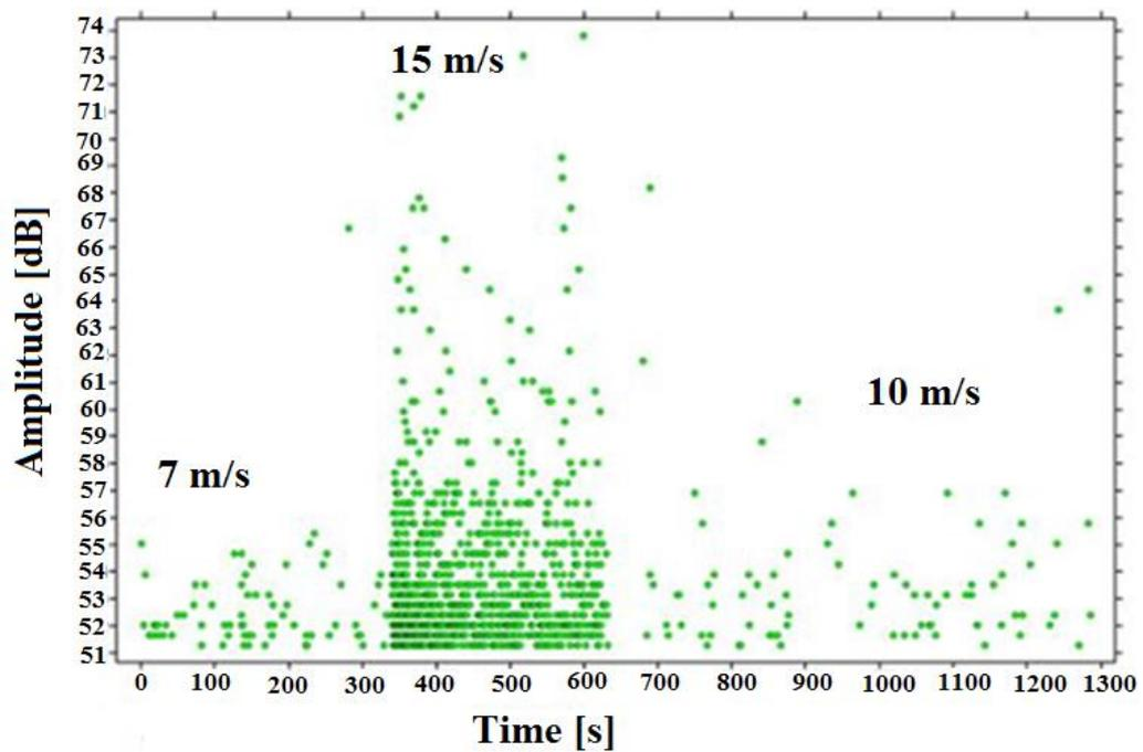
Figure 5.15: Raw data of noise test with pump running at varied flow velocities (7, 10, 15 m/s) and threshold set at 50.9 dB.
