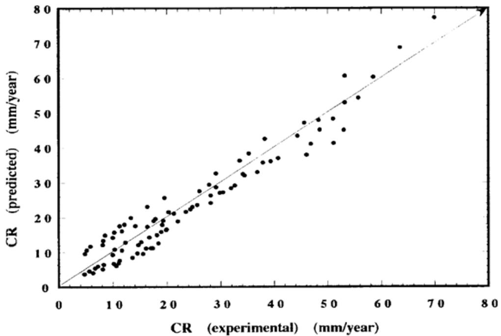
Figure 3.6: Predicted corrosion rate vs. experimental values [76].
