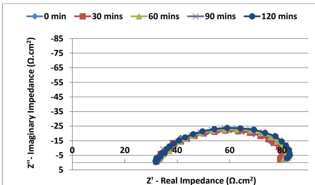
Figure 9.2: Nyquist plot at different exposure times for 10 m/s with process brine without sand, 50°C and CO<sub>2</sub> saturated at 1 bar.
