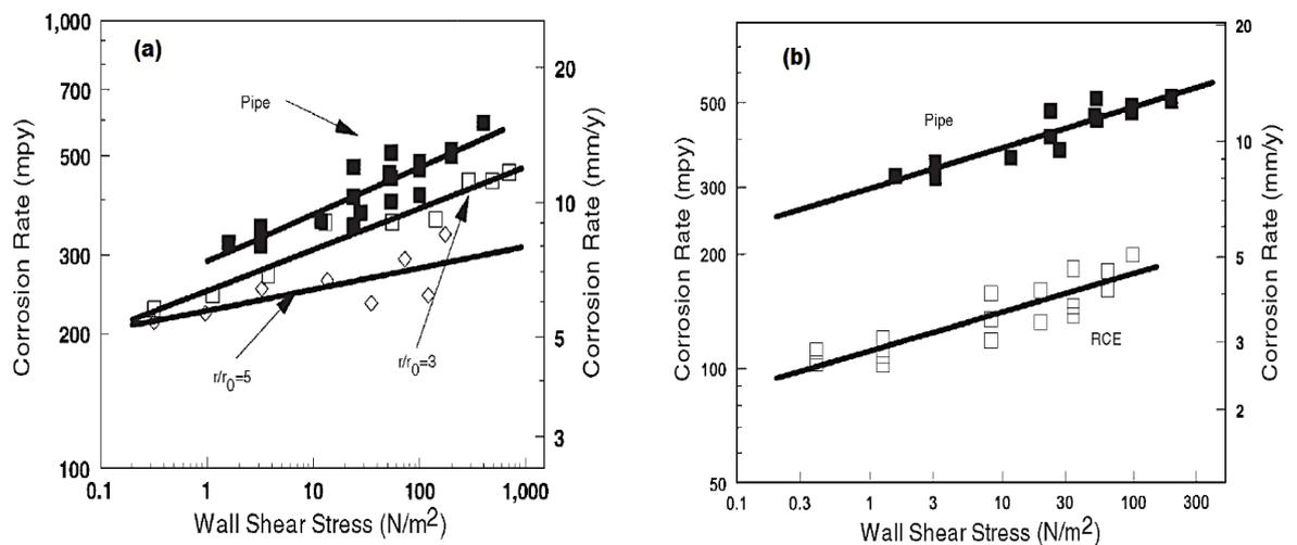
**Figure 3.2: Corrosion rate of carbon steel as a function of wall shear stress value for (a) pipe flow and jet impingement rings at  $r/r_0=3$  and  $r/r_0=5$ , and (b) RCE and pipe flow [74].**
