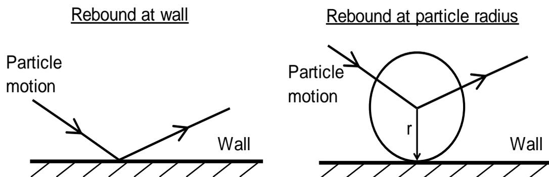
**Figure 7.19: Illustration of particle rebound at wall and rebound at particle radius, with 'r' representing particle radius which was set to 125  $\mu\text{m}$  [110].**
