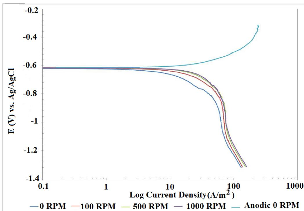
**Figure 3.10: Cathodic polarisation curves at pH 3, 25°C and  $p\text{CO}_2 = 10$  bar [70].**
