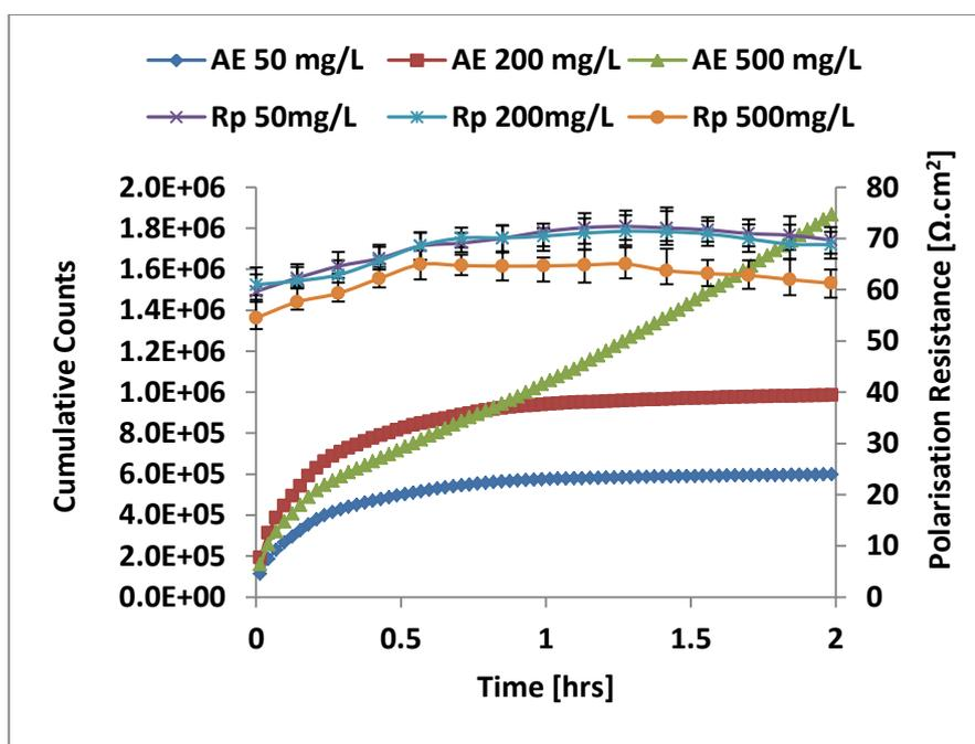
Figure 8.9: Results for erosion-corrosion test showing polarisation resistance variation with AE cumulative counts for 7 m/s in CO<sub>2</sub> saturated brine (pH 5.5) at 50°C.
