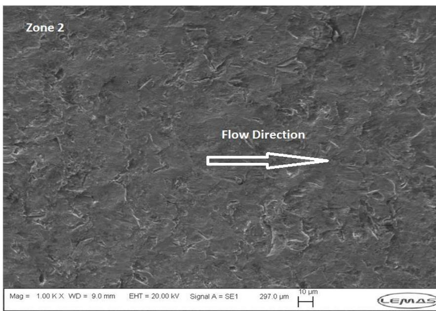
**Figure 6.18: SEM image showing the degradation mechanisms in zone 2, the transition region for 15 m/s flow velocity, 500 mg/L sand and temperature of 50°C in tap-water saturated with N<sub>2</sub> (pH≈7.0).**
