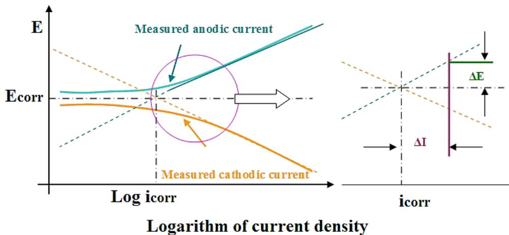
Figure 2.4: Electrochemical corrosion curves [43].
