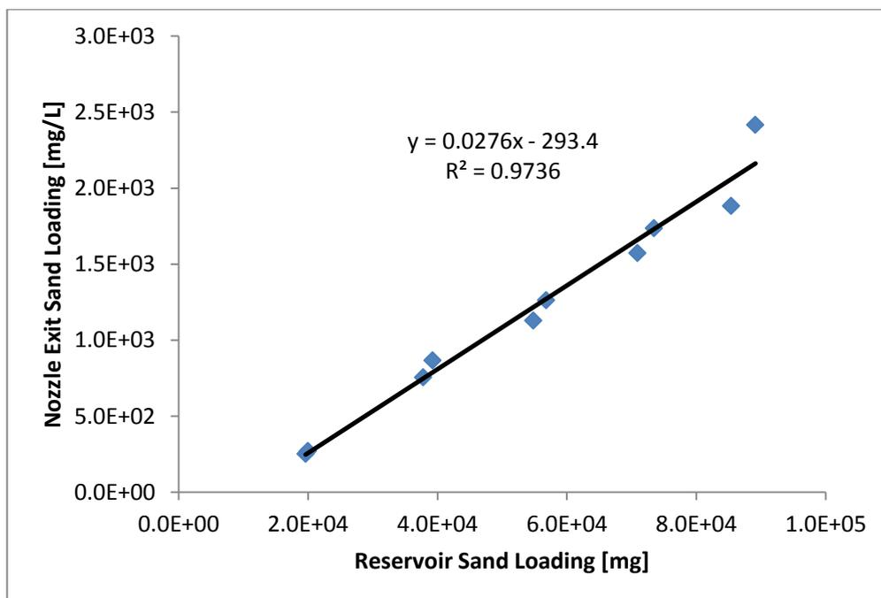
**Figure 5.9: Plot of nozzle exit sand concentration variation with sand loading added to the reservoir during the sand loading calibration for 15 m/s flow velocity.**
