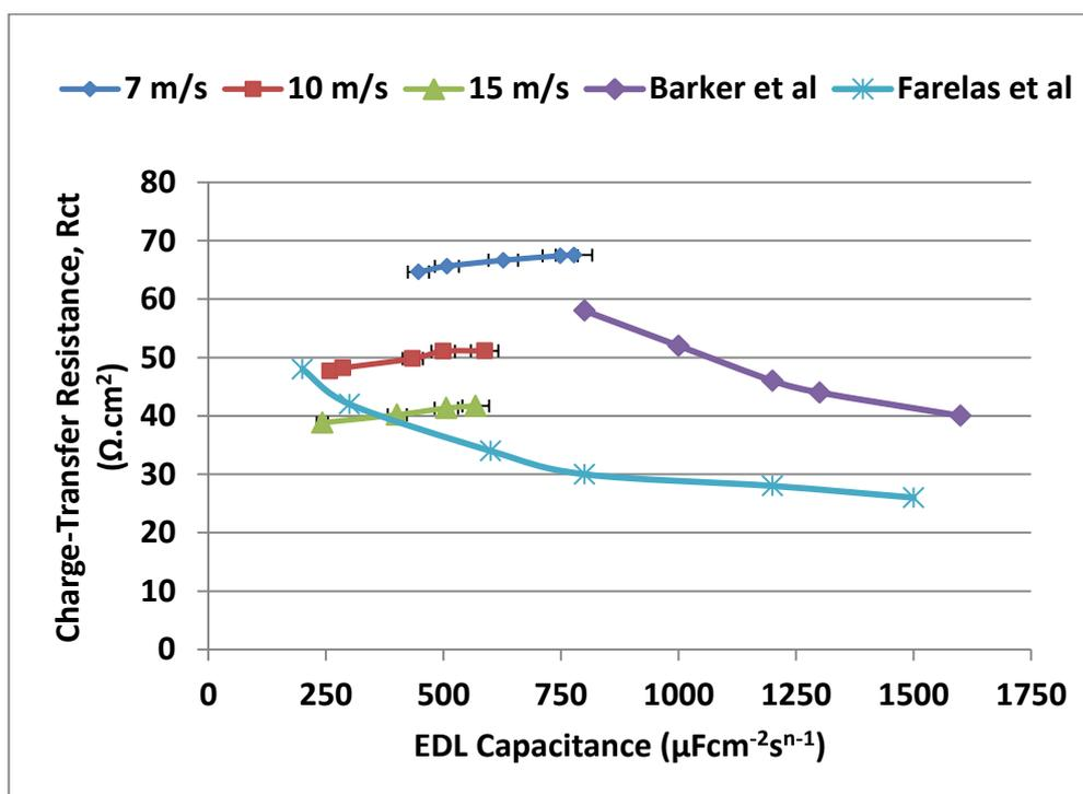
**Figure 9.14: Comparison of the relationship between charge-transfer and EDL capacitance in this study and those from Barker *et al.* [207] and Farelas *et al.* [218].**
