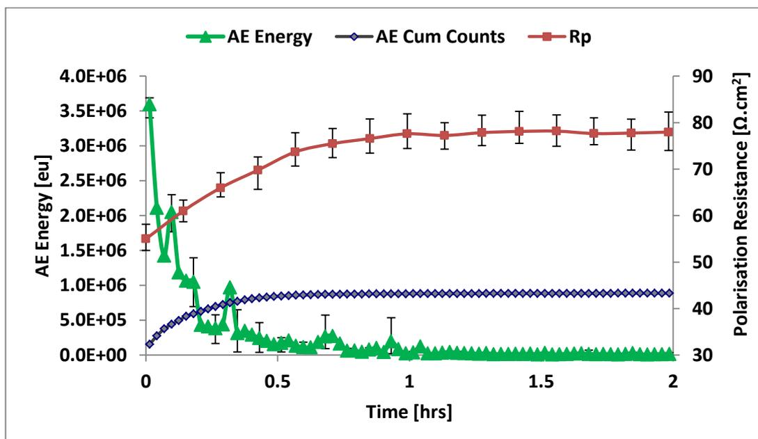
**Figure 8.7: Results of AE Energy and cumulative counts with polarisation resistance for 10 m/s flow in CO<sub>2</sub> saturated brine (pH 5.5) at 50°C. Corrosion rates were obtained from LPR measurement using Stern-Geary coefficient of 26 mV.**
