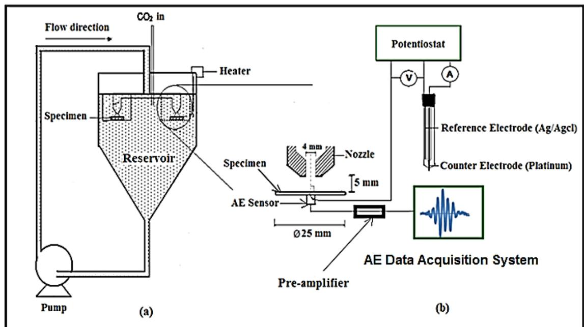
**Figure 5.1: Schematic illustration of experimental rig set-up.**
