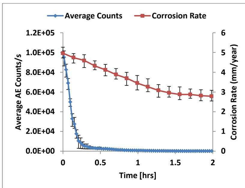
Figure 8.1: Flow-induced corrosion rate variation with AE count rate for 7 m/s flow in CO<sub>2</sub> saturated brine (pH 5.5) at 50°C. Corrosion rates were obtained from LPR measurement using Stern-Geary Coefficient of 26 mV.
