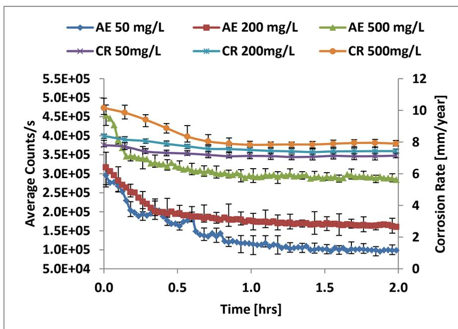
Figure 8.12: Results for erosion-corrosion test showing corrosion rate with AE count rate for 15 m/s in  $\text{CO}_2$  saturated brine (pH 5.5) at  $50^\circ\text{C}$ . Corrosion rates were obtained from LPR measurement using Stern-Geary coefficient of 26 mV.
