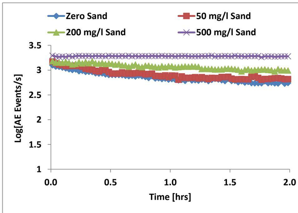
Figure 7.5: AE event count rate for baseline and different sand concentrations for 10 m/s at 90° impingement angle and 50°C temperature in tap-water saturated with N<sub>2</sub> (pH ≈ 7.0).
