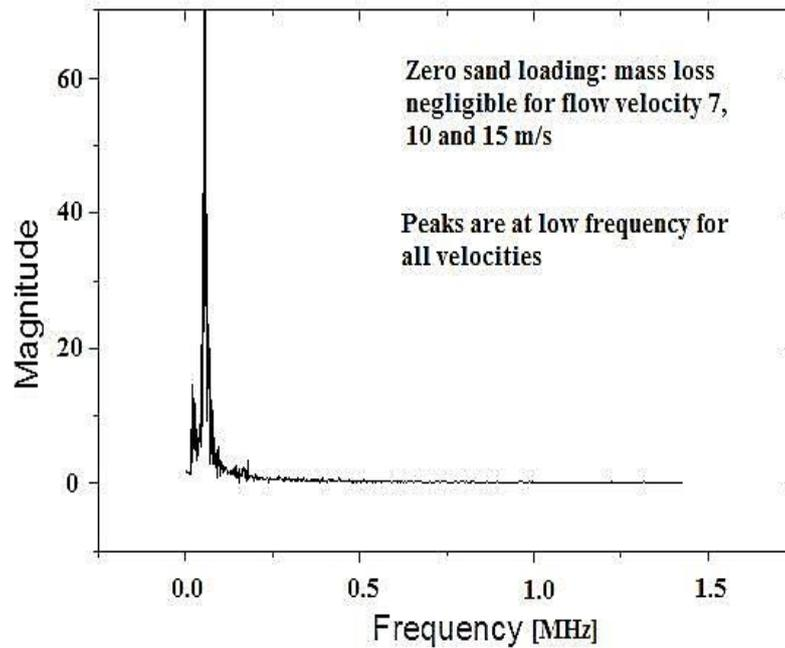
**Figure 6.25: Frequency spectrum of AE waveform without sand at 90° impingement angle and 50°C temperature in tap-water saturated with N<sub>2</sub> (pH ≈ 7.0).**
