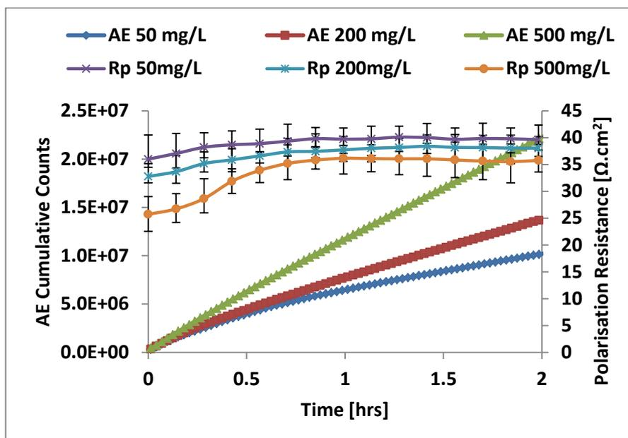
Figure 8.13: Results for erosion-corrosion test showing polarisation resistance variation with AE cumulative counts for 15 m/s in CO<sub>2</sub> saturated brine (pH 5.5) at 50°C.
