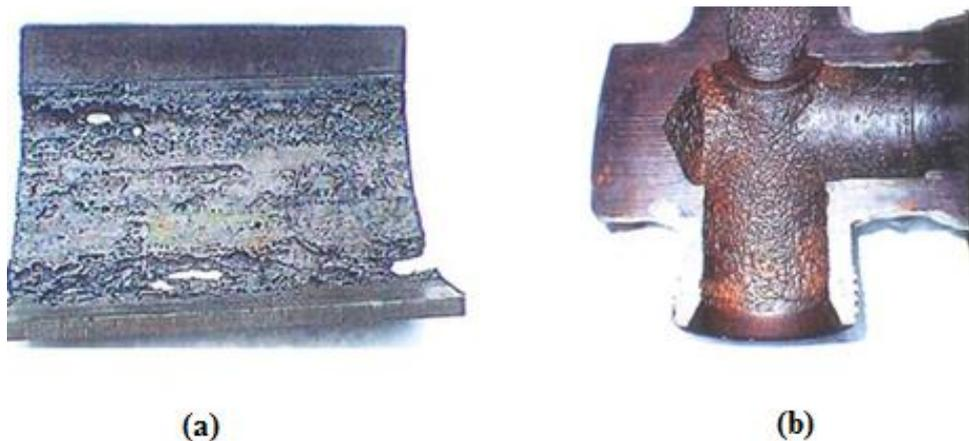
**Figure 1.1: Typical  $\text{CO}_2$  erosion-corrosion damage in (a) X65 carbon steel pipeline and (b) in a choke (a device used to control the flow of fluid in pipelines) [5].**
