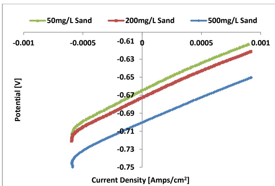
Figure 8.14: LPR data for 15 m/s erosion-corrosion test showing the effect of sand on corrosion potential in CO<sub>2</sub> saturated brine (pH 5.5) at 50°C.
