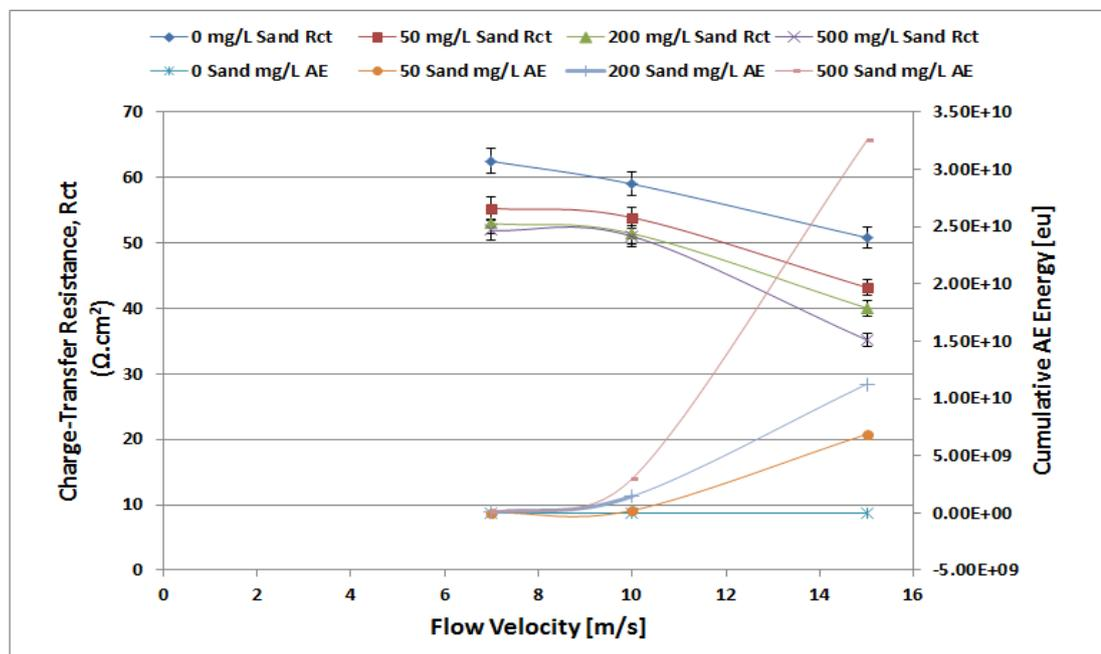
Figure 9.20: The relationship between the charge-transfer resistance and flow velocity (LHS) with Cumulative AE and flow velocity (RHS) for all sand concentrations.
