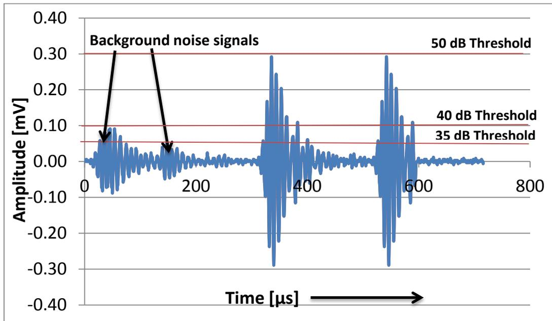
Figure 5.19: Illustration of optimized threshold setting using measured waveform at 7m/s flow velocity, 200 mg/L sand loading, 90° impingement angle and 50°C temperature with tap-water saturated with N<sub>2</sub> (pH ≈ 7.0).
