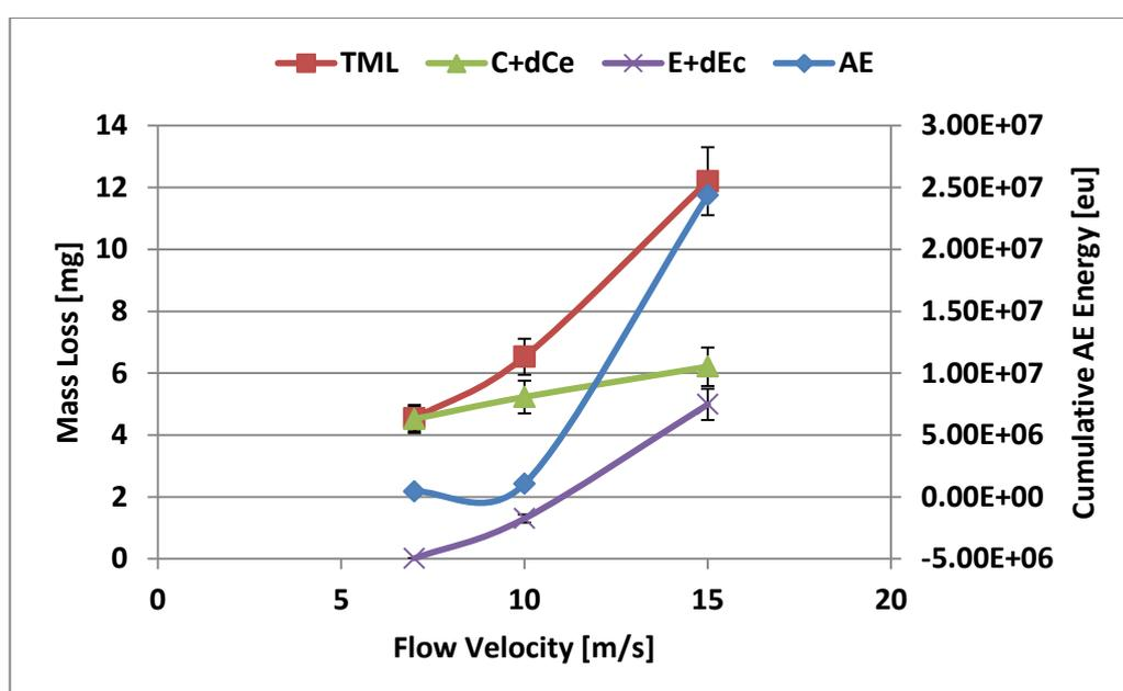
**Figure 9.23: Total erosion-corrosion damage with its components and measured cumulative AE Energy for 2 hours expressed in energy unit [eu, 1eu =1E-18J] for all the flow velocities investigated without sand.**
