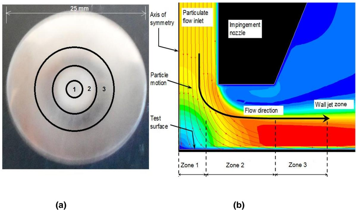
**Figure 6.16: (a) Surface wear zones on tested specimen, (b) CFD prediction of the zones**
