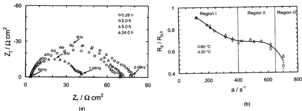
**Figure 9.19: (a) Nyquist plot and (b) AC impedance parameter as a function of hydrodynamic constant by Orazem and Filho [229].**
