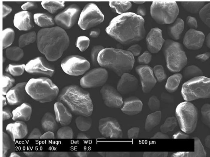
Figure 5.5: Sand particles' shape and sizes from Scanning Electron Microscopy (SEM).
