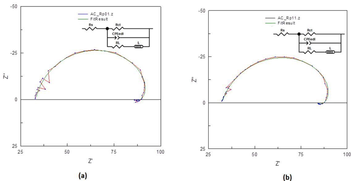
**Figure 9.12:** Illustration of the fit of the model (green line) with the experimental data (red line) for 7 m/s at (a) the beginning of the test and (b) end of the test.
