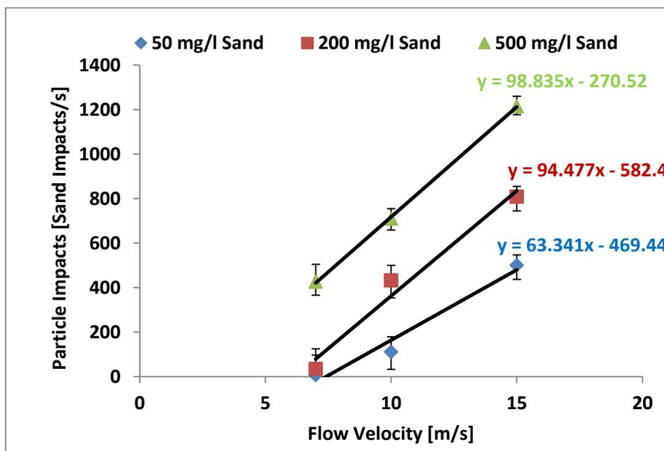
Figure 7.11: Variation of particle impacts with time for different sand concentrations and flow velocities at 90° impingement angle and 50°C temperature with tap-water saturated with N<sub>2</sub> (pH ≈ 7.0).
