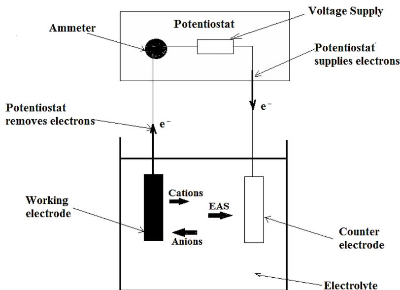
**Figure 2.6: Schematic illustration of current flow during polarisation [52].**
