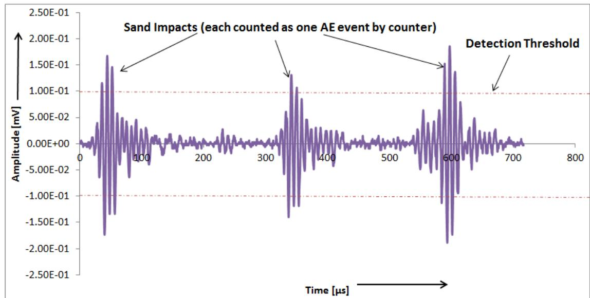
**Figure 7.3: Measured AE signal waveform due to multiple sand impacts at 7m/s flow velocity, 90° impingement angle and 50°C temperature with tap-water saturated with N<sub>2</sub> (pH ≈ 7.0).**
