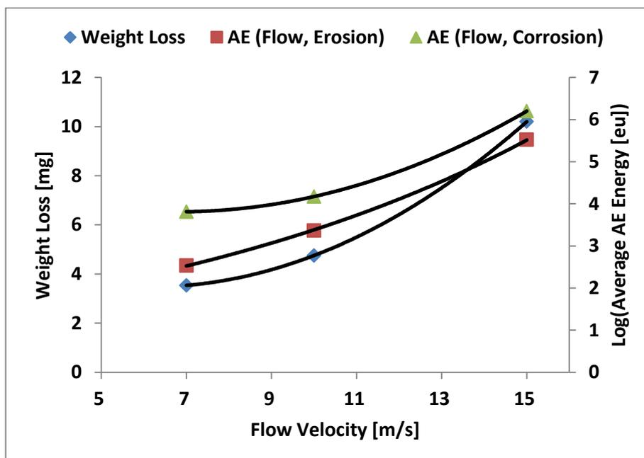
Figure 8.17: Results of the total weight loss with measured average AE energy in energy units ([eu],  $1\text{eu}=1\text{E}-18\text{J}$ ) in the presence and absence of corrosion for 0 mg/L sand concentration.
