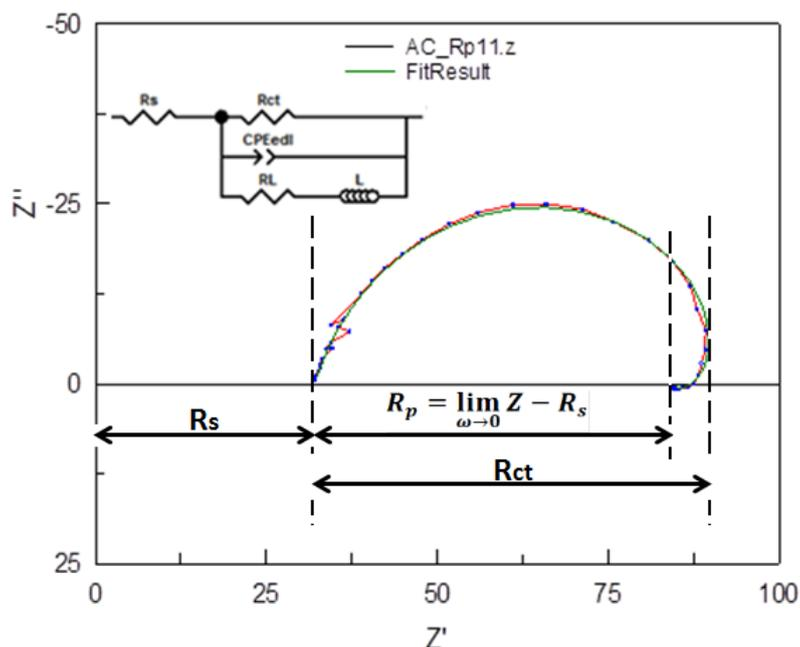
**Figure 9.22: Estimation of  $R_p$  and  $R_{ct}$  from EIS data with inductive loop.**
