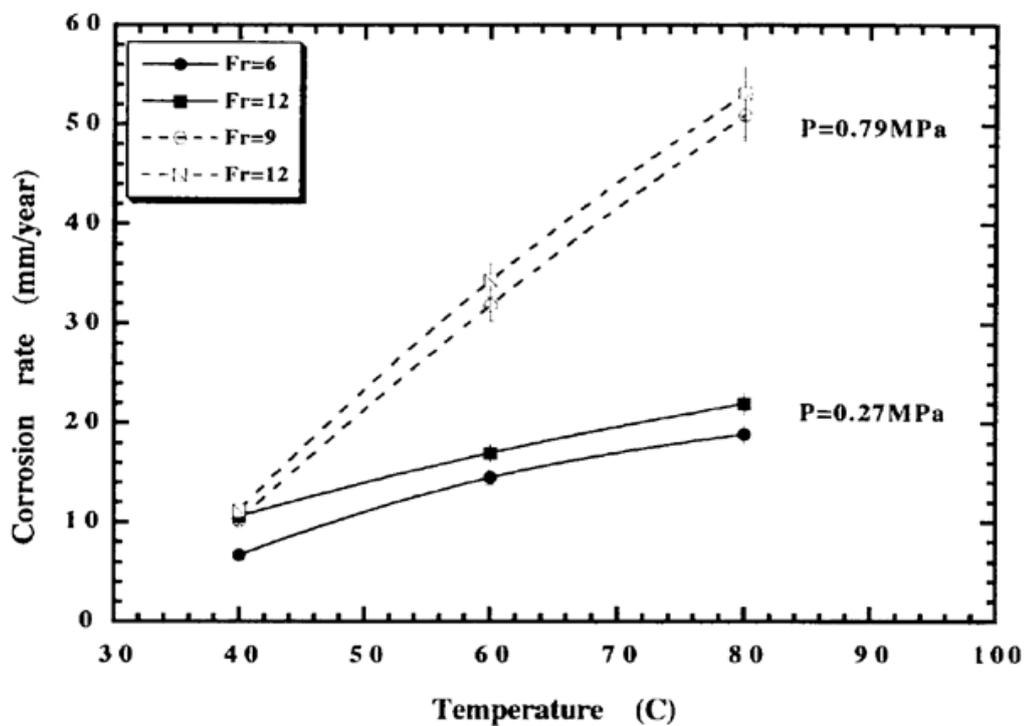
Figure 3.4: Corrosion rate vs. temperature for 80% water cut [76].
