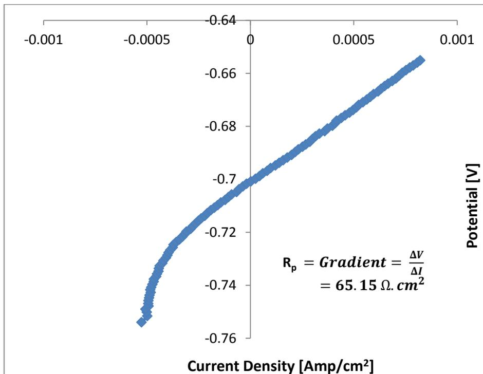
Figure 6.14: LPR data of X65 carbon steel under impingement at 90° impact angle, 50°C and 10 m/s flow velocity with brine saturated with CO<sub>2</sub> (pH=5.5).
