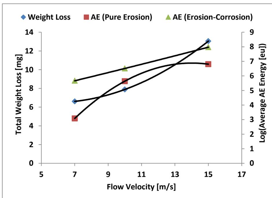
Figure 8.18: Results of the total weight loss with measured average AE energy in energy units ([eu],  $1\text{eu}=1\text{E}-18\text{J}$ ) in the presence and absence of corrosion for 50 mg/L sand concentration.
