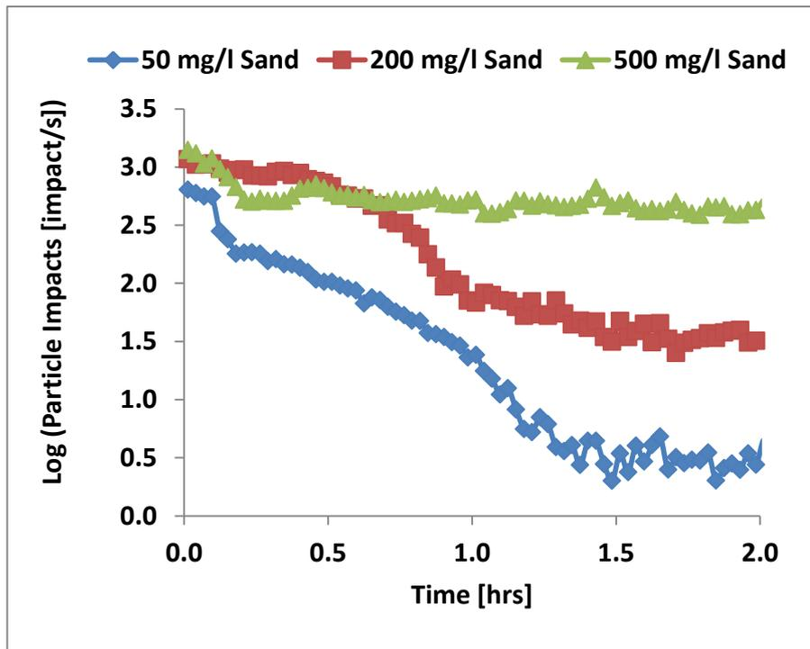
Figure 7.8: Variation of particle impacts with time for different sand concentrations for 7 m/s all at 90° impingement angle and 50°C temperature in tap-water saturated with N<sub>2</sub> (pH ≈ 7.0).
