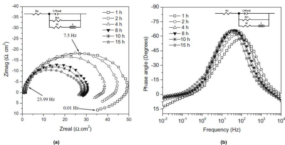
Figure 9.16: (a) Nyquist and (b) phase plots by Farelas *et al.* [218] for C1018 steel in 3% NaCl saturated with  $\text{CO}_2$  under 0.5 m/s flow velocity and 45°C.
