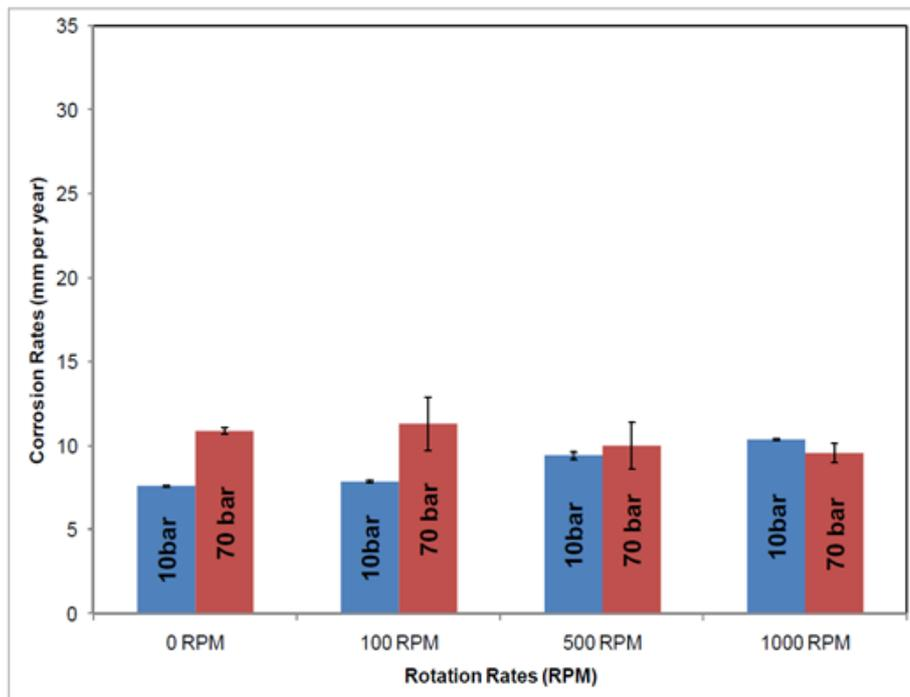
Figure 3.9: Variation of corrosion rate with flow velocity and  $p\text{CO}_2 = 10$  and 70 bar at  $25^\circ\text{C}$  [70].
