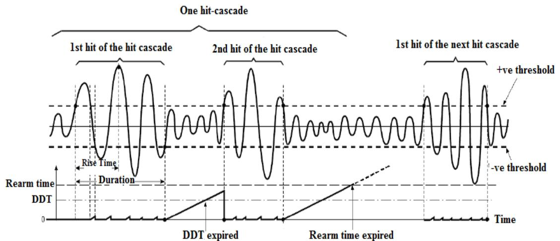
**Figure 7.1: Schematic illustration of duration discrimination time (DDT) [192].**
