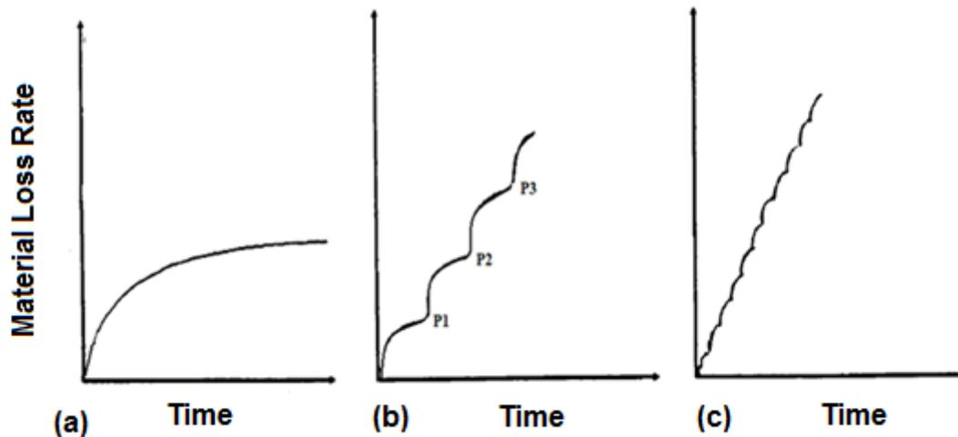
**Figure 3.18: Illustration of erosion-corrosion mechanism [136].**
