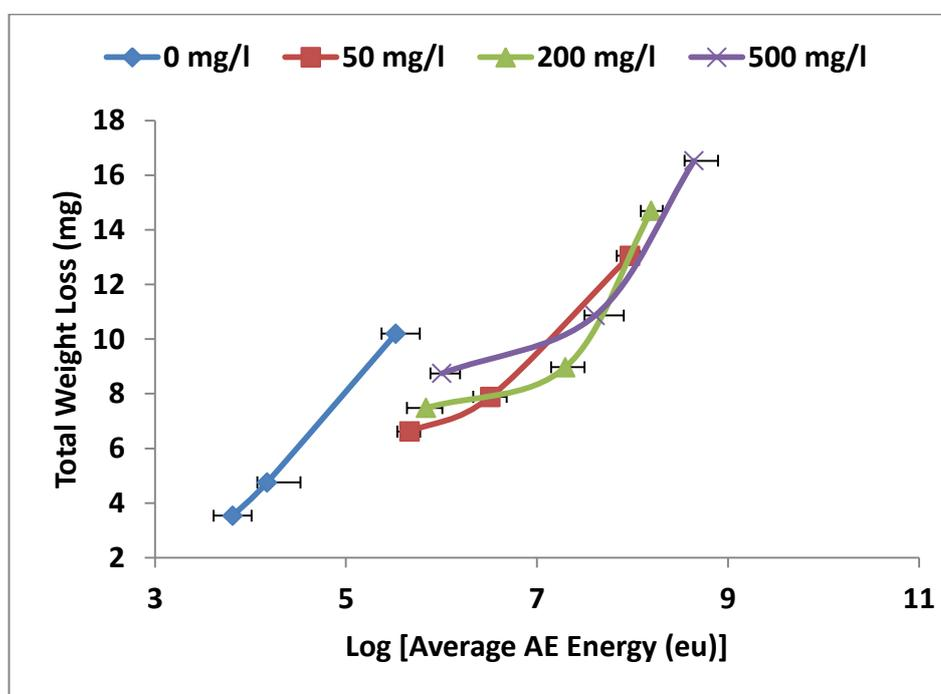
Figure 8.21: Relationship between total weight loss and measured average AE energy for CO<sub>2</sub> flow-induced corrosion and erosion-corrosion (1eu=1E-18J).
