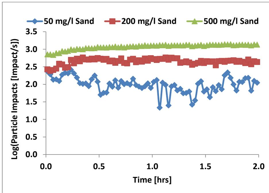
Figure 7.9: Variation of particle impacts with time for different sand concentrations for 10 m/s all at 90° impingement angle and 50°C temperature in tap-water saturated with N<sub>2</sub> (pH ≈ 7.0).
