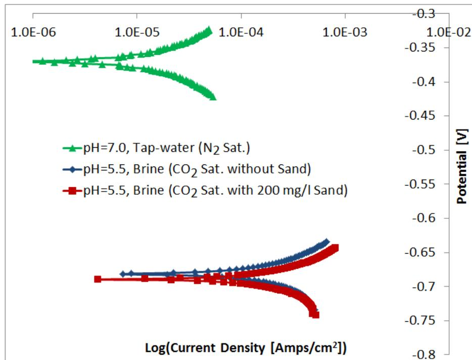
Figure 6.12: Polarization behaviour of X65 carbon steel under impingement at 90° impact angle, 50°C and 10 m/s flow velocity with process brine saturated with CO<sub>2</sub> (pH=5.5) and tap-water saturated with N<sub>2</sub> (pH≈7.0).
