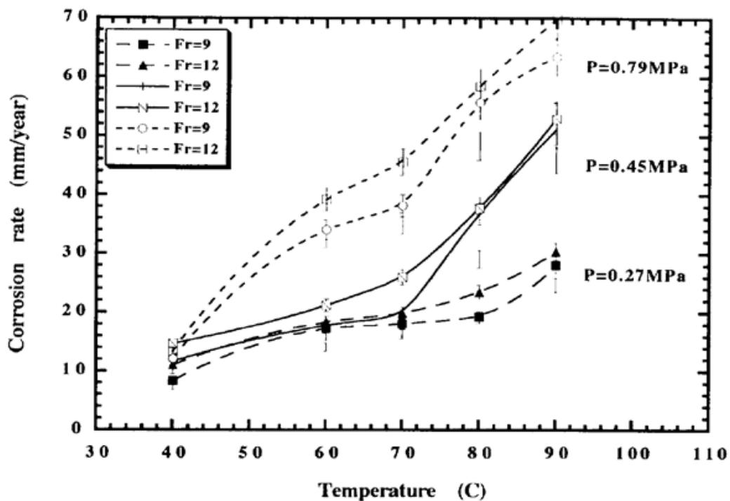
Figure 3.3: Corrosion rate vs. temperature for brine [76].
