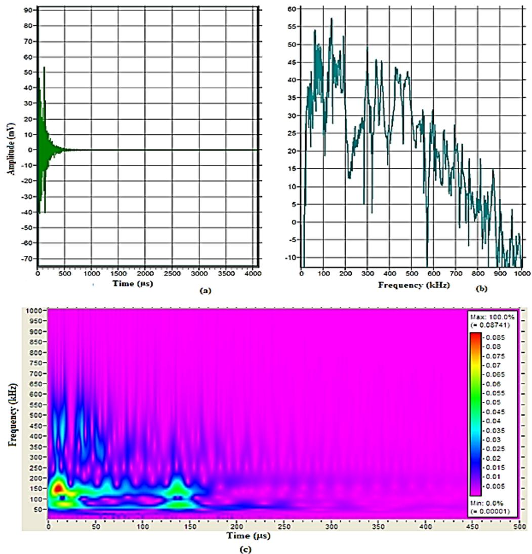
**Figure 5.13: Lead pencil break signal results in (a) time-domain, (b) frequency-domain and (c) frequency-time domain.**
