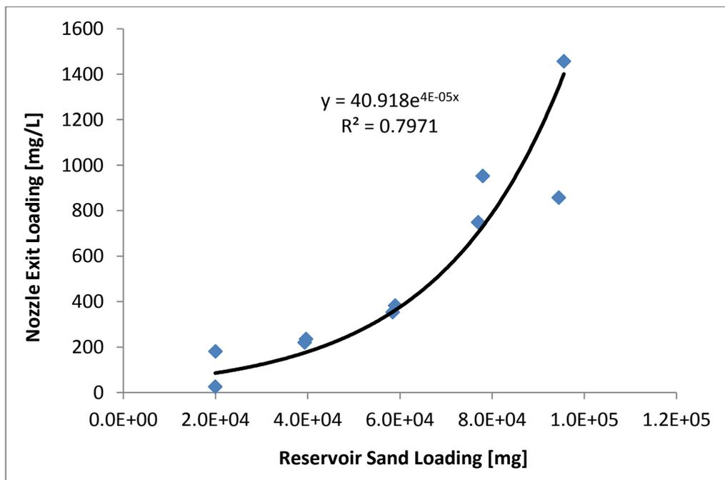
Figure 5.8: Plot of nozzle exit sand concentration variation with sand loading added to the reservoir during the sand loading calibration for 10 m/s flow velocity.
