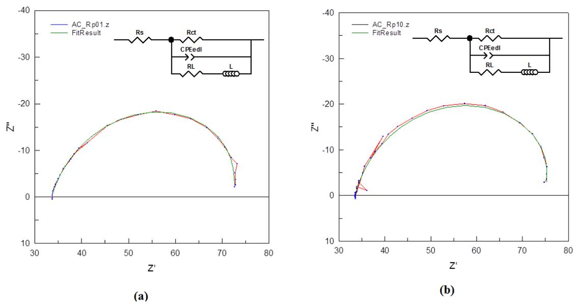
**Figure 9.13:** Illustration of the fit of the model (green line) with the experimental data (red line) for 10 and 15 m/s at (a) the beginning of the test and (b) end of the test.
