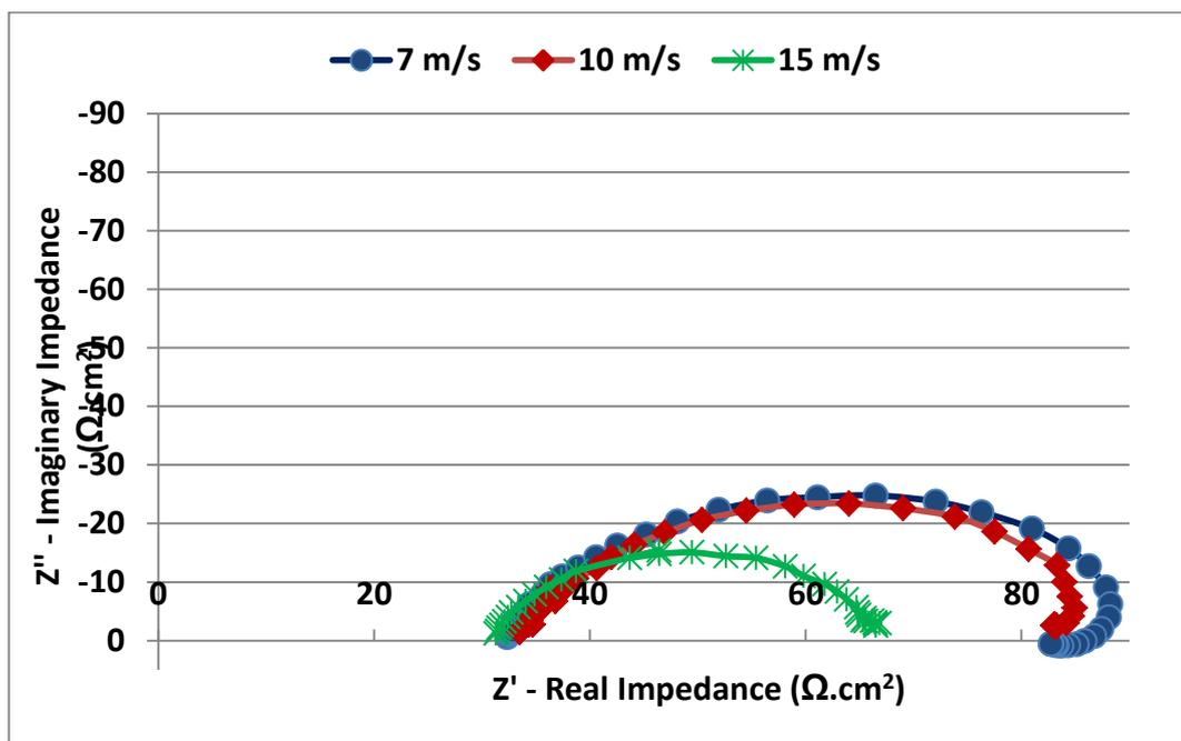
Figure 9.9: Nyquist plots after 2 hours for 7, 10 and 15 m/s flow velocities. Test conditions: process brine, 500 mg/L sand loading, 50°C and CO<sub>2</sub> saturated at 1 bar.
