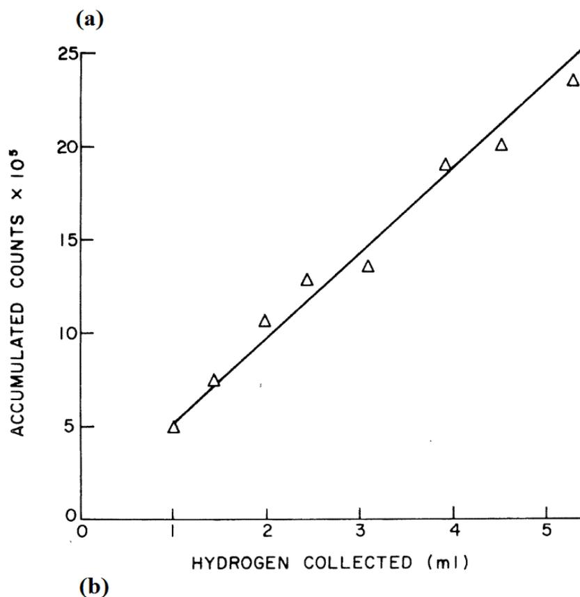
Figure 4.5: Schematic illustration of (a) AE output from the apparatus and (b) correlation of hydrogen generation with Acoustic Emission [155].
