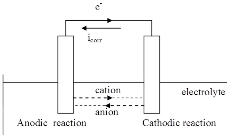
**Figure 2.1: Schematic illustration of the components of a corrosion cell [43].**
