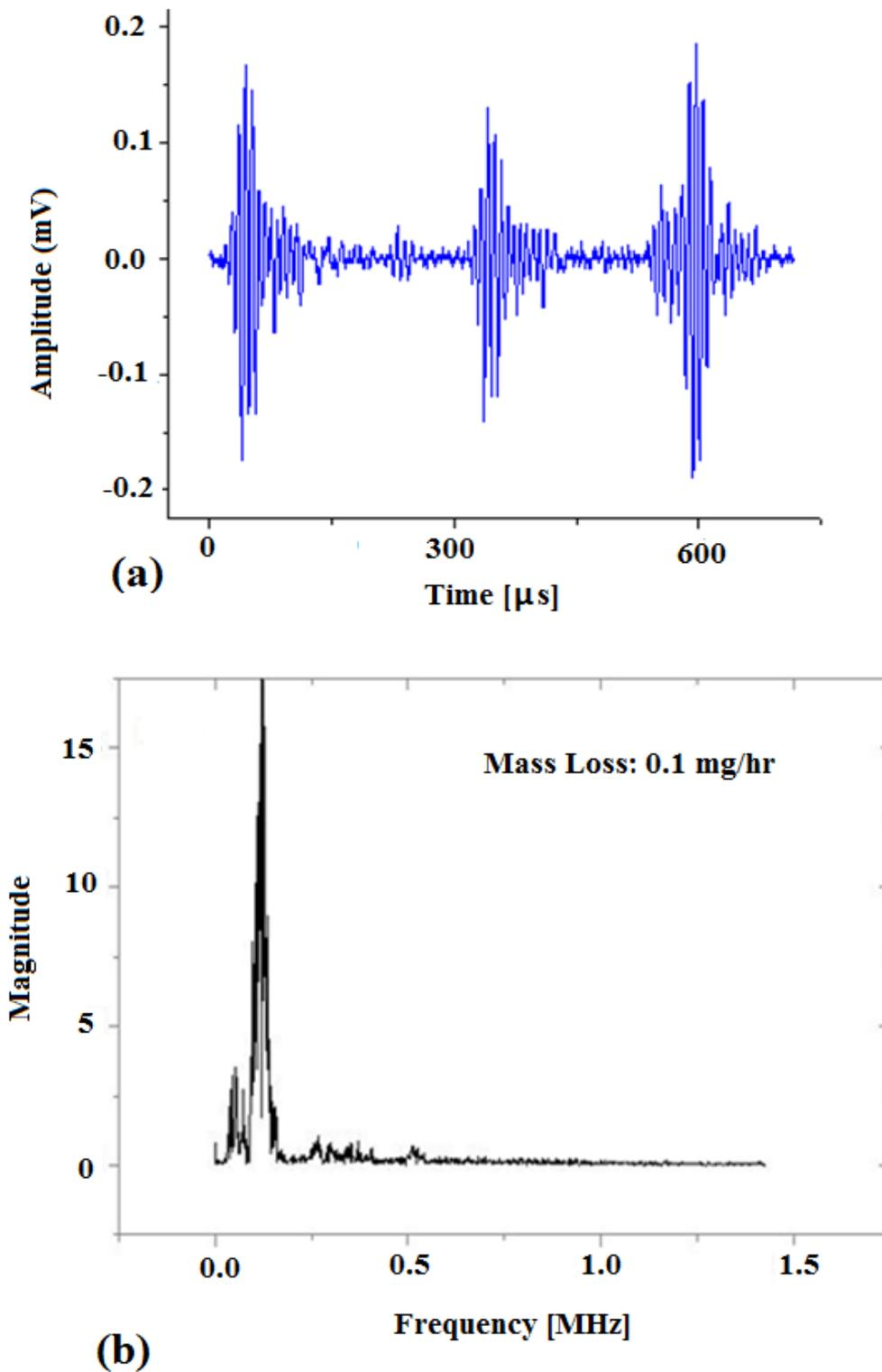
Figure 6.26: (a) Measured AE waveform (time-domain) and (b) frequency-domain for 7 m/s flow velocity, 200 mg/L sand loading at  $90^\circ$  impingement angle and  $50^\circ\text{C}$  temperature in tap-water saturated with  $\text{N}_2$  ( $\text{pH} \approx 7.0$ ).
