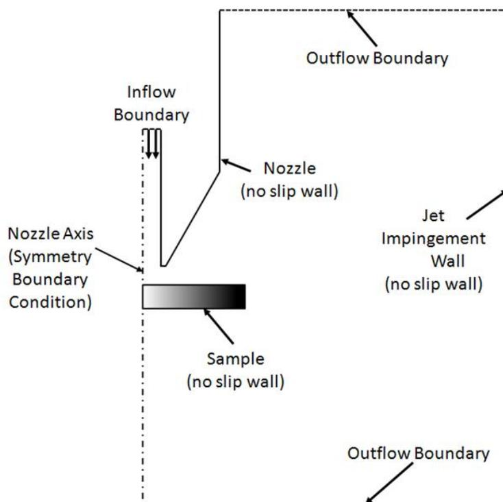
**Figure 7.18: The geometry of the SIJ with boundary conditions and computational domain developed using Gambit.**
