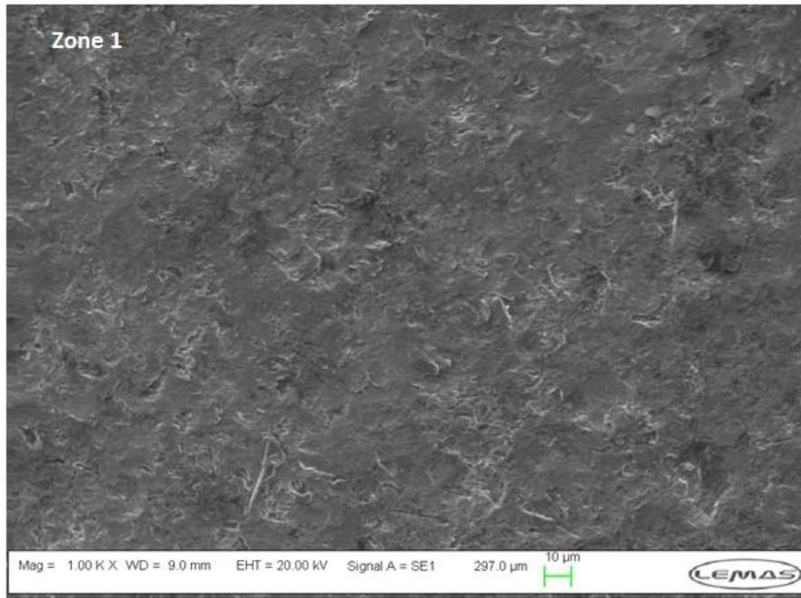
**Figure 6.17: SEM image showing the degradation mechanisms of zone 1, the stagnation region for 15 m/s flow velocity, 500 mg/L sand and temperature of 50°C in tap-water saturated with N<sub>2</sub> (pH≈7.0).**
