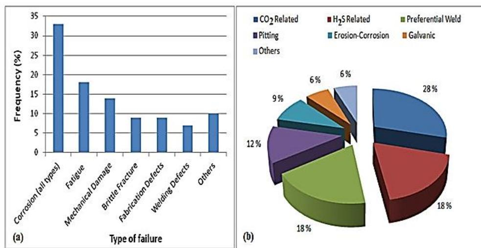
**Figure 1.2 (a) Survey of selected number of failures and (b) causes of corrosion related failures in oil and gas related industries [8].**
