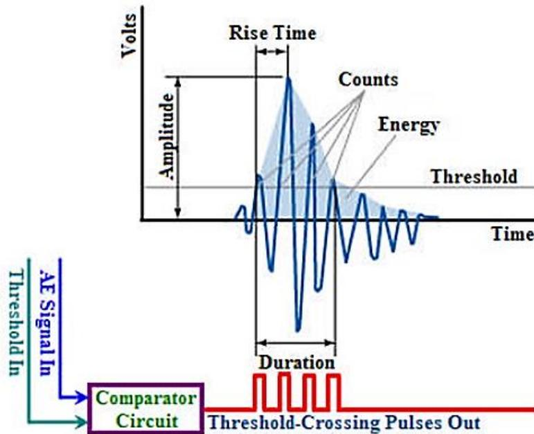
Figure 4.3: Illustration of count and energy of AE signal [154].
