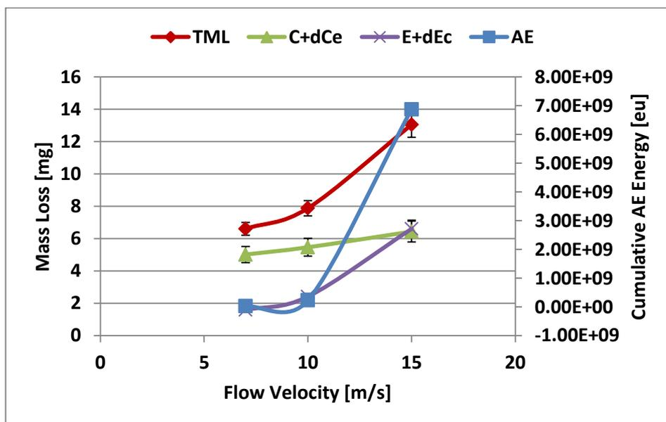
Figure 9.24: Total erosion-corrosion damage with its components and measured cumulative AE Energy for 2 hours expressed in energy unit [eu, 1eu =1E-18J] for all the flow velocities investigated with 50 mg/L sand loading.
