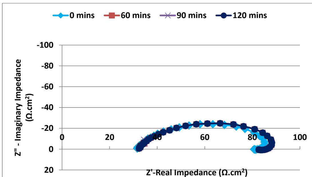
Figure 9.6: Nyquist plot at different exposure times for 7 m/s with process brine, 500 mg/L sand loading, 50°C and CO<sub>2</sub> saturated at 1 bar.
