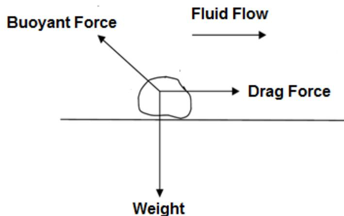
**Figure 3.13: Schematic illustration of the major forces acting on a solid particle within a flowing fluid [83]**
