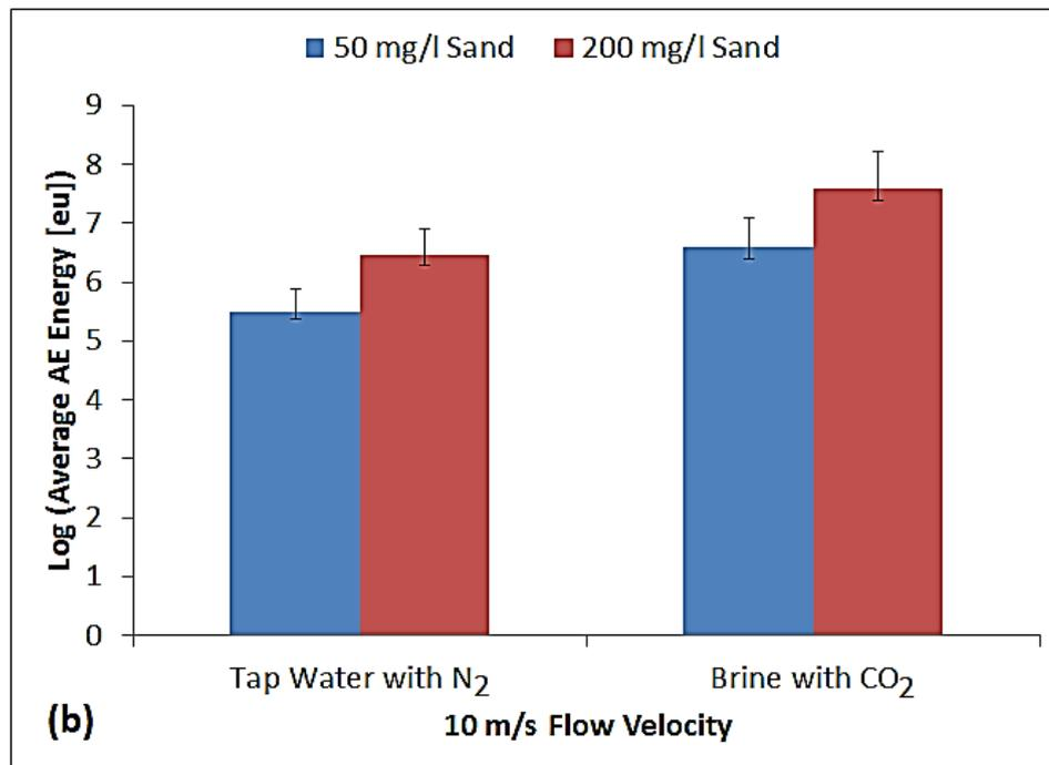
Figure 6.15: Comparison of X65 behaviour in corrosive and inert environment using (a) total weight loss and (b) average AE energy.
