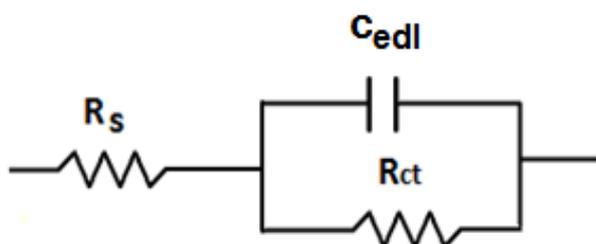
**Figure 2.7: Simple electrical circuit having electrical properties similar to an EDL [43].**
