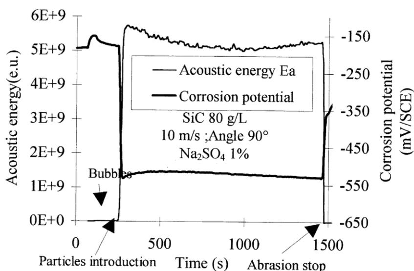
**Figure 4.12: Simultaneous variation of acoustic energy and corrosion potential for high abrasion rate [173].**
