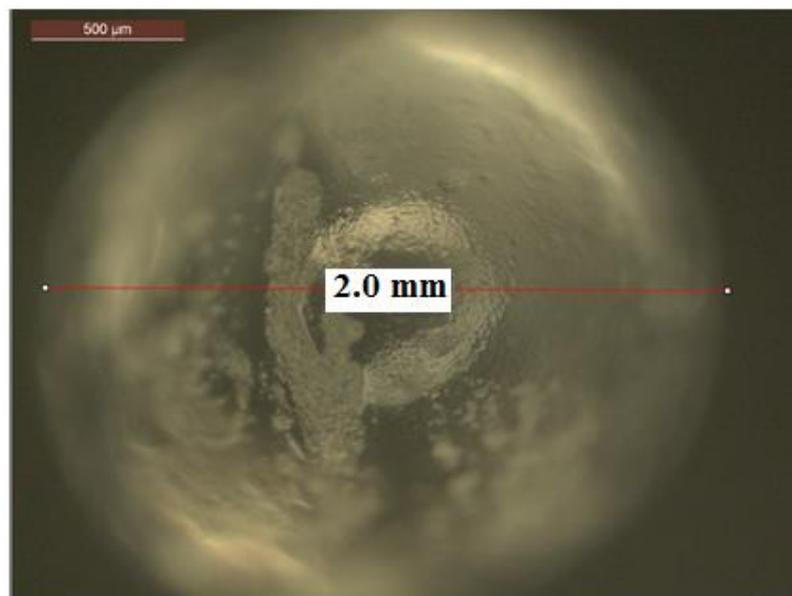
**Figure 6.1: Optical microscope image of the spherical glass bead**
