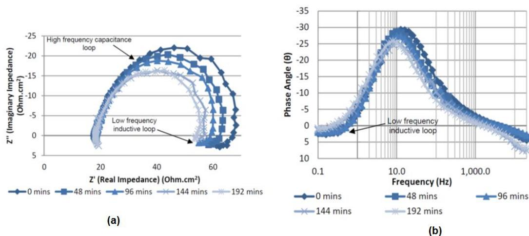
Figure 9.15: (a) Nyquist and (b) phase plots by Barker *et al.* [207] for ASTM A106 grade B carbon steel in oilfield process brine under 7 m/s flow velocity, 45°C and  $\text{CO}_2$  saturated at 1 bar.
