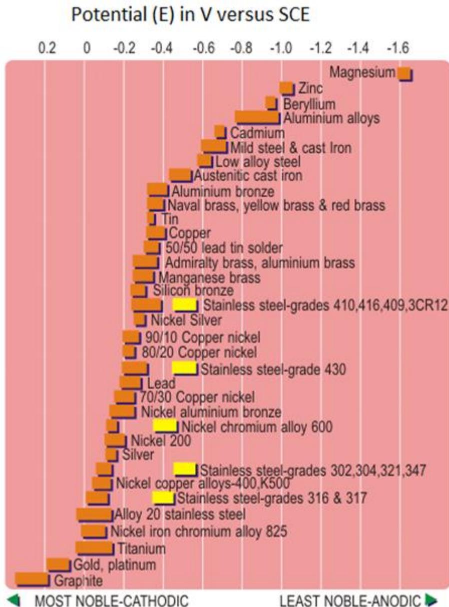
**Figure 2.14: Galvanic series of metals and alloys according to ASTM 982-98.**
