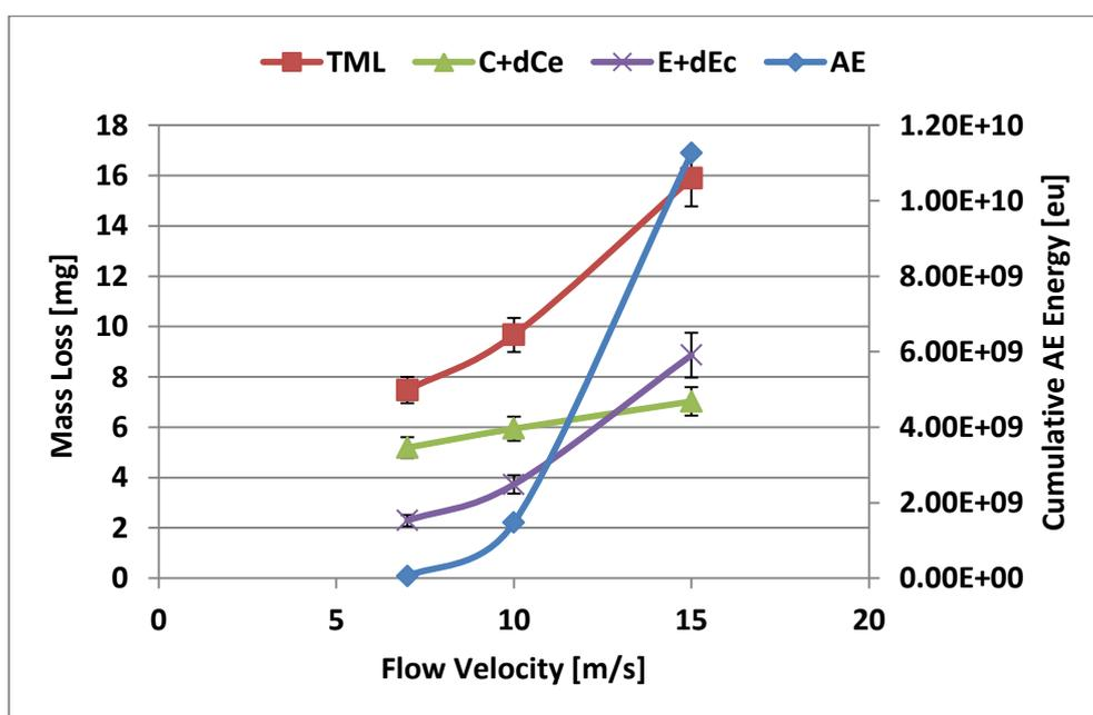
Figure 9.25: Total erosion-corrosion damage with its components and measured cumulative AE Energy for 2 hours expressed in energy unit [eu, 1eu =1E-18J] for all the flow velocities investigated with 200 mg/L sand loading.
