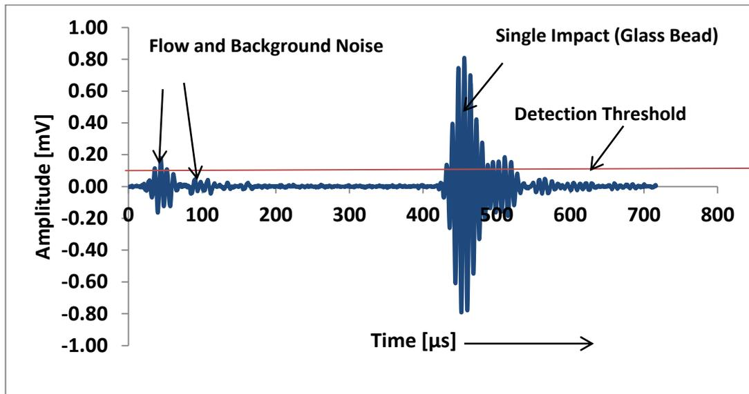
Figure 6.2: Measured AE signal waveform due to glass bead with flow and background noise at 7m/s flow velocity, 90° impingement angle and 50°C temperature with tap-water saturated with N<sub>2</sub> (pH ≈ 7.0).
