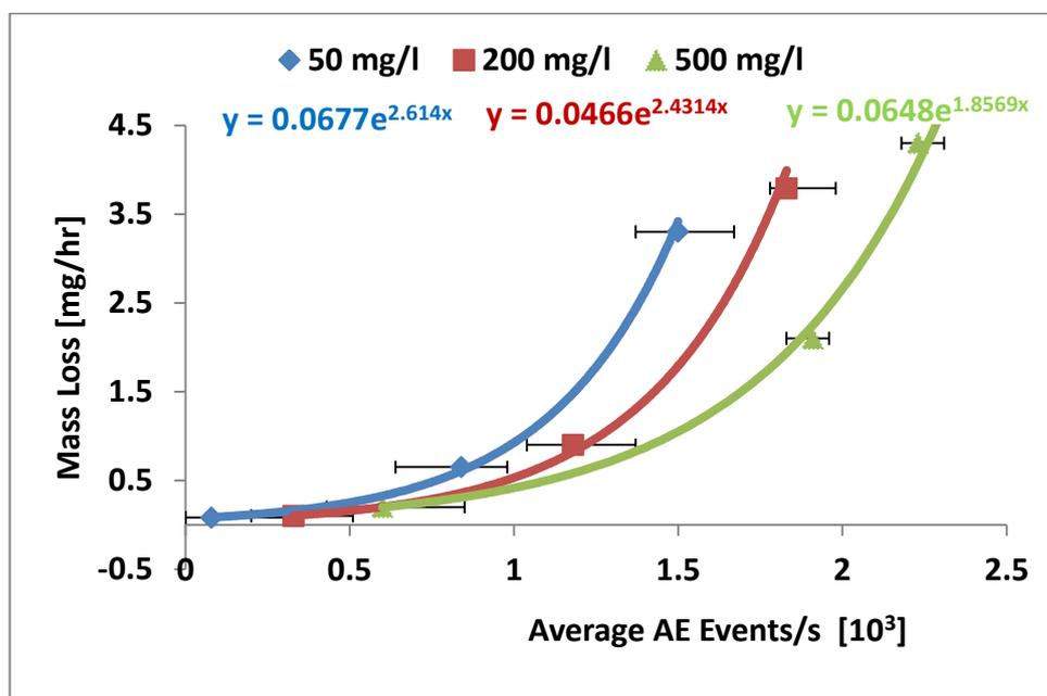
**Figure 7.25: Relationship between mass loss and AE event count per second. Tests performed at  $90^\circ$  impingement angle and  $50^\circ\text{C}$  temperature in tap-water saturated with  $\text{N}_2$  ( $\text{pH} \approx 7.0$ ).**
