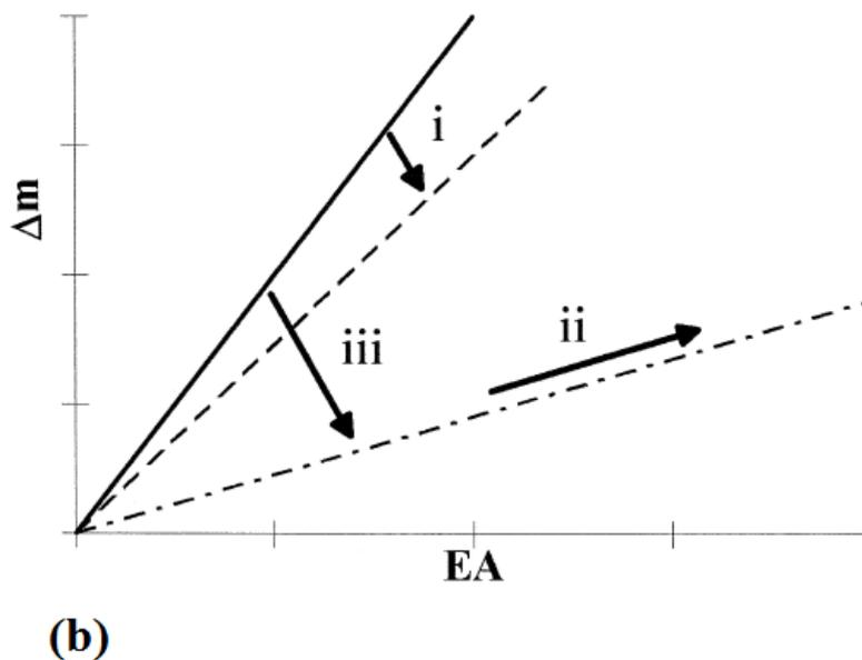
Figure 4.10: Illustration of (a) AE energy vs. particle K.E for different impingement angles and (b) Weight loss vs. AE energy for increasing flow velocities (i), increasing particle loading (ii) and increasing impingement angle (iii) [187].
