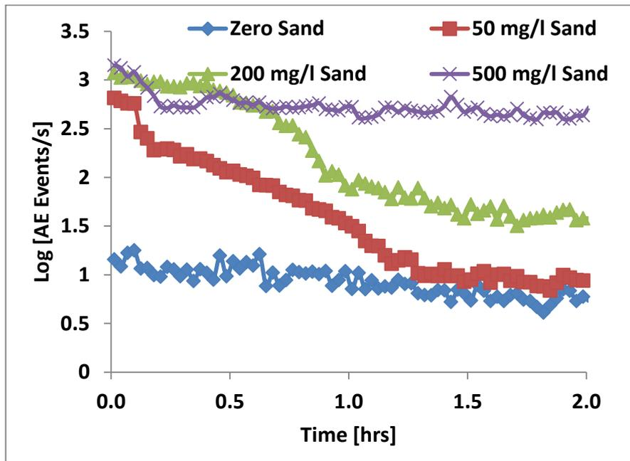
Figure 7.4: AE event count rate for baseline and different sand concentrations for 7 m/s at 90° impingement angle and 50°C temperature in tap-water saturated with N<sub>2</sub> (pH ≈ 7.0).
