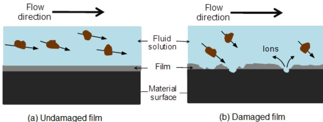
**Figure 3.16: Illustration of (a) undamaged corrosion product film preventing corrosion loss and (b) enhancement of corrosion loss due to particle impacts removing the corrosion product film [110].**
