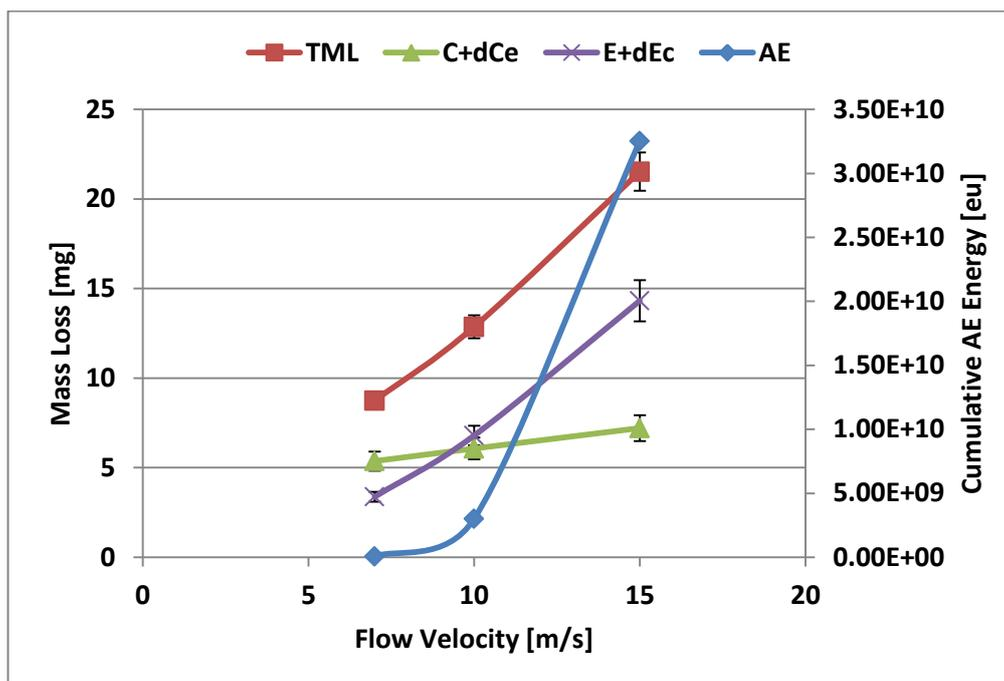
**Figure 9.26: Total erosion-corrosion damage with its components and measured cumulative AE Energy for 2 hours expressed in energy unit [eu, 1eu =1E-18J] for all the flow velocities investigated with 500 mg/L sand loading.**
