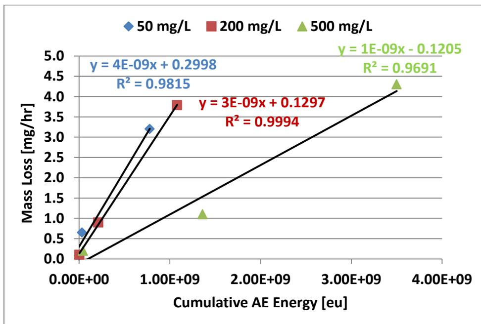
Figure 6.22 Relationship between mass loss and cumulative AE energy for the flow velocities and sand loading investigated with tap-water saturated with N<sub>2</sub>.
