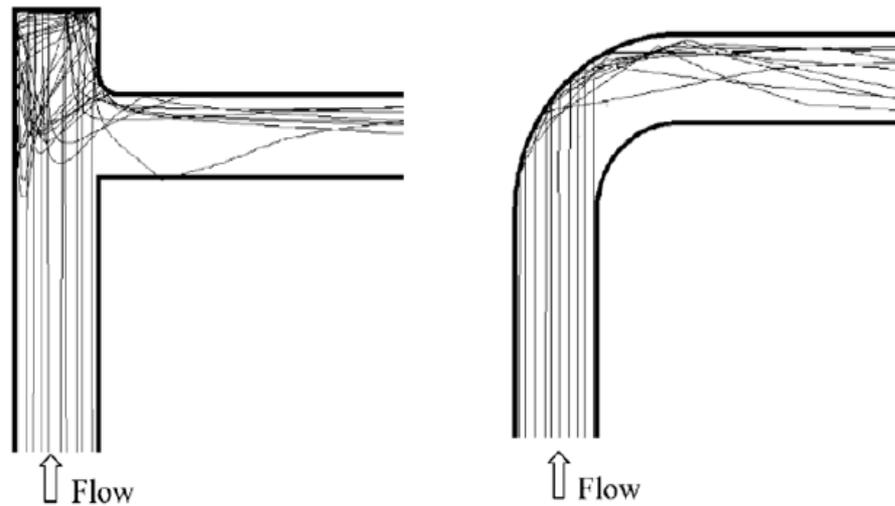
**Figure 3.15: An illustration of predicted particle impact trajectories in a plugged tee and elbow [108].**
