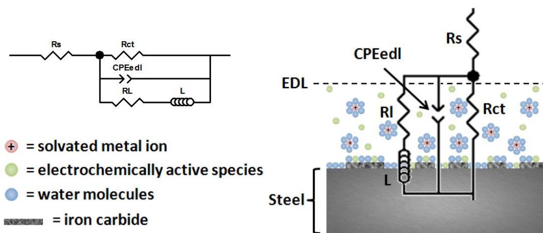
**Figure 9.11: Equivalent circuit used for modelling the EIS data:  $R_s$  is the solution resistance,  $CPE_{edl}$  is a constant phase element describing the capacitance of the electric double layer,  $R_l$  is the inductive resistance,  $L$  is the inductance and  $R_{ct}$  is the charge-transfer resistance [207].**
