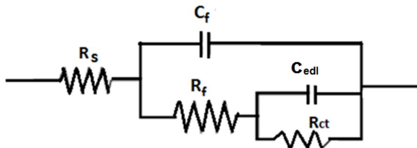
**Figure 2.10: Equivalent circuit with two time constants used to model a corroding, coated metal.  $C_{edl}$  is the EDL capacitance.  $R_{ct}$  is the charge-transfer resistance,  $C_f$  is the capacitance of the film,  $R_f$  is the resistance of the film and  $R_s$  is the solution resistance [43].**
