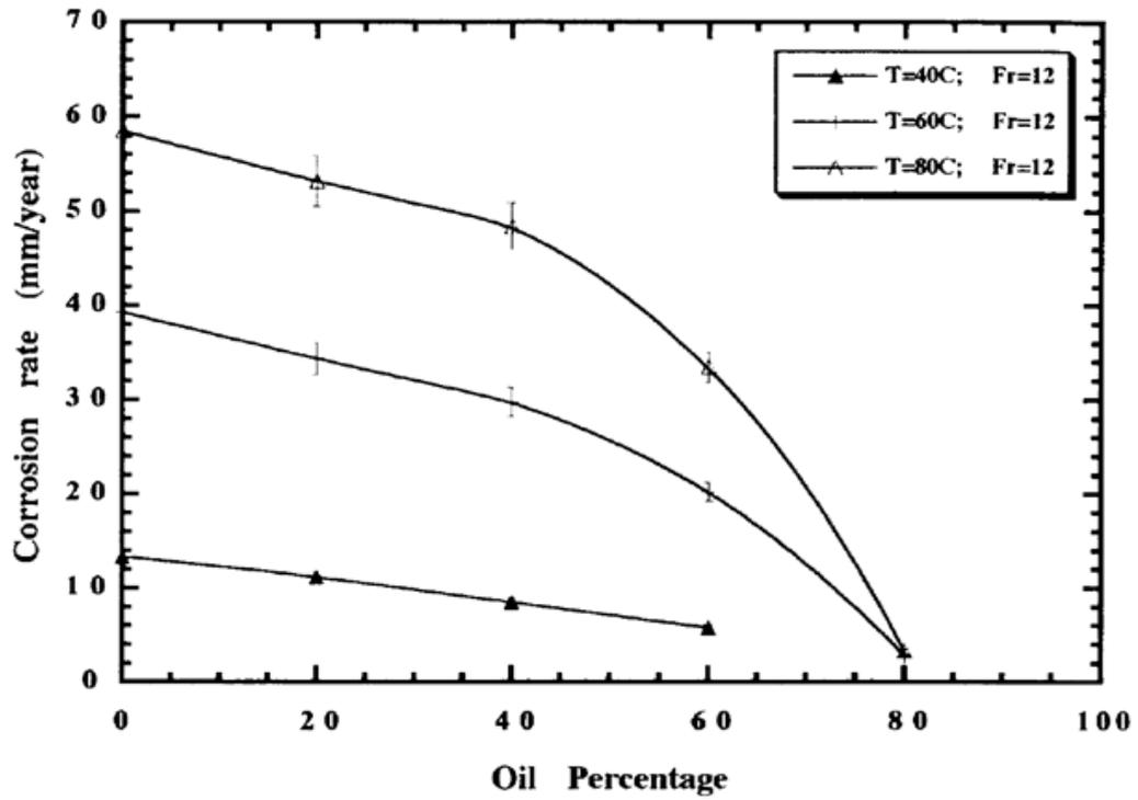
Figure 3.5: Corrosion rate vs. oil composition at  $\text{CO}_2$  partial pressure of 0.79 MPa and Froude number of 12 [76].
