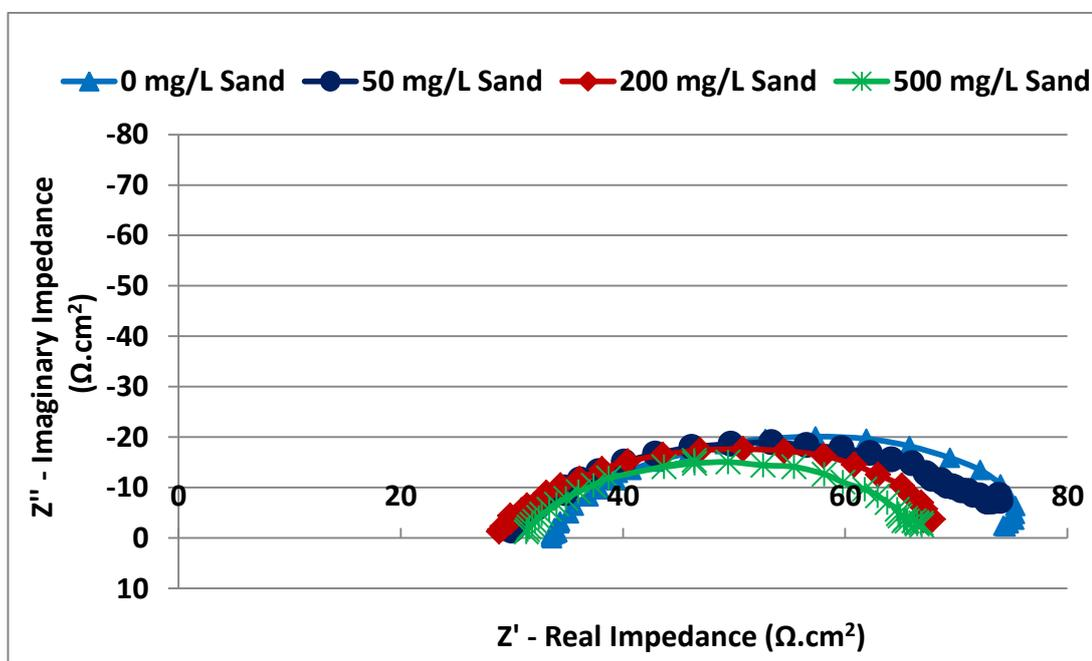
Figure 9.10: Nyquist plot after 2 hours for 15 m/s flow velocity with different sand concentrations. Test conditions: Process brine, 50°C and CO<sub>2</sub> saturated at 1 bar.
