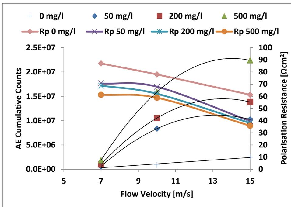
**Figure 8.16: Summary of results for polarisation resistance and AE cumulative Counts. Tests with brine saturated with CO<sub>2</sub> at 1bar.**
