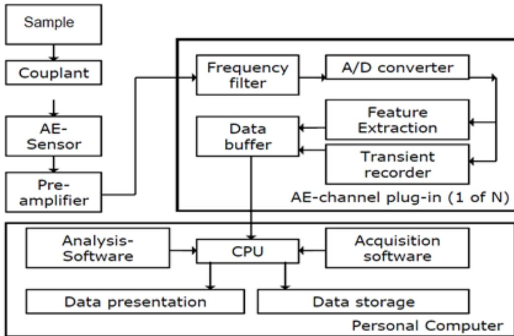
**Figure 4.4: Block diagram of AE instrumentation [168].**
