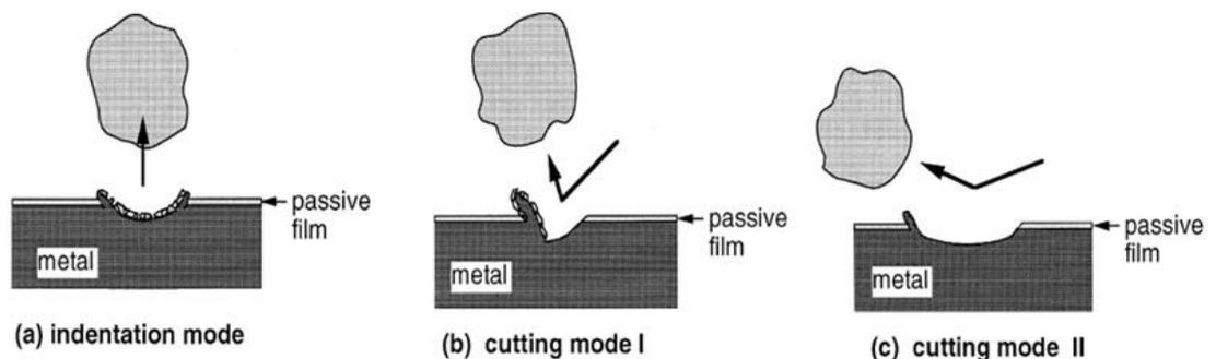
**Figure 3.17: Illustration of erosion-corrosion process [130].**
