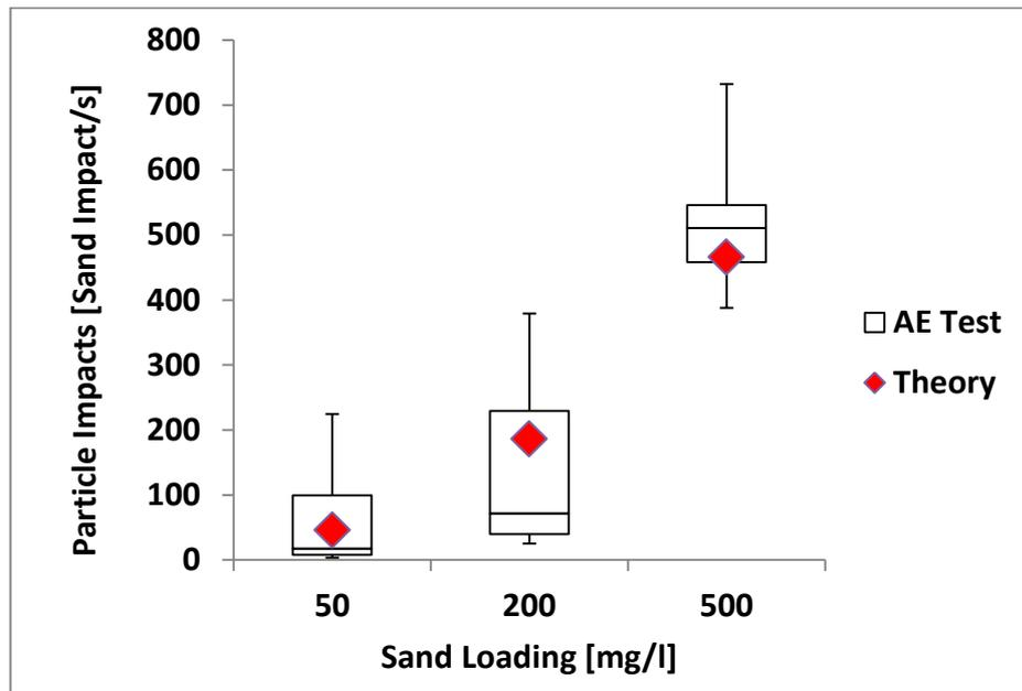
Figure 7.13: Comparison of measured particle impacts with theory for 7 m/s flow velocity.
