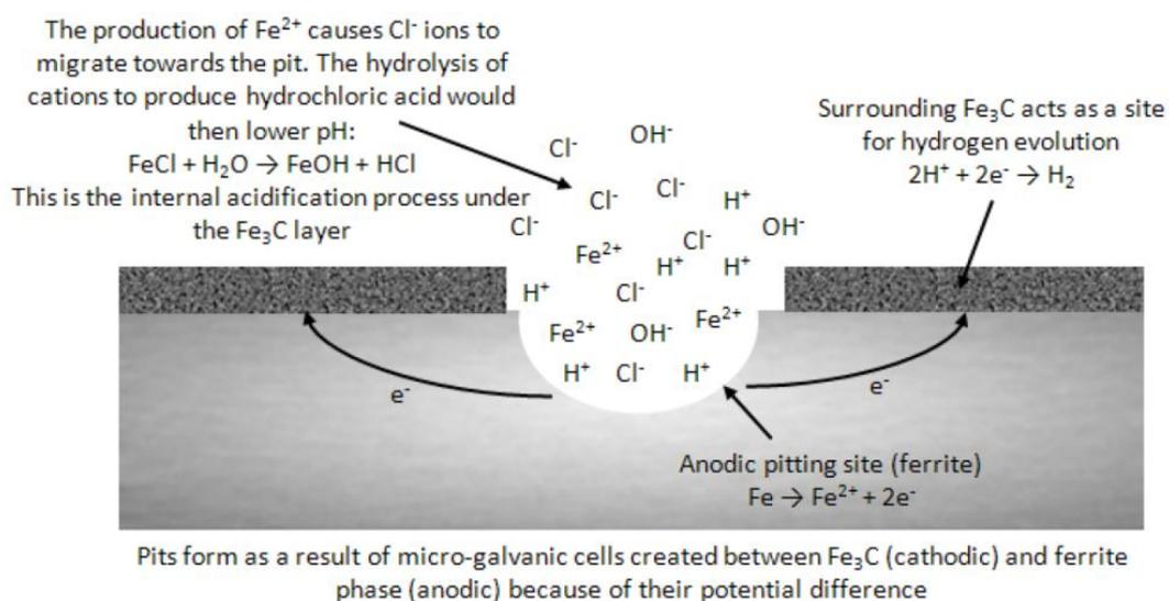
**Figure 9.18: An illustration of anodic pit with a large cathodic  $\text{Fe}_3\text{C}$  surface which enhances the material dissolution [207].**
