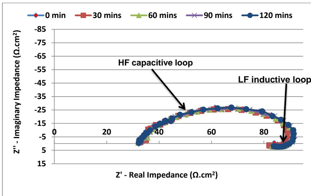
Figure 9.1: Nyquist plot at different exposure times for 7 m/s with process brine without sand, 50°C and CO<sub>2</sub> saturated at 1 bar.
