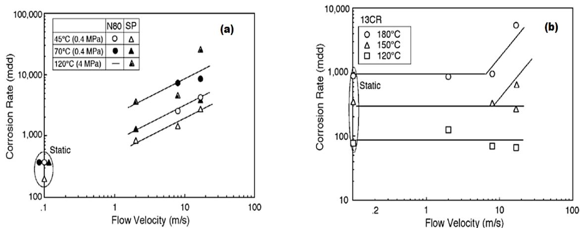
**Figure 3.11: Effect of flow velocity and temperature on corrosion rate for (a) carbon steel and low alloy steel and (b) stainless steel (13%Cr) [77].**
