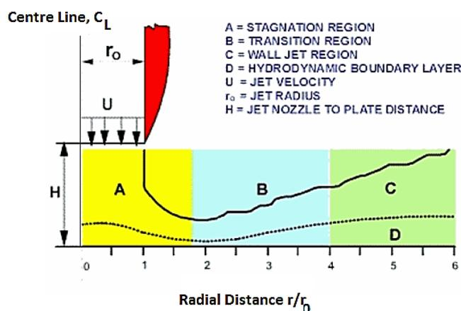
**Figure 3.19: Hydrodynamic features of a jet impingement on a flat plate [78]**
