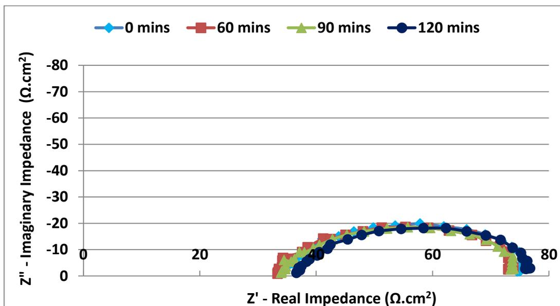
**Figure 9.8: Nyquist plot at different exposure times for 15 m/s with process brine, 500 mg/L sand loading, 50°C and CO<sub>2</sub> saturated at 1 bar.**
