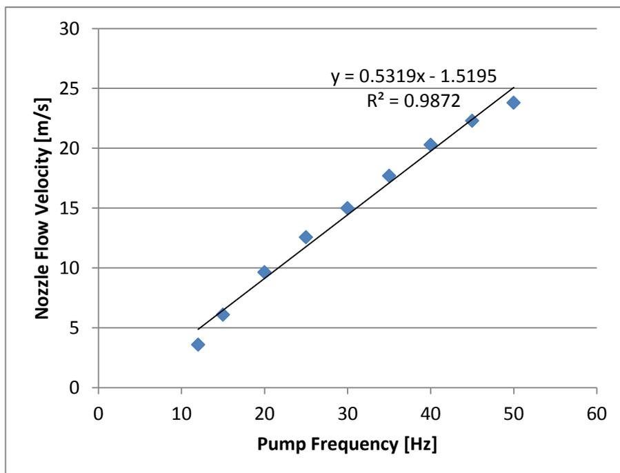
**Figure 5.6: Plot of nozzle flow velocity variation with pump frequency during the flow velocity calibration.**
