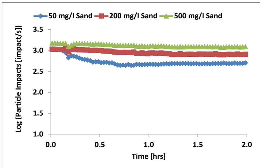
Figure 7.10: Variation of particle impacts with time for different sand concentrations for 15 m/s all at 90° impingement angle and 50°C temperature in tap-water saturated with N<sub>2</sub> (pH ≈ 7.0).
