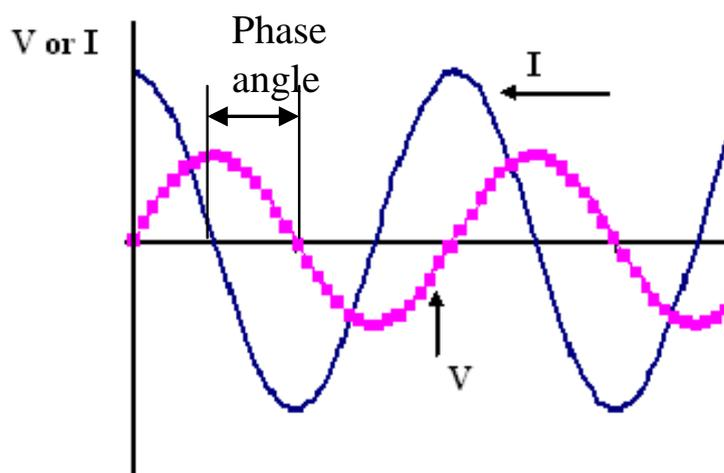
**Figure 2.8: AC voltage and current response [43].**
