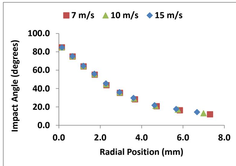
Figure 7.21: Predicted variation of particle impact angle with radial distance.
