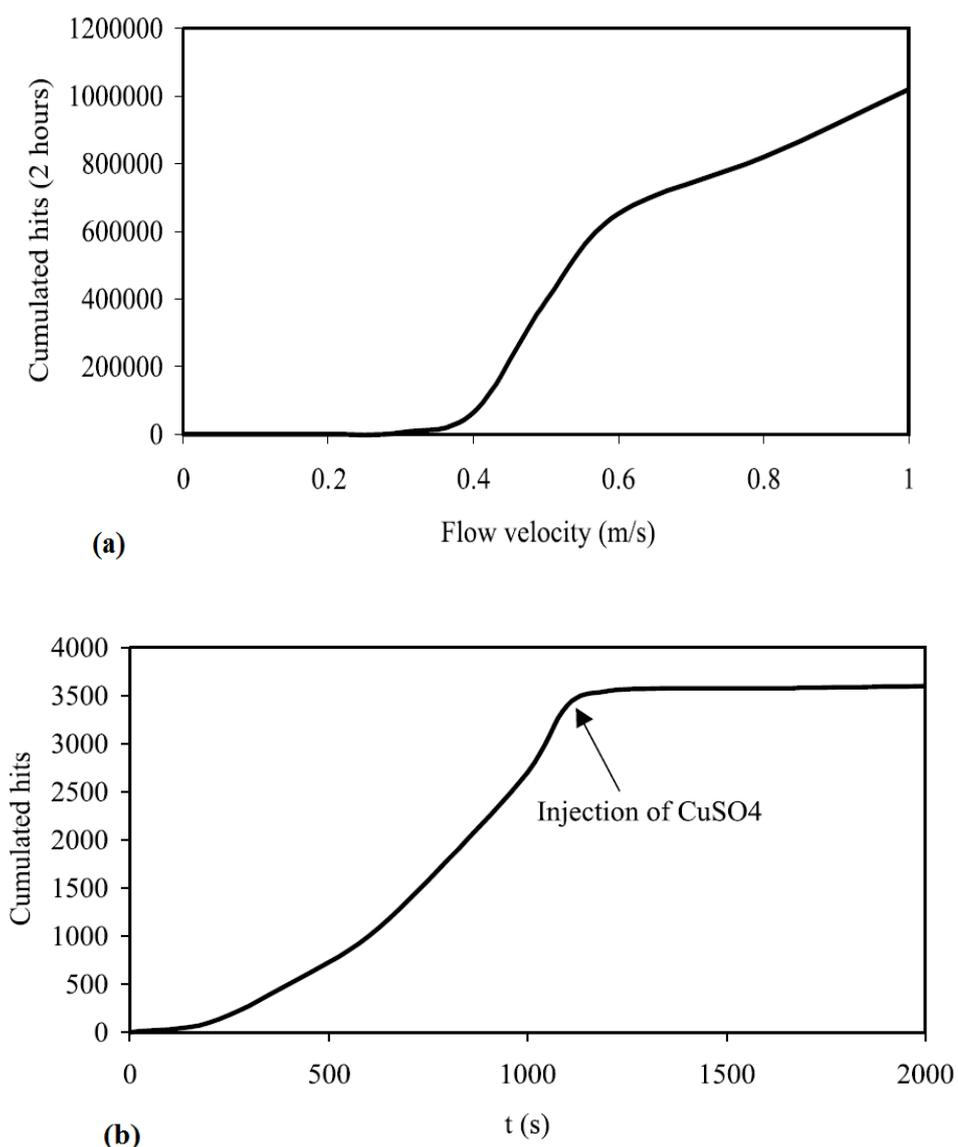
**Figure 4.11: Illustration of (a) AE activity variation with flow velocity in erosion-corrosion test and (b) the effect of an inhibitor on the AE activity at 2 m/s [172].**
