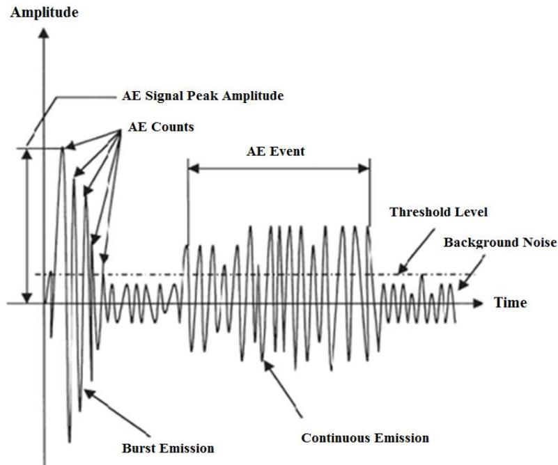
**Figure 4.2: Illustration of the features of an AE signal [162].**
