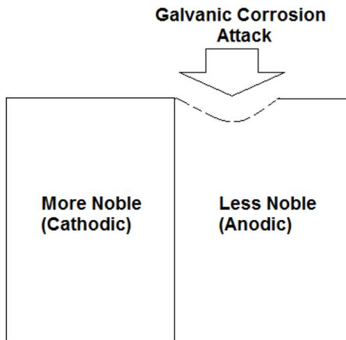
**Figure 2.13: Illustration of galvanic corrosion.**
