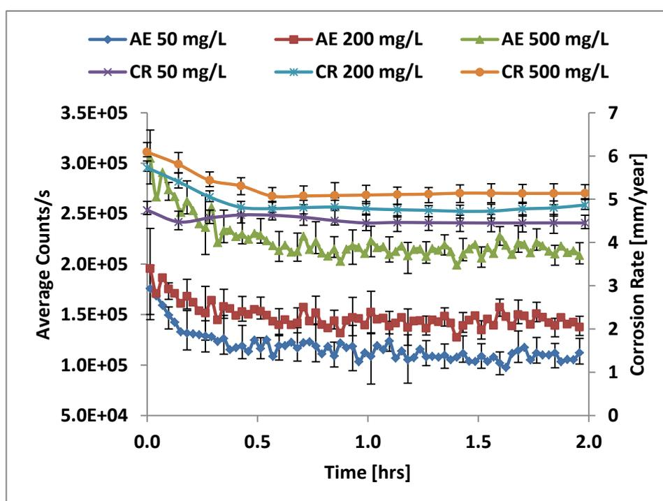
Figure 8.10: Results for erosion-corrosion test showing corrosion rate with AE count rate for 10 m/s in  $\text{CO}_2$  saturated brine (pH 5.5) at  $50^\circ\text{C}$ . Corrosion rates were obtained from LPR measurement using Stern-Geary coefficient of 26 mV.
