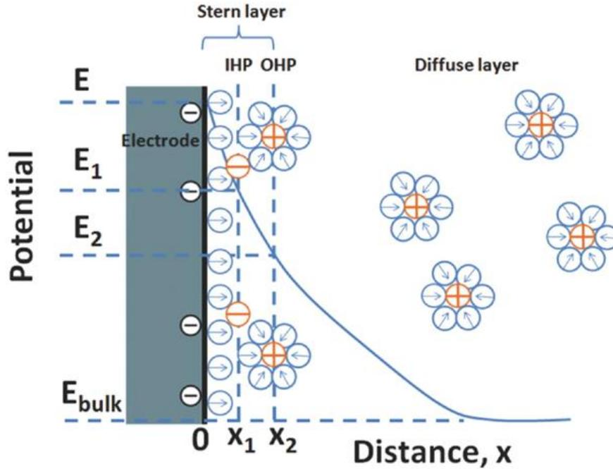
**Figure 2.3: Stern-Grahame model for electrical double layer [56].**
