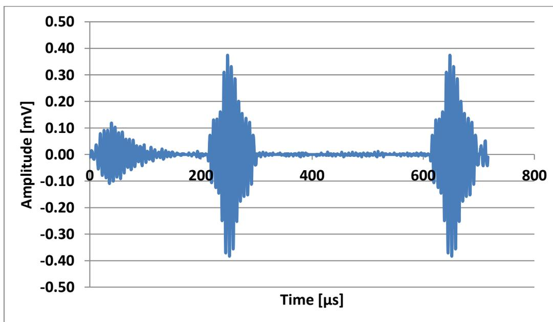
**Figure 9.5: Detected AE signal waveform. Test conditions: process brine, 7 m/s flow velocity with 200 mg/L sand loading, 50°C and CO<sub>2</sub> saturated at 1 bar.**
