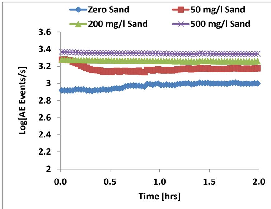
Figure 7.6: AE event count rate for baseline and different sand concentrations for 15 m/s at 90° impingement angle and 50°C temperature in tap-water saturated with N<sub>2</sub> (pH ≈ 7.0).
