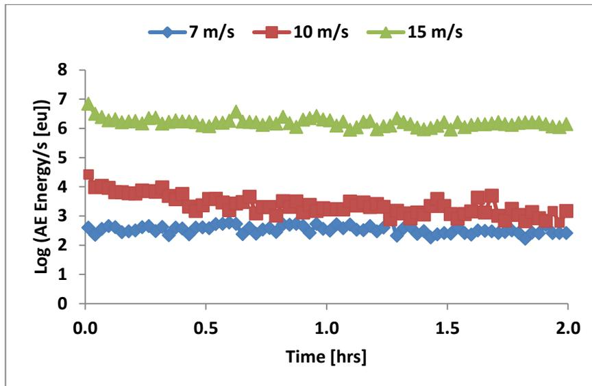
Figure 6.5: Variation of average AE energy with time for different flow velocities and zero sand loading at 90° impingement angle and 50°C temperature in tap-water saturated with N<sub>2</sub> (pH ≈ 7.0).
