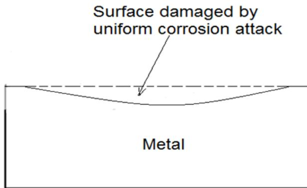
**Figure 2.11: Illustration of general corrosion.**
