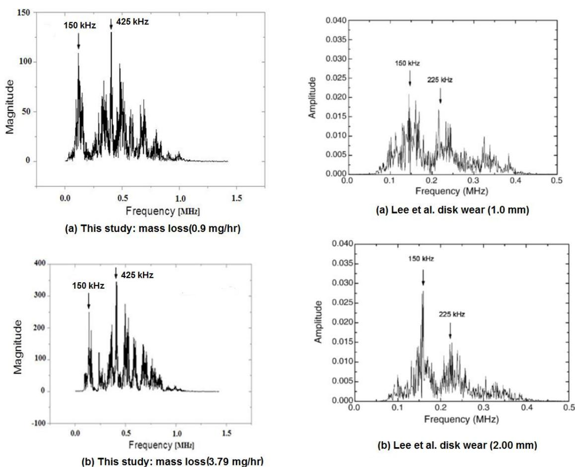
**Figure 10.2: Comparison of the frequency spectra of waveform in this study (LHS) with frequency spectra from Lee *et al.* [241] (RHS) disk wear study.**
