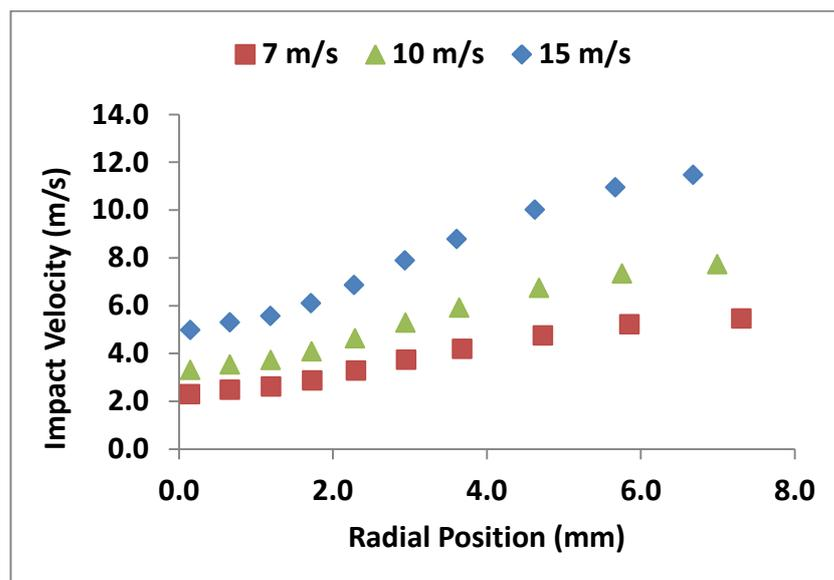
Figure 7.22: Predicted variation of particle impact velocity with radial distance.
