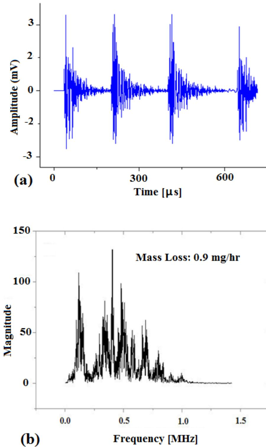
Figure 6.27: (a) Measured AE waveform (time-domain) and (b) frequency-domain for 10 m/s flow velocity, 200 mg/L sand loading at 90° impingement angle and 50°C temperature in tap-water saturated with N<sub>2</sub> (pH  $\approx$  7.0).
