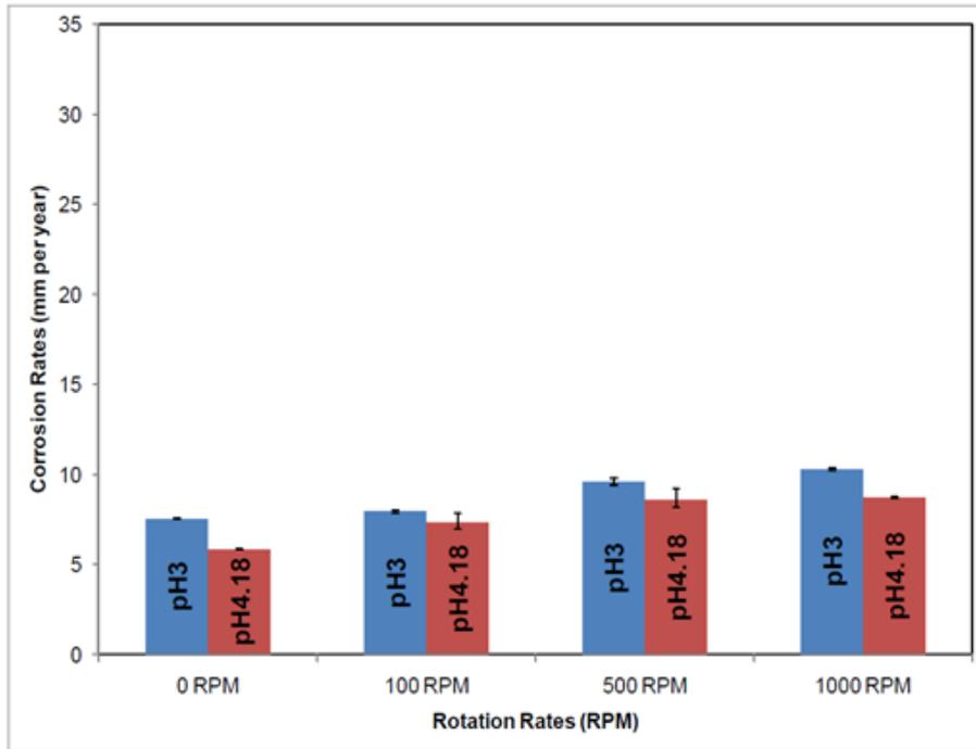
Figure 3.8: Variation of corrosion rate with flow velocity for pH 3 and 4.14 at  $p\text{CO}_2 = 10 \text{ bar}$  [70].
