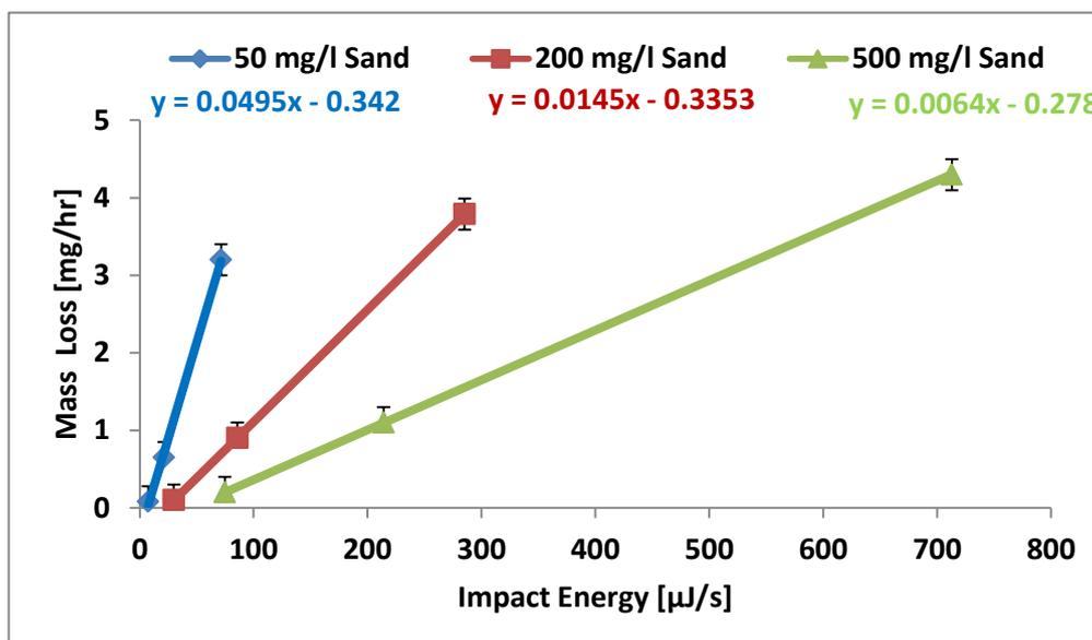
**Figure 7.26: Relationship between mass loss and impact energy per second. Tests performed at 90° impingement angle and 50°C temperature with tap-water saturated with N<sub>2</sub> (pH ≈ 7.0).**
