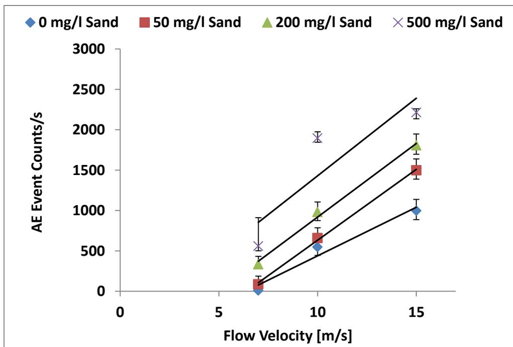
Figure 7.7: Summary of the results for AE event count rate for baseline and different sand concentrations and flow velocities at 90° impingement angle and 50°C temperature in tap-water saturated with N<sub>2</sub> (pH ≈ 7.0).
