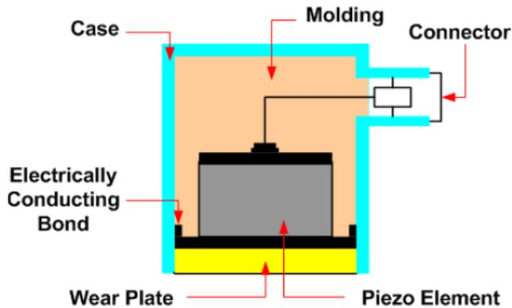
**Figure 5.11: Illustration of the components of piezoelectric sensor [168].**
