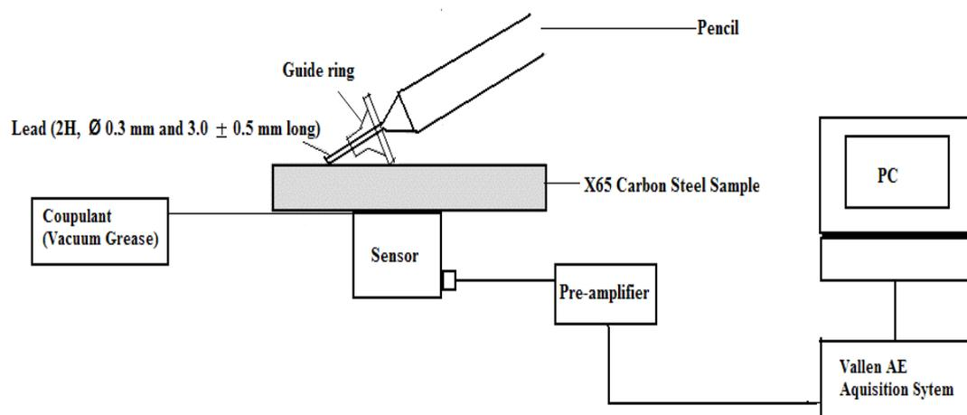
**Figure 5.12: Schematic illustration of AE sensor calibration set-up.**
