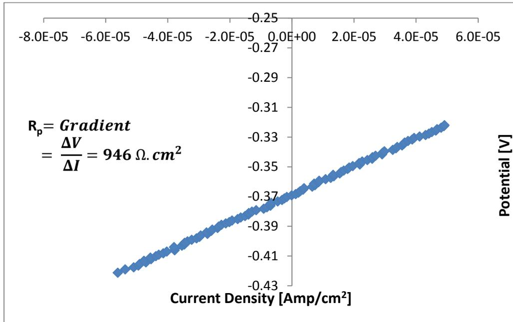
Figure 6.13: LPR data of X65 carbon steel under impingement at 90° impact angle, 50°C and 10 m/s flow velocity with tap-water saturated with N<sub>2</sub> (pH≈7.0).
