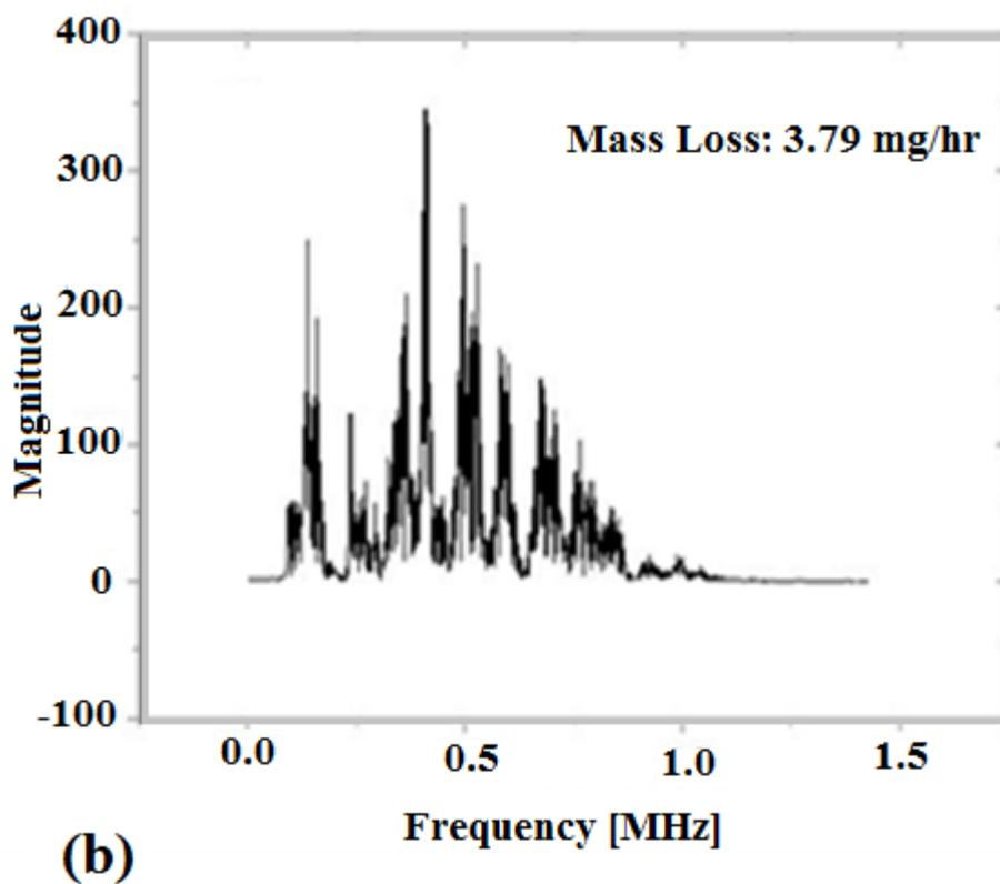
Figure 6.28: (a) Measured AE waveform (time-domain) and (b) frequency-domain for 15 m/s flow velocity, 200 mg/L sand loading at  $90^\circ$  impingement angle and  $50^\circ\text{C}$  temperature in tap-water saturated with  $\text{N}_2$  ( $\text{pH} \approx 7.0$ ).
