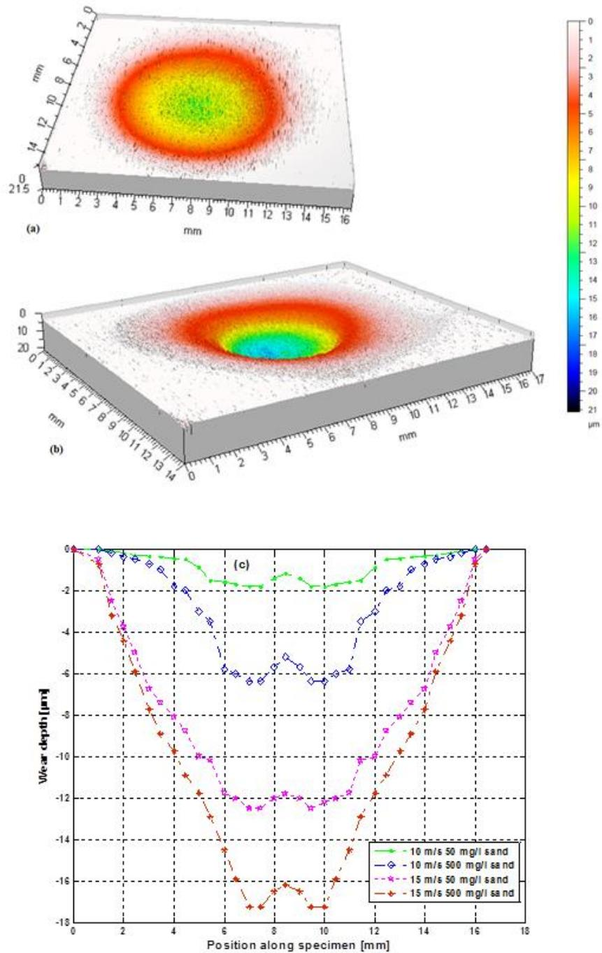
Figure 6.20: 3D profilometry of the erosion scars on the X65 carbon steel for 15 m/s flow velocity (a) 50 mg/L (b) 500 mg/L sand concentrations and (c) the profile of the wear scar depth across the specimen's surface for 2 hours test duration in tap-water saturated with  $N_2$  ( $pH \approx 7.0$ ).
