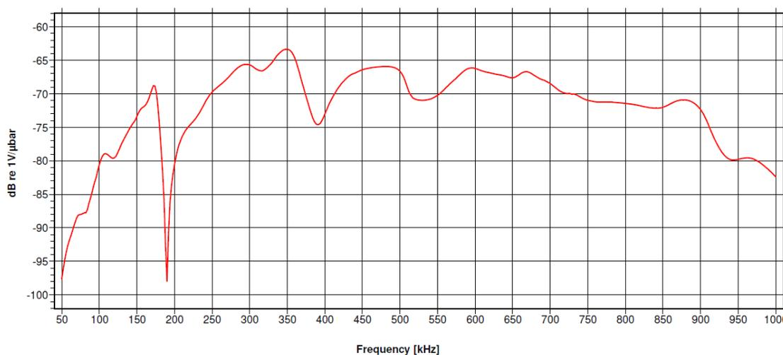
**Figure 5.10: Published AE sensor (VS900-M) calibration certificate [194].**
