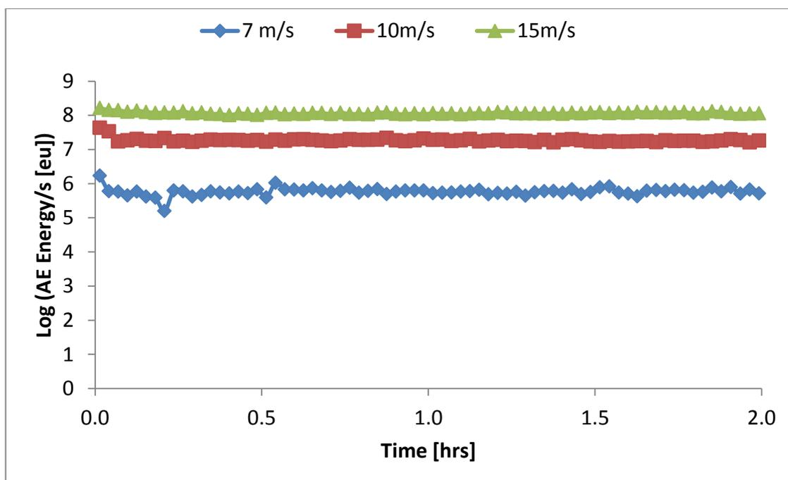
Figure 6.8: Variation of average AE energy with time for different flow velocities and fixed sand loading of 500 mg/L all at 90° impingement angle and 50°C temperature in tap-water saturated with N<sub>2</sub> (pH ≈ 7.0).
