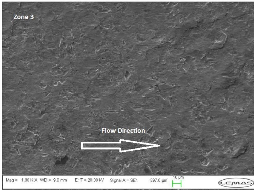
**Figure 6.19: SEM image showing the degradation mechanism in zone 3, the wall jet region for 15 m/s flow velocity, 500 mg/L sand and temperature of 50°C in tap-water saturated with N<sub>2</sub> (pH≈7.0).**
