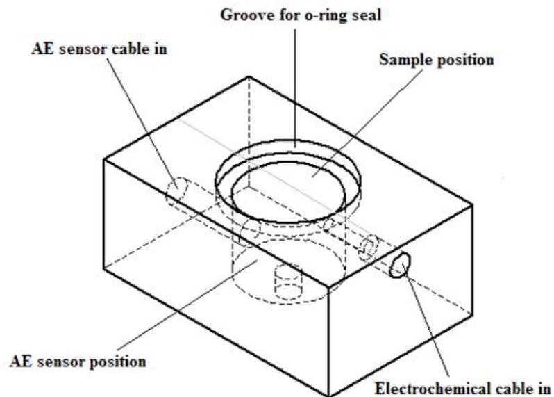
**Figure 5.3: Isometric view of AE test cell/specimen holder.**
