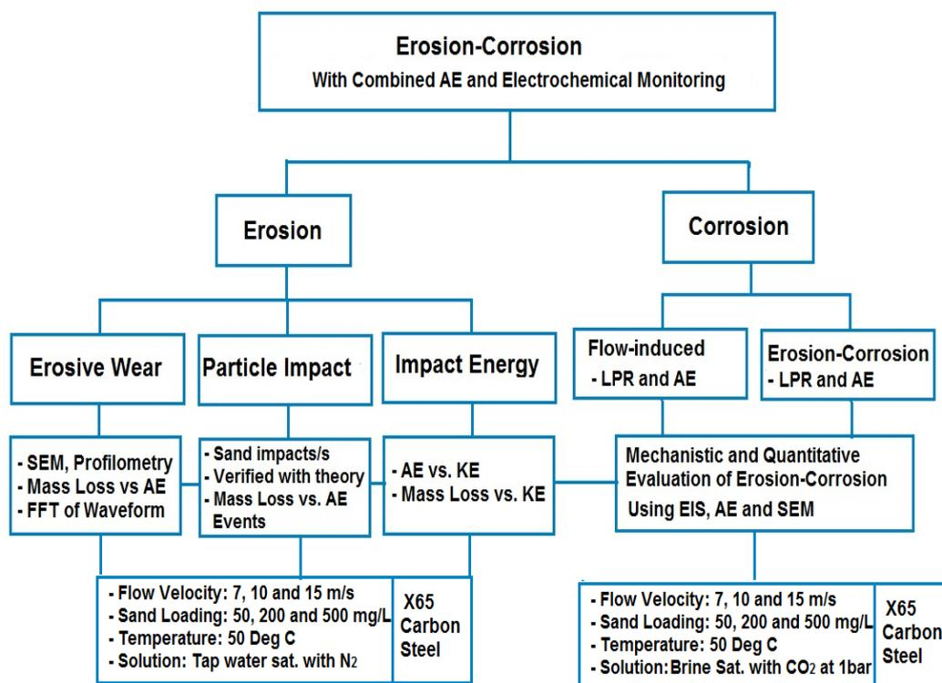
**Figure 10.1: An overview of study and the approaches applied to gain proper understanding of the interaction between erosion and corrosion**
