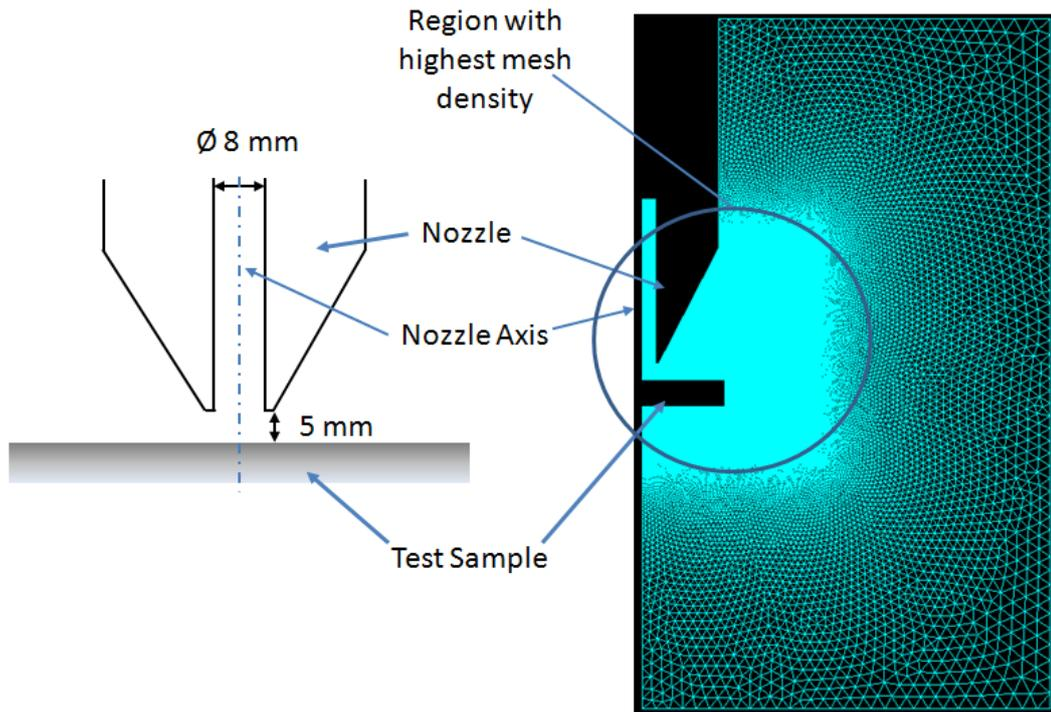
**Figure 7.17: Illustration of actual geometry (left) and flow domain simplified to 2D using Gambit (right) (domain size is 120 mm x 220 mm and mesh consists of approximately 130,000 elements).**
