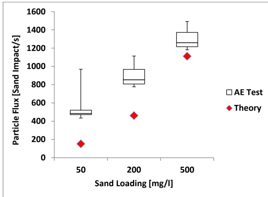
Figure 7.15: Comparison of measured particle impacts with theory for 15 m/s flow velocity.
