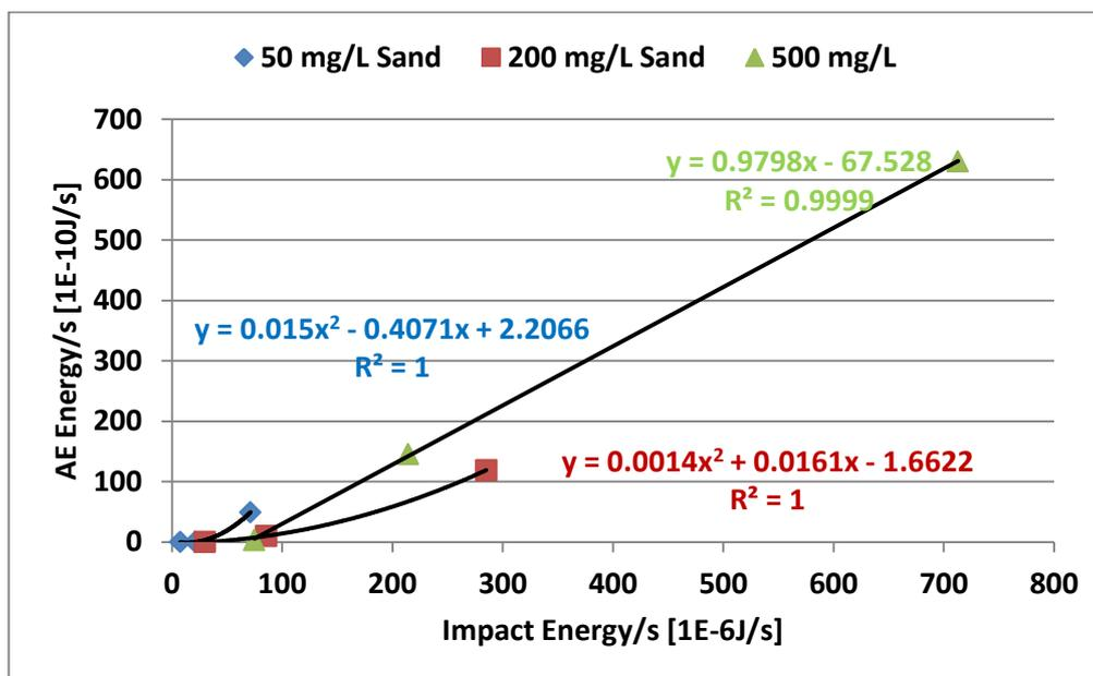
Figure 7.24: Relationship between measured AE energy and impact energy predicted from theory for 50, 200, 500 mg/L sand loading multiple impacts.
