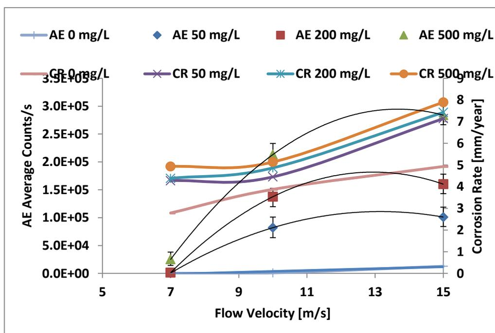
Figure 8.15: Summary of results for corrosion rate and AE count rate. Tests with brine saturated with CO<sub>2</sub> at 1 bar.
