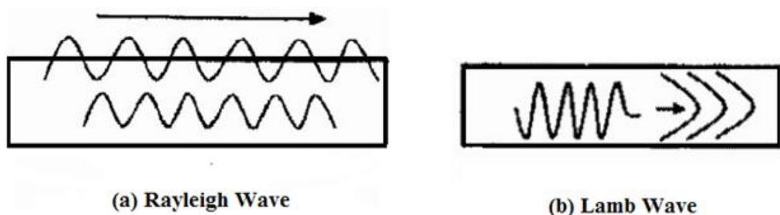
**Figure 4.1: Schematic illustration of (a) Rayleigh wave and (b) Lamb wave propagation in a structure [166].**
