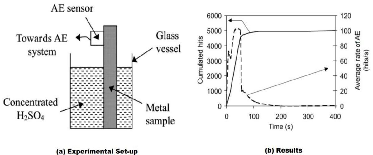
**Figure 4.7: AE static corrosion test (a) experimental set-up (b) results [172].**
