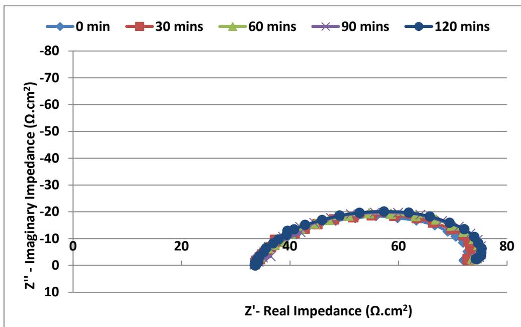
**Figure 9.3: Nyquist plot at different exposure times for 15 m/s with process brine without sand, 50°C and CO<sub>2</sub> saturated at 1 bar.**
