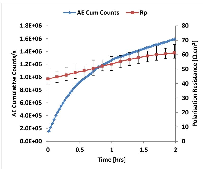
Figure 8.6: Polarisation resistance variation with AE cumulative counts for 15 m/s flow in CO<sub>2</sub> saturated brine (pH 5.5) at 50°C.
