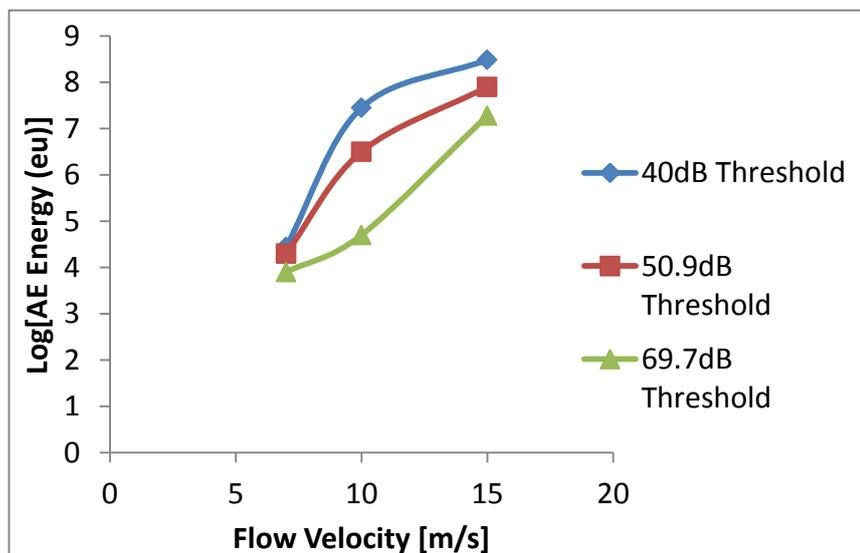
**Figure 5.18: Illustration of the optimized threshold setting used in all test at 90° impingement angle, 200 mg/L sand loading and 50°C temperature, tap-water saturated with N<sub>2</sub> (pH ≈ 7.0).**
