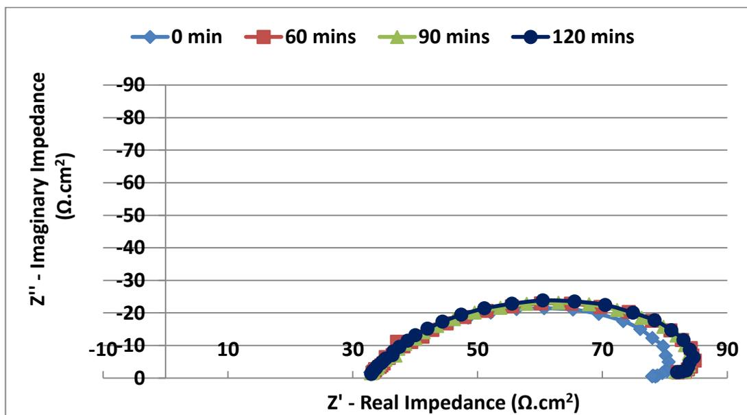
Figure 9.7: Nyquist plot at different exposure times for 10 m/s with process brine, 500 mg/L sand loading, 50°C and CO<sub>2</sub> saturated at 1 bar.
