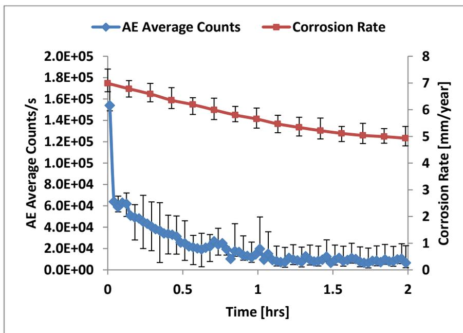
Figure 8.5: Flow-induced corrosion rate variation with AE count rate for 15 m/s flow in CO<sub>2</sub> saturated brine (pH 5.5) at 50°C. Corrosion rates were obtained from LPR measurement using Stern-Geary Coefficient of 26 mV.
