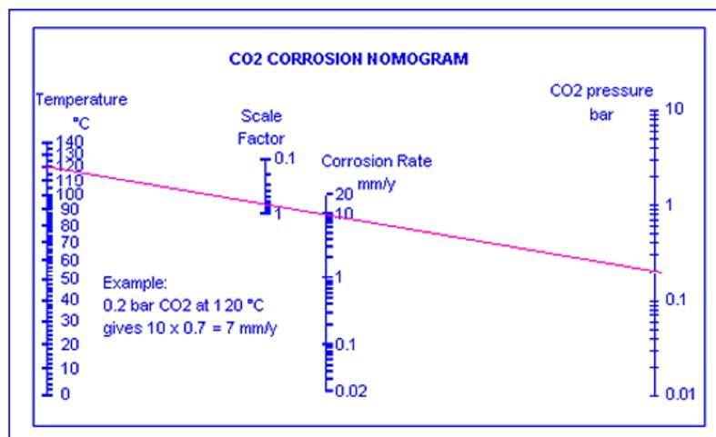
Figure 3.1: CO<sub>2</sub> corrosion nomogram [43].
