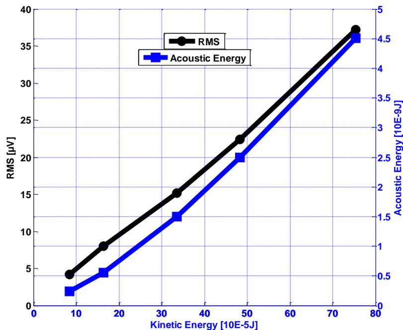
Figure 6.3: Relationship between AE energy and RMS due to single glass bead impact and its kinetic energy at 90° impingement angle and 50°C temperature with tap-water saturated with N<sub>2</sub> (pH ≈ 7.0).
