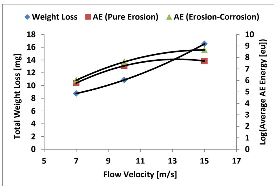
Figure 8.20: Results of the total weight loss with measured average AE energy in energy units ([eu],  $1\text{eu}=1\text{E}-18\text{J}$ ) in the presence and absence of corrosion for 500 mg/L sand concentration.
