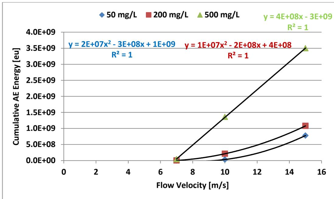
**Figure 6.23: Relationship between cumulative AE energy and flow velocity for all the sand loadings investigated with tap-water saturated with N<sub>2</sub>.**
