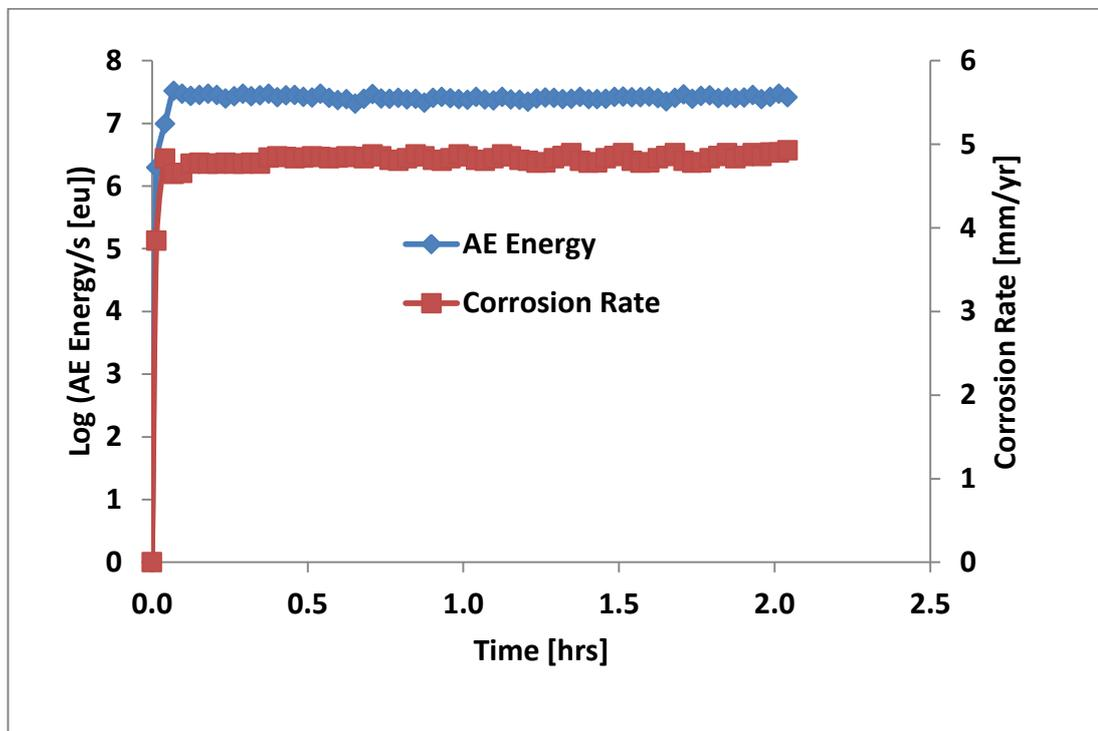
Figure 6.10: Correlation of AE energy with corrosion rate at  $90^\circ$  impingement angle,  $50^\circ\text{C}$ ,  $10 \text{ m/s}$  flow velocity and  $200 \text{ mg/L}$  sand loading in brine saturated with  $\text{CO}_2$  ( $\text{pH}=5.5$ ).
