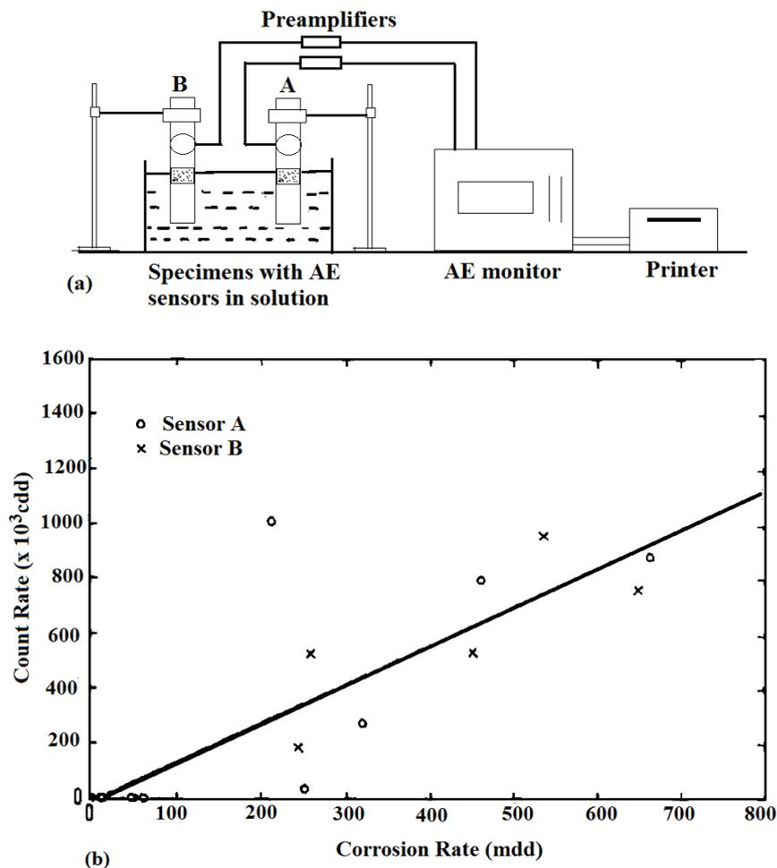
Figure 4.6: (a) Experimental set-up and (b) AE count rate vs. corrosion rate [170].
