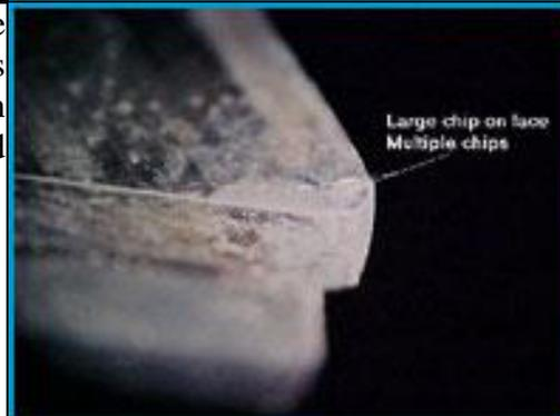
**Notching Wear** is caused by the formation of an individual groove at the same time on the face and flank of the tool whose size corresponds to the depth of cut. Notching will lead to a substandard finish on the workpiece and may lead to fracture of the tool.
