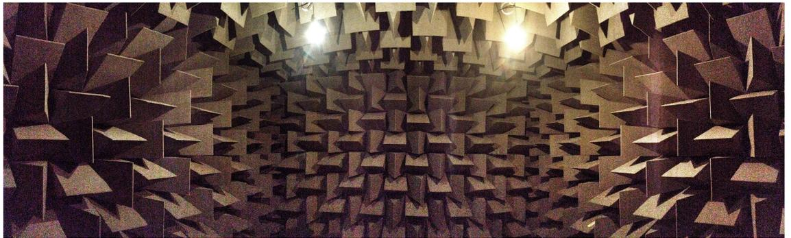
Figure 4.2: 6-sided anechoic chamber.
