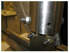
12. Position rig such that Femur head is directly under the centre of the upper loading plate.
