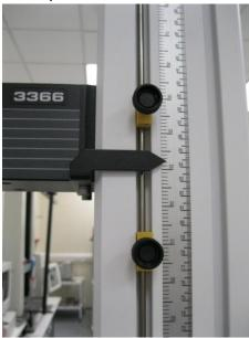
15. Attach safety screen (with cut out for mechanical stoppers on right hand side)
