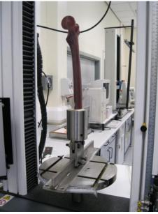
11. Position 10mm bolt through 0degree holes on loading rig and secure using a 10mm nut
