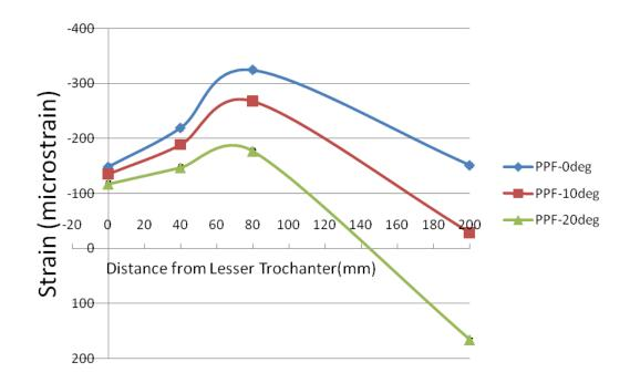
Figure 39 Strain along the medial length of the Sawbone Femur on the medial side, for the plate specimens at 0°, 10° and 20° loading angle.
