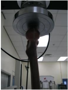
13. Secure loading rig to base plate using machining blocks with T nuts placed inside base plate groves. N.B for best attachment, bolts should be sited as close to rig end of machining blocks as possible. The back of the machining blocks need to be at the same level or higher than at the rig end.
