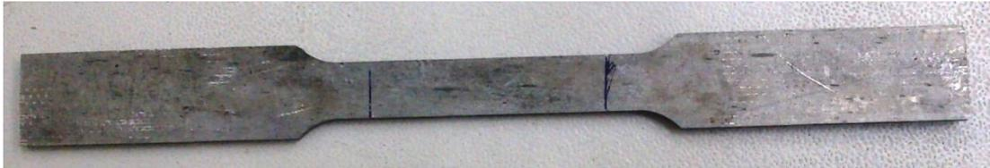
Figure 3.7 – Tensile specimen prepared according to ASTM standard E8/E8M – 09[148]
