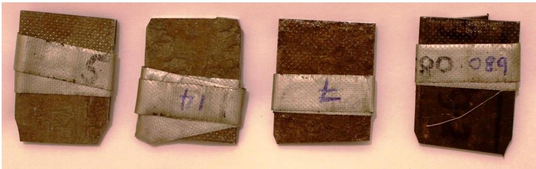
Figure 3.1 – Images of tensile test bar grip heads received from Tata Steel for characterisation
