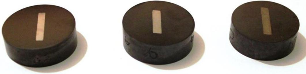
Figure 3.8 – Sample mounted in bakelite for optical microscopy, SEM and TEM carbon extraction replicas
