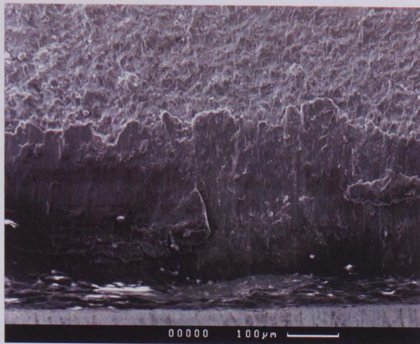
Figure 4.140: A region of rubbing corresponding to specimen number 17; an aluminium alloy 2024 T351 specimen in contact with a BS S98 steel bridge subjected to a normal pressure of 40 MPa and an axial stress amplitude of 100 MPa.
