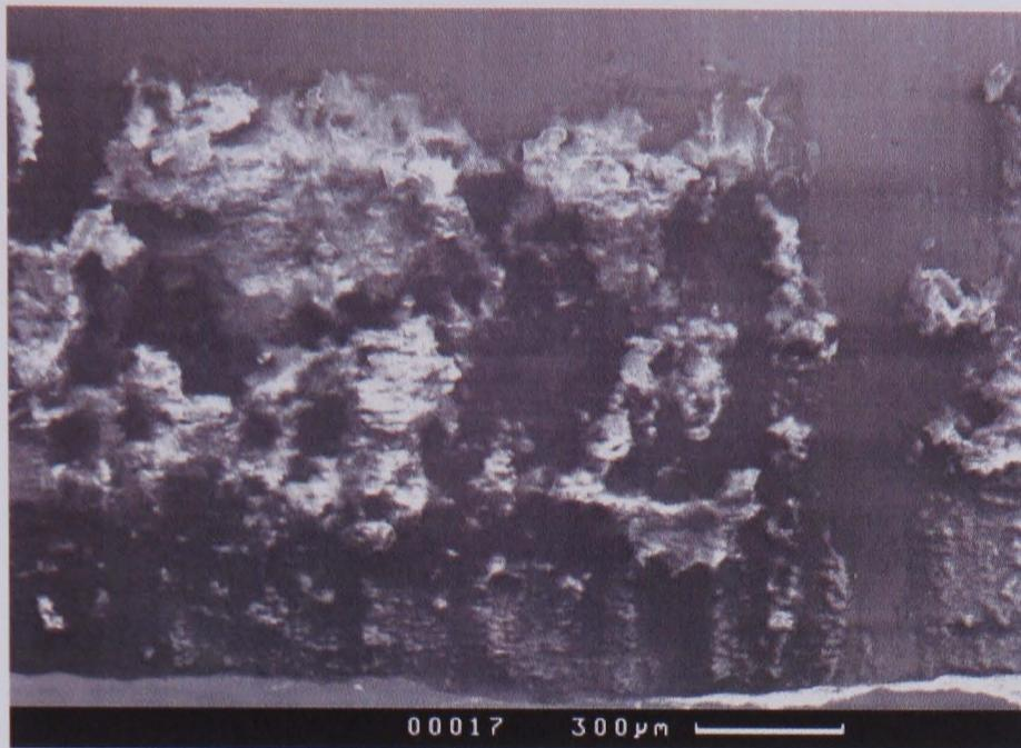
Figure 4.125: Evidence of adhesion relating to specimen number 105; an aluminium alloy 2024 T351 specimen in contact with an aluminium alloy 2024 T351 bridge subjected to a normal pressure of 20 MPa and an axial stress amplitude of 70 MPa.
