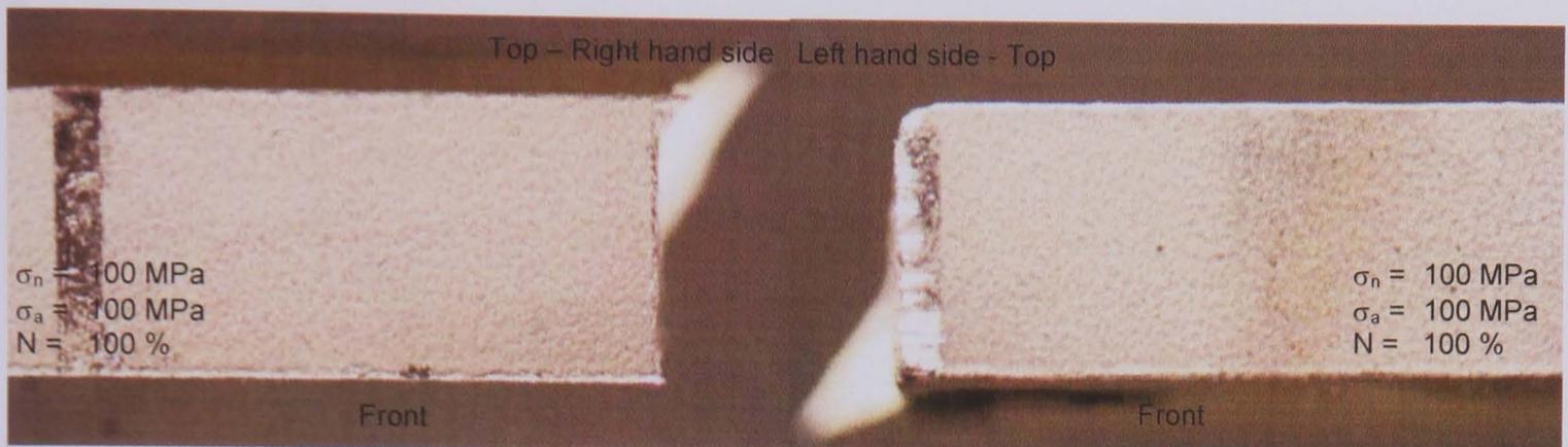
Figure 4.116: Crack initiation at the leading edge of the contact area on the top surface of a peened specimen.
