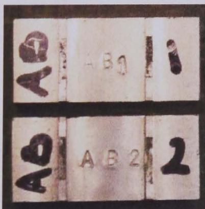
Figure 4.30: The wear scars from an unpeened bridge with a pad span of 16.5 mm having been in contact with a peened specimen subjected to a normal pressure of 100 MPa and an axial stress amplitude of 100 MPa for 25% of the total expected life of that specimen.
