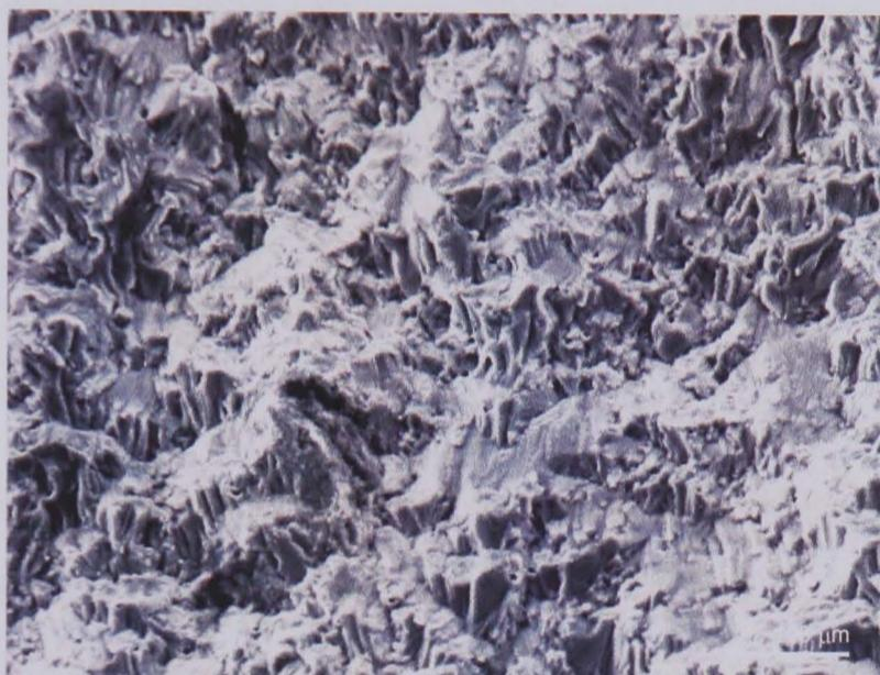
Figure 4.144: (A): A fractograph demonstrating a region of stage I crack propagation relating to specimen number 13; an aluminium alloy 2024 T351 specimen in contact with a BS S98 steel bridge subjected to a normal pressure of 80 MPa and an axial stress amplitude of 100 MPa.
