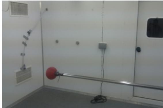
Figure 4.6: Scenario 1: Isotropic release from inside red diffuser ball in centre of room
