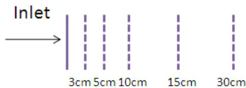
Figure 4.15: Measurement surfaces away from the grille
