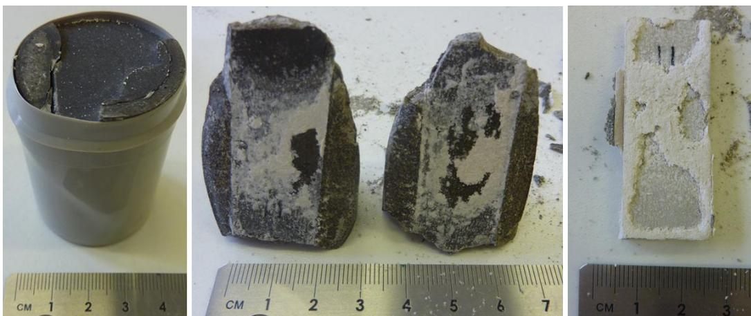
**(c) 360 days**
