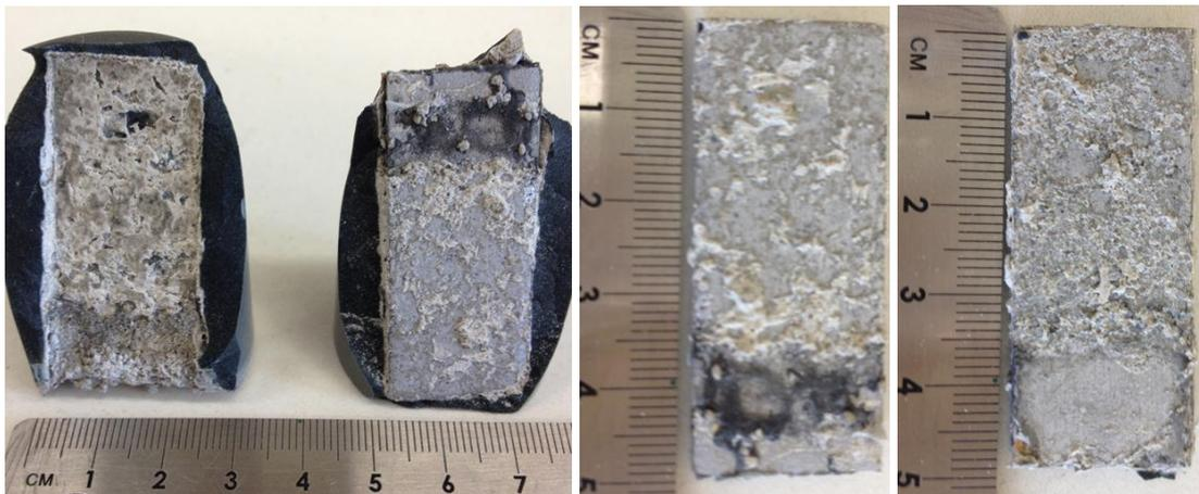
**Figure 6.8 Corrosion of aluminium in BFS/PC system: (a) 90 days, (b) 180 days and (c) 360 days**
