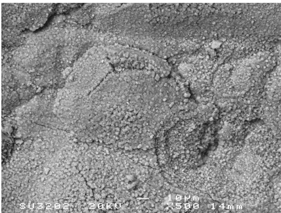
Figure A. 24 SEM BEI of the surface of aluminium encapsulated in CAP 1 for 360 days (x500)
