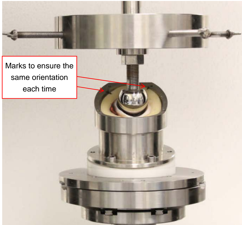
Figure 8.1 Experimental setups. The acetabulum was held in a cup holder which can move horizontally. The load was applied vertically to the head.
