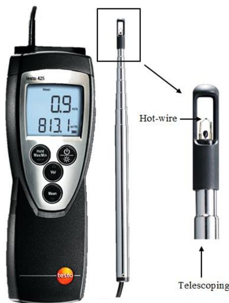
**Figure 4.37** Testo 425 hot-wire anemometer.
