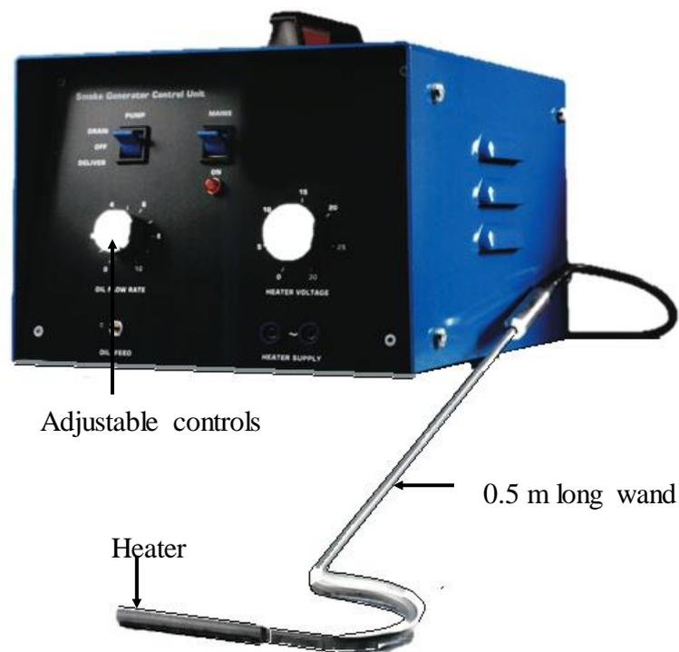
**Figure 4.44** AFA 10 Smoke generator unit.
