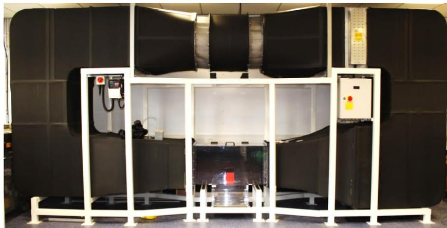
(a) Actual subsonic closed loop wind tunnel system
