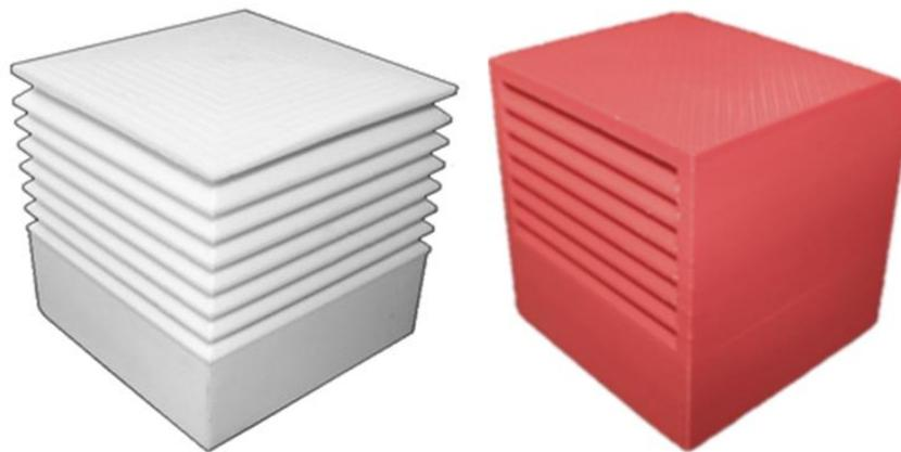
**Figure 6.1** 1:10 scale benchmark wind tower models (a) four-sided (b) one-sided.
