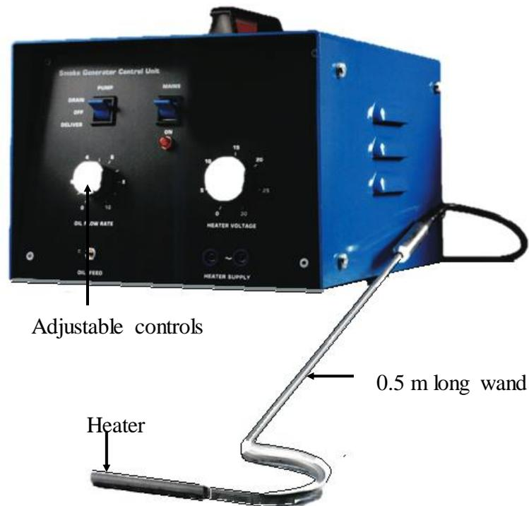
**Figure 4.44** AFA 10 Smoke generator unit.
