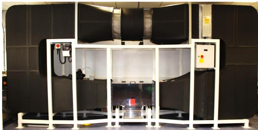
(a) Actual subsonic closed loop wind tunnel system
