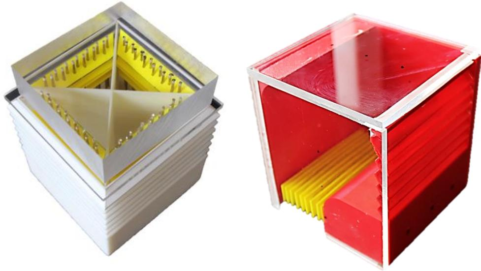
**Figure 6.20** 1:10 prototype model of the four and one-sided wind tower design incorporating heat transfer devices and extended surfaces.
