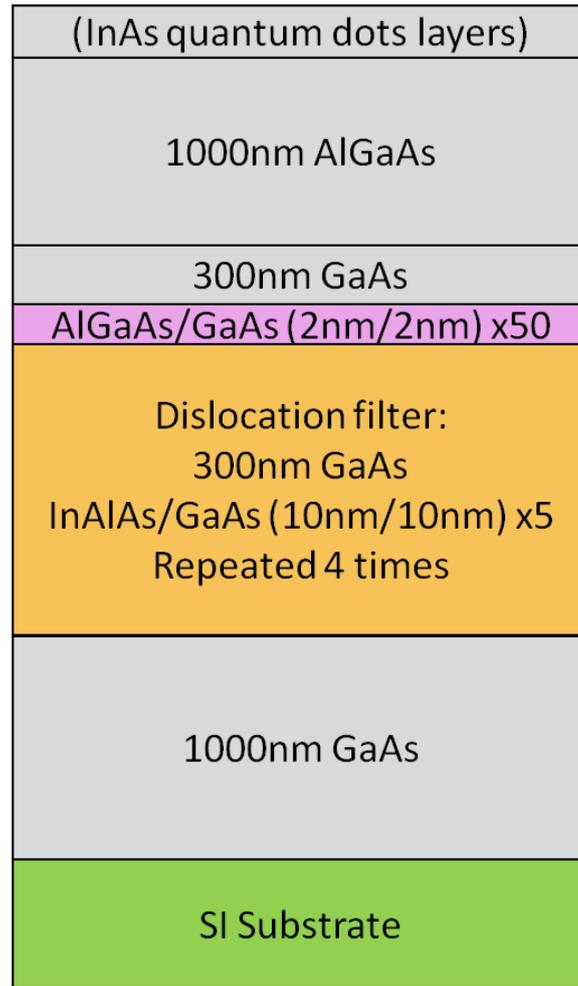
Figure 3.1: Schematics of the layer structure of the sample.
