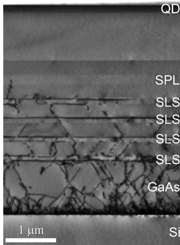
Figure 2.4: TEM image of the layer structure. The clearer layer on the bottom of the image is Si, strain formation can be seen on the upper III-V layers.
