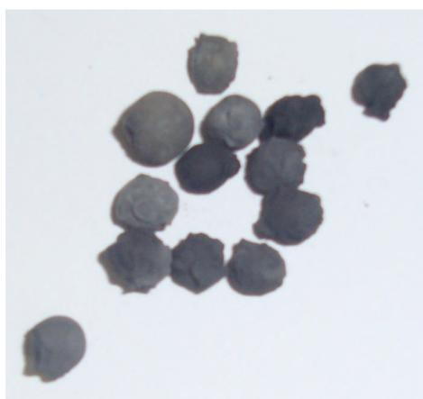
Figure 5-16 Micrograph of the Reacted Ni(10) Al<sub>2</sub>O<sub>3</sub>
