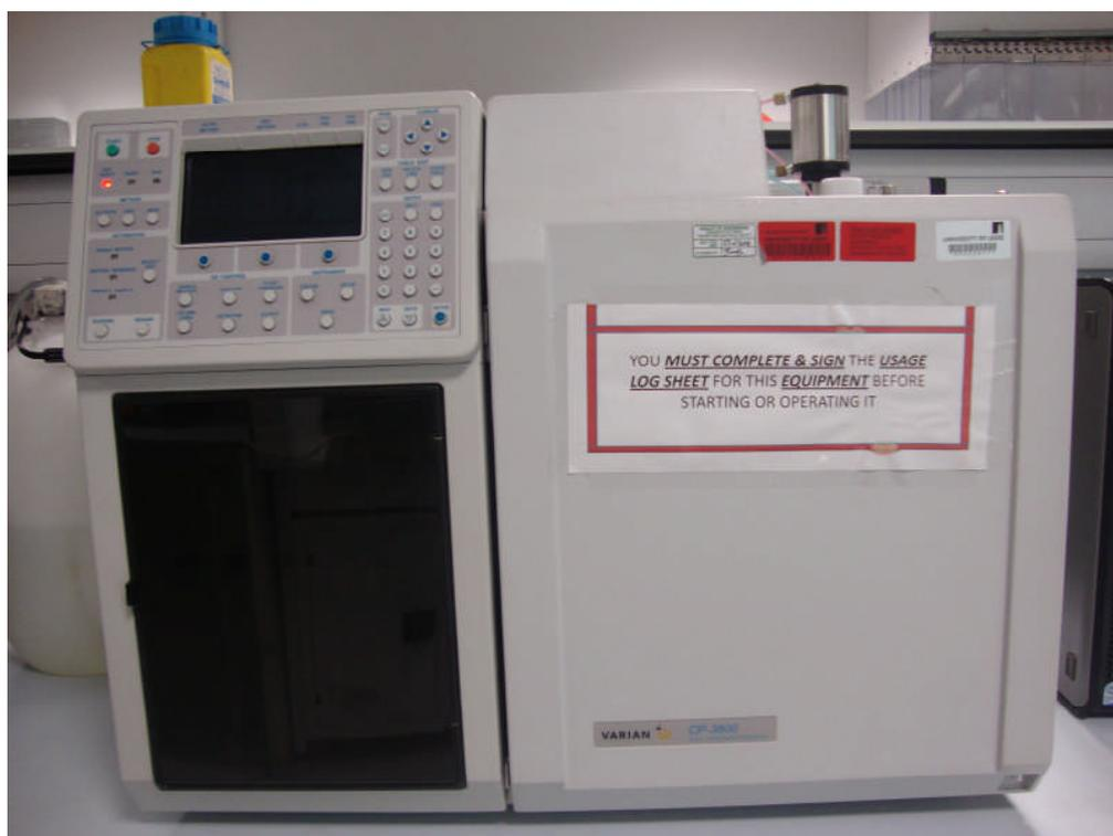
Figure 3-6 Photograph of a Varian GC with TCD and FID.
