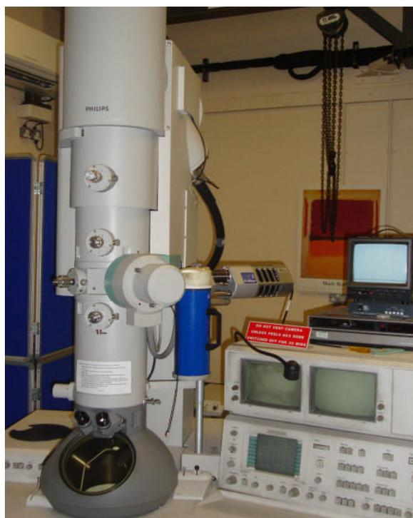
Figure 3-23 Photograph of the Philips CM200 TEM-EDXS equipment
