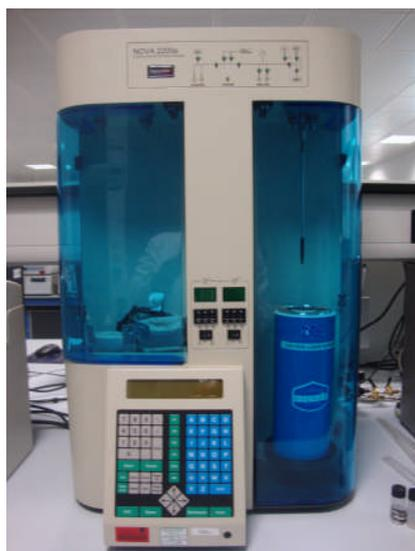
Figure 3-16 Photograph of the Quantachrome BET equipment
