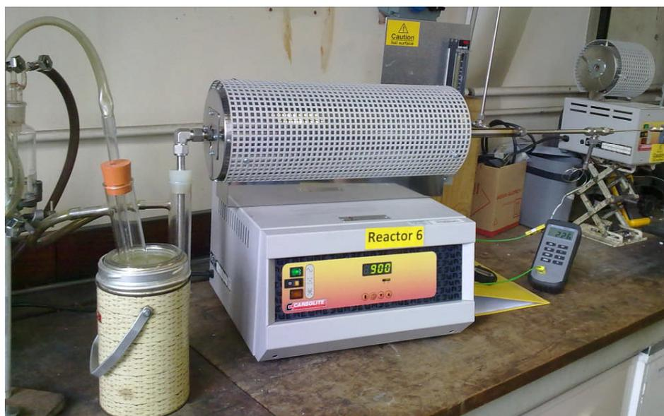
Figure 3-2 Photograph of the horizontal fixed bed reactor
