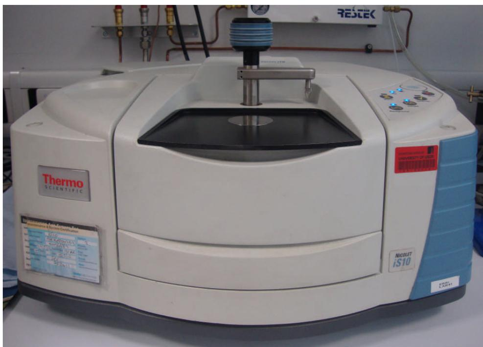
Figure 3-11 Photograph of the ThermoScientific Nicolet iS10 spectrometer
