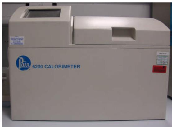
Figure 3-15 Photograph of the Parr Isooperibol calorimeter
