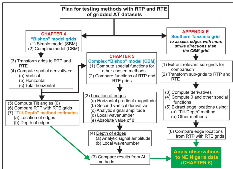
**Figure 4.1:** Work-flow adopted for evaluating estimates obtained from “Bishop” model (BM) and real Southern Tanzania  $\Delta T$  datasets, using the “Tilt-Depth” and other methods.
