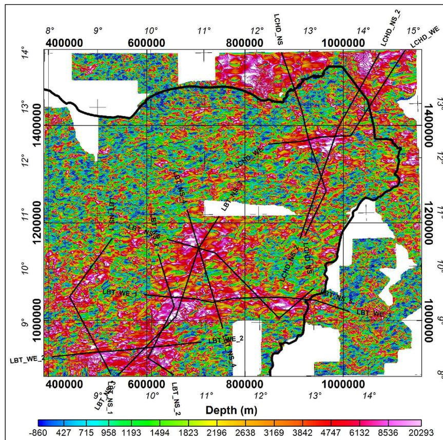
Figure H.13: Local wavenumber (LW) method depth estimates shown in figure 6.16.
