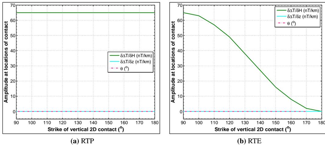
**Figure 3.19:** Effect of strike direction on amplitudes of Cartesian derivatives and  $\theta$  of  $\Delta T$  at locations of vertical contacts, at RTP or RTE. Cartesian derivatives shown are: total horizontal derivatives (Green line); vertical derivatives (Cyan line); and  $\theta$  (Pink dashed line). Note that  $\theta$  does not exist when other derivatives are essentially zero.
