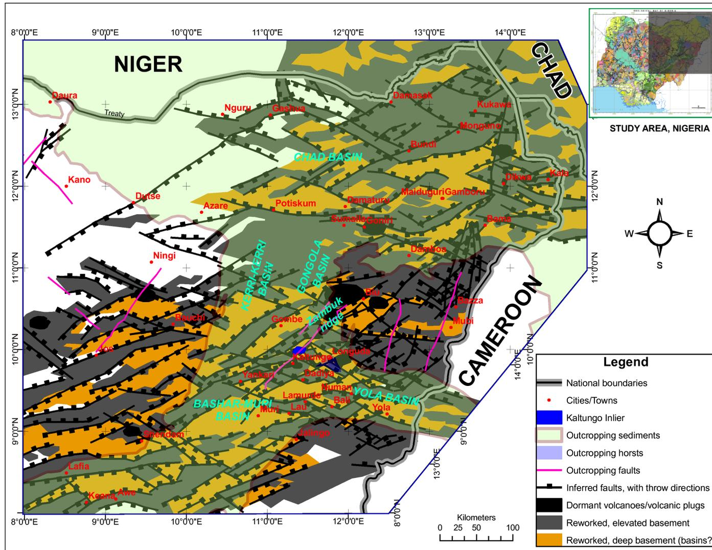
Figure H.10: Gross magnetic basement structure map of NE Nigeria (Figure 6.12).
