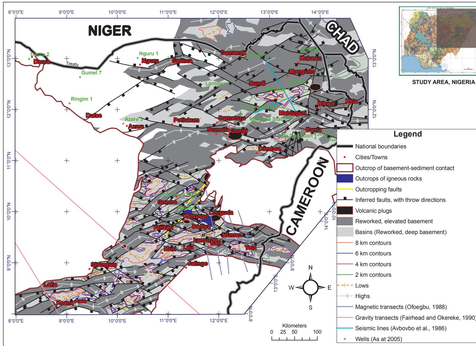
Figure H.15: Depth-structure map of sedimentary basin area of NE Nigeria showing the major depositional centers and horst structures (Figure 6.19).
