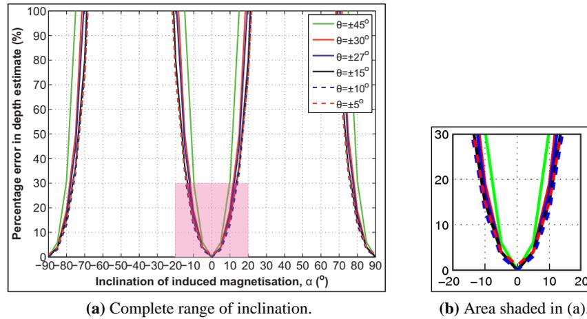
**Figure 3.7:** Percentage error ( $Err_{(z)}(\%)$ ) in depth estimates using "Tilt-Depth" method from  $|\theta| = 45, 30, 26.6, 15, 10$  and  $5$ : Effects of induced magnetisation and magnetic anomaly interference on vertical, East-West contacts. Note that error exceeds 20% for  $\theta = \pm 45$  and  $\theta = \pm 27$  at  $7$  and  $10^\circ$ , respectively, from the vertical or horizontal direction of magnetisation.
