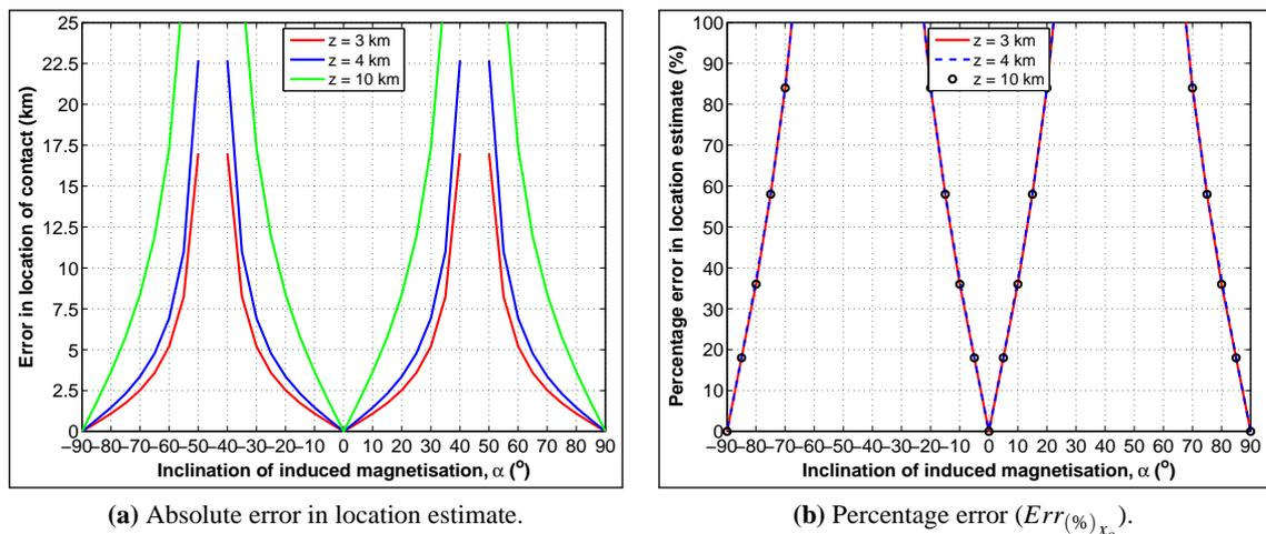
**Figure 3.4:** Effects of depth and inclination of induced magnetisation ( $\alpha$ ) on ‘‘Tilt-Depth’’ method estimates of the location of edges of vertical, East-West striking, 2D contacts. Only error ranging from 0 to 100% is shown. Remanent magnetisation is absent. Note that errors in location estimates are invariant with depth (Figure 3.4b).
