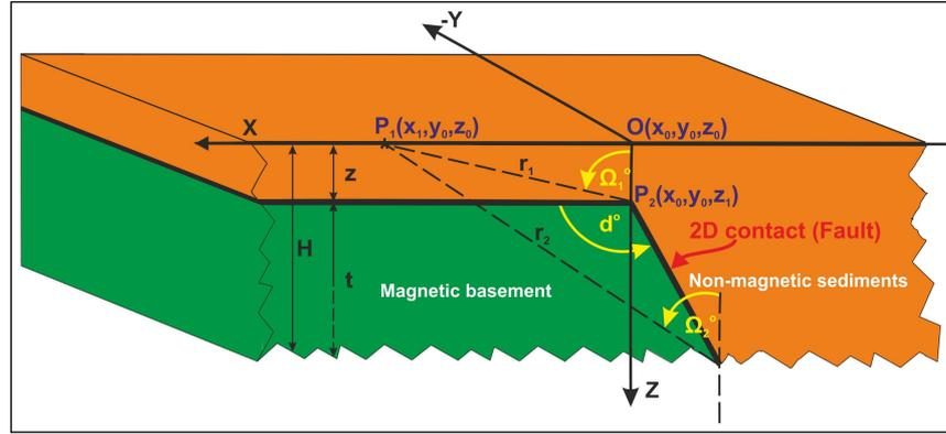
**Figure 2.9:** Sketch showing the spatial relationship between the magnetic contact/step model and the variables used to derive its  $\Delta T$  and spatial Cartesian derivatives. Note that the profile is along the  $x$ -axis, the contact strike is along the  $y$ -axis, and depth is positive downward along the  $z$ -axis. The figure is modified from Nabighian (1972).
