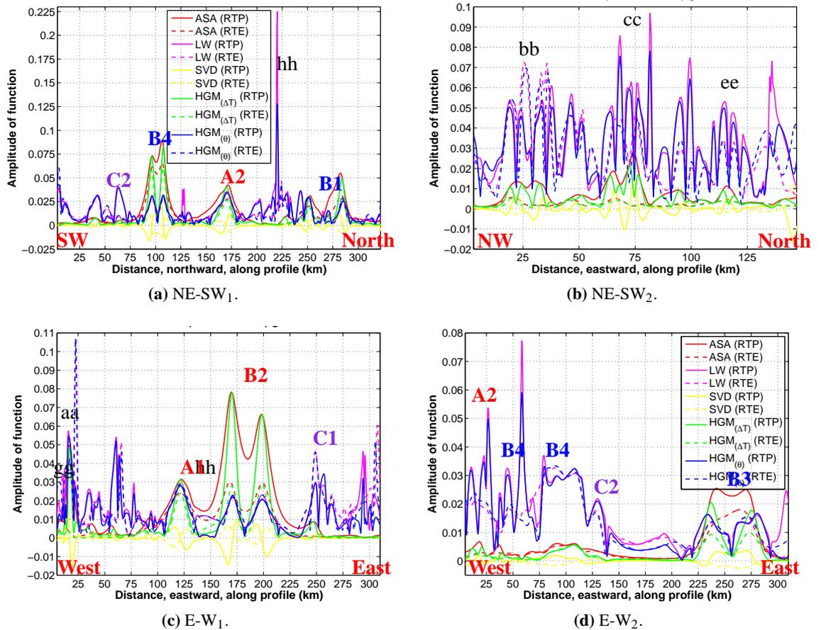
**Figure 5.6:** NE-SW and E-W oriented profiles of method-specific special functions of CBM (RTP and RTE) grids. W, E, NW, NE and SW, respectively, represent West, East, NorthWest, NorthEast and SouthWest, of the variously transformed CBM (RTP and RTE) grids. Profiles are shown in figure 5.4a. Actual cardinal direction of profile on the grids are shown at the bottom right and left corner of each figure. Legend is the same for all figures.
