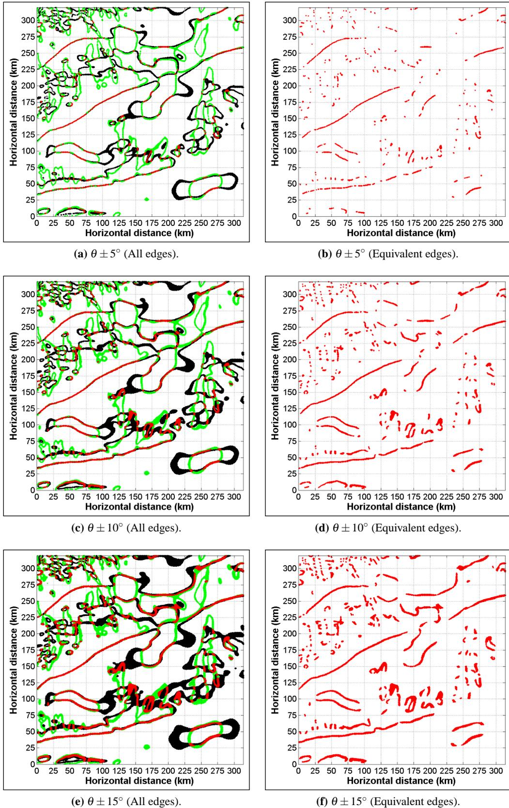
**Figure D.3:** Equivalent locations obtained from  $\theta$  of CBM (RTP and RTE) grids (In red), compared with  $\theta$  of CBM (RTP and RTE) grid locations (In green and black, respectively). Continuity and complexity of equivalent edges increased as the  $\theta^\circ$  range used increased. Using  $|\theta| > 15^\circ$  range offered no further advantage, in this example.
