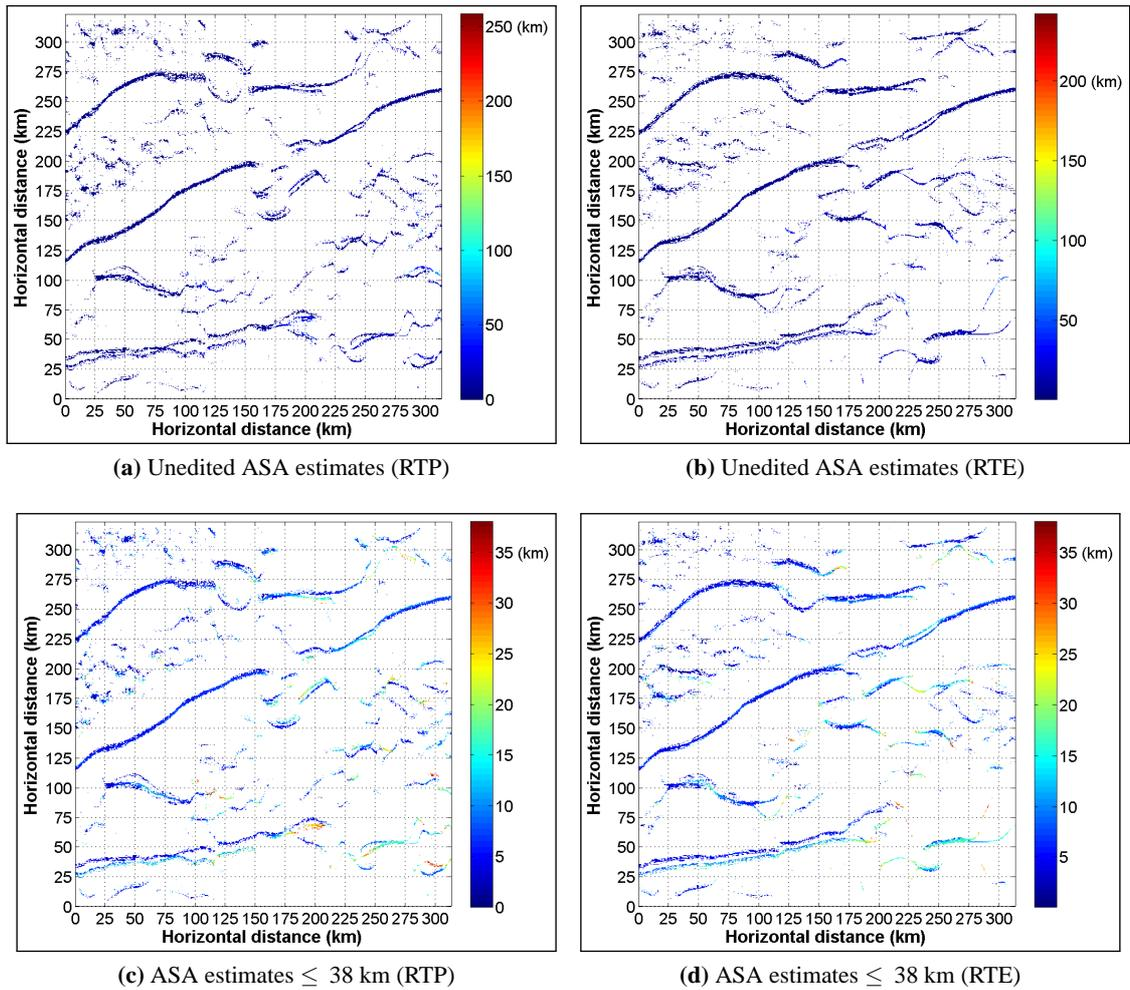
**Figure 5.10:** Unedited and edited ASA estimates from CBM (RTP and RTE) grid sources. Estimated depths are for source edges shown in figure 4.8b. Maximum of unedited ASA estimates were up to 250 km (Figures 5.10a and 5.10b), more than  $20 \times$  the maximum of actual BM basement depths (Figure 4.9b). Estimates were edited using maximum of  $\theta = \pm 27$  estimate, 38 km (Figures 4.14c and 4.14d).
