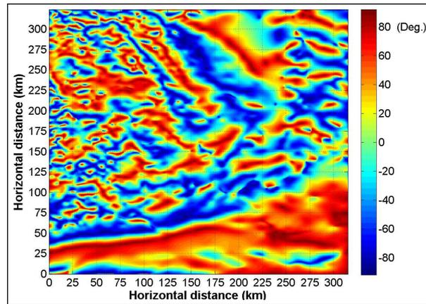
(a)  $\theta$  of SBM grid (RTE).
