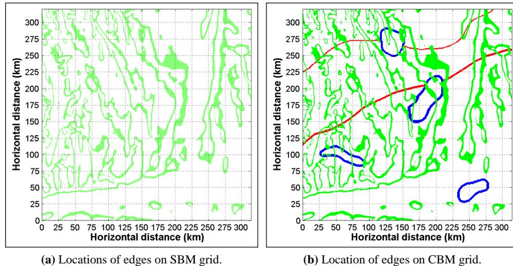
**Figure 4.8:** Locations of edges of  $\Delta T$  sources on the input BM basement grids. Edges of SBM and CBM anomaly sources are colour-coded for clarity: FS (Green), 2D magnetic contacts (Red) and non-2D (3D) magnetic contacts (Blue).
