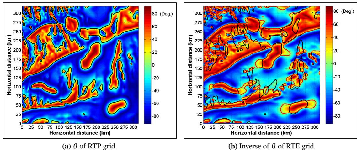
**Figure 4.7:**  $\theta$  equivalents of the CBM grid (Figure 4.3b). Black contour lines in figures 4.7a and 4.7b trace  $\theta = 0$  on figure 4.7a, but also marks the edges of all magnetic contacts on the magnetic susceptibility grid (Figure 4.2b) and *some FS* on the basement depth grid (Figure 4.2a). Red contour in figure 4.7b traces  $\theta = 0$  on the RTE  $\theta$  grid. Note that the black contour line in figure 4.7b is same as that in figure 4.7a.
