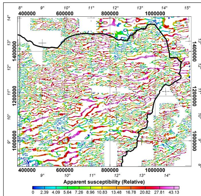
**Figure 6.20:** Relative magnetic susceptibility contrasts estimated for NE Nigeria using “Tilt-Depth”-analytic signal amplitude method (Equation (2.5.9c)). These estimates were derived from the Low-Pass NE Nigeria (RTE) grid (Figure 6.7b). An interpretation of these  $\delta k$  estimates is presented in figure 6.21.
