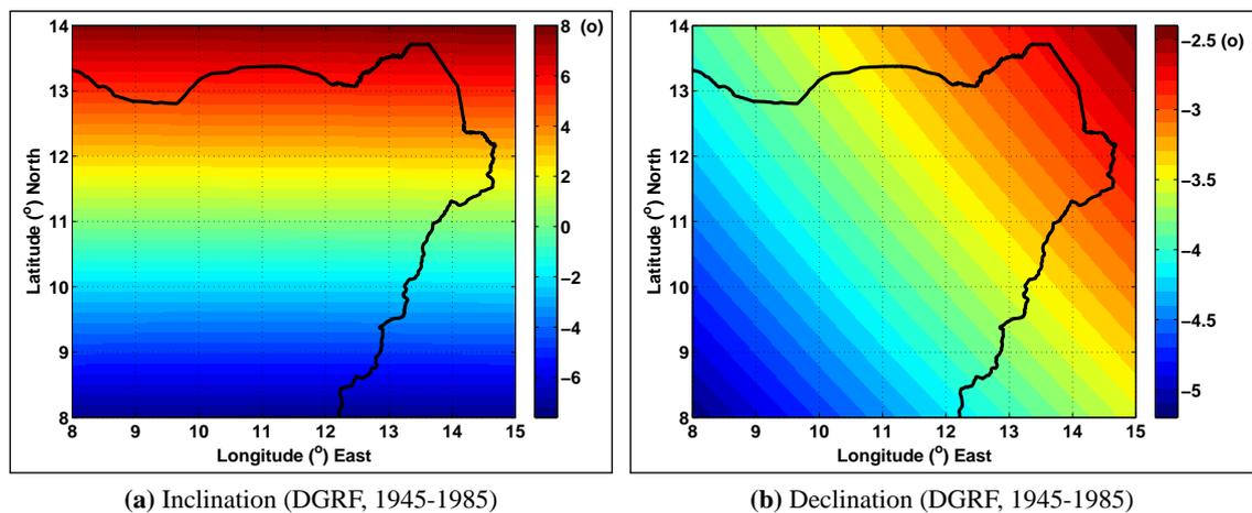
**Figure 6.5:** Inclination and declination of the regional DGRF (1945-1985), NE Nigeria, during mean aeromagnetic data acquisition date of 1<sup>st</sup> January, 1975. The Nigerian boundary around NE Nigeria is shown in black.
