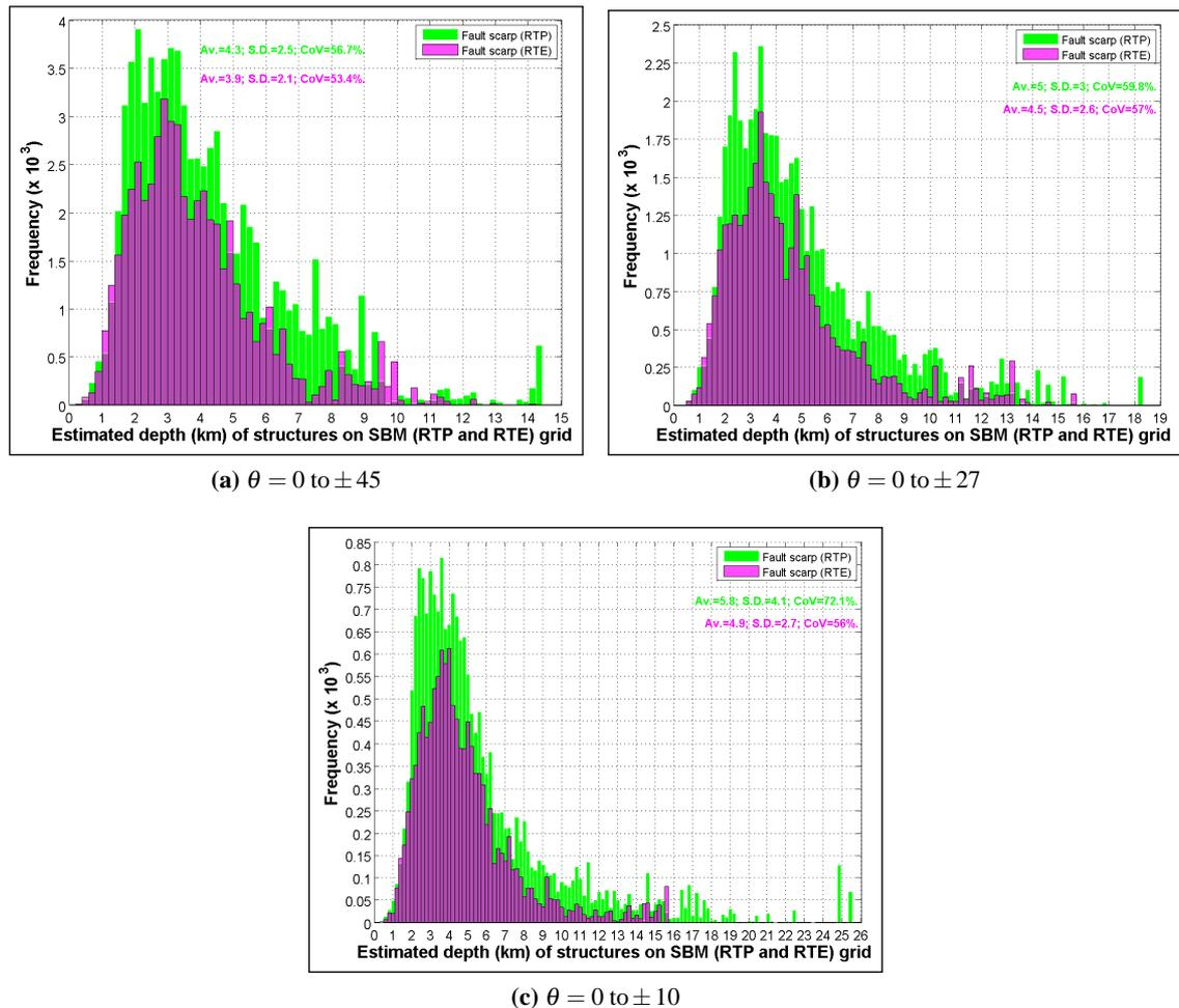
**Figure 4.13:** Histograms showing the distribution of “Tilt-Depth” method estimates of model source depths from SBM (RTP and RTE) grids. The method was implemented in three modes;  $\theta = \pm 45$ ,  $\pm 27$  and  $\pm 10$ .
