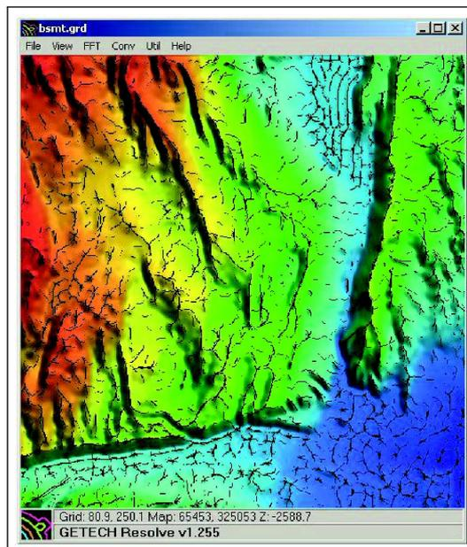
**Figure C.7:** An attempt to extract the actual locations of structural edges on the model “Bishop” basement grid, using analytic signal amplitude. Figure also shows traces of edges using maxima or peaks) of fault scarps (Black-coloured traces obtained from method of [Blakely & Simpson \(1986\)](#), introduced in section [2.5.2](#).
