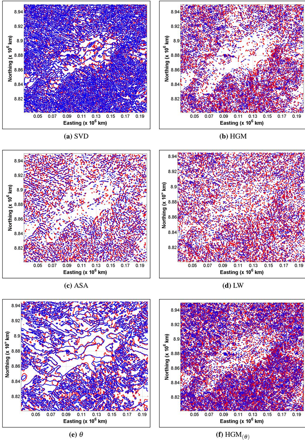
**Figure E.4:** Comparisons between locations of sources estimated from the RTP or RTE versions of the **Ruhuhu subgrid** (Figures E.3e and E.3h). Locations estimated from the RTP subgrid are in red, while those from the RTE subgrid are in blue.
