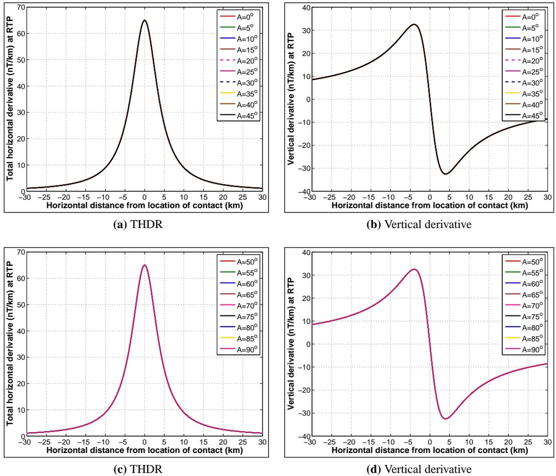
**Figure B.5:** Effects of the strike azimuth of vertical, 2D contacts on first-order Cartesian derivatives (total horizontal derivatives, THDR and vertical derivatives) of their  $\Delta T$  (RTP). THDR is  $\frac{\partial \Delta T}{\partial H}$ , while vertical derivative is  $\frac{\partial \Delta T}{\partial z}$ . Note that amplitudes and shapes of derivatives are the same, irrespective of the strike of 2D contact.
