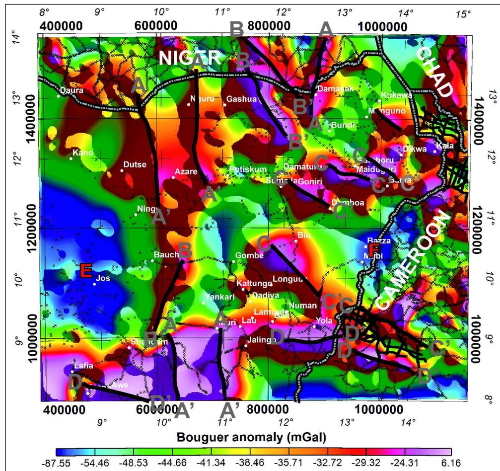
**Figure H.6:** Bouguer gravity anomaly (BA) grid shown in figure 6.8. Trends of linear short wavelength BA of positive or negative amplitude are shown (in black) and labelled (in grey). Note that isolated three-dimensional (3D) anomalies (labelled E and F, in red) also occur.
