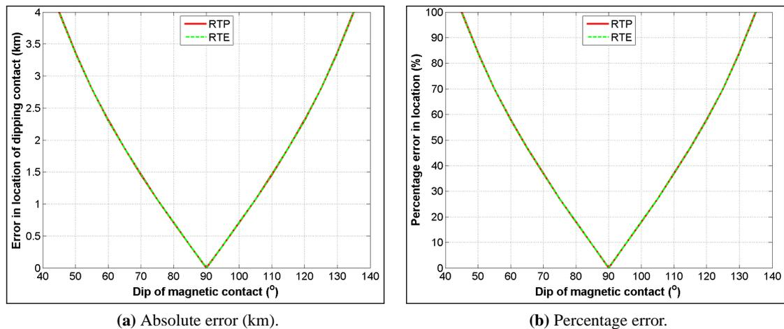
**Figure 3.14:** Effect of dips ( $d$ ) of East-West striking contacts on their location estimates. Only error ranging from 0 to 100% is shown.
