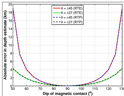
**Figure B.4:** Absolute error in depths of dipping East-West striking, 2D contacts at RTP or RTE, estimated using the  $\theta = \pm 27$  or  $45$  range. Depth estimates and percentage errors are presented in figure 3.15. Only error ranging from 0 to 100% are shown in figure 3.15b.
