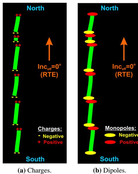
**Figure 2.8:** An illustration to show the generation of linear dipolar  $\Delta T$  (string of pearls) from magnetostatic charges along East-West (E-W) corners of locally discontinuous or en-echelon North-South (N-S) striking 2D magnetic contacts. The 2D magnetic contacts in this figure are the North-South (N-S) edges of the green-coloured structure (See also figure 2.6c).
