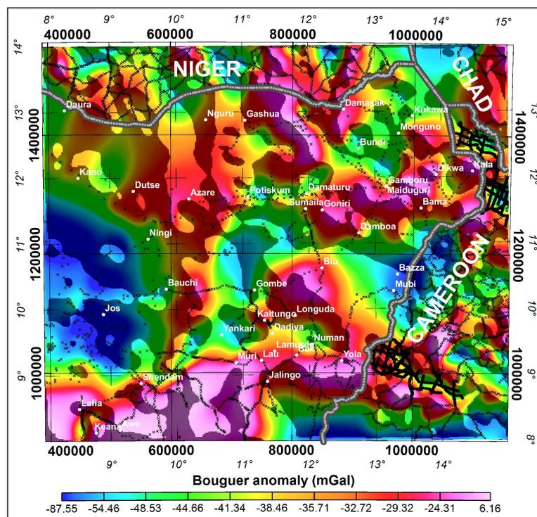
**Figure 6.8:** Bouguer gravity anomaly (BA) grid of NE Nigeria. Locations of gravity stations from which the grid was obtained is superimposed to indicate the limited constraint that can be derived from this sparse dataset within NE Nigeria. The data provides better constraint outside the study area. White labels refer to neighbouring countries and selected towns/cities in Nigeria. A magnified version of this figure, with more annotations, is shown in appendix H (Figure H.6).
