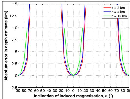
**Figure B.3:** Absolute error in depth estimates from "Tilt-Depth" method for vertical, East-West striking, 2D magnetic contacts: Effects of induced magnetisation and depth of the contact.
