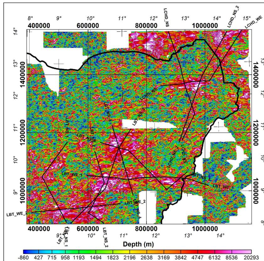
**Figure 6.16:** Local wavenumber (LW) method depth estimates. Superimposed are selected profiles, which are also shown in figure 6.17 and compared in figures 6.18, F.10, F.11 and F.12. A magnified version of figure 6.16 is presented in appendix H (Figure H.13).
