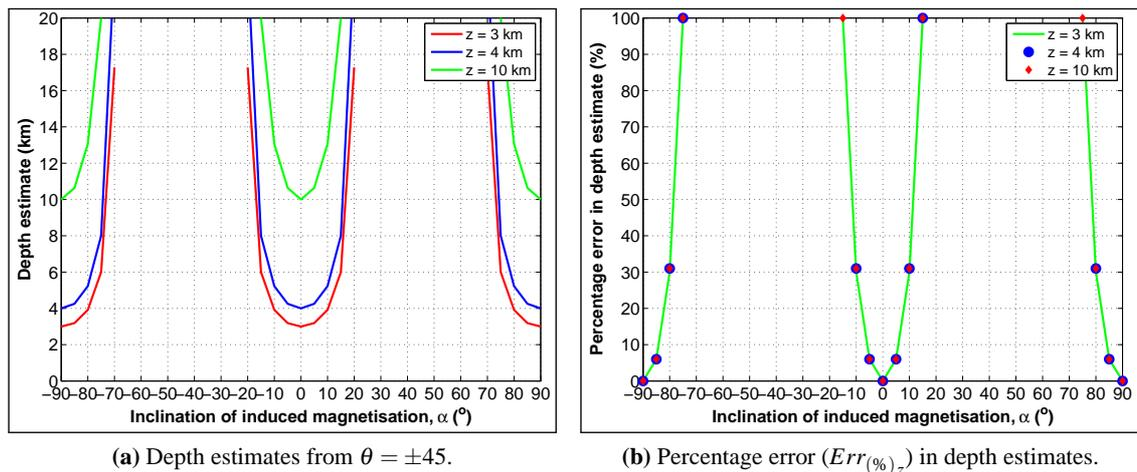
**Figure 3.5:** Effects of depth and inclination of induced magnetisation ( $\alpha$ ) on "Tilt-Depth" method estimates of depths of East-West striking, vertical, 2D contacts. Only percentage error ranging from 0 to 100% is shown. Note that errors in depth estimates are invariant with depth (Figure 3.5b).
