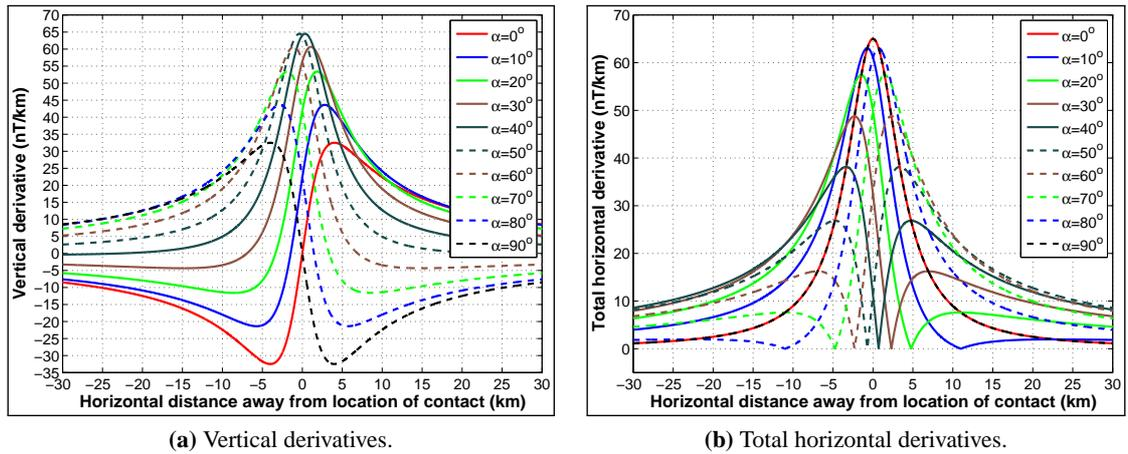
**Figure 3.2:** Effects of inclination of induced magnetisation ( $\alpha$ ) on the shape and amplitude of spatial Cartesian derivatives: (a) Vertical derivatives ( $\frac{\partial \Delta T}{\partial z}$ ); and (b) Total horizontal derivatives ( $\frac{\partial \Delta T}{\partial H}$ ), of  $\Delta T$  from vertical, E-W striking 2D magnetic contacts (depth=4 km) in the northern geomagnetic hemisphere.
