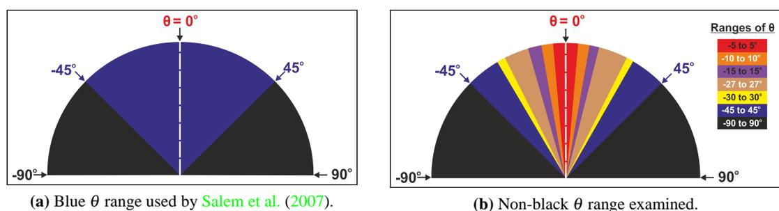
**Figure 3.6:** Length of arc (Ranges) of  $\theta$  ( $\theta_s$ ) used in testing the "Tilt depth" method. Black-coloured sectors on the  $\theta$  range-defined semicircle were not tested.
