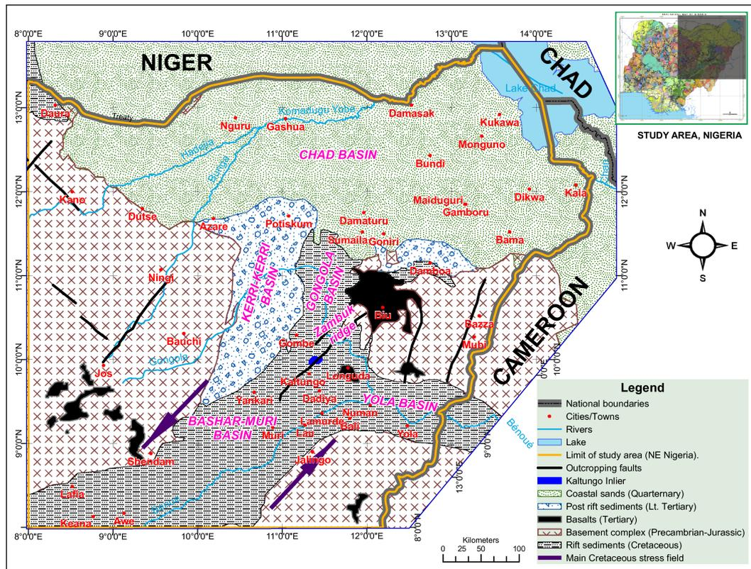
**Figure 6.2:** Simplified geological map of NE Nigeria, showing the major tectonic magnetic distinct rock units (Modified from Benkheilil et al., 1989, NGSA, 2006 and Frere, 2010). Superimposed on this map is the main Cretaceous stress field, purple arrows (Fairhead & Binks, 1991). Note outcropping NE-SW, NW-SE, and NNE-SSW trending faults. Inset is geological map of Nigeria, showing study area (shaded). A magnified version of this figure is shown in appendix H (Figure H.2).
