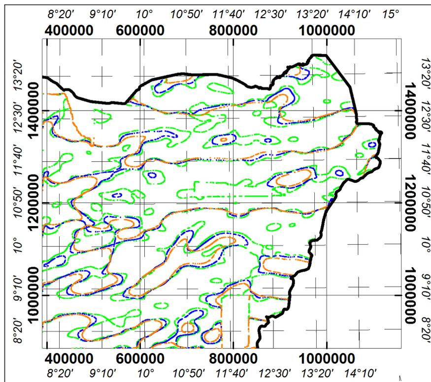
(b)  $\theta=0^\circ$  contours: 8, 20 and 30 km upward-continued (Figure 6.14b).
