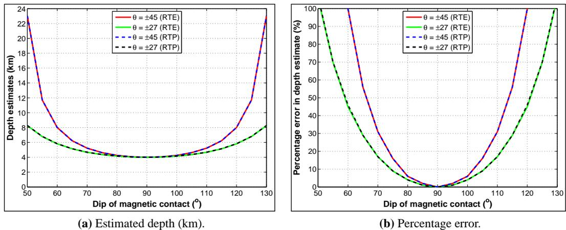
**Figure 3.15:** “Tilt-depth” method estimates of depths of dipping, East-West striking magnetic contacts at RTP and RTE, using  $\theta = \pm 27$ , or 45 range. Only error ranging from 0 to 100% is shown in figure 3.15b. Absolute error is presented in figure B.4.
