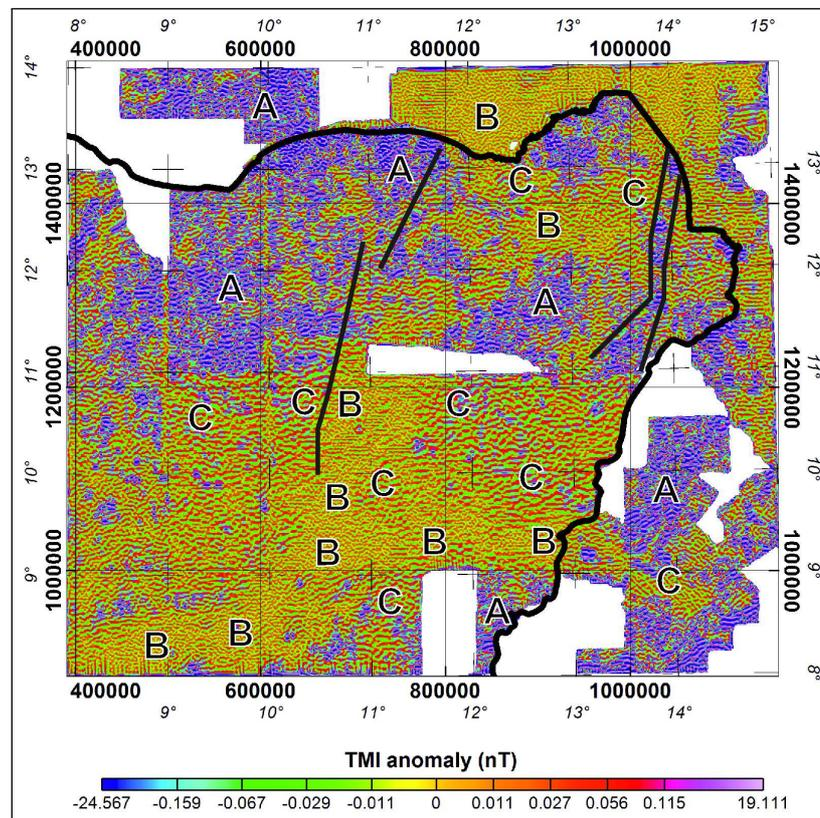
(a) High-Pass Butterworth-filtered NE Nigeria  $\Delta T$  grid (Figure 6.7a).
