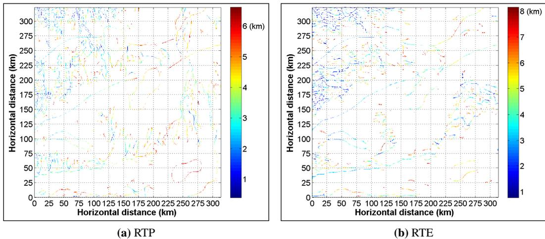
**Figure 5.11:** LW estimates from CBM (RTP and RTE) grid sources. Estimated depths are for source edges shown in figure 4.8b. LW estimates may be deeper for some shallow sources (Compare estimates for sources in NW of CBM grid and actual depths on basement depth grid in figure 4.2a). Maximum LW estimates were within the range of actual depths of BM sources (Figure 4.9b).
