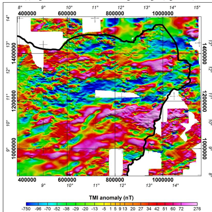
(b) Low-Pass Butterworth-filtered NE Nigeria  $\Delta T$  grid (Figure 6.7b).
