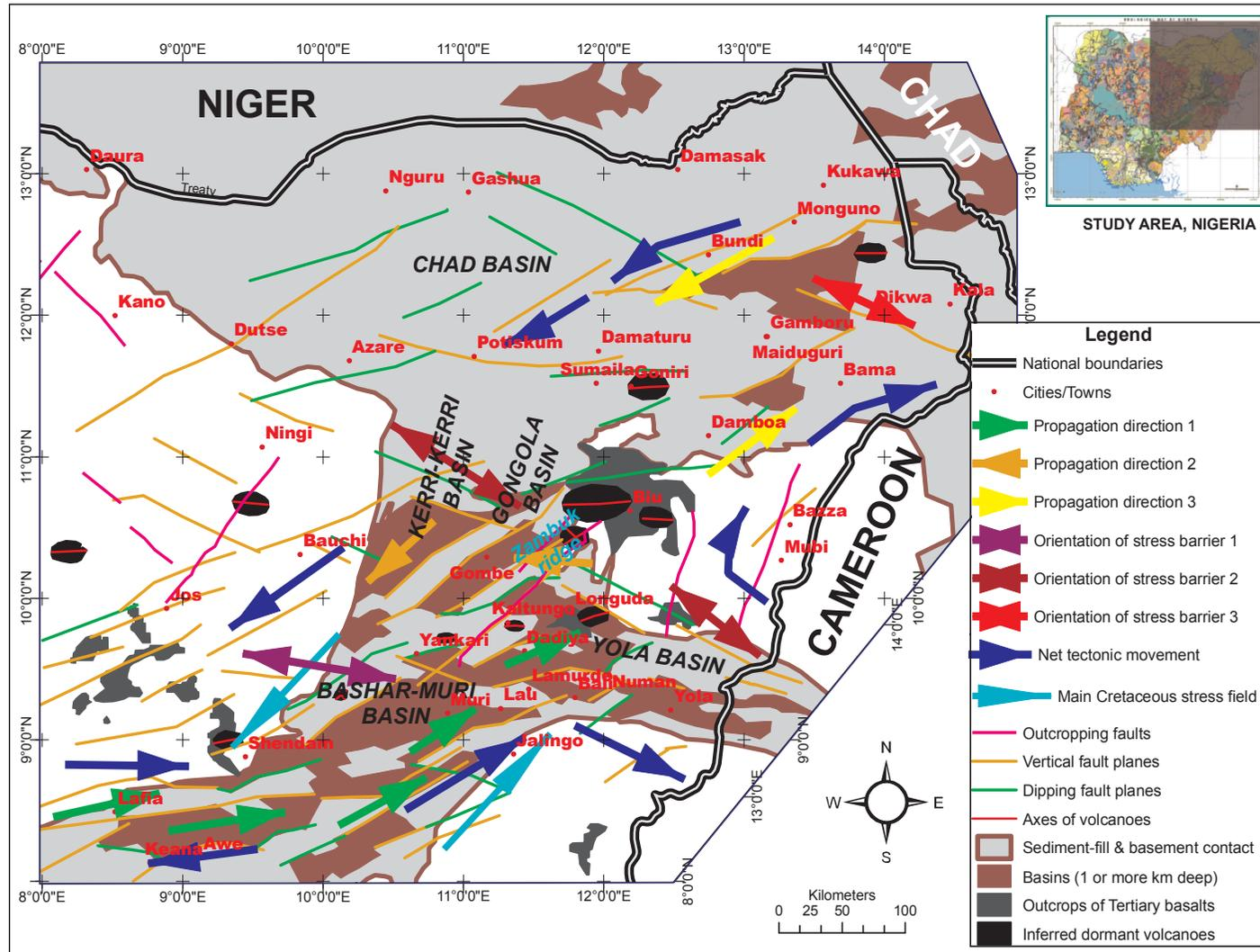
**Figure H.17:** Inferred directions of propagation of the Benue rift and Mesozoic tectonism in study area (Figure 7.1).
