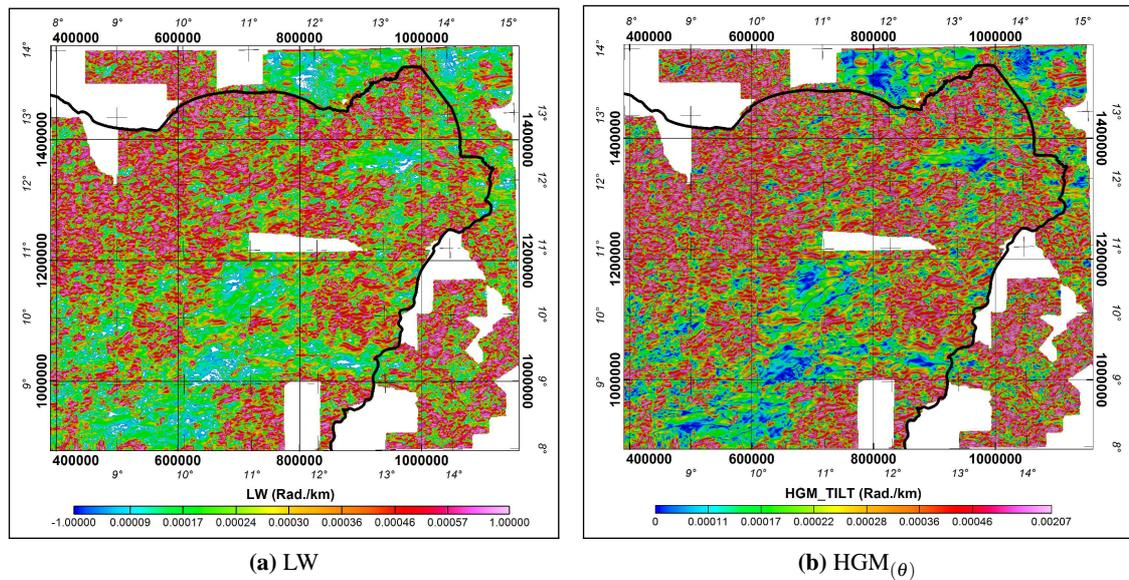
**Figure 6.11:** LW and  $HGM_{(\theta)}$  maps of NE Nigeria. Maps were derived from the Low-Pass filtered  $\Delta T$  grid (Figure 6.7b). Local maxima of LW or  $HGM_{(\theta)}$  estimate locations of structural edges. Note that values that tend very close to 0 have been masked from the LW grid (Figure 6.11a). Magnified versions of these figures are presented in appendix H (Figure H.9).
