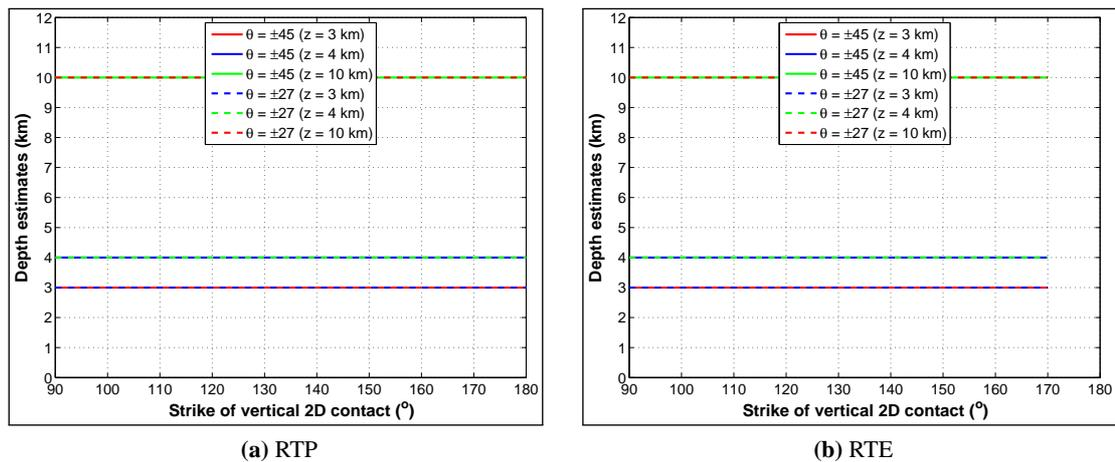
**Figure 3.20:** Effect of azimuthally varying strike of vertical contacts on “Tilt-Depth” estimates of depth, when contact is either at RTP or RTE. The method works well on contacts of all strike directions when RTP, but only for contacts with non-North-South strike directions (90 to 170°), when at RTE. See Figure 3.19 and text for explanation.
