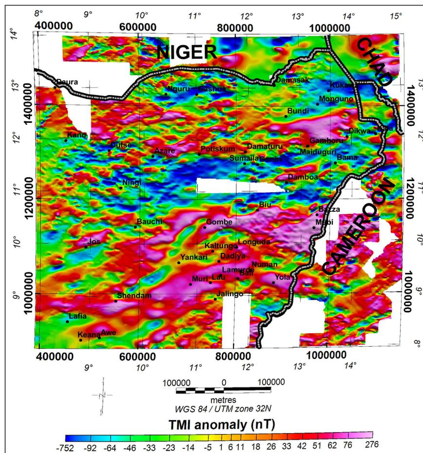
**Figure 6.6:** RTE of NE Nigeria  $\Delta T$  grid (Figure 6.4). The Nigerian border with Niger, Chad and Cameroon is shown. Major cities/towns are shown in white for easy reference. A more annotated, magnified version of this figure is shown in appendix H (Figure H.4).
