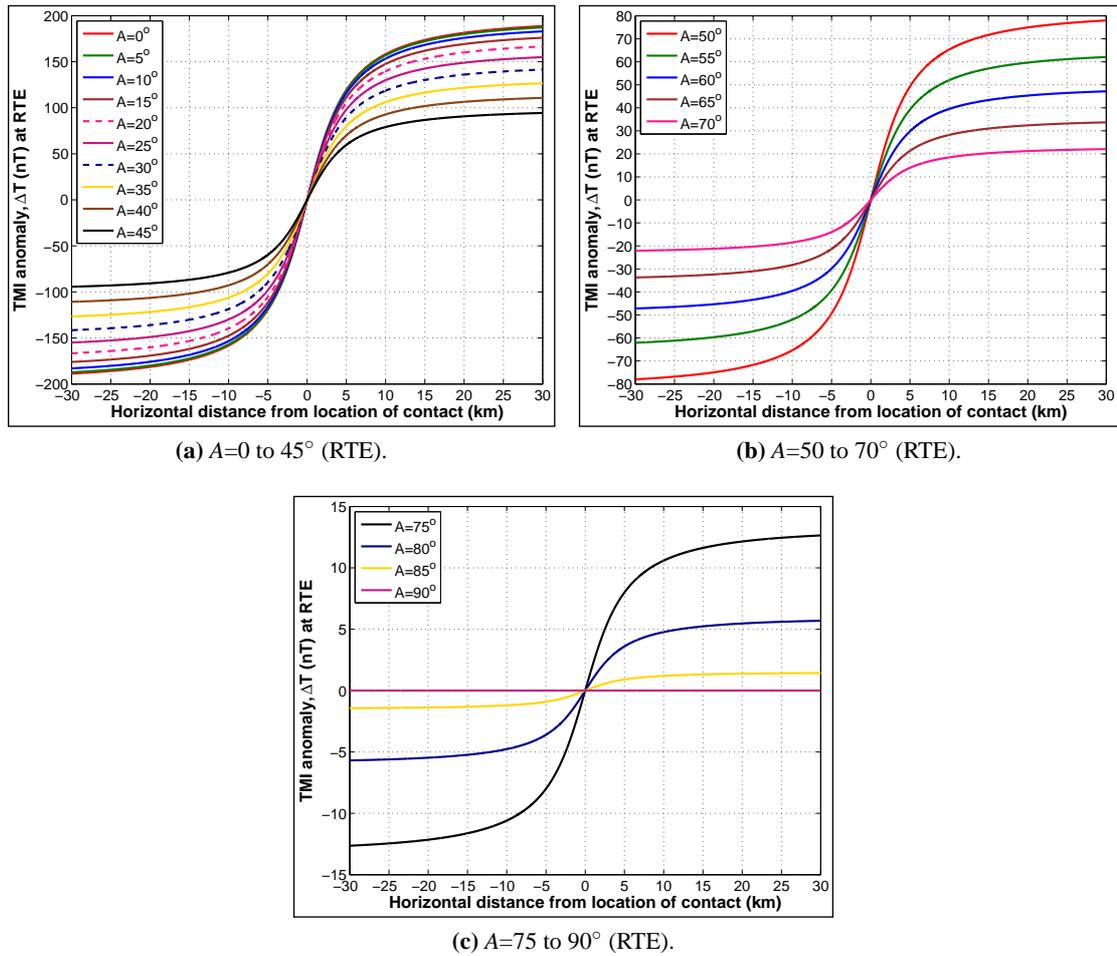
**Figure 3.17:** Effect of strike azimuth of vertical contacts on amplitude and shape of  $\Delta T$ , when effective and induced magnetisations are horizontal (RTE). Unlike the case in figure 3.16, amplitudes of  $\Delta T$  vary systematically from a maximum when the contact strikes East-West ( $A = 0^\circ$ ) to 0 when the contact strikes North-South ( $A = 90^\circ$ ). Also, the maximum amplitude when the contact strike is East-West is half its equivalent at RTP.
