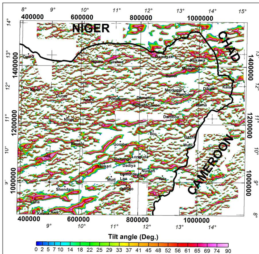
**Figure F.8:** Additive inverse ( $\times -1$ ) of  $\theta \geq 0$  map of NE Nigeria. Map was obtained from grid in figure 6.9b, by masking grid locations where  $\theta < 0$ , leaving only locations where possibly elevated basement (horsts or plutons) may occur.
