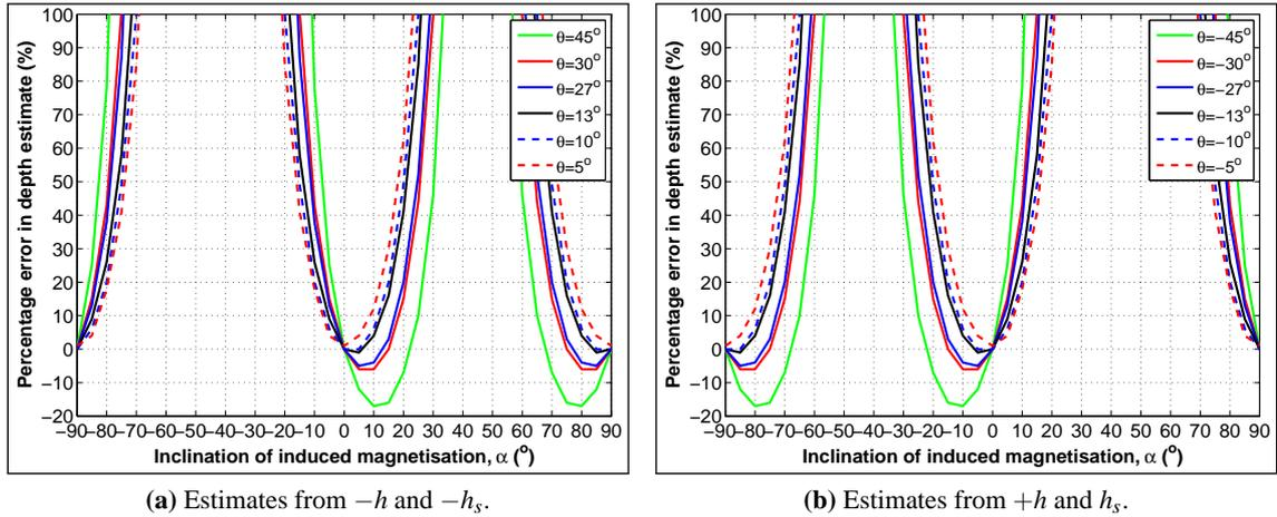
**Figure 3.8:** Percentage error ( $Err_{(\%)}$ ) in depth estimates from  $\Delta T$  data from either  $+\theta$  ( $-h$  or  $-h_s$ ) or  $-\theta$  ( $+h$  or  $+h_s$ ) values for vertical, E-W contacts.  $+h$  or  $+h_s$  is distance between  $\theta = 0$  and  $-\theta$  values, while  $-h$  or  $-h_s$  is distance between  $\theta = 0$  and  $+\theta$  values.
