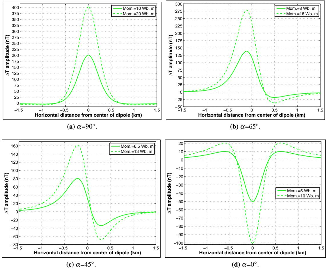
**Figure 2.3:** Comparisons between South-North (S-N) profiles across grids shown in figure 2.2 and equivalent grids with twice as much dipole moment ( $m$ ) magnitudes.  $\alpha$  is inclination of induced magnetisation. Dashed green profiles are from grids with dipole moment magnitude ( $m$ ) twice those of grids from which the solid green profiles were extracted. South is left, while North is right of the figure.
