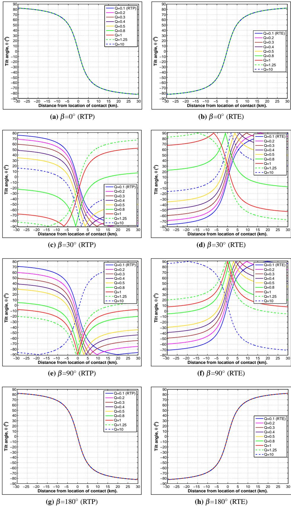
**Figure 3.12:**  $\theta$ -transformed  $\Delta T$  curves obtained from vertical, West-East striking contacts when at RTP or RTE, and characterised by remanent magnetisations of various  $Q$  and inclinations ( $\beta=0, 30, 90$  and  $180^\circ$ ). Note that anomalies are only simplified when  $\beta=0, 90$  or  $180^\circ$ .
