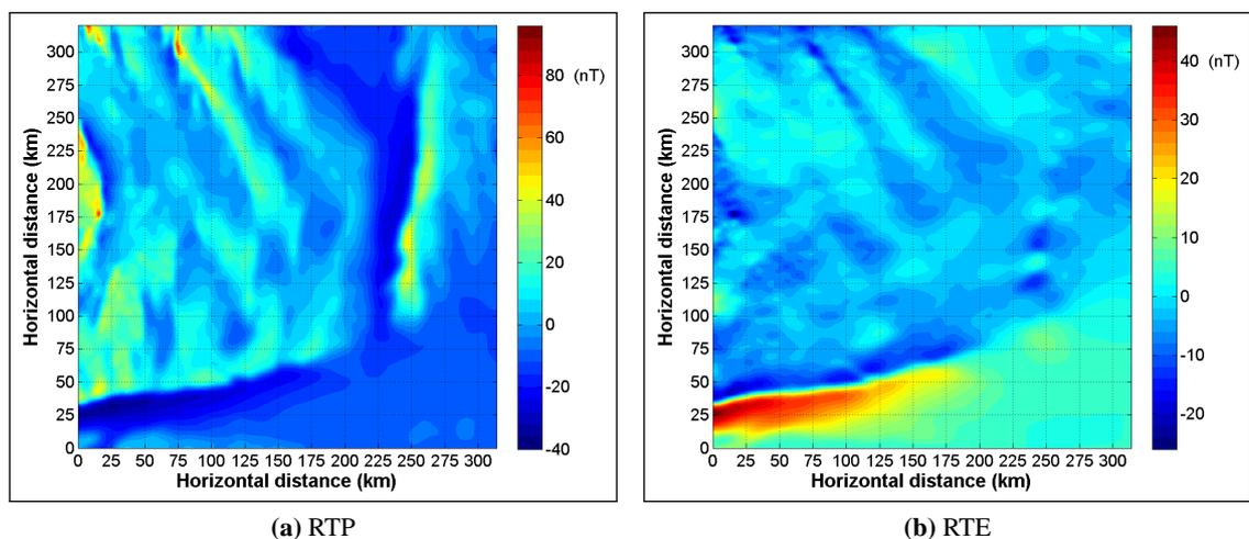
**Figure 4.4:** RTP and RTE transformed equivalents of the SBM grid (Figure 4.3a). All fault scarps (FS) in figure 4.2a are visible on SBM (RTP) grid (Figure 4.4a) irrespective of strike directions. Of the three major FS strike directions (N-S, E-W and NW-SE) in figure 4.2a, the E-W striking FS is well imaged, NW-SE striking FS are poorly imaged, while N-S trending FS are not imaged at all on the SBM (RTE) grid (Figure 4.4b).
