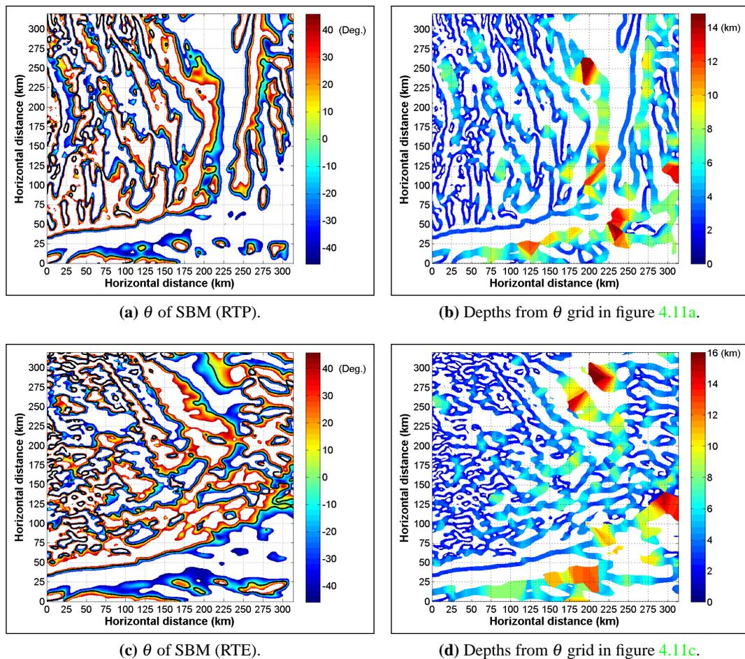
**Figure 4.11:** “Tilt-Depth” estimation of depth of fault scarp (FS) edges from SBM (RTP and RTE) grids, using  $0 \leq |\theta| \leq 45$  range. Black contour lines in figures 4.11a and 4.11c trace  $\theta = 0$ . Note that estimated depths are for locations traced by the  $\theta = 0$  contours. Erroneous locations (discussed in text) are introduced in RTE grids, and depths for such locations are spatially misplaced.
