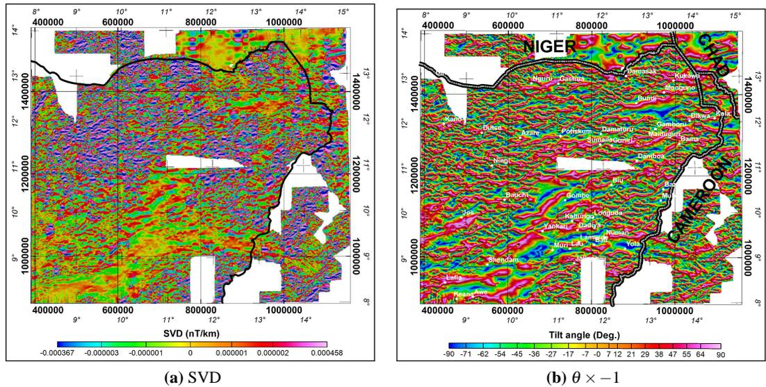
**Figure 6.9:** SVD and  $\theta$  maps of NE Nigeria. These maps were derived from the Low-Pass filtered  $\Delta T$  grid (Figure 6.7b). Locations of structural edges are estimated using SVD=0 or  $\theta = 0$  contours. Magnified versions of these figures are presented in appendix H (Figure H.7).
