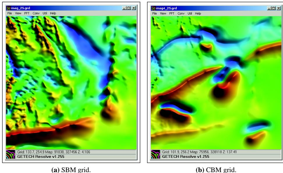
**Figure C.2:** Enhanced (GETgrid<sup>TM</sup>) visualization of the “Bishop” model  $\Delta T$  grids for inclination of induced magnetisation of 25°: (a) SBM grid, same as in figure 4.3a; and (b) CBM grid, same as in figure 4.3b.
