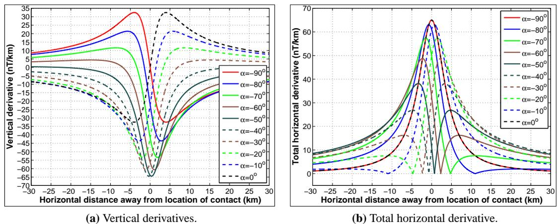
**Figure B.2:** Effects of inclination of induced magnetisation ( $\alpha$ ) on the shape and amplitude of derivatives of  $\Delta T$  from vertical, E-W, 2D contacts in the Southern geomagnetic hemisphere.  $\alpha$  ranged from  $0$  to  $-90^\circ$ : (a) Vertical derivatives; and (b) Total horizontal derivative.
