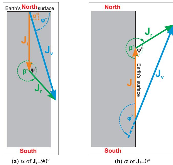
**Figure 3.9:** Spatial relationship between induced, remanent and effective (net) magnetisations ( $J_i$ ,  $J_r$  and  $J_v$ ) at the: (a) North pole (RTP); or (b) equator (RTE). The relative magnitude (length) of  $J_r$  and  $J_i$  is expressed by the Koenigsberger ratio ( $Q$ ). Magnetisation vectors are shown in cross-section through an appropriately oriented, section of a magnetic rock unit (grey-coloured) at the Earth's surface.
