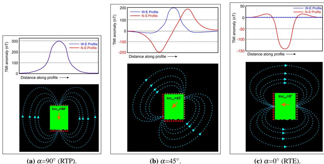
**Figure 2.7:** Schematic showing North-South, N-S (Red-coloured) and East-West, E-W (Blue-coloured) profiles across North-South (N-S) cross sections of  $\Delta T$  resulting from the magnetostatic charge distributions shown in figure 2.6. The green-coloured structure and its magnetic 2D contacts strike perpendicularly into the page.
