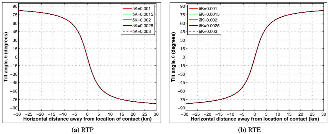
**Figure B.1:** Testing computer codes using the independence of  $\theta$  from vertical, E-W magnetic 2D contacts at RTP on susceptibility contrasts ( $\delta k$ ).
