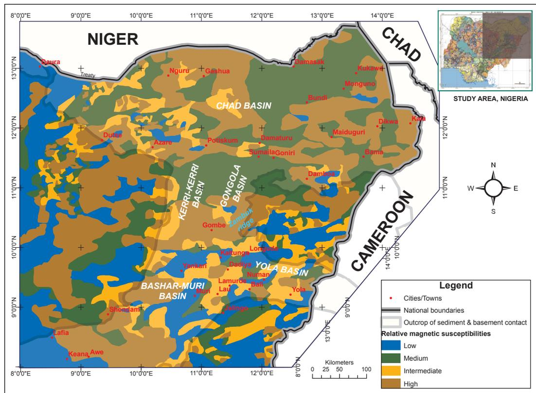
**Figure 6.21:** Relative magnetic susceptibility distribution map for NE Nigeria basement. This map is based on the susceptibility estimates shown in figure 6.20. Geological basins in these vicinities are labelled, in line with figure 6.2, to provide context. Locations of outcropping sediments and/or basement-sediment contact in NE Nigeria extracted from figure 6.2 is superimposed to ease comparisons.
