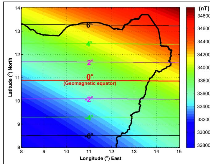
**Figure F.2:** Spatial relationship between inclination (Horizontal lines) and TMI amplitude of the regional DGRF (Barracough, 1987) in NE Nigeria, for 1<sup>st</sup> January, 1974. The Nigerian boundary is shown in black. Extracted contours of  $\alpha$  (The lines) show the: geomagnetic equator ( $\alpha = 0^\circ$  in red);  $\alpha = 2^\circ$  and  $-2^\circ$  (in pink);  $\alpha = 4^\circ$  and  $-4^\circ$  (in green); and  $\alpha = 6^\circ$  and  $-6^\circ$  (in black).
