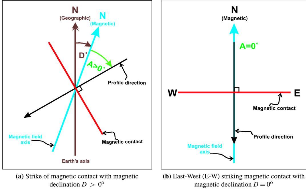
**Figure 2.10:** Strike (Spatial horizontal orientation) of 2D magnetic contacts relative to the geomagnetic north (N) pole. NB: For all variations of the contact, the profile direction is always perpendicular to the strike of the 2D contact.
