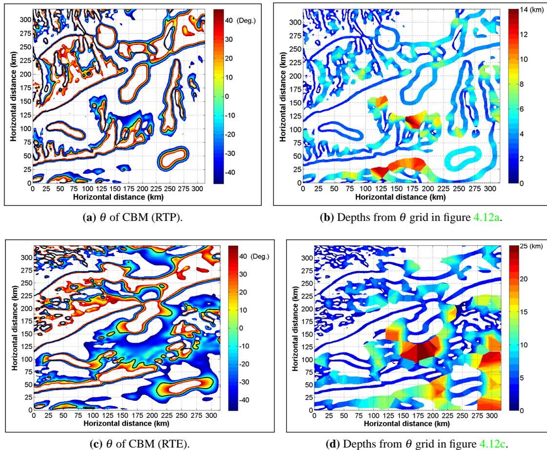
**Figure 4.12:** “Tilt-Depth” estimation of depth of geological structures; fault scarp (FS) and magnetic contact edges, on CBM (RTP and RTE) grids, using  $0 \leq |\theta| \leq 45$  range. Black contour lines in figures 4.12a and 4.12c trace  $\theta = 0$ . Note that estimated depths are for locations traced by the  $\theta = 0$  contours. Erroneous locations (discussed in text) are introduced in RTE grids, and depths for such locations are spatially misplaced.
