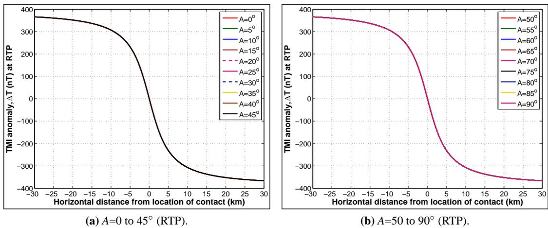
**Figure 3.16:** Effect of strike azimuth of vertical contacts on amplitude and shape of  $\Delta T$ , when effective and induced magnetisations are vertical (RTP). Amplitudes and shapes of  $\Delta T$  for the various strike directions ( $A$ ) are the same, so these plots stack on top of each other irrespective of the strike of contact.
