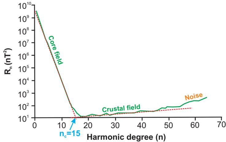
**Figure 2.1:** A sketch of the radial average power ( $R_n$ ) of models of the geomagnetic field obtained from the low-Earth orbiting (LEO) satellite: MAGSAT, as a function of spherical harmonic ( $n$ ). The red dashed lines indicate linear fits to  $2 \leq n \leq 15$  and  $n > 15$ , believed to indicate the two main sources of the Earth’s magnetic field. Modified from (Cain et al., 1989; Sabaka et al., 2004 and Gubbins, 2010).
