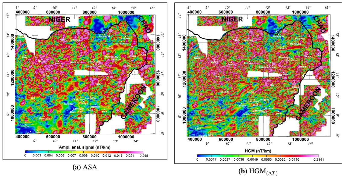
**Figure 6.10:** ASA and  $HGM_{(\Delta T)}$  maps of NE Nigeria. Maps were derived from the Low-Pass filtered  $\Delta T$  grid (Figure 6.7b). Local maxima of ASA or  $HGM_{(\Delta T)}$  estimate locations of structural edges. Magnified versions of these figures are presented in appendix H (Figure H.8).
