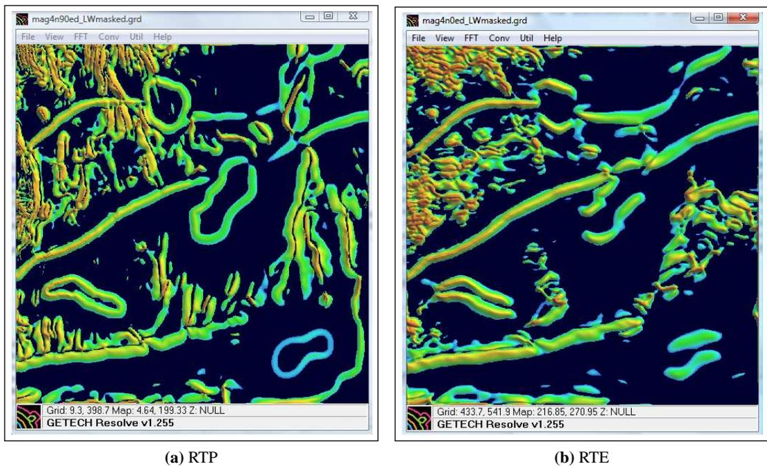
**Figure D.8:** Windowed versions of the LW of CBM (RTP and RTE) grids (Figures 5.3a and 5.3b). Grids were windowed using cut-off LW value determined using equation 5.4.1. LW depths in figure 5.11 were estimated from maxima extracted from these grids.
