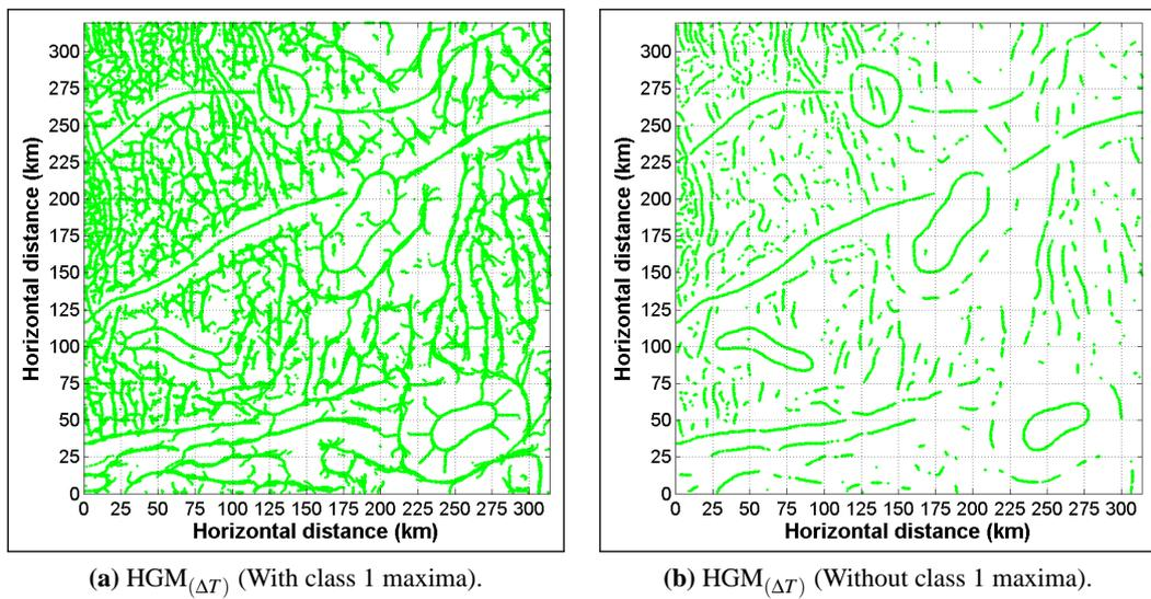
**Figure D.2:** Demonstrating the additional clarity gained by editing estimated locations obtained from CBM (RTP) grid, using  $HGM_{(\Delta T)}$  method. Continuity of  $HGM_{(\Delta T)}$  peaks (edges) reduced as lower class peaks were removed. Location estimates in figure D.2b are more representative of actual CBM sources (Figure 4.8b) and easier to interpret than those in figure D.2a.
