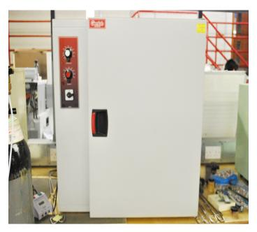
Figure 4: Picture of the oven used for sample heating for moisture content analyses. Samples were collected after harvest and heated for one hour until the moisture was completely driven off.
