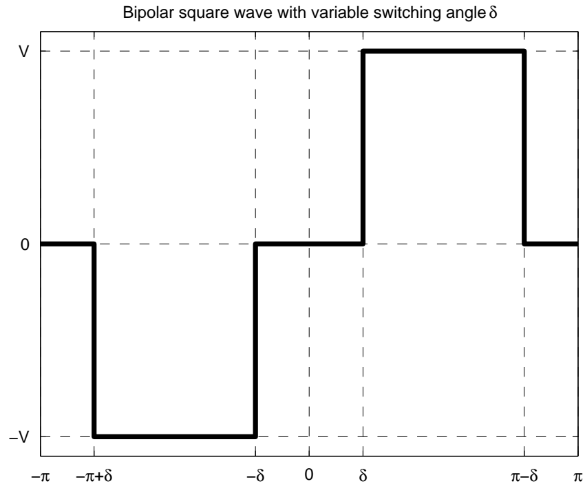
Figure 5.3: Bipolar square wave with variation of switching angle \delta
