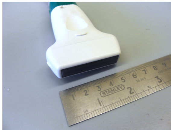
Figure 4.76: Photograph of the L3-8/40EP array transducer (Prosonic Co Ltd., Gyong-Buk, Korea), 128 elements, \lambda pitch, 4.8 MHz average centre frequency, 57% fractional bandwidth.
