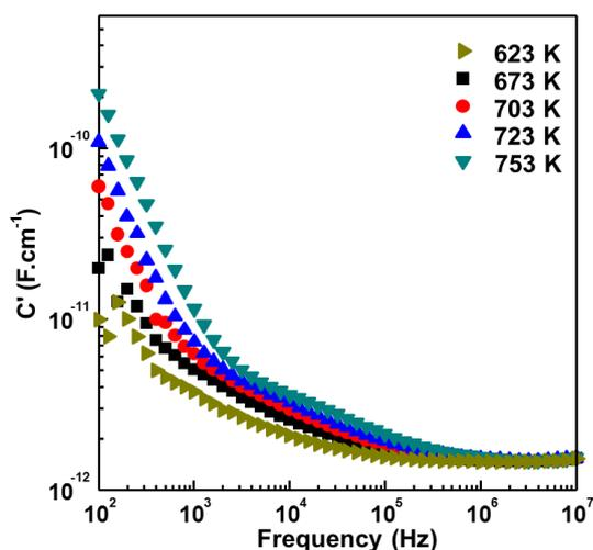
**Figure 9.16**  $C'$  spectroscopic plot showing the capacitance fluctuation at various temperatures for  $\text{Bi}_{12}(\text{Bi}_{0.4}\text{Al}_{0.6})\text{O}_{19.5}$ .
