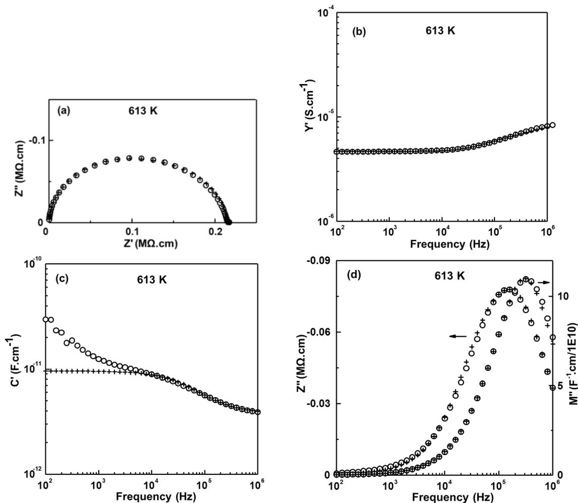
**Figure 9.12** High temperature IS experimental data points (○) and the fitting results (+) to
