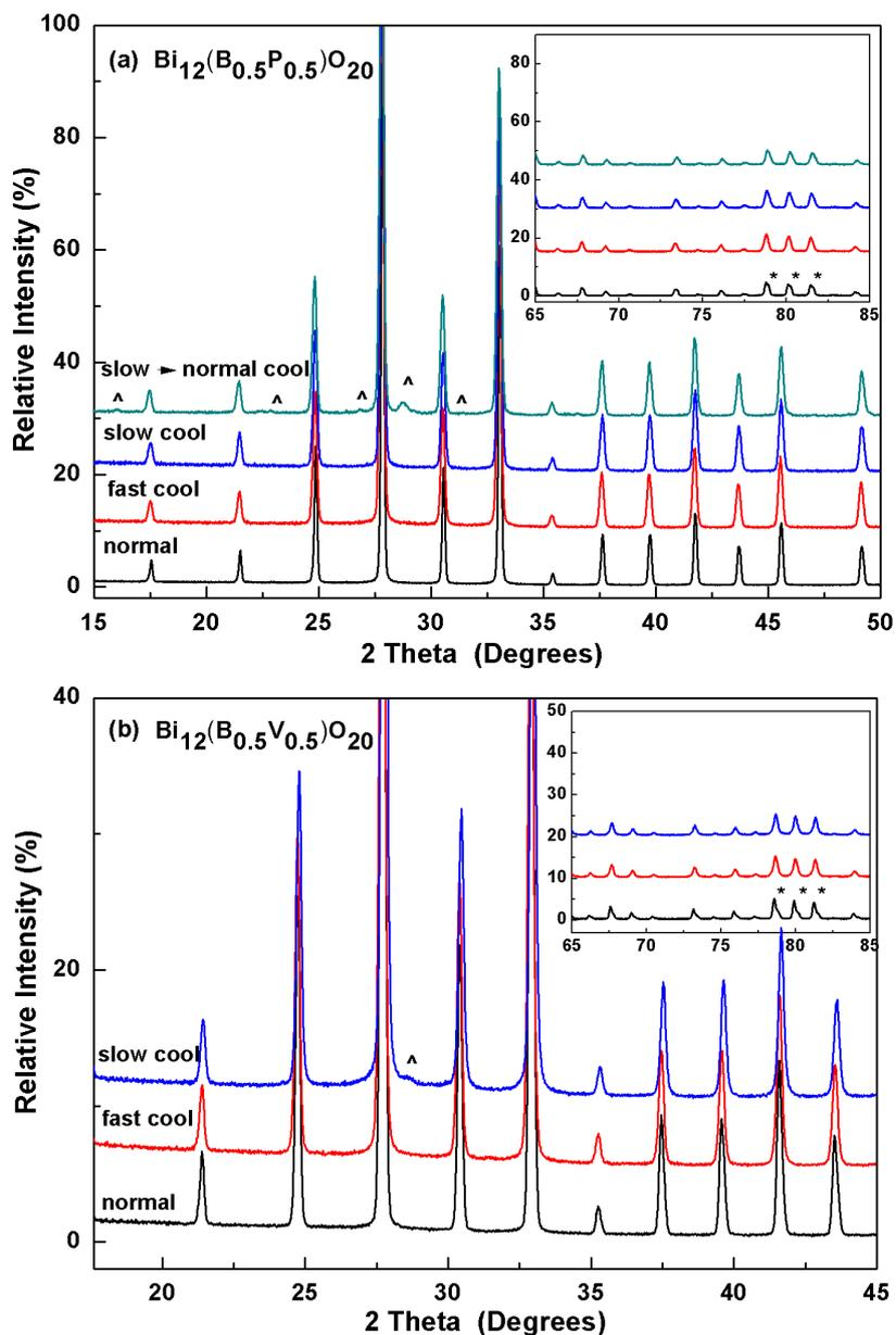
**Figure 5.7** XRPD results of (a)  $Bi_{12}(B_{0.5}P_{0.5})O_{20}$  reacted at 730 °C for 36h and (b)  $Bi_{12}(B_{0.5}V_{0.5})O_{20}$  at 740 °C for 48h with a normal (standard) cooling rate of 10 °C/min; a fast cooling rate (i.e. air quenching) and a slow cooling rate of 1 °C/min, respectively. Notation \* and ^ indicate the second sillenite phase with a smaller unit cell and a secondary phase of  $Bi_4B_2O_9$  (ICCD card [70-1458]), respectively.
