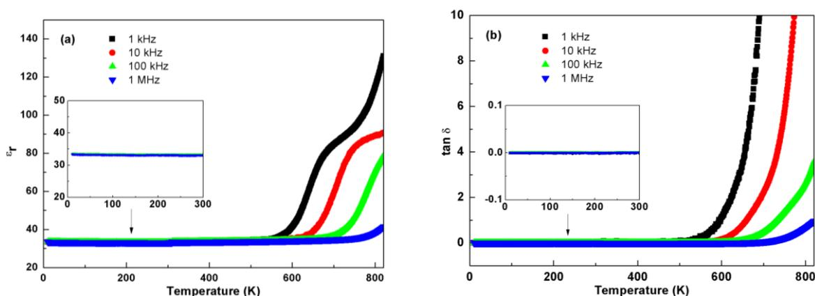
**Figure 4.27** Temperature dependence of (a) permittivity and (b) dielectric losses of compound  $\text{Bi}_{12}(\text{Bi}_{0.67}\text{Zn}_{0.33})\text{O}_{19.33}$ . Insets are expanded view of lower temperature data between 10 and 300 K.
