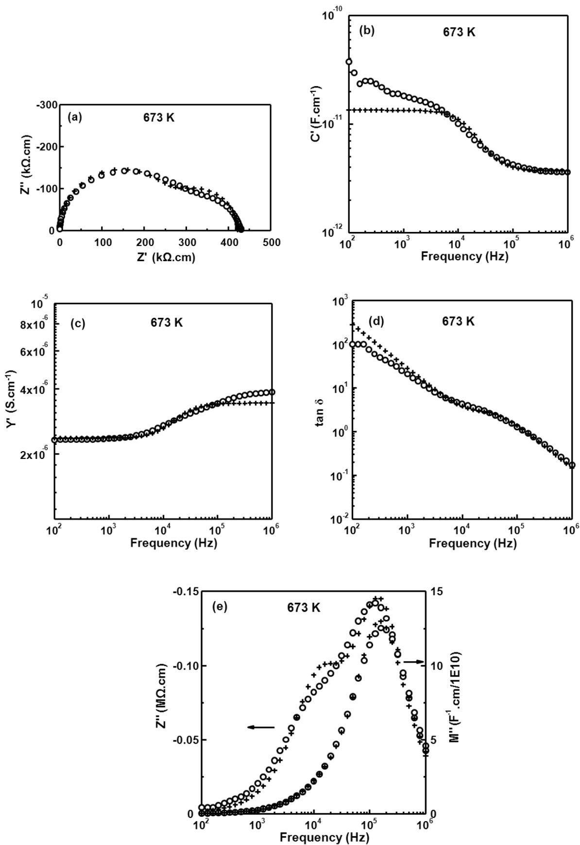
**Figure 3.13** (a) Impedance  $Z^*$  plot and spectroscopic plots of (b)  $C'$ , (c)  $Y'$ , (d)  $\tan \delta$  and (e)  $-Z''$  and  $M''$  of  $\text{Bi}_{12}\text{SiO}_{20}$  measured at 673 K (open symbols) and the best-fit results (cross
