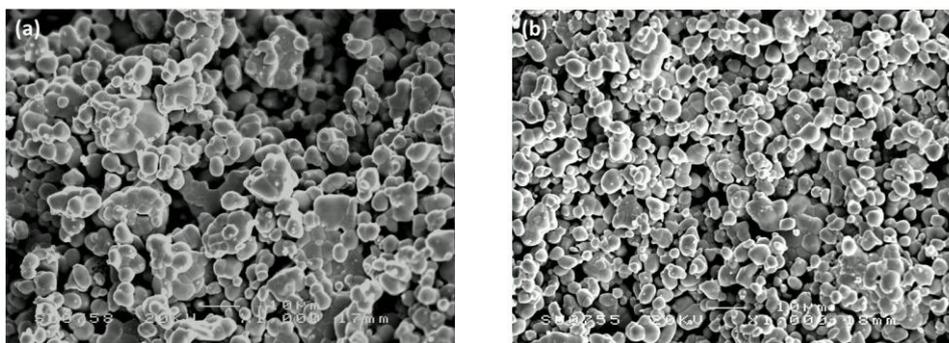
**Figure 4.12** SEM image of (a)  $\text{Bi}_{0.4}\text{Al}_{0.6}$  and (b)  $\text{Bi}_{0.3}\text{Al}_{0.7}$ .
