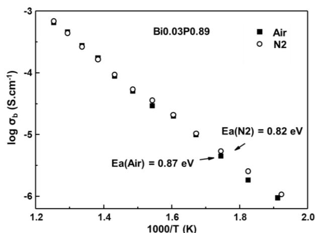
**Figure 6.13** Conductivity of  $Bi_{0.03}P_{0.89}$  measured in air (filled square) and nitrogen (empty circle).
