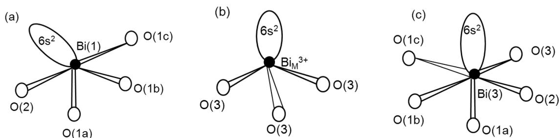
**Figure 4.36** Schematic representation of Bi-polyhedron in  $M^{2+}/M^{3+}$  sillenites with (a)  $\text{Bi}(1)\text{O}_4\text{LP}$ ; (b)  $\text{Bi}_M\text{O}_3\text{LP}$  and (c)  $\text{Bi}(3)\text{O}_5\text{LP}$ .<sup>[9]</sup>
