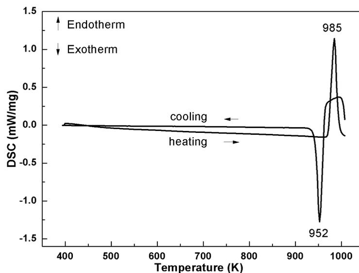
**Figure 4.19** DSC trace of Bi<sub>0.7</sub>In<sub>0.3</sub>.
