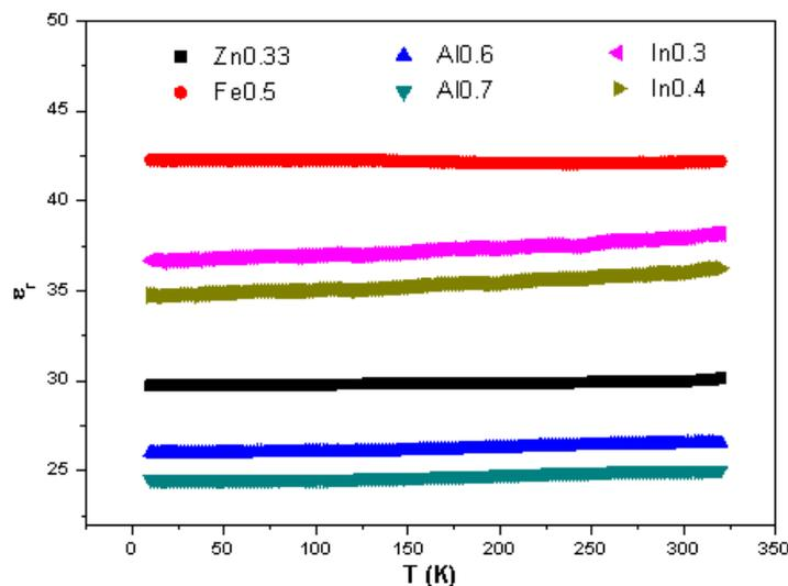
**Figure 4.26**  $\epsilon_r$  versus T for six sillenites:  $\text{Bi}_{0.67}\text{Zn}_{0.33}$ ,  $\text{Bi}_{0.5}\text{Fe}_{0.5}$ ,  $\text{Bi}_{0.3}\text{Al}_{0.7}$ ,  $\text{Bi}_{0.4}\text{Al}_{0.6}$ ,  $\text{Bi}_{0.6}\text{In}_{0.4}$  and  $\text{Bi}_{0.7}\text{In}_{0.3}$  extracted from an LCR meter (at 1 MHz) with a Cryocooler (10 – 320 K).
