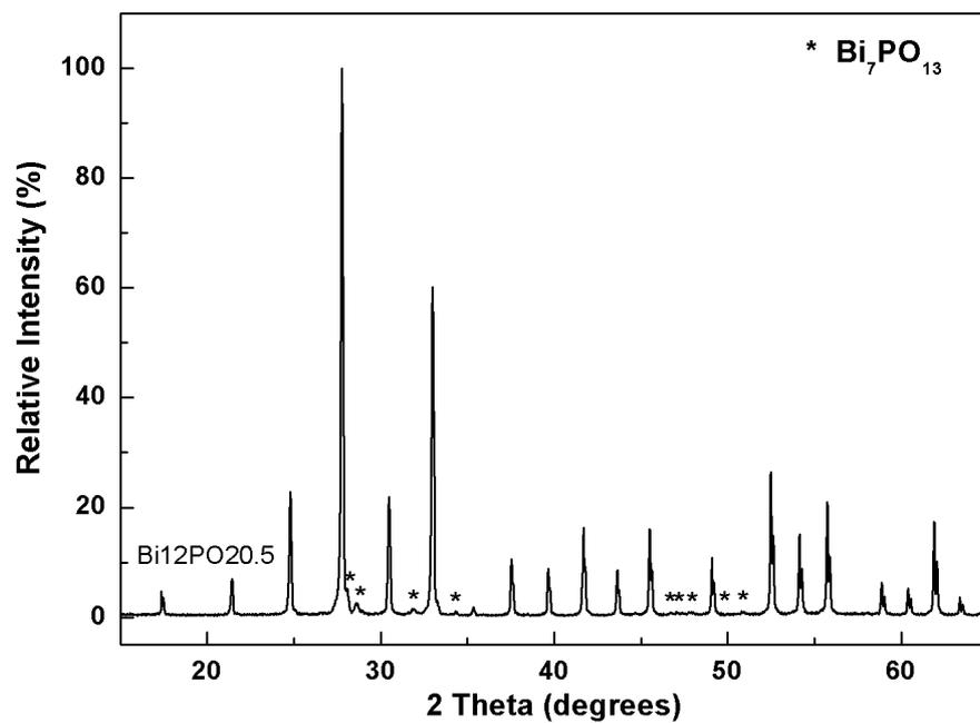
**Figure 9.7** XRPD result of Bi<sub>12</sub>PO<sub>20.5</sub> heated at 800 °C for 72 hours shows a phase mixture of sillenite and impurity phase of Bi<sub>7</sub>PO<sub>13</sub> (ICCD card [49-38], notation \*).
