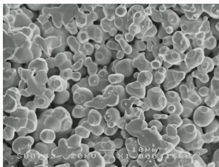
**Figure 4.8** SEM image of  $\text{Bi}_{12}(\text{Bi}_{2/3}\text{Zn}_{1/3})\text{O}_{19.33}$ .
