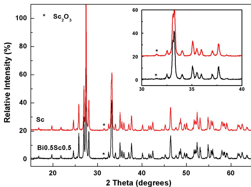
**Figure 9.3** XRPD results of Bi<sub>12</sub>(Bi<sub>0.5</sub>Sc<sub>0.5</sub>)O<sub>19.35</sub> and Bi<sub>12</sub>ScO<sub>19.5</sub> heated at 820 °C for 72 hours. Impurity phases are Sc<sub>2</sub>O<sub>3</sub> (ICCD card [5-629]) labelled as \* and α-Bi<sub>2</sub>O<sub>3</sub> (ICCD card [41-1449]).
