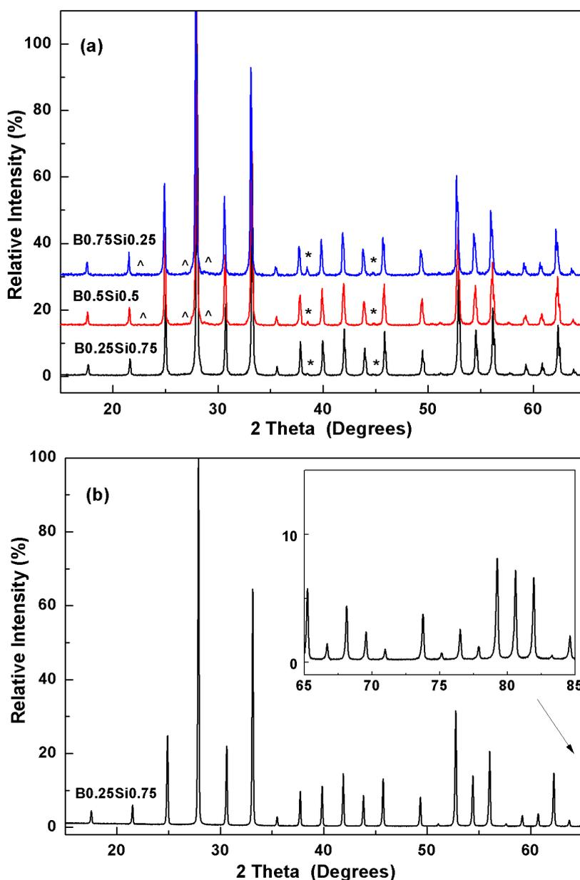
**Figure 5.4** XRPD results of (a)  $Bi_{12}(B_{0.25}Si_{0.75})O_{19.875}$ ,  $Bi_{12}(B_{0.5}Si_{0.5})O_{19.75}$  and  $Bi_{12}(B_{0.75}Si_{0.25})O_{19.625}$  prepared from mixing of two end-members  $Bi_{12}BO_{19.5}$  and  $Bi_{12}SiO_{20}$ .
