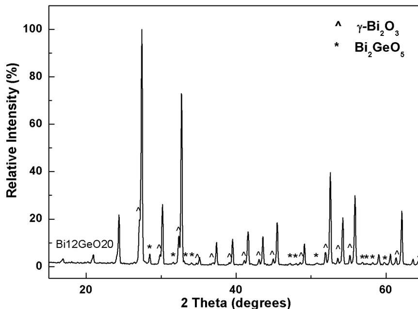
**Figure 9.5** XRPD results of Bi<sub>12</sub>GeO<sub>20</sub> heated at 800 °C for 48 hours. Notations ^ and \* indicate impurity phases of  $\gamma$ -Bi<sub>2</sub>O<sub>3</sub> (ICCD card [45-1344]) and Bi<sub>2</sub>GeO<sub>5</sub> (ICCD card [36-289]), respectively.
