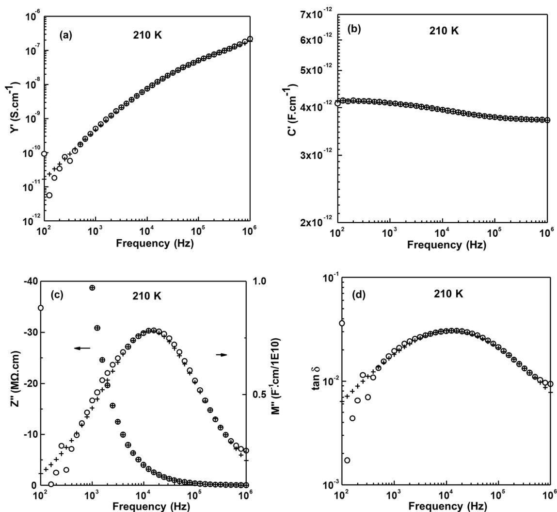
**Figure 9.23** Low temperature IS experimental data points ( $\circ$ ) and the fitting results ( $+$ ) to equivalent circuit shown in Figure 9.10 (b) with (a)  $Y'$ ; (b)  $C'$ , (c)  $-Z''/M''$ , and (d)  $\tan \delta$  spectroscopic plots at 210 K for  $\text{Bi}_{12}(\text{B}_{0.25}\text{Si}_{0.75})\text{O}_{19.875}$ .
