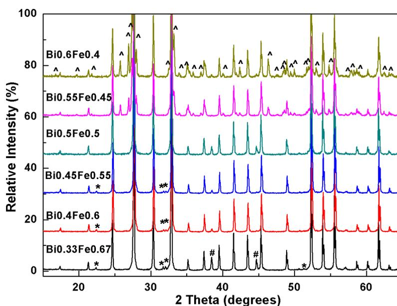
**Figure 4.3** XRPD results of iron sillenites, where  $\text{Bi}_{0.5}\text{Fe}_{0.5}$  is phase-pure. Notation of \*, # and ^ marked as impurity phase  $\text{BiFeO}_3$  (ICCD card [72-2035]); Al metal peaks from sample holder (ICCD card [4-787]) and  $\alpha\text{-Bi}_2\text{O}_3$  phase (ICCD card [41-1449]), respectively.
