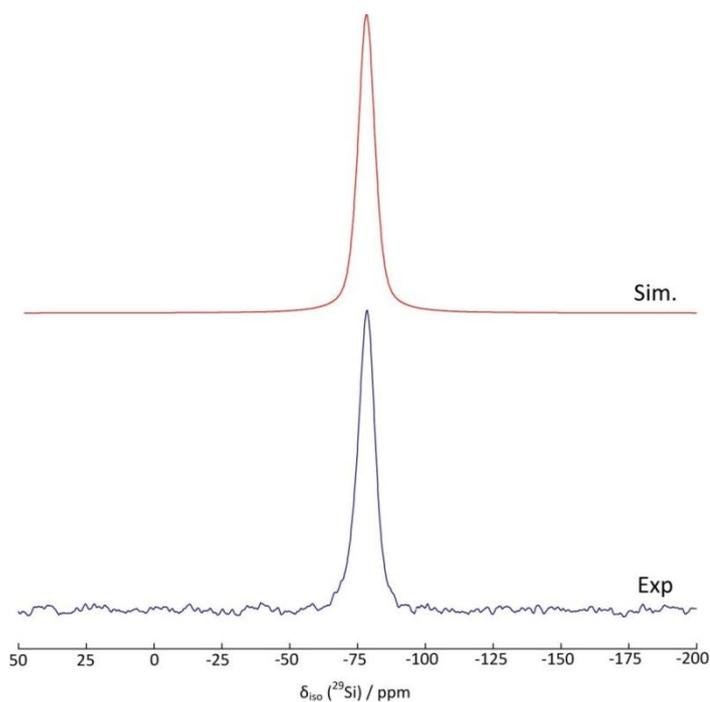
**Figure 3.23** Simulated (red) and Experimental (black) NMR spectra of isotope  $^{29}\text{Si}$  one pulse spectra of  $\text{Bi}_{12}\text{SiO}_{20}$  carried out at 7.05 T (5 kHz MAS).
