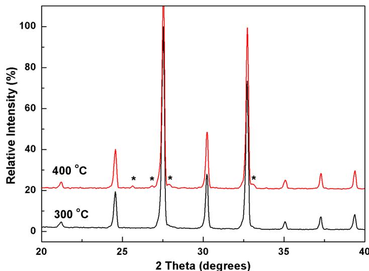
**Figure 4.20** XRPD pattern of  $\text{Bi}_{12}(\text{Bi}_{0.67}\text{Zn}_{0.33})\text{O}_{19.33}$  annealing at 300 and 400 °C for 36 hours, respectively. Notation \* represents  $\alpha\text{-Bi}_2\text{O}_3$  phase.
