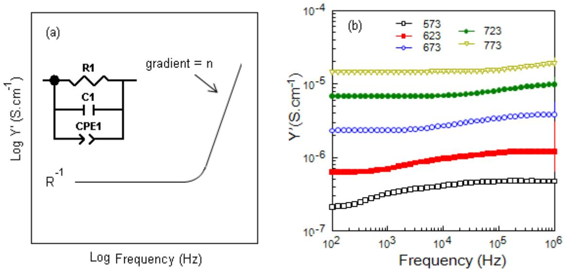
**Figure 3.16** Log  $Y'$  spectroscopic plot (a) for a typical equivalent circuit of parallel  $R_1$ ,  $C_1$  and CPE1 components and (b) log  $Y'$  spectroscopic data for  $\text{Bi}_{12}\text{SiO}_{20}$  between 573 and 773 K.
