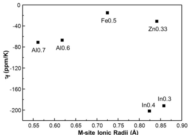
**Figure 4.22**  $\tau_f$  as a function of the M-ions ionic radii of  $\text{M}^{2+}/\text{M}^{3+}$  sillenites. (Note: M-site ionic radii were from Shannon<sup>[8]</sup> with  $\text{Bi}^{3+}_{(\text{VI})} = 0.96 \text{ \AA}$ ,  $\text{Zn}^{2+}_{(\text{VI})} = 0.6 \text{ \AA}$ ,  $\text{Fe}^{3+}_{(\text{VI})} = 0.49 \text{ \AA}$ ,  $\text{Al}^{3+}_{(\text{VI})} = 0.39 \text{ \AA}$  and  $\text{In}^{3+}_{(\text{VI})} = 0.62 \text{ \AA}$ )
