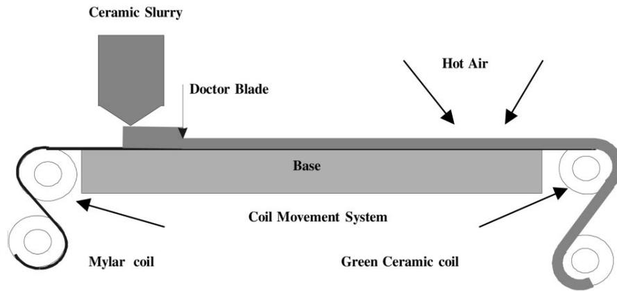
**Figure 1.8**<sup>[56]</sup> A doctor blade set-up for casting LTCC tape.
