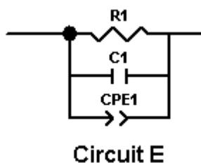
Circuit E is a common equivalent circuit to model the non-ideal Debye response of the bulk component. It is mentioned here as the impedance data of the sample showed only bulk-type electrical behaviour. However, it cannot be used to model the dielectric relaxation behaviour of this sample, as it displayed two capacitance plateaux in  $C'$  spectroscopic plots whereas Circuit E gives rise to a single plateau in such plots.
