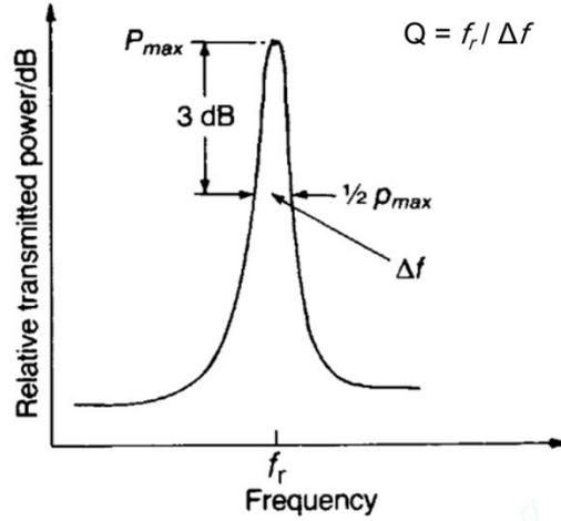
**Figure 1.9**<sup>[55]</sup> Schematic representation of resonant peak showing the definition of Q.f.
