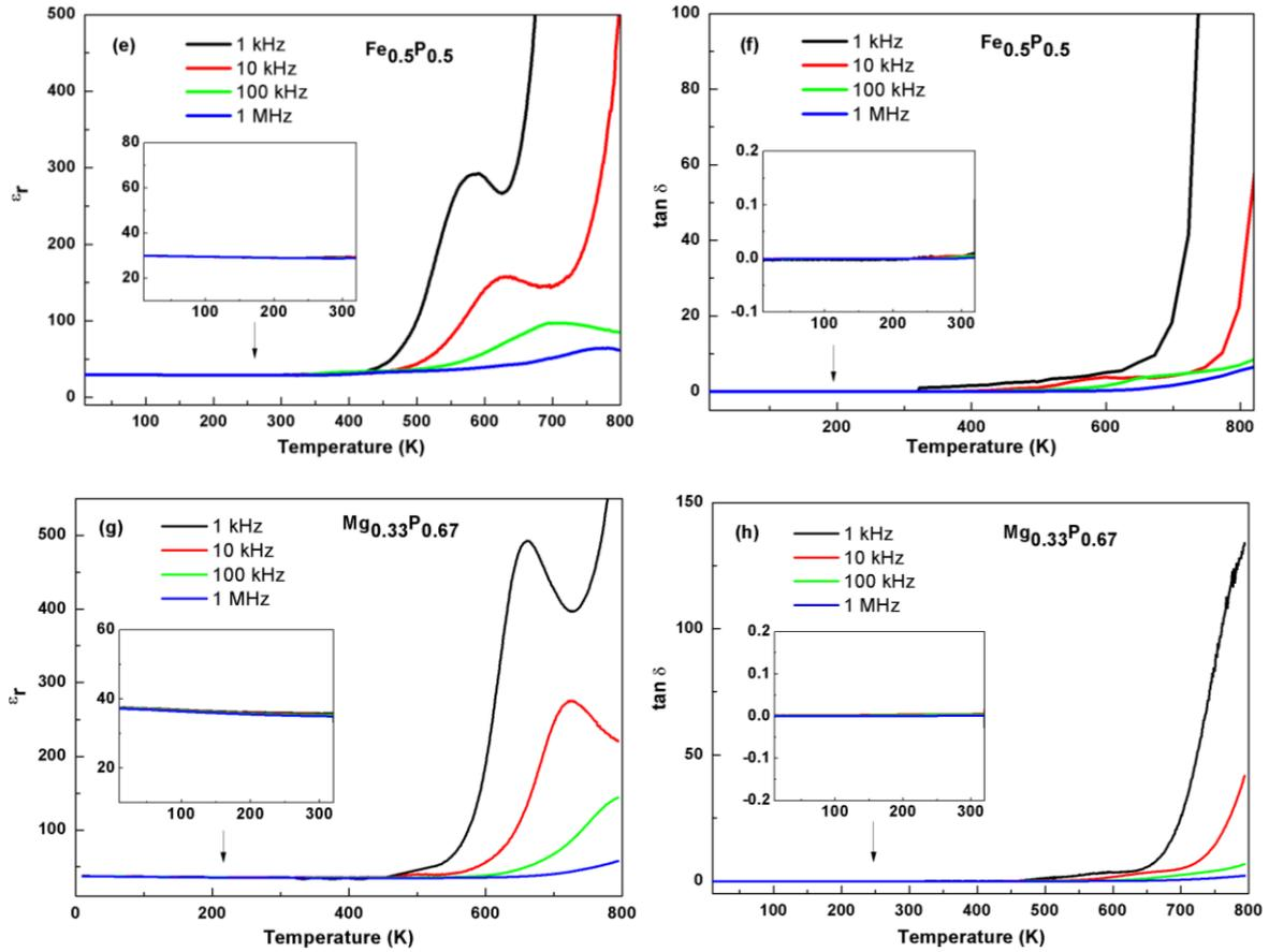
**Figure 6.6** Temperature dependence of permittivity ( $\epsilon_r$ ) and dielectric loss ( $\tan \delta$ ) of (a) and (b)  $\text{Bi}_{12}(\text{Bi}_{0.03}\text{P}_{0.89}\square_{0.08})\text{O}_{20.27}$ ; (c) and (d)  $\text{Bi}_{12}(\text{P}_{0.86}\square_{0.14})\text{O}_{20.15}$ ; (e) and (f)  $\text{Bi}_{12}(\text{Fe}_{0.5}\text{P}_{0.5})\text{O}_{20}$ ; (g) and (h)  $\text{Bi}_{12}(\text{Mg}_{0.33}\text{P}_{0.67})\text{O}_{20}$ , respectively.
