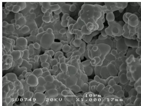
**Figure 4.10** SEM image of  $\text{Bi}_{12}(\text{Bi}_{0.5}\text{Fe}_{0.5})\text{O}_{19.5}$ .
