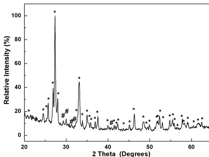
**Figure 4.18** XRPD pattern of  $\text{Bi}_{12}(\text{Bi}_{0.3}\text{Al}_{0.7})\text{O}_{19.5}$  after the DSC measurement. Notations \* and # indicate  $\alpha$ - $\text{Bi}_2\text{O}_3$  (ICCD card [41-1449]) and  $\text{Bi}_2\text{Al}_4\text{O}_9$  (ICCD card [25-1048]), respectively.
