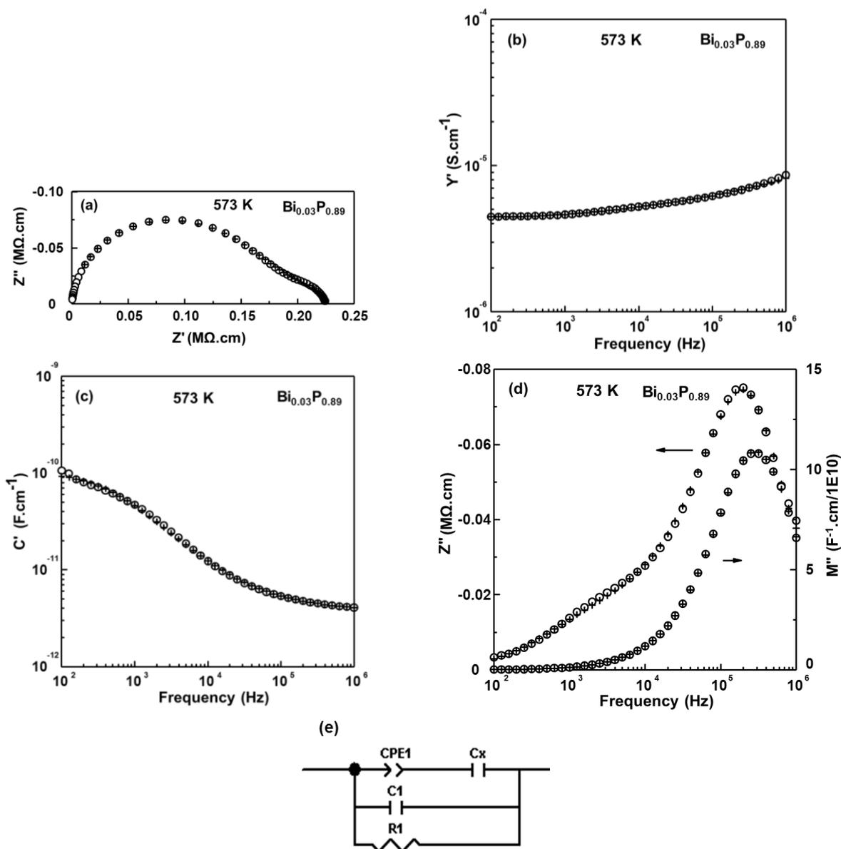
**Figure 6.9** High temperature IS experimental data points (O) and the fitting results (+) to equivalent circuit shown in (e) with (a)  $Z^*$  plot; (b)  $Y'$ , (c)  $C'$ , and (d)  $-Z''/M''$  spectroscopic plots at 573 K for  $Bi_{12}(Bi_{0.03}P_{0.89})O_{20.27}$ .
