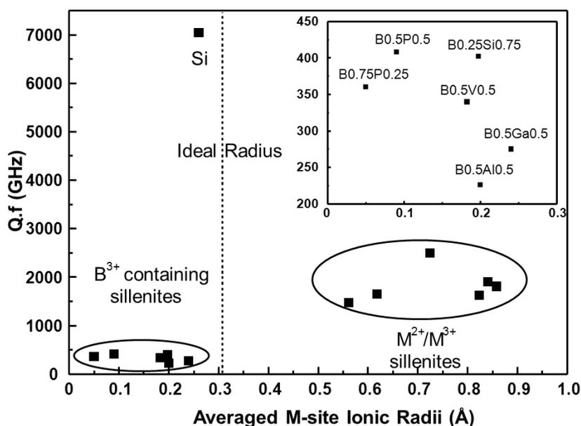
**Figure 5.20**  $Q \cdot f$  values versus the M-site ionic radii of ideal sillenite ( $Bi_{12}SiO_{20}$ ),  $M^{2+}/M^{3+}$  sillenites and  $B^{3+}$  containing sillenites. Inset is an expanded view for all  $B^{3+}$  containing sillenites.
