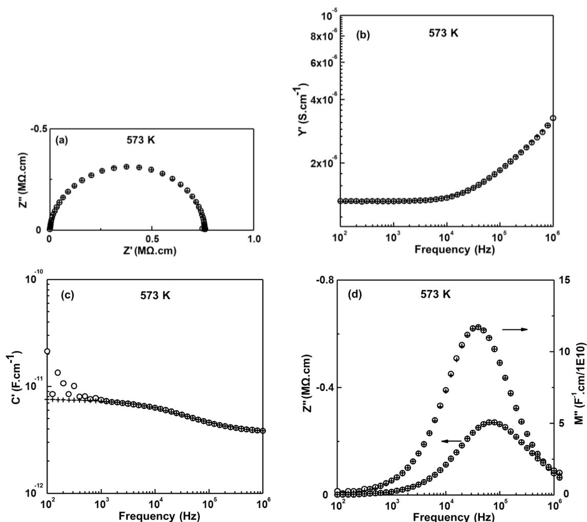
**Figure 9.17** High temperature IS experimental data points (○) and the fitting results (+) to equivalent circuit in Figure 9.10 (a) with (a)  $Z^*$  plot; (b)  $Y'$ , (c)  $C'$ , and (d)  $-Z''/M''$  spectroscopic plots at 573 K for  $\text{Bi}_{12}(\text{Bi}_{0.6}\text{In}_{0.4})\text{O}_{19.5}$ .
