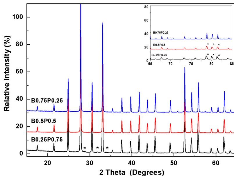
**Figure 5.2** XRPD results of  $Bi_{12}(B_{0.25}P_{0.75})O_{20.25}$ ,  $Bi_{12}(B_{0.5}P_{0.5})O_{20}$  and  $Bi_{12}(B_{0.75}P_{0.25})O_{19.75}$  with  $x = 0.75, 0.50$  and  $0.25$  from the formula  $Bi_{12}(B^{3+}_{1-x}P^{5+}_x)O_{19.5+x}$ , respectively. Inset shows XRPD patterns at higher  $2\theta$  angles  $65-85^\circ$ , where peak splitting was observed. Notations \* and ^ indicate impurity  $Bi_4B_2O_9$  (ICCD card [70-1458]) and unknown sillenite phase, respectively.
