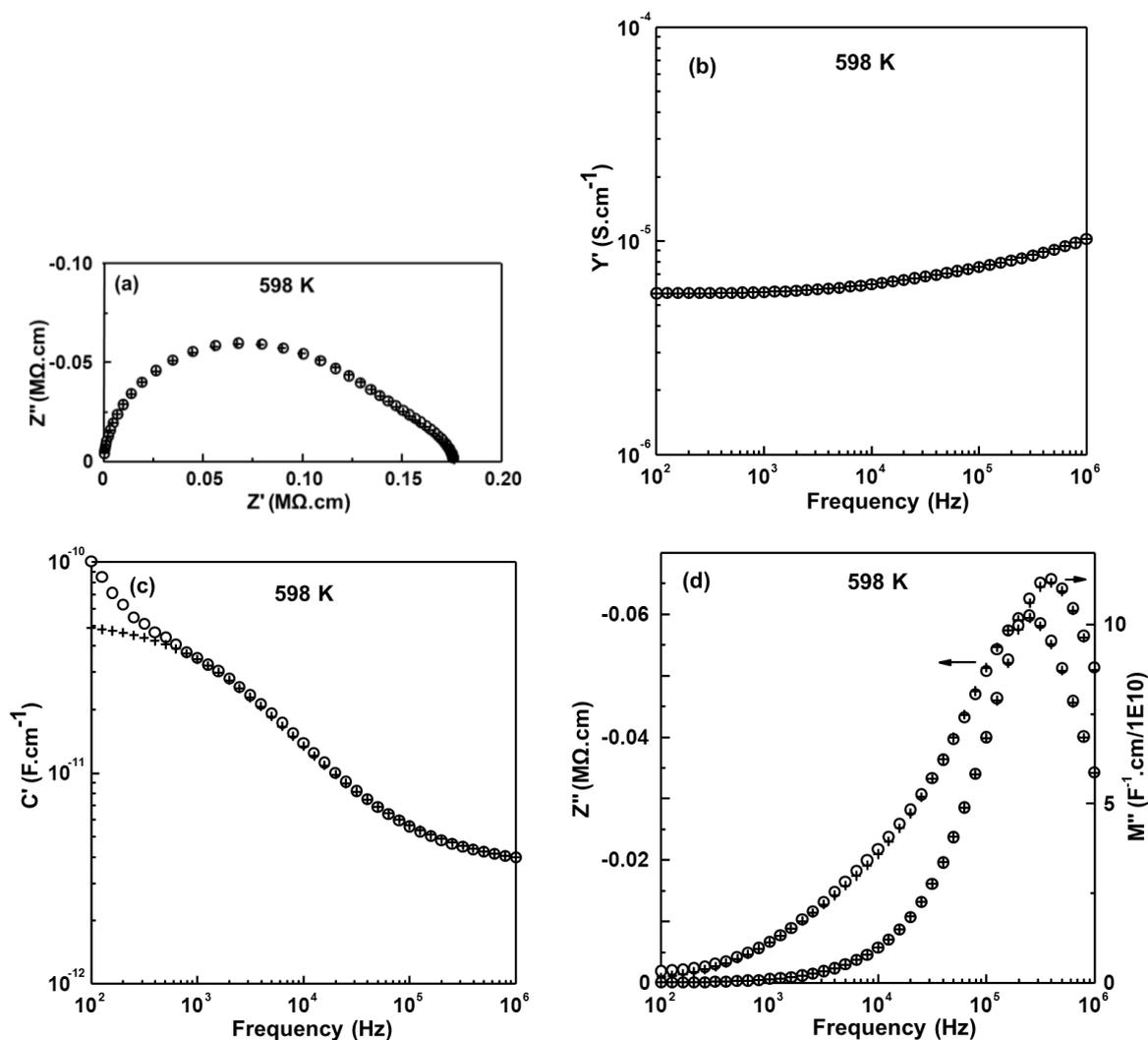
**Figure 9.28** High temperature IS experimental data points ( $\circ$ ) and the fitting results (+) to equivalent circuit shown in Figure 9.10 (a) with (a)  $Z^*$  plot; (b)  $Y'$ , (c)  $C'$ , and (d)  $-Z''/M''$
