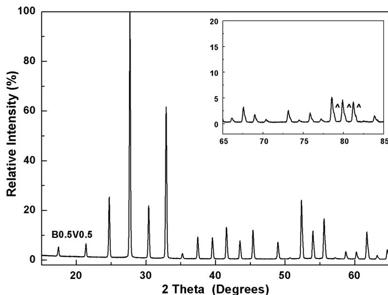
Figure 5.6 XRPD results of  $Bi_{12}(B_{0.5}V_{0.5})O_{20}$ .
