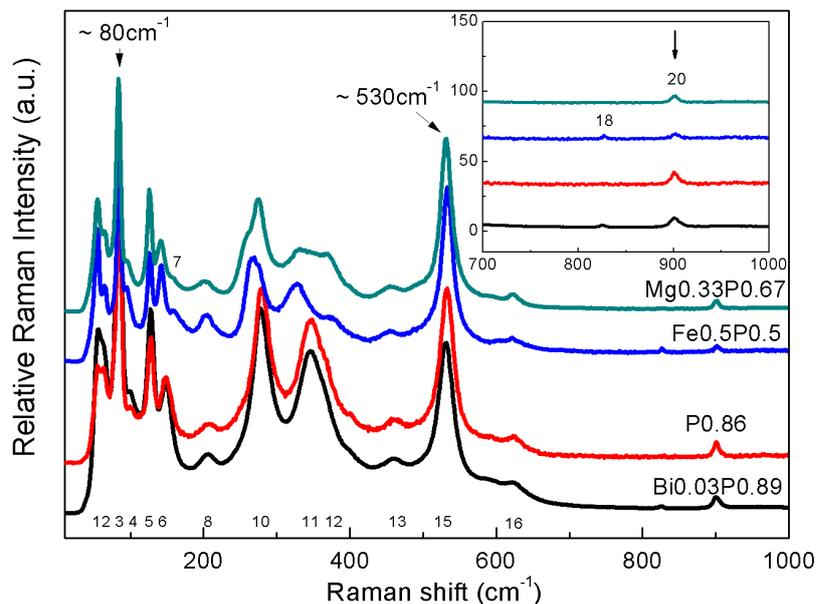
**Figure 6.3** Room temperature Raman Spectra of  $\text{Bi}_{12}(\text{Bi}^{3+}_{0.03}\text{P}^{5+}_{0.89}\square_{0.08})\text{O}_{20.27}$ ,  $\text{Bi}_{12}(\text{P}^{5+}_{0.86}\square_{0.14})\text{O}_{20.15}$ ,  $\text{Bi}_{12}(\text{Fe}^{3+}_{0.5}\text{P}^{5+}_{0.5})\text{O}_{20}$  and  $\text{Bi}_{12}(\text{Mg}^{2+}_{0.33}\text{P}^{5+}_{0.67})\text{O}_{20}$ . Peak intensities are normalized by peak  $\sim 530\text{ cm}^{-1}$ .
