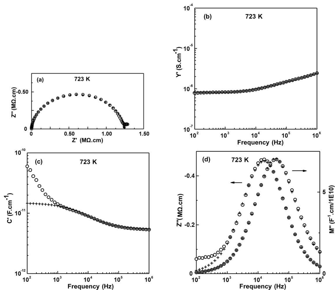
**Figure 9.20** High temperature IS experimental data points (○) and the fitting results (+) to equivalent circuit shown in Figure 9.10 (a) with (a)  $Z^*$  plot; (b)  $Y'$ , (c)  $C'$ , and (d)  $-Z''/M''$  spectroscopic plots at 723 K for  $\text{Bi}_{12}(\text{B}_{0.5}\text{Al}_{0.5})\text{O}_{19.5}$ .
