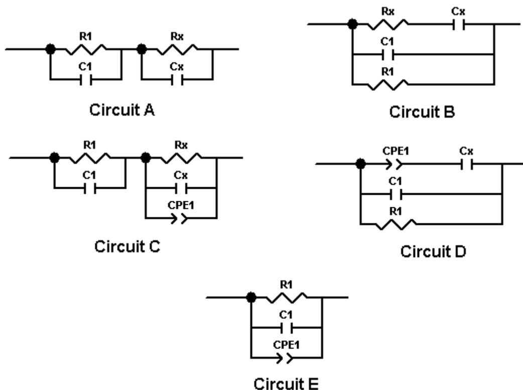
**Figure 3.11** Equivalent circuits A, B, C, D and E to model high temperature IS data for  $\text{Bi}_{12}\text{SiO}_{20}$  ceramic. Circuit D is the correct circuit (see Section 3.2.3.4 for details)
