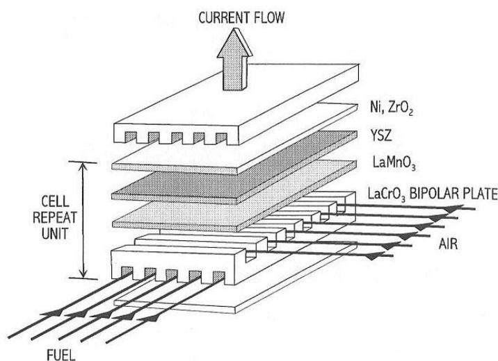
**Figure 1.11** <sup>[70]</sup> Structure of a planar SOFC.
