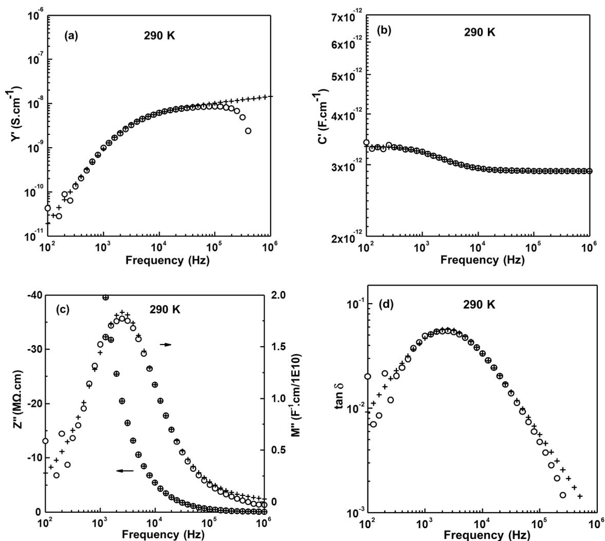
**Figure 9.29** Low temperature IS experimental data points ( $\circ$ ) and the fitting results ( $+$ ) to equivalent circuit shown in Figure 9.10 (b) with (a)  $Y'$ ; (b)  $C'$ , (c)  $-Z''/M''$ , and (d)  $\tan \delta$
