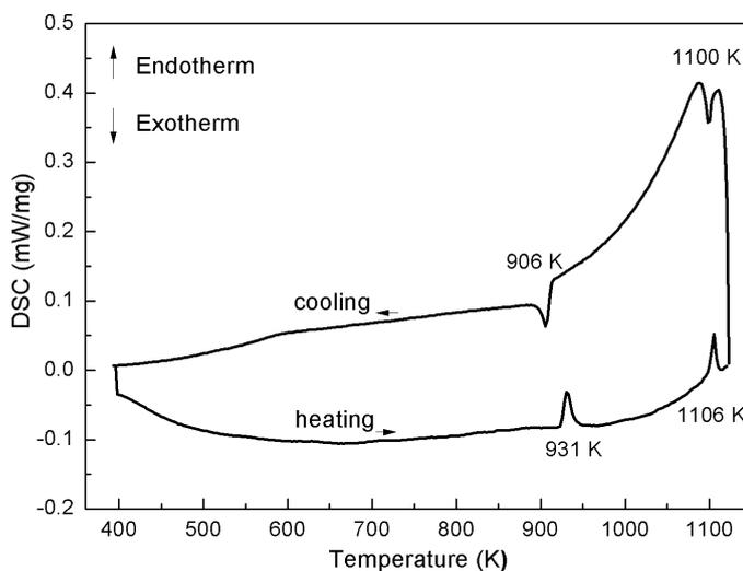
**Figure 3.4** DSC trace of  $\text{Bi}_{12}\text{SiO}_{20}$  powder.
