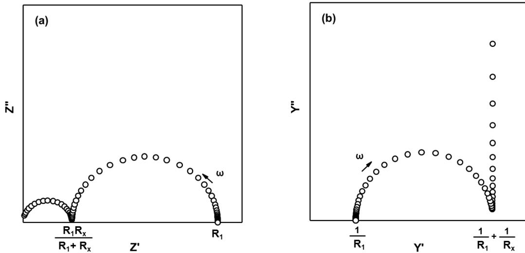
**Figure 9.9** Simulated (a) complex impedance  $Z^*$  plot and (b) complex admittance  $Y^*$  plot for the Cole-Cole branch in parallel with R and C elements.
