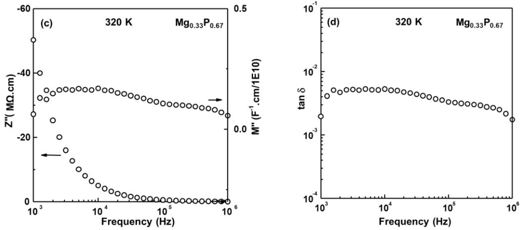
**Figure 6.7** (a)  $C'$ ; (b)  $Y'$ ; (c)  $-Z''/M''$  and (d)  $\tan \delta$  spectroscopic plots for  $\text{Bi}_{12}(\text{Mg}_{0.33}\text{P}_{0.67})\text{O}_{20}$  at 320 K to show that no low temperature relaxation behaviour was present.
