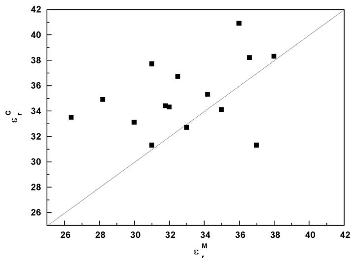
**Figure 7.3** The measured permittivity,  $\epsilon_r^M$  versus the calculated permittivity,  $\epsilon_r^C$  for sillenites listed in Table 7.4.
