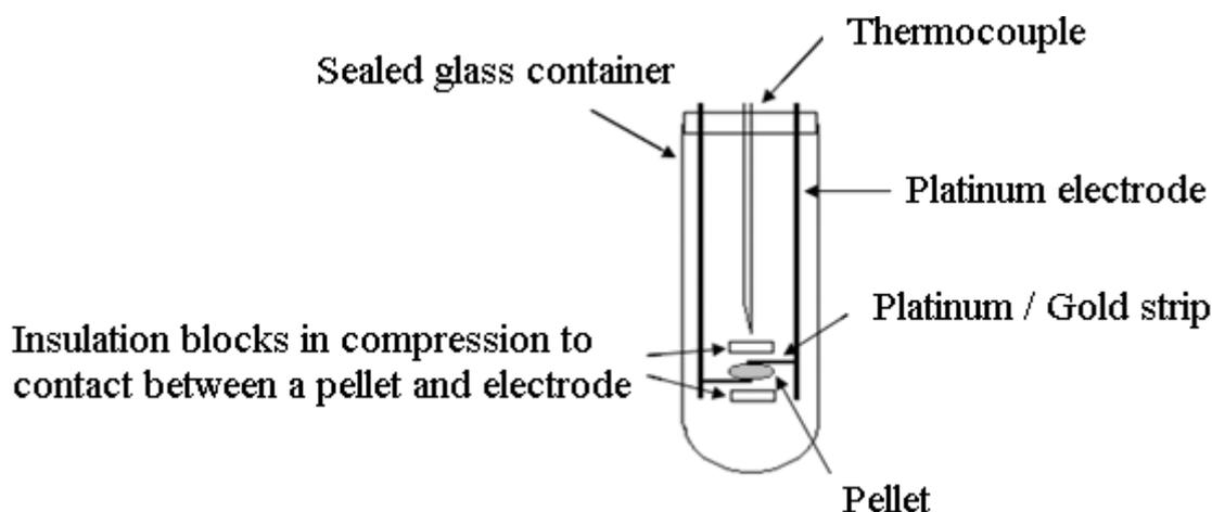
**Figure 2.8** Schematic diagram of high temperature IS equipment setup, where pellet connected with platinum electrodes in a compression jig.
