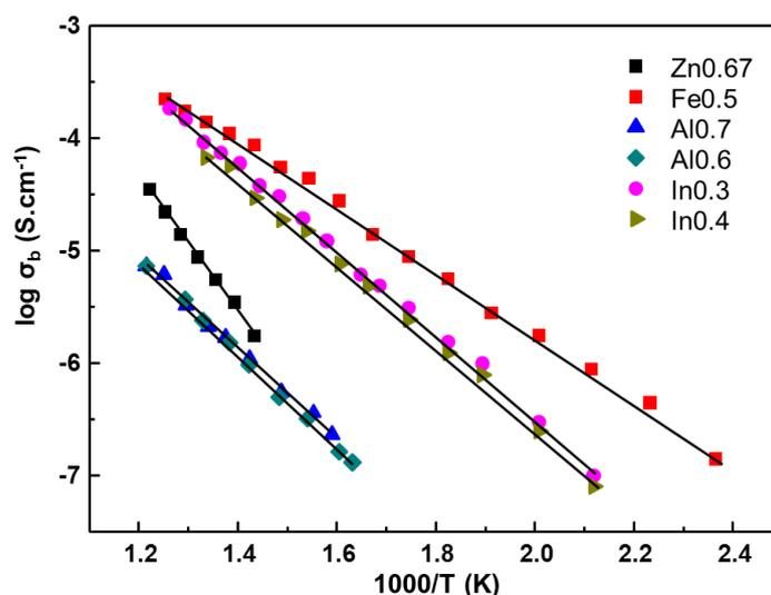
**Figure 4.33** Arrhenius plot of bulk conductivity versus reciprocal temperature for all  $M^{2+}/M^{3+}$  sillenites.
