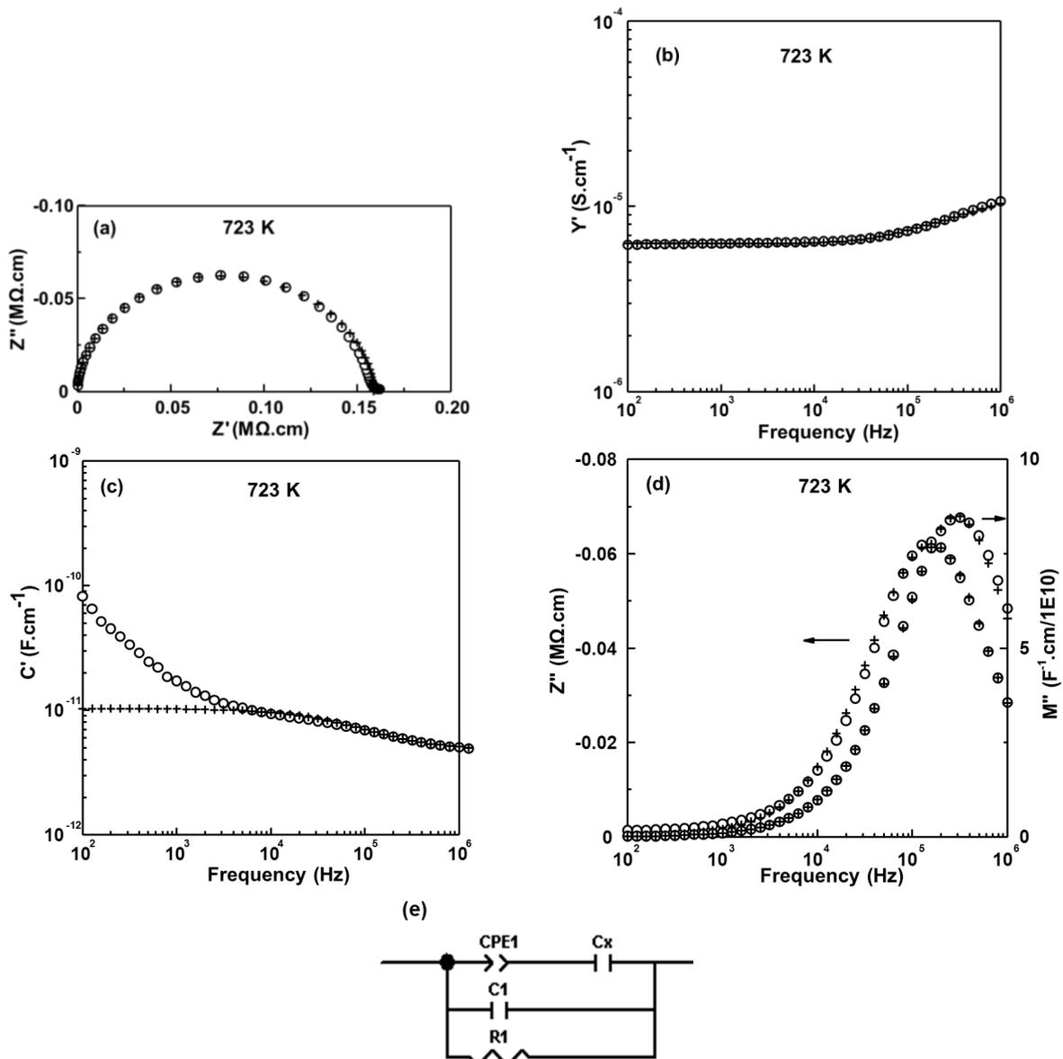
**Figure 5.13** High temperature IS experimental data points (○) and the fitting results (+) to equivalent circuit shown in (e) with (a)  $Z^*$  plot; (b)  $Y'$ , (c)  $C'$ , and (d)  $-Z''/M''$  spectroscopic plots at 723 K for Bi<sub>12</sub>(B<sub>0.75</sub>P<sub>0.25</sub>)O<sub>19.75</sub>.
