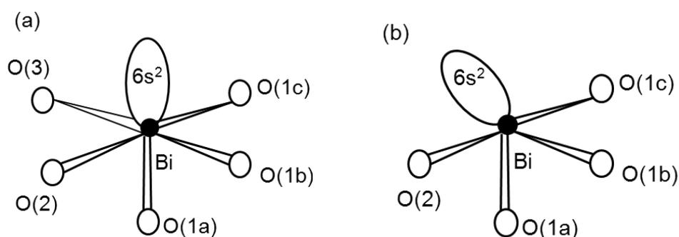
**Figure 1.5** [25] The structure of (a) a distorted octahedron - BiO<sub>5</sub>LP in the ideal sillenite structure and (b) a distorted trigonal bipyramid - BiO<sub>4</sub>LP in a distorted sillenite structure with partial O(3) atoms missing (e.g. Bi<sub>12</sub>(Bi<sub>0.5</sub>Fe<sub>0.5</sub>)O<sub>19.5</sub>).
