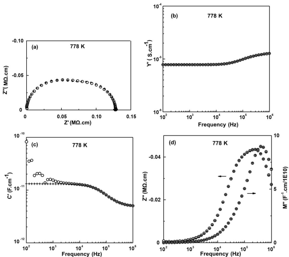
**Figure 9.11** High temperature IS experimental data points (○) and the fitting results (+) to equivalent circuit in Figure 9.10 (a) with (a)  $Z^*$  plot; (b)  $Y'$ , (c)  $C'$ , and (d)  $-Z''/M''$  spectroscopic plots at 778 K for  $\text{Bi}_{12}(\text{Bi}_{0.67}\text{Zn}_{0.33})\text{O}_{19.33}$ .
