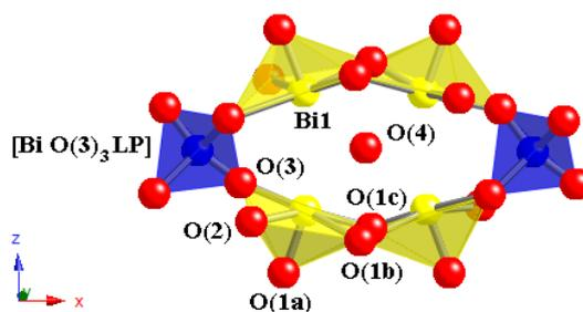
**Figure 4.1**<sup>[3]</sup> Fragment of distorted sillenite structure viewed along the (001) plane with  $\text{Bi}^{3+}$  cations occupying the tetrahedral site; blue, red and yellow spheres represent the  $\text{M}^{n+}$ , oxygen and bismuth ions, respectively.
