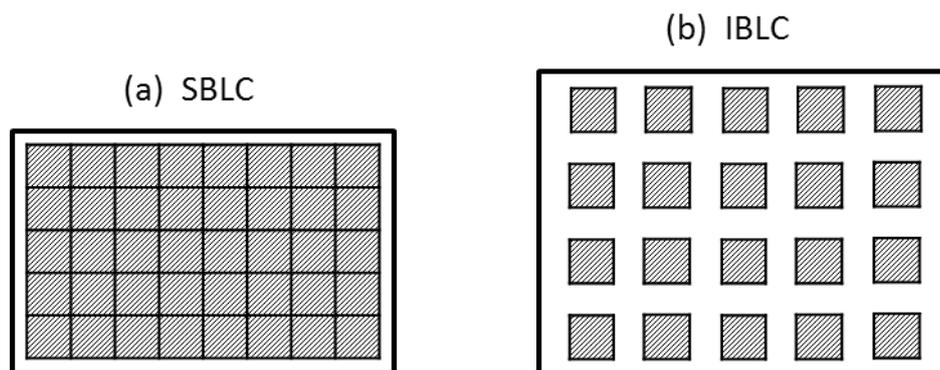
**Figure 1.20** Cross-section of (a) SBLC and (b) IBLC ceramic.
