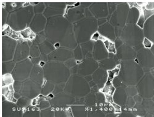
**Figure 3.5** SEM image of  $\text{Bi}_{12}\text{SiO}_{20}$  ceramic.
