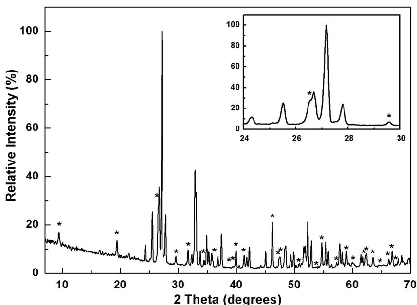
**Figure 9.1** XRPD results of  $\text{Bi}_{12}\text{LiO}_{18.5}$  heated at 725 °C for 72 hours. Impurity phases are
