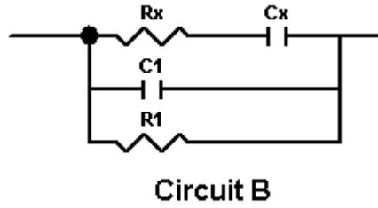
Circuit B is a typical equivalent circuit to model dielectric relaxation behaviour in materials. The series combination of  $R_x$  and  $C_x$  is known as a Cole-Cole branch which is used to describe interactions e.g. dipole-dipole, or lattice relaxations in the structure.<sup>[29]</sup>  $R_1$  represents the long-range dc conduction and  $C_1$  represents the bulk capacitance.
