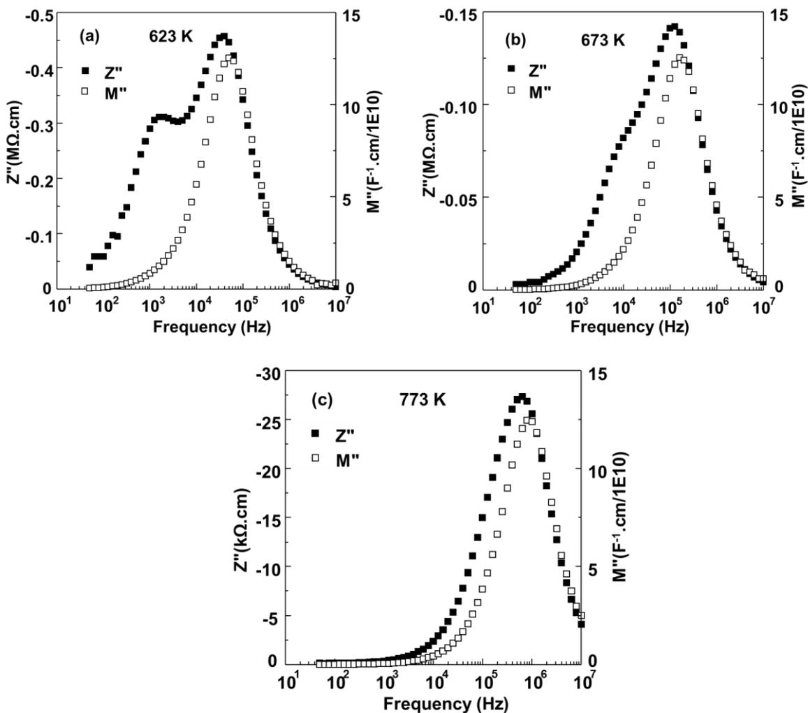
**Figure 3.10** Combined of  $-Z''$  and  $M''$  spectroscopic plots of  $\text{Bi}_{12}\text{SiO}_{20}$  at (a) 623 and (b) 673 and (c) 773 K.
