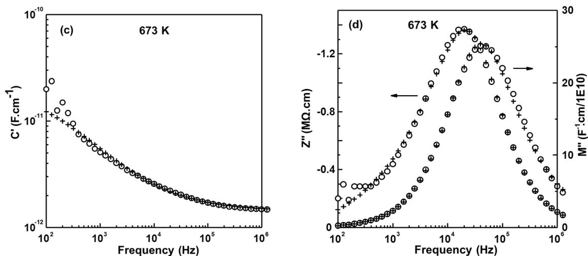
**Figure 9.15** High temperature IS experimental data points ( $\circ$ ) and the fitting results ( $+$ ) to equivalent circuit in Figure 9.10 (a) with (a)  $Z^*$  plot; (b)  $Y'$ , (c)  $C'$ , and (d)  $-Z''/M''$  spectroscopic plots at 673 K for  $\text{Bi}_{12}(\text{Bi}_{0.4}\text{Al}_{0.6})\text{O}_{19.5}$ .
