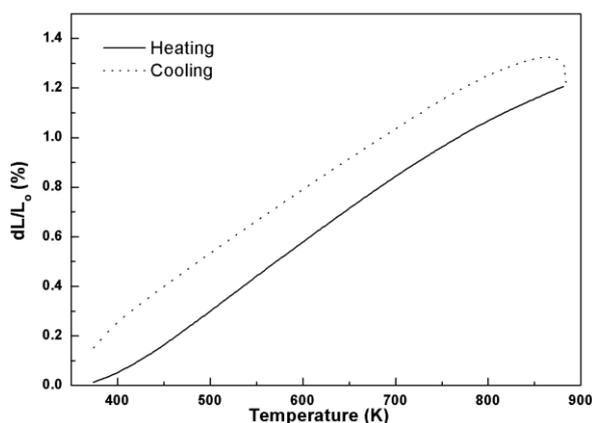
**Figure 3.22** DIL trace of  $\text{Bi}_{12}\text{SiO}_{20}$  pellet from 373 to 883 K.
