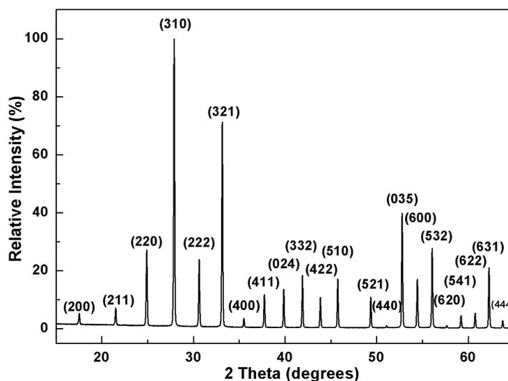
**Figure 3.3** XRPD results of single-phase sillenite  $\text{Bi}_{12}\text{SiO}_{20}$  after sintering at 850 °C for 48 hours indexed with ICDD card [80-627] after Horowitz *et al.* [3].
