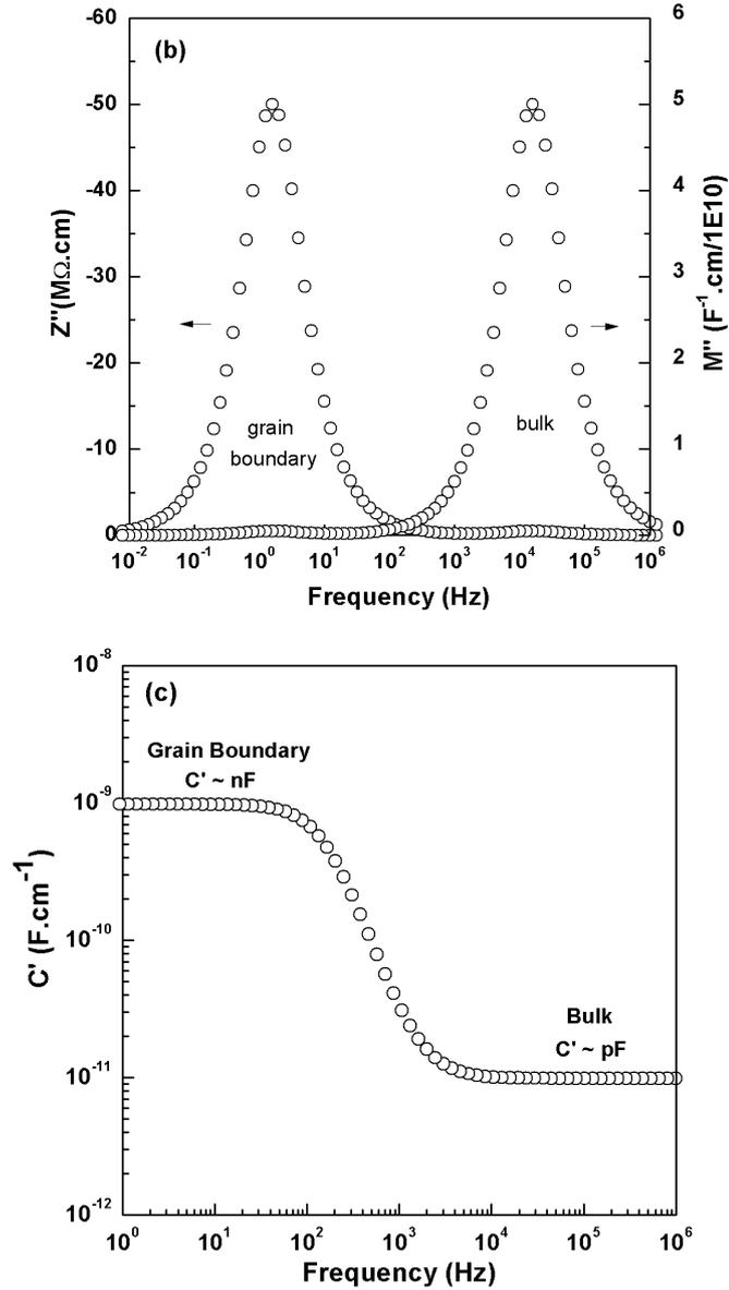
**Figure 2.7** (a) complex impedance plane  $Z^*$  plot (b) combined  $Z''$  and  $M''$  spectroscopic plot (c) real capacitance  $C'$  spectroscopic plot of stimulated IS data for Brick Layer Model.
