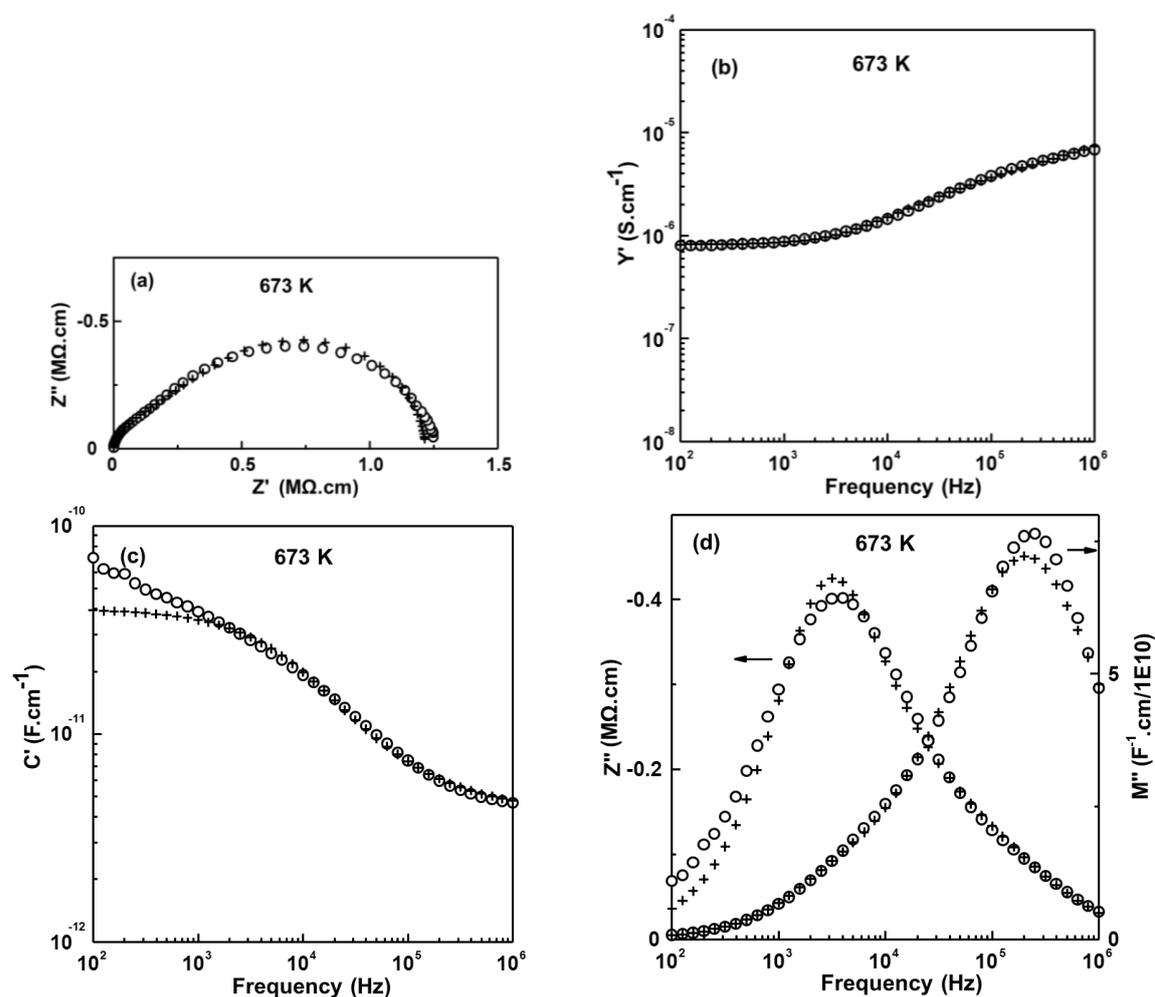
**Figure 9.24** High temperature IS data points (○) and the fitting results (+) to equivalent circuit shown in Figure 9.10 (a) with (a)  $Z^*$  plot; (b)  $Y'$ , (c)  $C'$ , and (d)  $-Z''/M''$  spectroscopic plots at 673 K for  $\text{Bi}_{12}(\text{B}_{0.5}\text{P}_{0.5})\text{O}_{19.5}$ .
