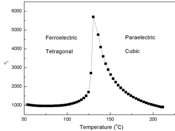
**Figure 1.13**<sup>[55]</sup> Temperature dependence of  $\epsilon_r$  showing the Ferroelectric-Paraelectric phase transition of undoped  $\text{BaTiO}_3$  ceramic.
