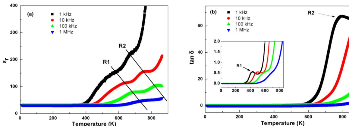
**Figure 4.28** Temperature dependence of (a) permittivity and (b) dielectric losses of  $\text{Bi}_{0.5}\text{Fe}_{0.5}$ . R1 and R2 indicate two relaxation events. Insets are an expanded view of the y-axis data to show R1.
