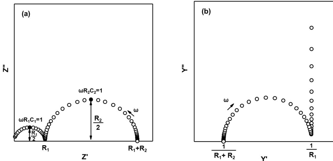
**Figure 9.8** Simulated (a) complex impedance  $Z^*$  plot and (b) complex admittance  $Y^*$  plot for two parallel RC elements in series.
