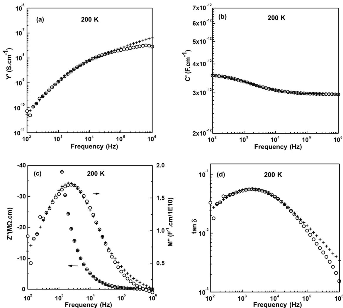
**Figure 9.27** Low temperature IS experimental data points ( $\circ$ ) and the fitting results ( $+$ ) to equivalent circuit shown in Figure 9.10 (b) with (a)  $Y'$ ; (b)  $C'$ , (c)  $-Z''/M''$ , and (d)  $\tan \delta$  spectroscopic plots at 200 K for  $\text{Bi}_{12}(\text{B}_{0.5}\text{V}_{0.5})\text{O}_{19.5}$ .
