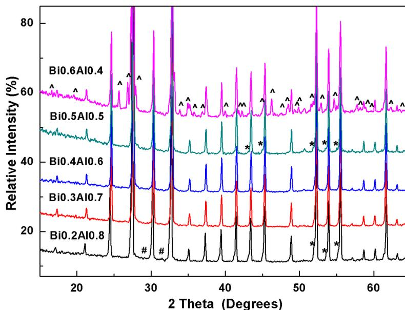
**Figure 4.4** XRPD results of aluminium sillenites, where a narrow solid solution range between  $\text{Bi}_{0.4}\text{Al}_{0.6}$  and  $\text{Bi}_{0.3}\text{Al}_{0.7}$  was obtained. Notations \*, # and ^ indicate  $\gamma\text{-Bi}_2\text{O}_3$  (ICCD card [45-1344]),  $\text{Bi}_2\text{Al}_4\text{O}_9$  (JCPDS card [25-1048]) and  $\alpha\text{-Bi}_2\text{O}_3$ , respectively.
