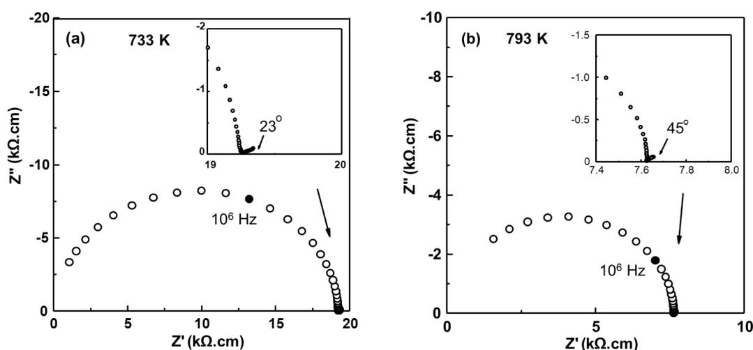
Figure 4.32  $Z^*$  plot of  $\text{Bi}_{0.7}\text{In}_{0.3}$  at (a) 733 and (b) 793 K.
