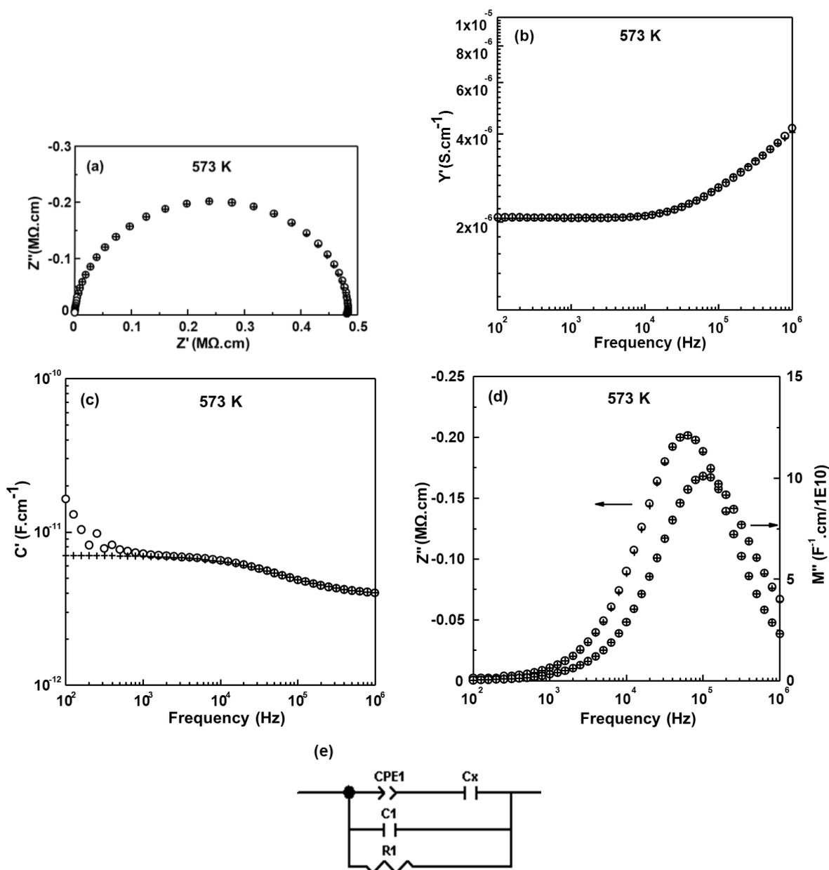
**Figure 4.30** Impedance spectroscopy data of the IS experimental data points and the fitting results to equivalent circuit shown in (e) with (a)  $Z^*$  plot; (b)  $Y'$ , (c)  $C'$ , and (d)  $-Z''/M''$  spectroscopic plots at 573 K for  $\text{Bi}_{12}(\text{Bi}_{0.7}\text{In}_{0.3})\text{O}_{19.5}$ .
