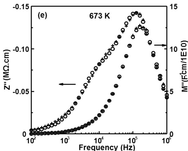
**Figure 3.14** (a) Impedance  $Z^*$  plot and spectroscopic plots of (b)  $C'$ , (c)  $Y'$ , (d)  $\tan \delta$  and (e)  $-Z''$  and  $M''$  of  $\text{Bi}_{12}\text{SiO}_{20}$  measured at 673 K (open symbols) and the best-fit results (cross symbols) for Circuit D.
