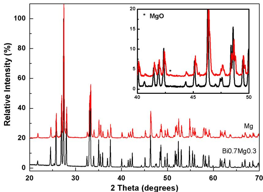
**Figure 9.2** XRPD results of  $\text{Bi}_{12}(\text{Bi}_{0.7}\text{Mg}_{0.3})\text{O}_{19.35}$  and  $\text{Bi}_{12}\text{MgO}_{19}$  heated at 800 °C for 72 hours. Notion \* in the inset indicates the strongest peak of MgO (ICCD card [78-430]) in  $\text{Bi}_{12}\text{MgO}_{19}$ .
