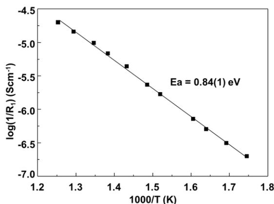
**Figure 3.17** Arrhenius plot of bulk conductivity for  $\text{Bi}_{12}\text{SiO}_{20}$ .
