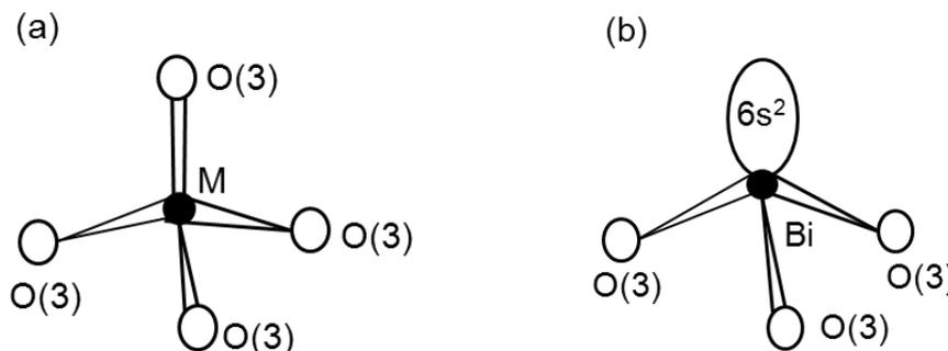
**Figure 1.6** The structure of (a) a regular tetrahedron –  $\text{MO}_4$  and (b) an ‘umbrella-like’ distorted tetrahedron –  $\text{BiO}_3\text{LP}$  in a distorted sillenite structure with partial O(3) atoms missing (e.g.  $\text{Bi}_{12}\text{Bi}_{0.5}\text{Fe}_{0.5}\text{O}_{19.5}$ ).
