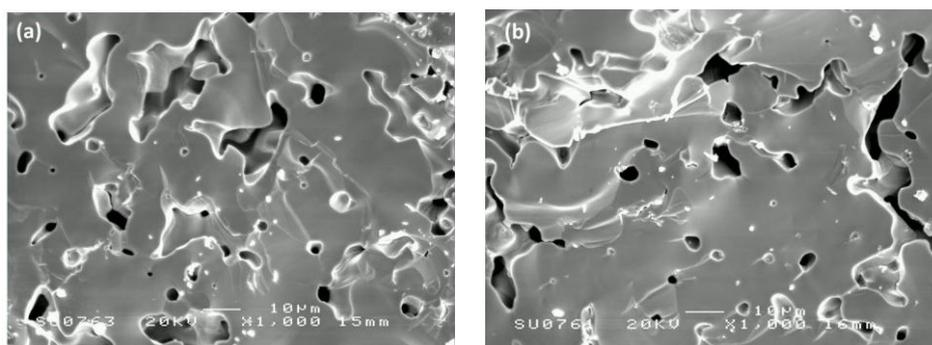
**Figure 4.13** SEM image of (a)  $\text{Bi}_{0.7}\text{In}_{0.3}$  and (b)  $\text{Bi}_{0.6}\text{In}_{0.4}$ .
