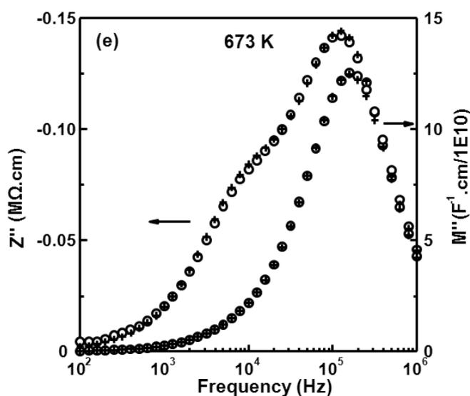
**Figure 3.15** (a) Impedance  $Z^*$  plot and spectroscopic plots of (b)  $C'$ , (c)  $Y'$ , (d)  $\tan \delta$  and (e)  $-Z''$  and  $M''$  of  $\text{Bi}_{12}\text{SiO}_{20}$  measured at 673 K (open symbols) and the best-fit results (cross symbols) for Circuit D.
