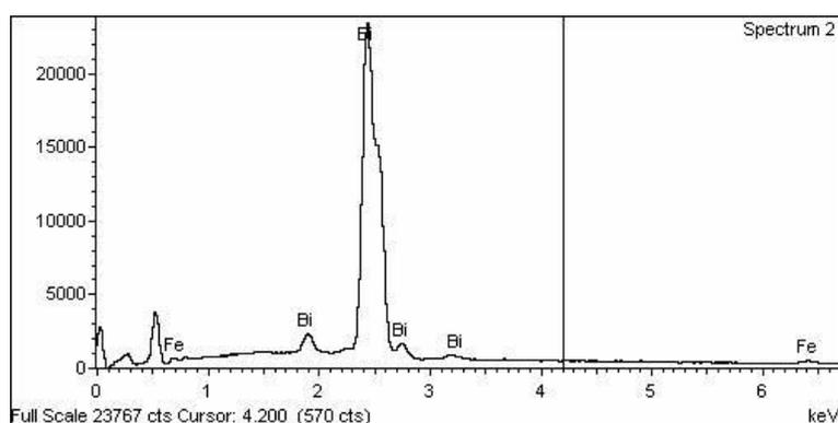
**Figure 4.11** EDS spectrum of  $\text{Bi}_{12}(\text{Bi}_{0.5}\text{Fe}_{0.5})\text{O}_{19.5}$ .
