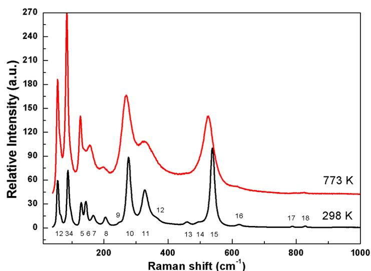
**Figure 3.19** Raman Spectra from the same grain of a  $\text{Bi}_{12}\text{SiO}_{20}$  pellet at 298 and 773 K. Peak
