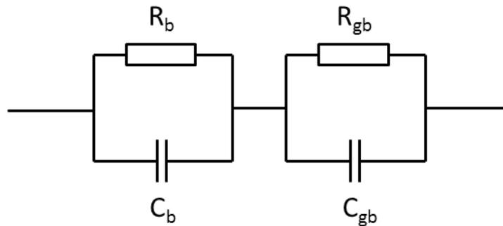
**Figure 2.6** An equivalent circuit consisting of two parallel RC elements in series.
