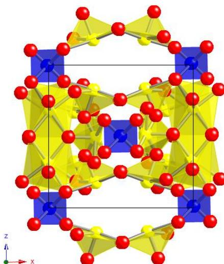
**Figure 3.1**<sup>[1]</sup> The structure of an ideal  $\text{Bi}_{12}\text{M}^{4+}\text{O}_{20}$  sillenite viewed along the (001) plane, where yellow, blue and red spheres represent  $\text{Bi}^{3+}$ ,  $\text{M}^{4+}$  and  $\text{O}^{2-}$  ions, respectively; black lines indicate the body-centred cubic unit cell of the structure.
