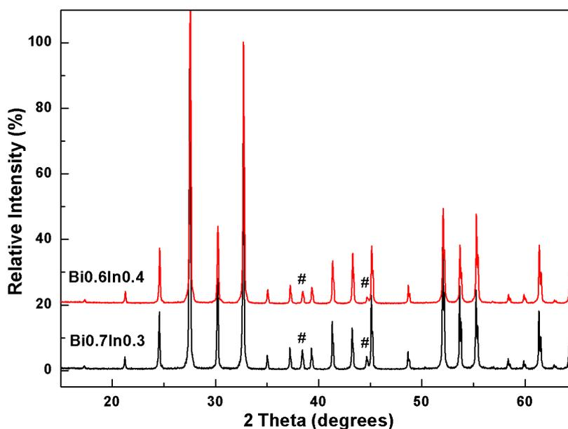
**Figure 4.6** XRPD of single-phase  $\text{Bi}_{12}(\text{Bi}_{0.6}\text{In}_{0.4})\text{O}_{19.5}$  and  $\text{Bi}_{12}(\text{Bi}_{0.7}\text{In}_{0.3})\text{O}_{19.5}$ . All peaks caused by the sample holders are marked as #.
