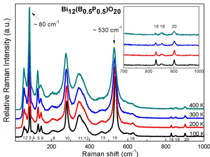
**Figure 5.11** Raman spectra of Bi<sub>12</sub>(B<sub>0.5</sub>P<sub>0.5</sub>)O<sub>20</sub> at 100, 200, 300 and 400 K.
