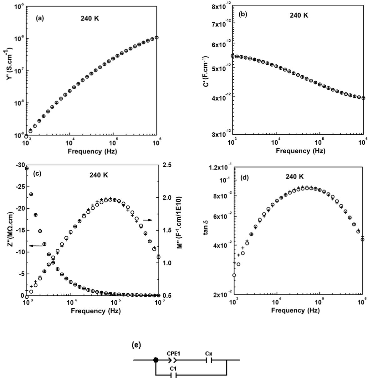
**Figure 5.16** Low temperature IS experimental data points (O) and the fitting results (+) to equivalent circuit shown in (e) with (a)  $Y'$ ; (b)  $C'$ , (c)  $-Z''/M''$ , and (d)  $\tan \delta$  spectroscopic plots at 240 K for  $Bi_{12}(B_{0.75}P_{0.25})O_{19.75}$ .
