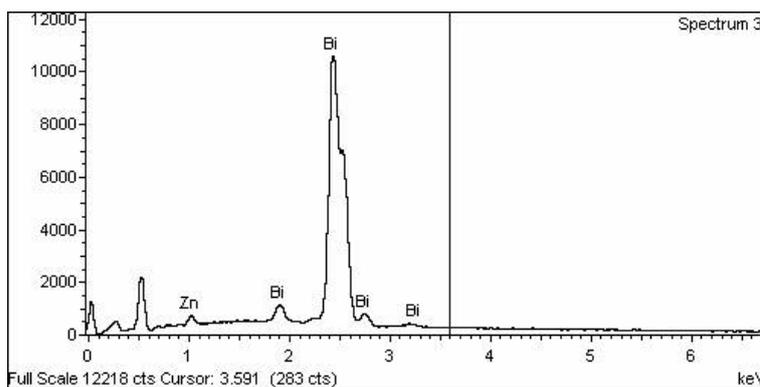
**Figure 4.9** EDS spectrum of  $\text{Bi}_{12}(\text{Bi}_{2/3}\text{Zn}_{1/3})\text{O}_{19.33}$ .
