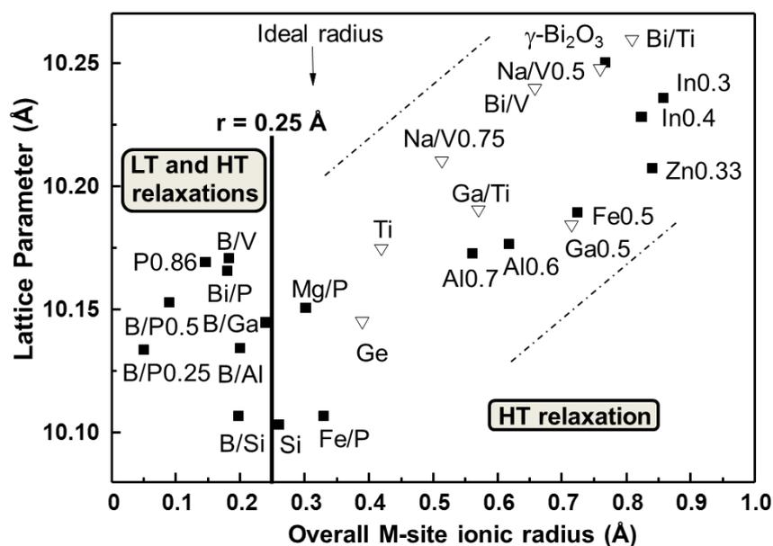
**Figure 7.1** The relationship between lattice parameter and the overall M-site ionic radius of single-phase sillenites from this work (shown as filled squares). Data for  $\gamma\text{-Bi}_2\text{O}_3$ <sup>[6]</sup> and from preliminary work by Hutton<sup>[5]</sup> (shown as open triangles) are also included for comparison. Dashed lines indicate a linear region between the overall M-cation ionic radius and the unit cell parameter of sillenites.
