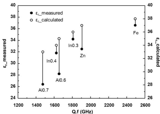
**Figure 4.25** Correlation between Q.f and measured  $\epsilon_r$  (○) / CM calculated  $\epsilon_r$  (●) for  $M^{2+}/M^{3+}$  sillenites.
