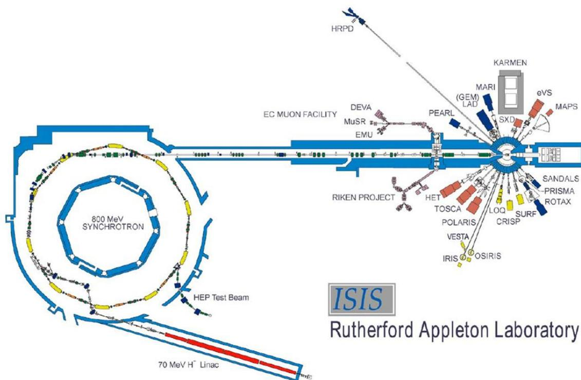
Figure 2.4<sup>[4]</sup> The instrument layout at ISIS.
