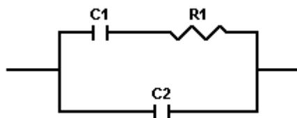
**Figure 1.16** A common equivalent circuit to model dielectric relaxation, where the series
