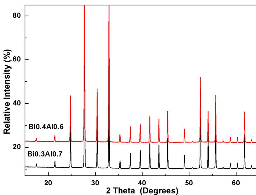
**Figure 4.5** XRPD results of single-phase compounds  $\text{Bi}_{0.3}\text{Al}_{0.7}$  and  $\text{Bi}_{0.4}\text{Al}_{0.6}$ .
