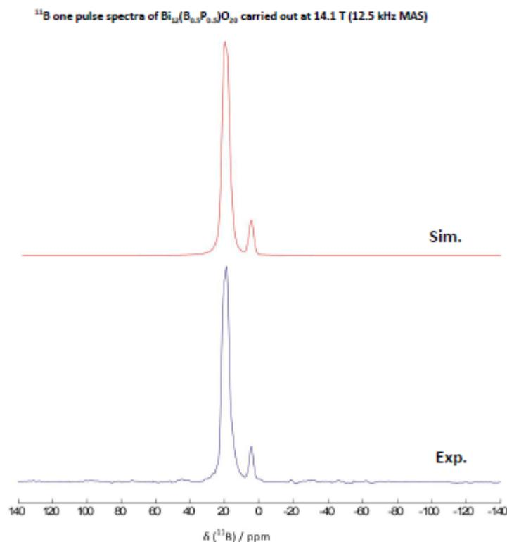
**Figure 5.9** Simulated (red) and Experimental (black) NMR spectra of isotope  $^{11}\text{B}$  one pulse spectra of  $\text{Bi}_{12}(\text{B}_{0.5}\text{P}_{0.5})\text{O}_{20}$  at magnetic field of 14.1 T (12.5 kHz MAS).
