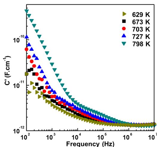
**Figure 9.14**  $C'$  spectroscopic plot showing the capacitance fluctuation at various temperatures for  $\text{Bi}_{12}(\text{Bi}_{0.3}\text{Al}_{0.7})\text{O}_{19.5}$ .
