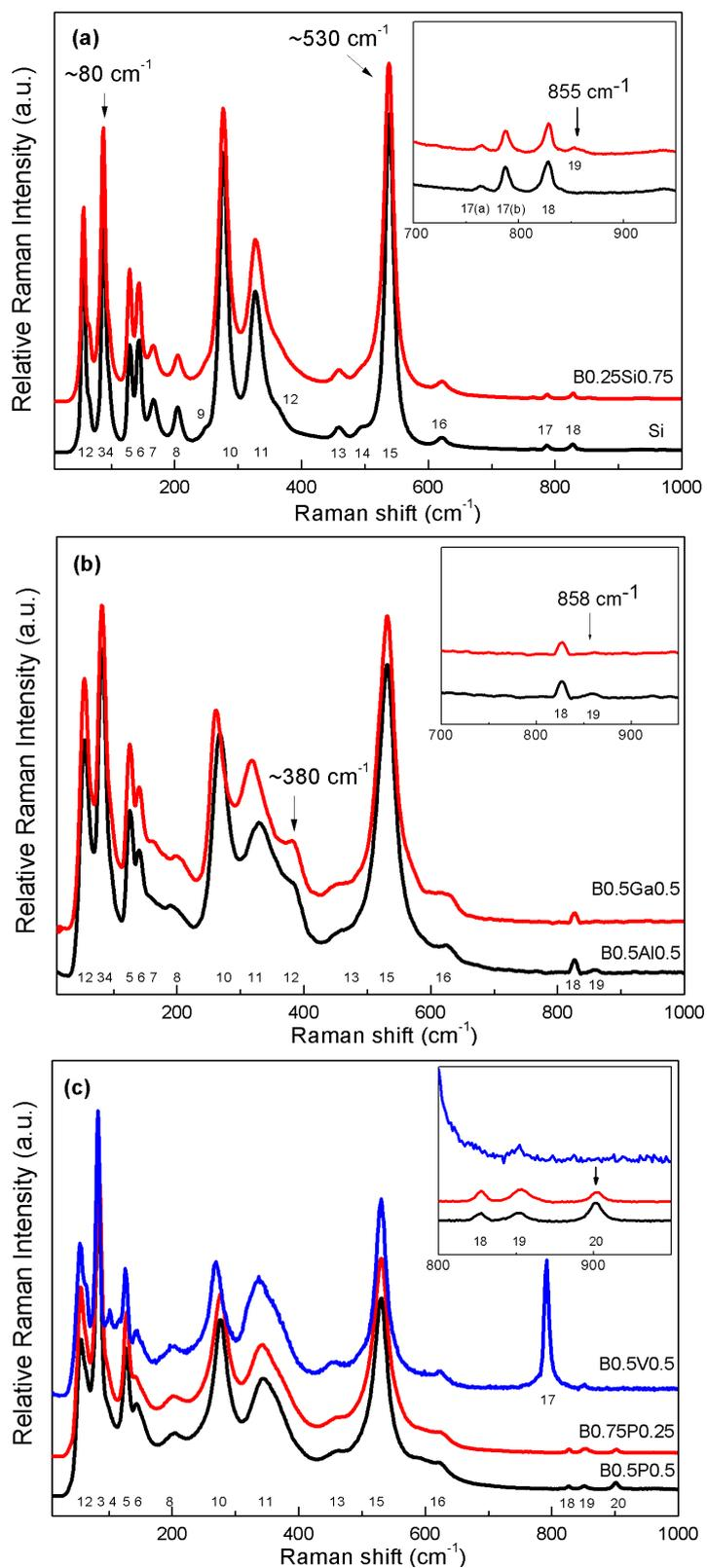
**Figure 5.10** Room temperature Raman Spectra of (a)  $Bi_{12}(B_{0.25}Si_{0.75})O_{19.875}$  in comparison with  $Bi_{12}SiO_{20}$ ; (b)  $Bi_{12}(B_{0.5}Ga_{0.5})O_{19.5}$  and  $Bi_{12}(B_{0.5}Al_{0.5})O_{19.5}$  and (c)  $Bi_{12}(B_{0.5}V_{0.5})O_{20}$ ,  $Bi_{12}(B_{0.75}P_{0.25})O_{19.75}$  and  $Bi_{12}(B_{0.5}P_{0.5})O_{20}$ .
