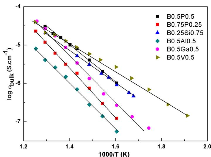
**Figure 5.15** Arrhenius plot of bulk conductivity versus reciprocal temperature for  $B^{3+}$  containing sillenites.
