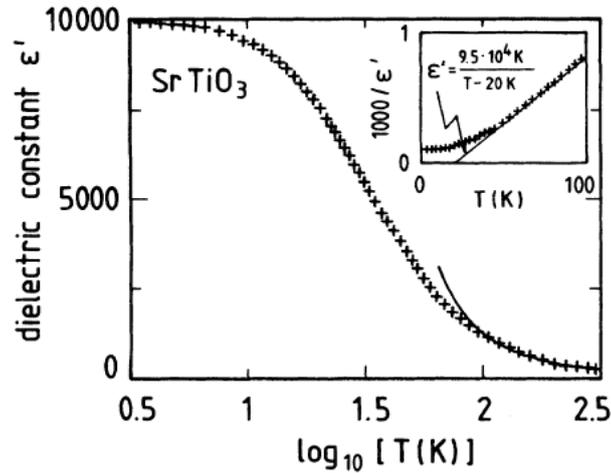
**Figure 1.14**<sup>[78]</sup> The dielectric constant  $\epsilon'$  as a function of temperature measured along the [110] direction of a SrTiO<sub>3</sub> single crystal. The curved line is a fit with the Curie-Weiss law and the inset shows the relation of the inverse  $\epsilon'$  versus temperature, after Viana *et al.*
