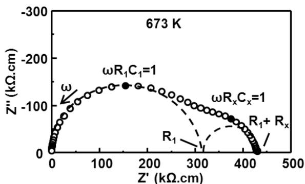
**Figure 3.12**  $Z^*$  plot of  $\text{Bi}_{12}\text{SiO}_{20}$  at 673 K.
