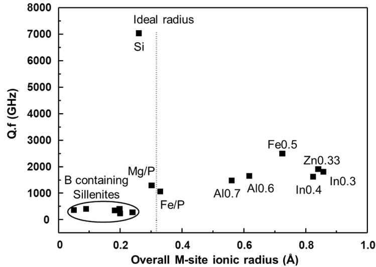
**Figure 7.5** Q.f versus the overall M-site ionic radius of sillenites.
