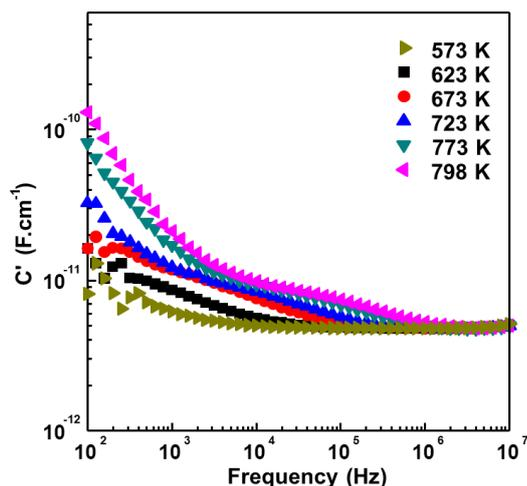
**Figure 5.14**  $C'$  spectroscopic plot at various temperatures for  $Bi_{12}(B_{0.75}P_{0.25})O_{19.75}$ .
