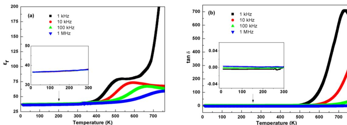
**Figure 4.29** Temperature dependence of (a) permittivity and (b) dielectric losses of compound  $\text{Bi}_{0.7}\text{In}_{0.3}$ . Insets are expanded view of lower temperature data between 10 and 300 K.
