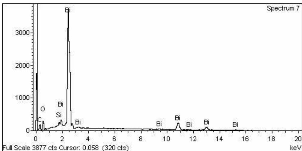
**Figure 3.6** EDS spectrum of  $\text{Bi}_{12}\text{SiO}_{20}$ .
