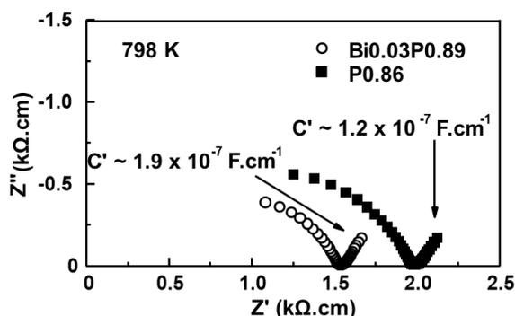
**Figure 6.12**  $Z^*$  plot of superstoichiometric sillenites  $Bi_{0.03}P_{0.89}$  (empty circles) and  $P_{0.86}$  (filled squares) at 798 K showing ionic conductivity.
