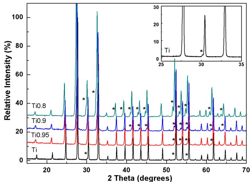
**Figure 9.4** XRPD results of titanium sillenites Bi<sub>12</sub>TiO<sub>20</sub>, Bi<sub>12</sub>Ti<sub>0.95</sub>O<sub>19.9</sub>, Bi<sub>12</sub>Ti<sub>0.9</sub>O<sub>19.8</sub> and Bi<sub>12</sub>Ti<sub>0.8</sub>O<sub>19.6</sub> heated at 750 °C for 72 hours. None of them are phase-pure sillenites with impurity phase of γ-Bi<sub>2</sub>O<sub>3</sub> (ICCD card [45-1344], notation \*).
