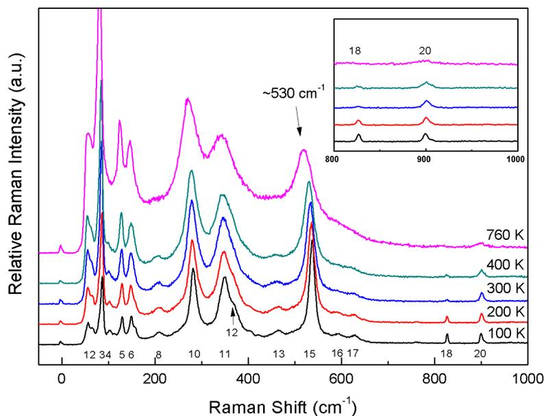
**Figure 6.4** Raman spectra of  $\text{Bi}_{0.03}\text{P}_{0.89}$  at 100, 200, 300, 400 and 760 K. Peak intensities are normalized by peak  $\sim 530\text{ cm}^{-1}$ . Inset is the enlarged version of showing Raman peak  $\sim 825\text{ cm}^{-1}$  (line 18) and  $\sim 901\text{ cm}^{-1}$  (line 20).
