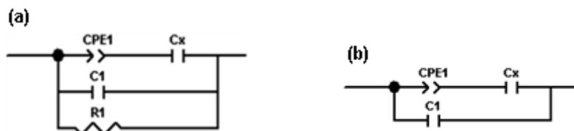
Figure 9.10 (a) and (b) Equation circuit for dielectric relaxation.
