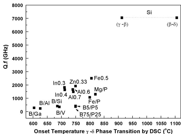
**Figure 7.7** Q.f versus polymorphic  $\gamma$ - $\delta$  phase transition temperature from DSC (heating cycles) for sillenites.
