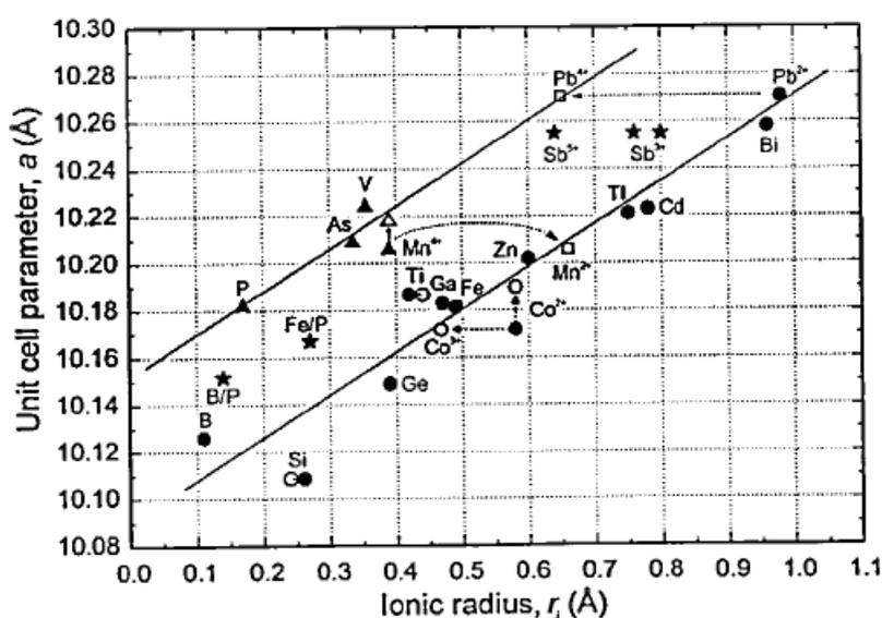
**Figure 1.7**<sup>[44]</sup> Relationships between unit cell parameter ( $a$ ) and ionic radius ( $r$ ) of various M-ion doped sillenites, after Poleti *et al.*
