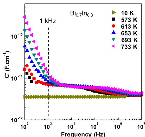
**Figure 4.31**  $C'$  spectroscopic plot at various temperatures for  $\text{Bi}_{12}(\text{Bi}_{0.7}\text{In}_{0.3})\text{O}_{19.5}$ .
