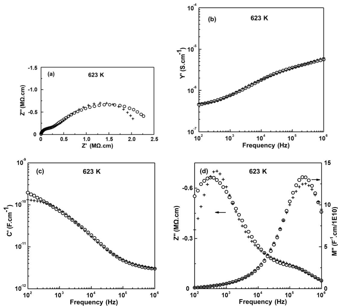
**Figure 9.30** High temperature IS experimental data points (○) and the fitting results (+) to equivalent circuit shown in Figure 9.10 (a) with (a)  $Z^*$  plot; (b)  $Y'$ , (c)  $C'$ , and (d)  $-Z''/M''$  spectroscopic plots at 623 K for  $\text{Bi}_{12}(\text{Fe}_{0.5}\text{P}_{0.5})\text{O}_{20}$ .
