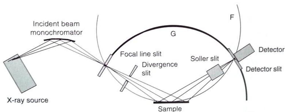
**Figure 2.1**<sup>[1]</sup> Schematic representation of an X-ray diffractometer with an incident beam monochromator, after Clearfield *et al.*
