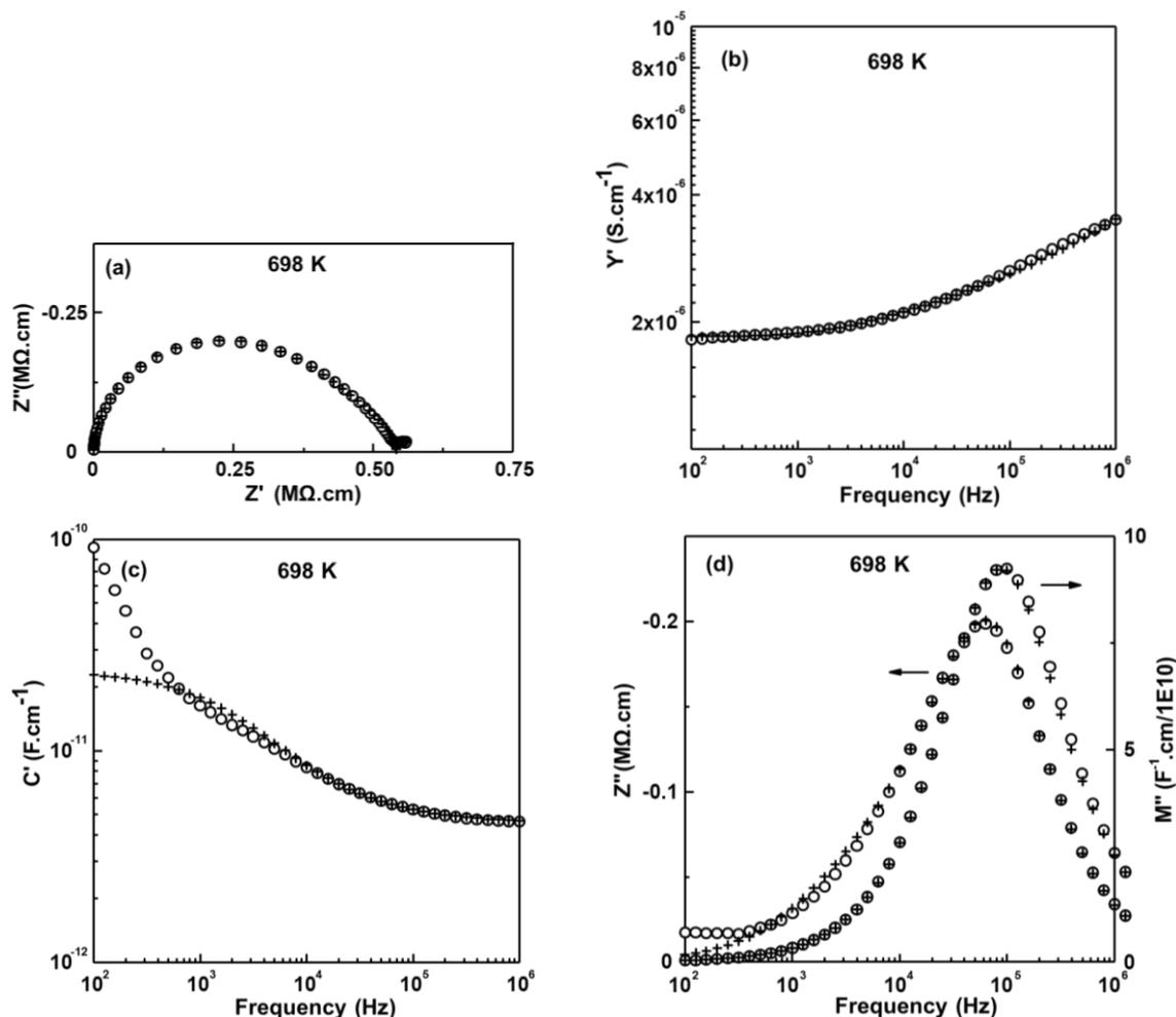
**Figure 9.18** High temperature IS experimental data points (○) and the fitting results (+) to equivalent circuit in Figure 9.10 (a) with (a)  $Z^*$  plot; (b)  $Y'$ , (c)  $C'$ , and (d)  $-Z''/M''$  spectroscopic plots at 698 K for  $\text{Bi}_{12}(\text{B}_{0.5}\text{Ga}_{0.5})\text{O}_{19.5}$ .
