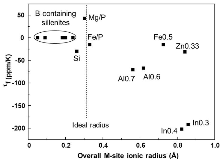
**Figure 7.4**  $\tau_f$  versus overall M-ion ionic radius of the studied sillenites.
