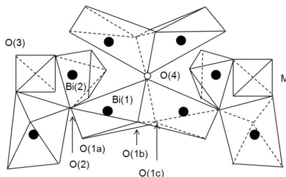
**Figure 6.1** Structural feature of superstoichiometric sillenite with additional oxygen O(4) atom occupied the  $6b$  site to show distinct Bi-O framework polyhedra.
