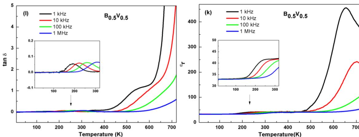
**Figure 5.12** Temperature dependence of permittivity ( $\epsilon_r$ ) and dielectric loss ( $\tan \delta$ ) of (a) and (b)  $Bi_{12}(B_{0.5}P_{0.5})O_{20}$ ; (c) and (d)  $Bi_{12}(B_{0.75}P_{0.25})O_{19.75}$ ; (e) and (f)  $Bi_{12}(B_{0.25}Si_{0.75})O_{19.875}$ ; (g) and (h)  $Bi_{12}(B_{0.5}Al_{0.5})O_{19.5}$ ; (i) and (j)  $Bi_{12}(B_{0.5}Ga_{0.5})O_{19.5}$ ; (k) and (l)  $Bi_{12}(B_{0.5}V_{0.5})O_{20}$ ; respectively.
