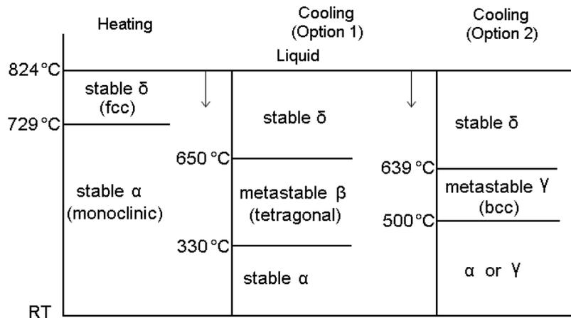
**Figure 1.1**<sup>[8]</sup> Transformation of  $\text{Bi}_2\text{O}_3$  polymorphs, of which  $\alpha$ - $\text{Bi}_2\text{O}_3$  is monoclinic with space group  $P2_1/c$ <sup>[9]</sup>;  $\beta$ - $\text{Bi}_2\text{O}_3$  is tetragonal with space group  $P-4b2$ <sup>[10]</sup>;  $\delta$ - and  $\gamma$ - $\text{Bi}_2\text{O}_3$  is cubic with space group  $Fm-3m$ <sup>[11]</sup> and  $I23$ <sup>[9]</sup>, respectively.
