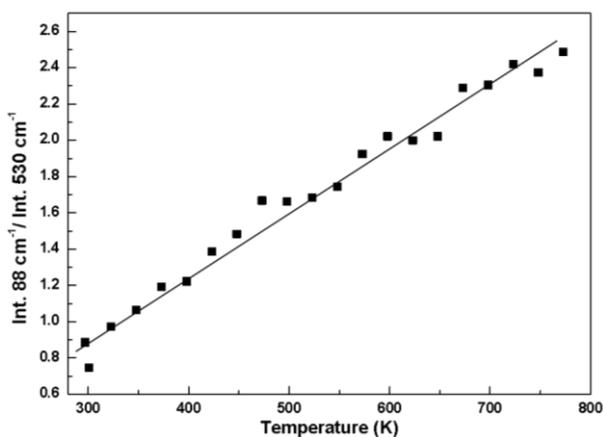
**Figure 3.21** The intensity ratio of Raman peak  $\sim 88\text{ cm}^{-1}$  to peak  $\sim 530\text{ cm}^{-1}$  versus temperature from the same grain of  $\text{Bi}_{12}\text{SiO}_{20}$  ceramic.
