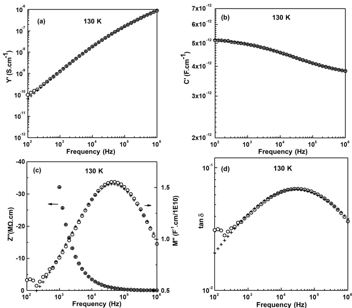
**Figure 9.21** Low temperature IS experimental data points ( $\circ$ ) and the fitting results ( $+$ ) to equivalent circuit shown in Figure 9.10 (b) with (a)  $Y'$ ; (b)  $C'$ , (c)  $-Z''/M''$ , and (d)  $\tan \delta$  spectroscopic plots at 130 K for  $\text{Bi}_{12}(\text{B}_{0.5}\text{Al}_{0.5})\text{O}_{19.5}$ .
