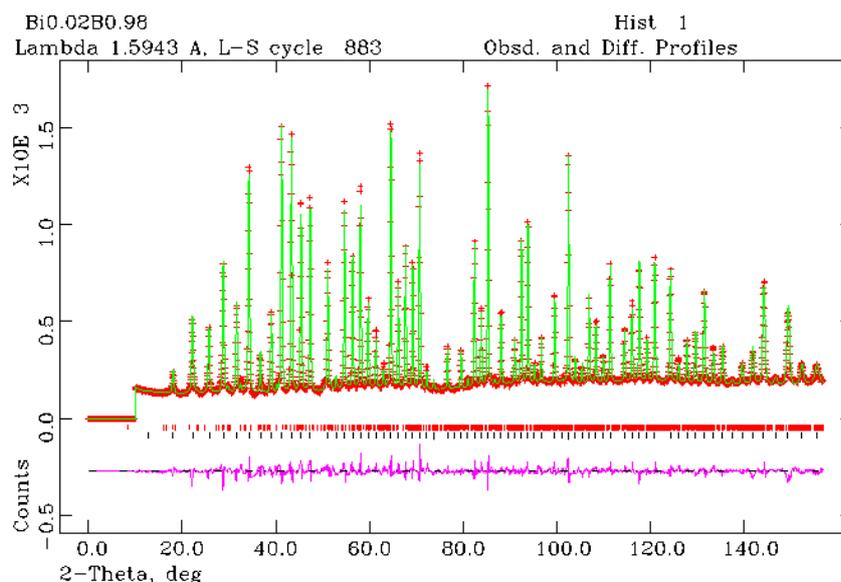
**Figure 5.8** Calculated, experimental and difference profile plot from Rietveld refinement of  $\text{Bi}_{12}(\text{Bi}_{0.02}\text{B}_{0.98})\text{O}_{19.5}$  using NPD data at room temperature to show the goodness of the fit between the R structural model (+) and the observed data (-). Black ticks (|) indicate Bragg reflections of the sillenite phase, whereas red ticks indicates reflection positions of secondary phase  $\text{Bi}_4\text{B}_2\text{O}_9$ .
