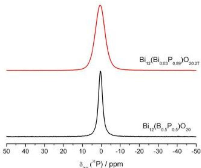
**Figure 6.5** NMR spectra of isotope  $^{31}\text{P}$  one pulse signal of  $\text{Bi}_{12}(\text{B}_{0.5}\text{P}_{0.5})\text{O}_{20}$  and  $\text{Bi}_{12}(\text{Bi}_{0.03}\text{P}_{0.89}\square_{0.08})\text{O}_{20.27}$  carried out at 7.05 T (12.5 kHz MAS).
