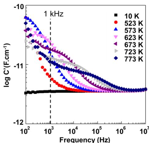
**Figure 3.9**  $C'$  spectroscopic plots at various temperatures for  $\text{Bi}_{12}\text{SiO}_{20}$  ceramic.
