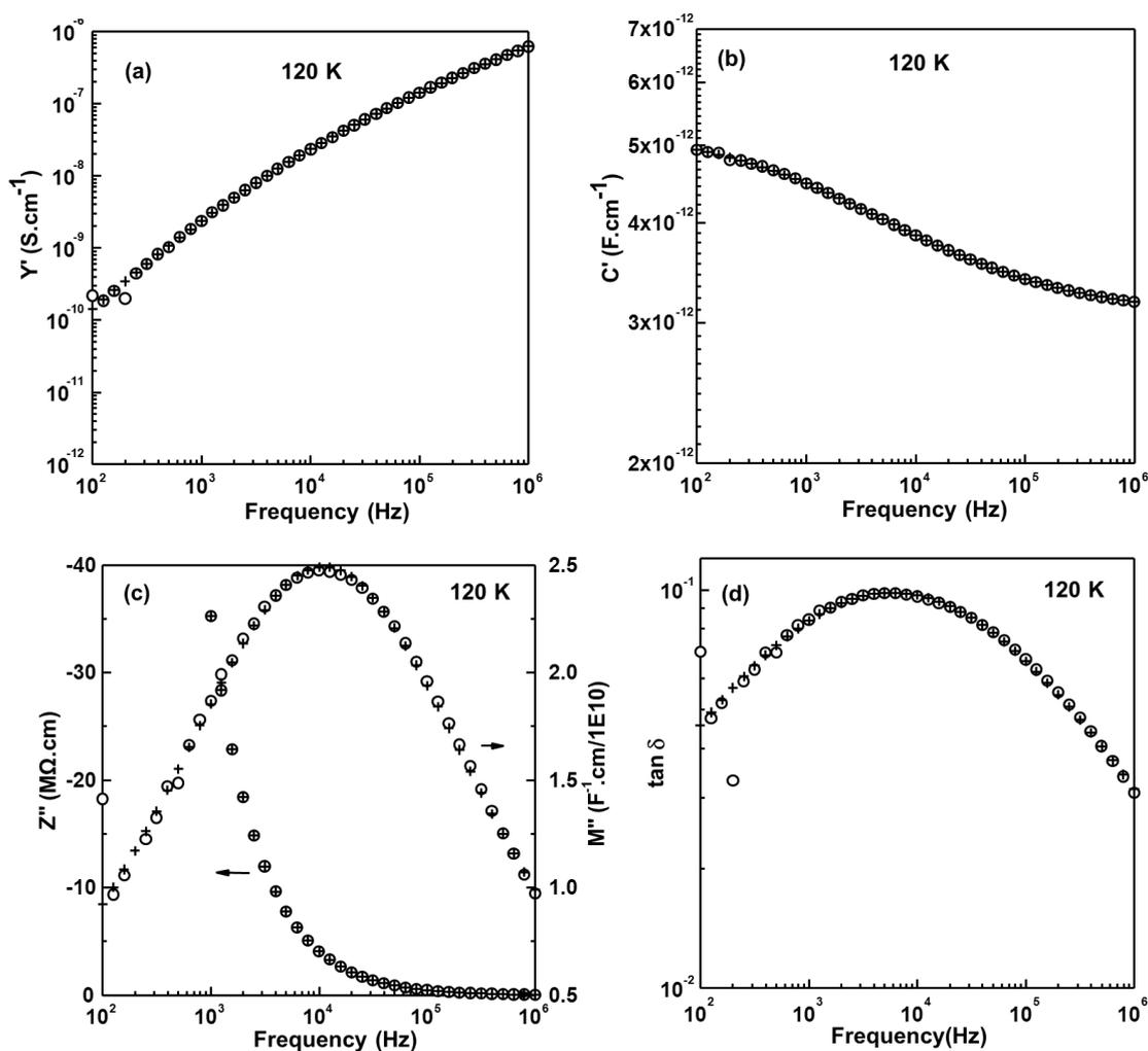
**Figure 9.19** Low temperature IS experimental data points ( $\circ$ ) and the fitting results ( $+$ ) to equivalent circuit shown in Figure 9.10 (b) with (a)  $Y'$ ; (b)  $C'$ , (c)  $-Z''/M''$ , and (d)  $\tan \delta$  spectroscopic plots at 120 K for  $\text{Bi}_{12}(\text{B}_{0.5}\text{Ga}_{0.5})\text{O}_{19.5}$ .
