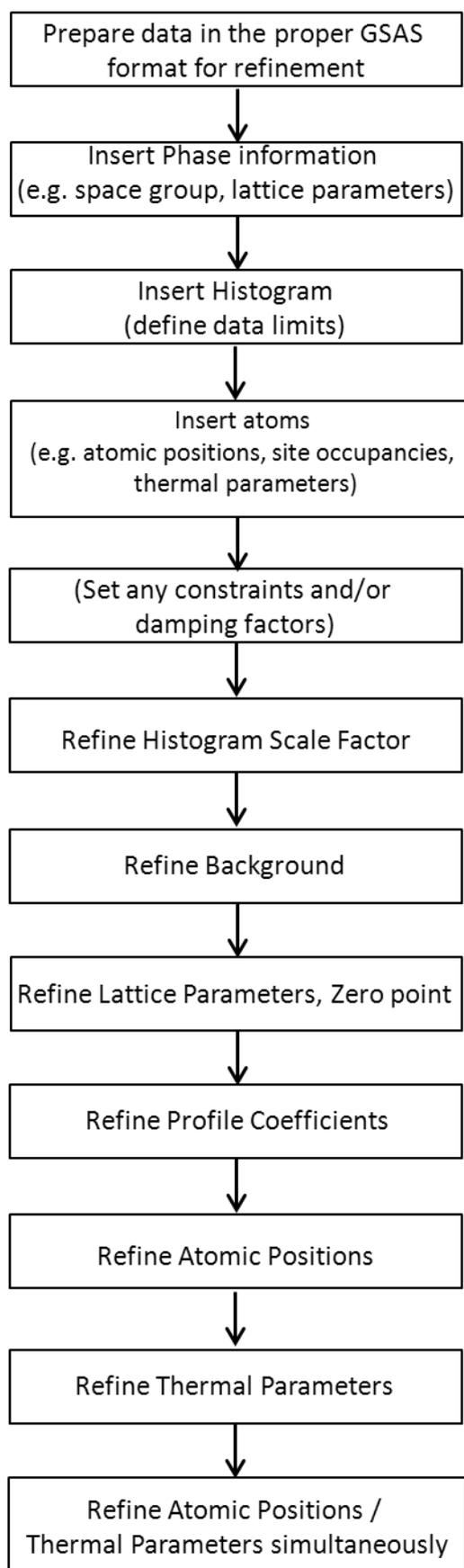
**Figure 2.5** Basic Rietveld refinement procedures.<sup>[7]</sup>
