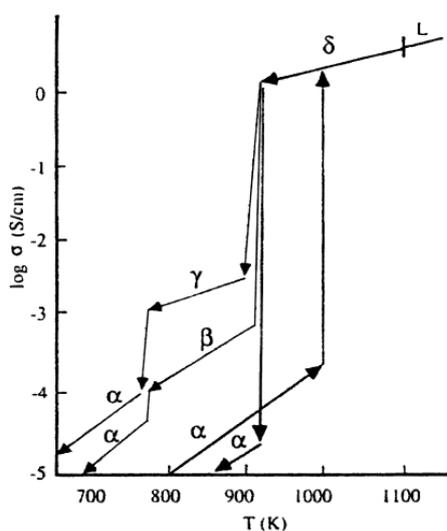
**Figure 1.2**<sup>[8]</sup> Electrical conductivity of  $\text{Bi}_2\text{O}_3$  polymorphs as a function of temperature during heating ( $\blacktriangleright$ ) and cooling ( $\blacktriangleleft$ ) cycles.
