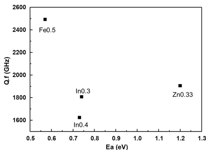
**Figure 4.37** Activation energy for bulk conduction versus Q.f for  $\text{Bi}_{0.67}\text{Zn}_{0.33}$ ,  $\text{Bi}_{0.7}\text{In}_{0.3}$ ,  $\text{Bi}_{0.6}\text{In}_{0.4}$  and  $\text{Bi}_{0.5}\text{Fe}_{0.5}$ .
