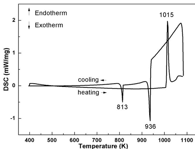
**Figure 4.17** DSC trace of  $\text{Bi}_{12}(\text{Bi}_{0.3}\text{Al}_{0.7})\text{O}_{19.5}$ .
