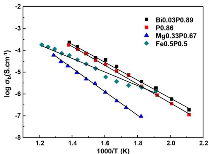
**Figure 6.14** Arrhenius plot of bulk conductivity versus reciprocal temperature for  $P^{5+}$  containing sillenites.
