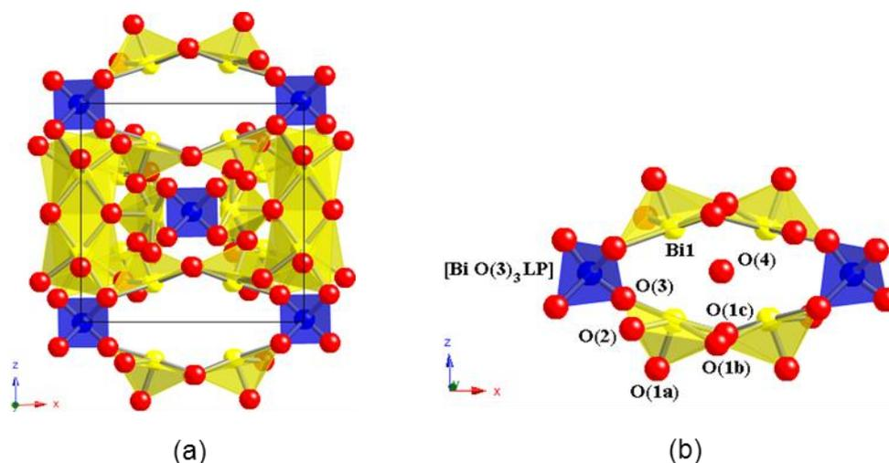
**Figure 1.3** Structure of (a) ideal ( $\text{Bi}_{12}\text{M}^{4+}\text{O}_{20}$ ) sillénite<sup>[22]</sup> viewed along the (001) plane,
