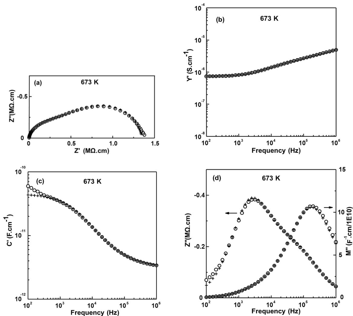
**Figure 9.26** High temperature IS experimental data points (○) and the fitting results (+) to equivalent circuit shown in Figure 9.10 (a) with (a)  $Z^*$  plot; (b)  $Y'$ , (c)  $C'$ , and (d)  $-Z''/M''$  spectroscopic plots at 673 K for  $\text{Bi}_{12}(\text{B}_{0.5}\text{V}_{0.5})\text{O}_{19.5}$ .
