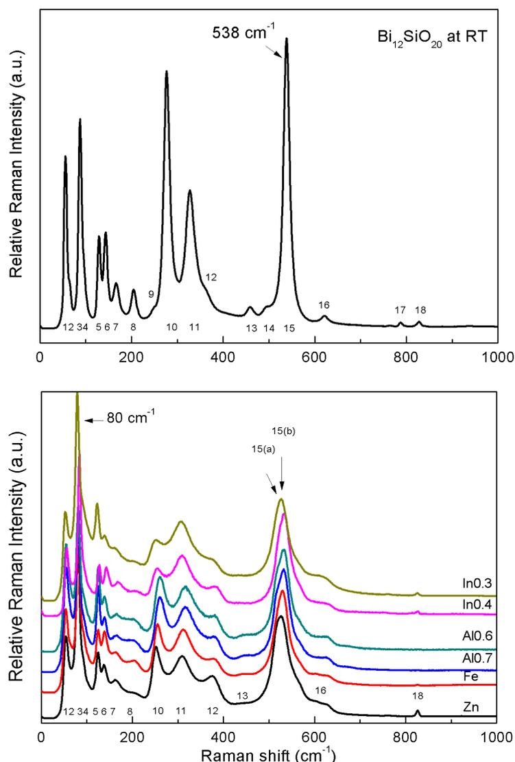
**Figure 4.21** Raman Spectra of  $M^{2+}/M^{3+}$  sillenites in comparison with  $\text{Bi}_{12}\text{SiO}_{20}$  at room temperature.
