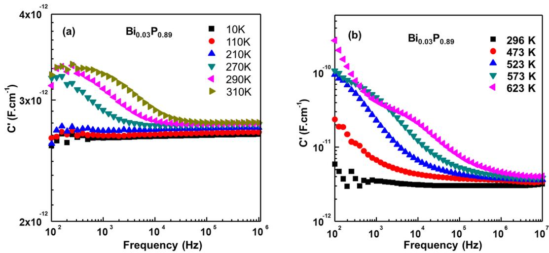
**Figure 6.10**  $C'$  spectroscopic plot at various temperatures for  $Bi_{12}(Bi_{0.03}P_{0.89})O_{20.27}$  to show (a) low and (b) high temperature relaxation behaviour.
