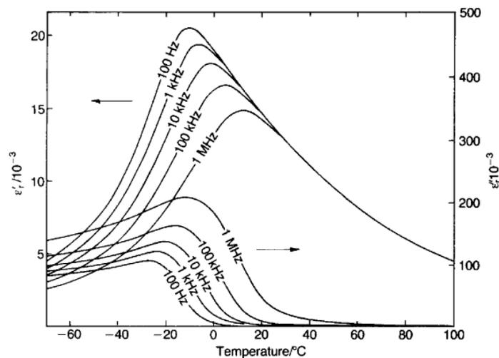
**Figure 1.15**<sup>[55]</sup> Temperature dependence of  $\epsilon'$  and  $\epsilon''$  of Pb(Mg<sub>1/3</sub>Nb<sub>2/3</sub>)O<sub>3</sub> (PMN).
