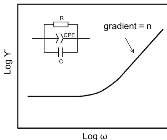
**Figure 1.19**<sup>[81]</sup> Log  $Y'$  versus log  $\omega$  plot. Inset shows a possible equivalent circuit to model the impedance response.
