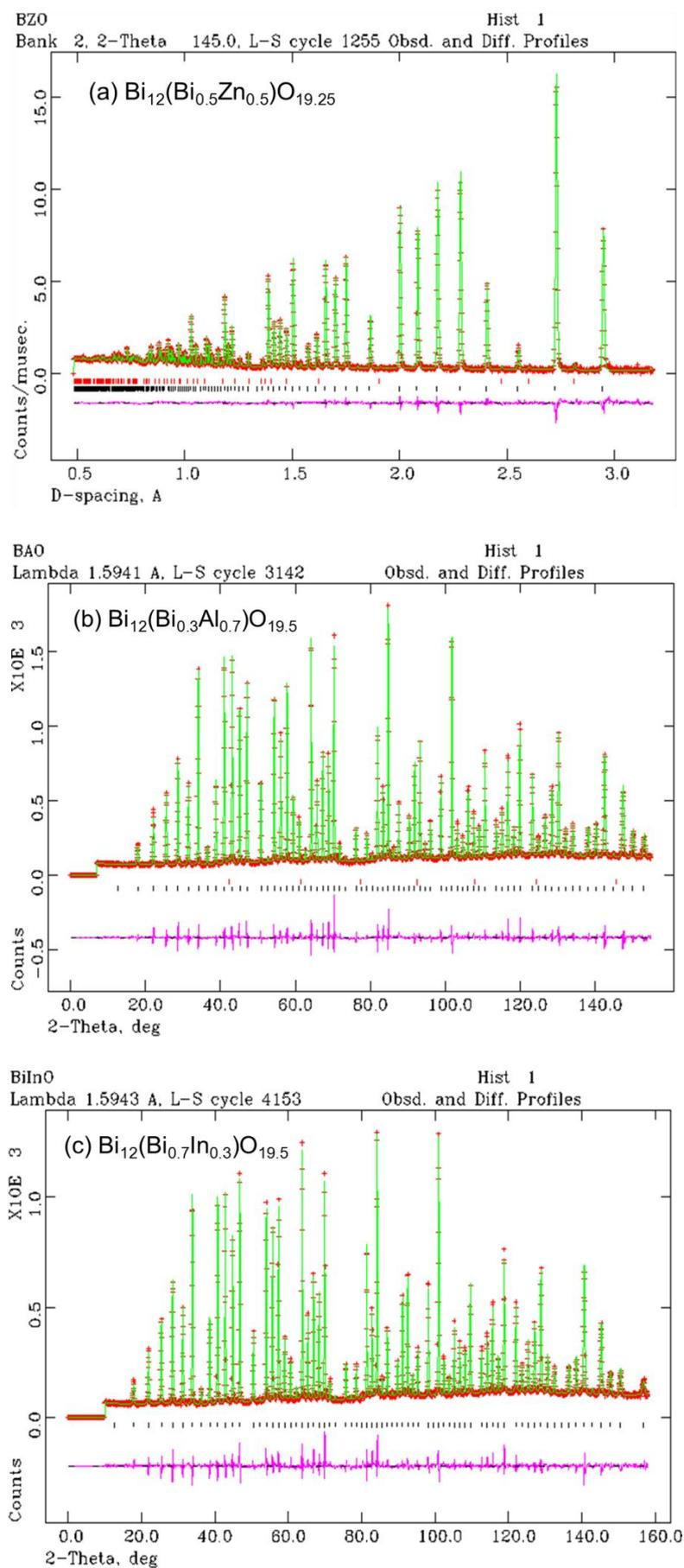
Figure 4.7 Calculated, experimental and difference profile plot from Rietveld refinement
