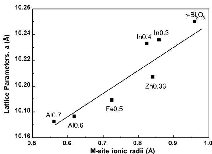
**Figure 4.34** The relationship between the unit cell parameters and the M-site ionic radii of  $M^{2+}/M^{3+}$  sillenites (as there is lack of data for four-fold coordinated  $Bi^{3+}$  ions in a M-site, ionic radius data of  $Bi^{3+}$  ions with a coordination number of five was used  $r_{Bi^{3+}(V)} = 0.96$  Å from Shannon<sup>[35]</sup>); data for  $\gamma$ - $Bi_2O_3$ <sup>[35]</sup> is included for comparison.
