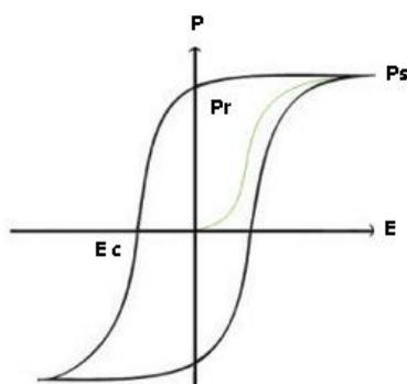
**Figure 1.12**<sup>[55]</sup> Hysteresis (P-E) loop of a ferroelectric material.
