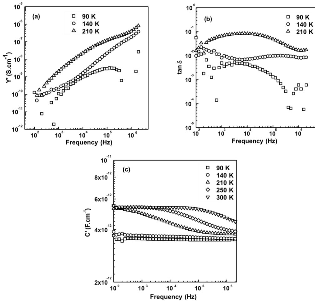
**Figure 5.17** (a)  $Y'$ , (b)  $\tan \delta$  and (c)  $C'$  spectroscopic plots of  $B_{0.75}P_{0.25}$  at various temperatures.
