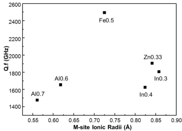
**Figure 4.24** Q.f as a function of M-site ionic radii of  $\text{M}^{2+}/\text{M}^{3+}$  sillenites.
