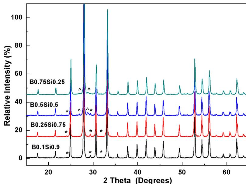
**Figure 5.3** XRPD results of sample  $Bi_{12}(B_{0.1}Si_{0.9})O_{19.95}$ ,  $Bi_{12}(B_{0.25}Si_{0.75})O_{19.875}$ ,  $Bi_{12}(B_{0.5}Si_{0.5})O_{19.75}$  and  $Bi_{12}(B_{0.75}Si_{0.25})O_{19.625}$  prepared directly from reagents  $Bi_2O_3$ ,  $B(OH)_3$  and  $SiO_2$ . Notations \* and ^ indicate the presence of secondary phases  $Bi_2SiO_5$  (ICCD card [75-1483]) and  $Bi_4B_2O_9$  (ICCD card [70-1458]), respectively.
