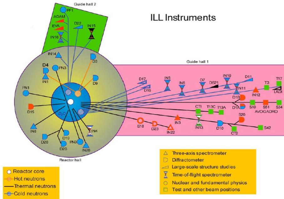
**Figure 2.3**<sup>[3]</sup> The instrument layout at the ILL.
