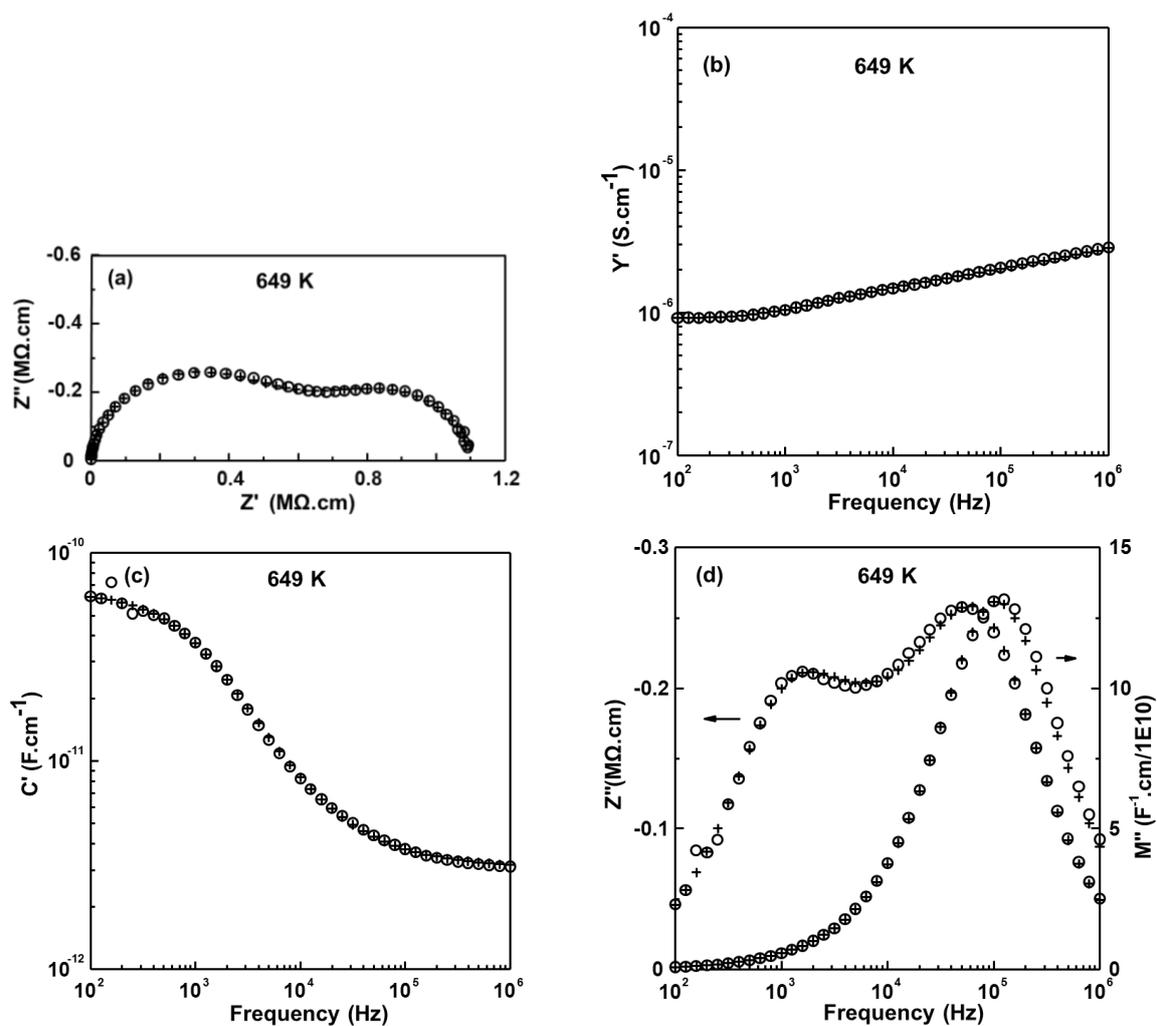
**Figure 9.31** High temperature IS experimental data points (o) and the fitting results (+) to
