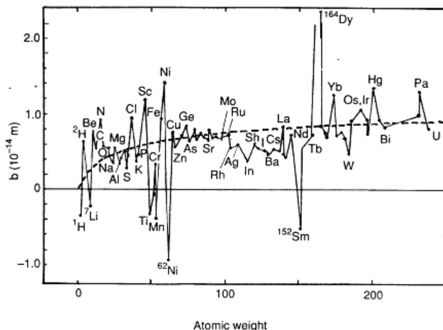
**Figure 2.2**<sup>[2]</sup> Nuclear scattering lengths for thermal neutrons shown as a function of atomic weight, after Young.
