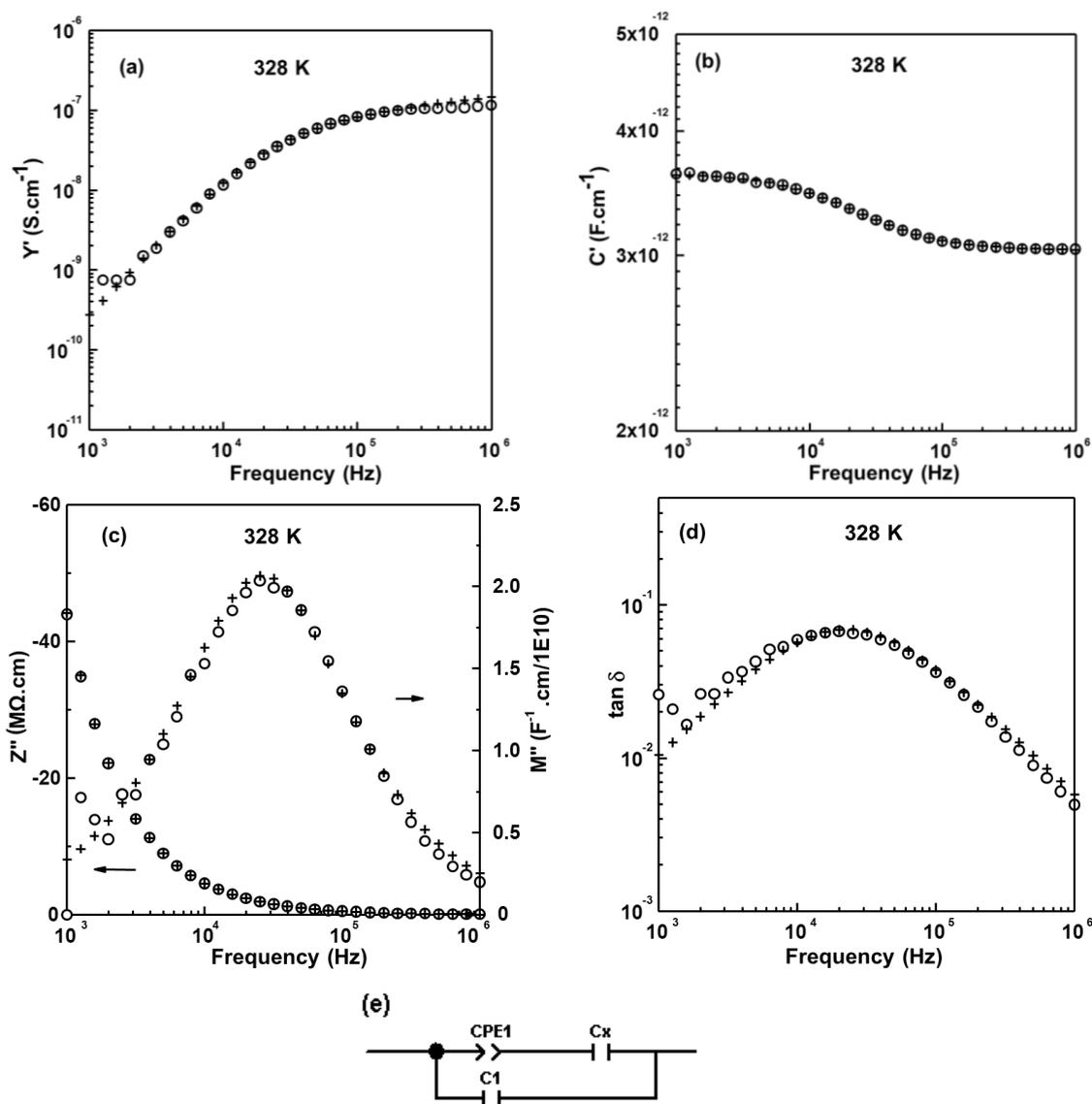
**Figure 6.8** Low temperature IS experimental data points ( $\circ$ ) and the fitting results ( $+$ ) to equivalent circuit shown in (e) with (a)  $Y'$ ; (b)  $C'$ , (c)  $-Z''/M''$ , and (d)  $\tan \delta$  spectroscopic plots at 328 K for  $Bi_{12}(Bi_{0.03}P_{0.89})O_{20.27}$ .
