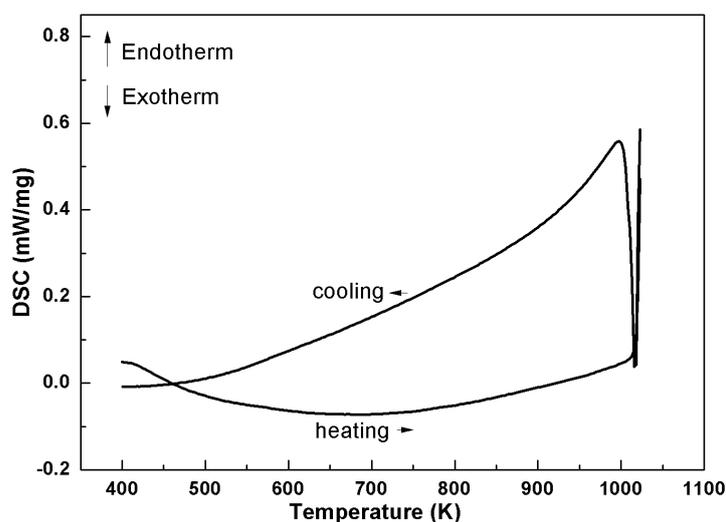
**Figure 4.15** DSC trace of  $\text{Bi}_{12}(\text{Bi}_{0.67}\text{Zn}_{0.33})\text{O}_{19.33}$ .
