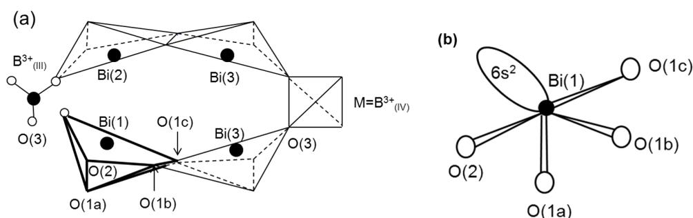
**Figure 5.19** Fragment of structure for (a)  $B^{3+}$  containing sillenites with unshared O(3) atom in  $Bi(1)O_5LP$  polyhedra; (b) distorted trigonal bipyramid  $Bi(1)O_4LP$  with unshared  $Bi^{3+}$  electron lone pairs in  $M^{2+}/M^{3+}$  sillenites.
