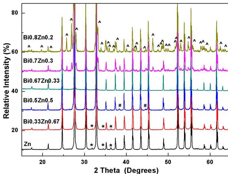
**Figure 4.2** XRPD results of zinc sillenites, where single-phase compounds are  $\text{Bi}_{0.67}\text{Zn}_{0.33}$  and  $\text{Bi}_{0.5}\text{Zn}_{0.5}$ . Notations \*, # and ^ indicate impurity ZnO phase (ICCD card [36-1451]), Aluminum metal peaks (ICCD card [4-787]) from the sample holder of the Philips D500 X-ray diffractometer and impurity  $\alpha\text{-Bi}_2\text{O}_3$  phase (ICCD card [41-1449]), respectively.
