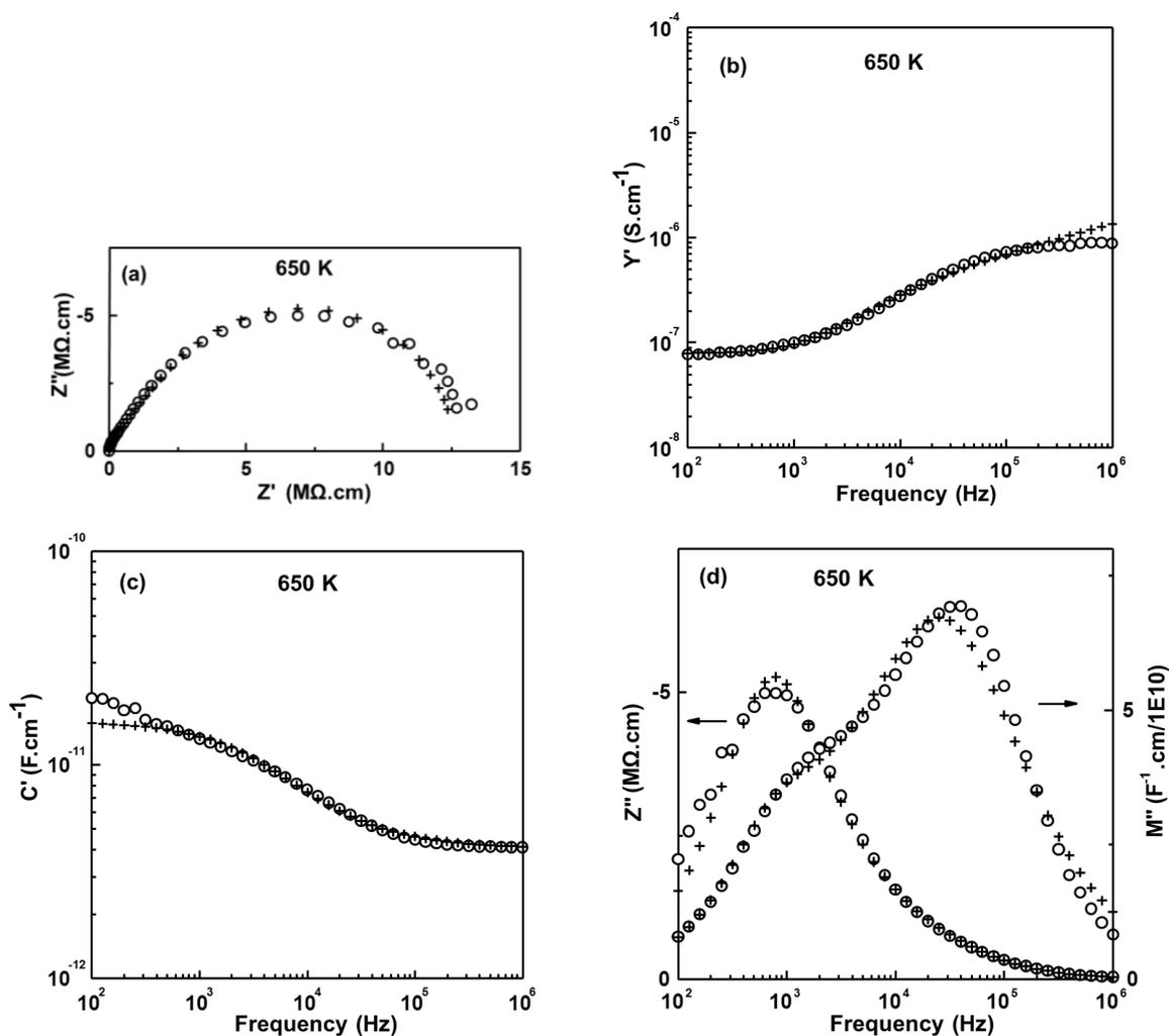
**Figure 9.22** High temperature IS experimental data points ( $\circ$ ) and the fitting results ( $+$ ) to equivalent circuit shown in Figure 9.10 (a) with (a)  $Z^*$  plot; (b)  $Y'$ , (c)  $C'$ , and (d)  $-Z''/M''$  spectroscopic plots at 650 K for  $\text{Bi}_{12}(\text{B}_{0.25}\text{Si}_{0.75})\text{O}_{19.875}$ .
