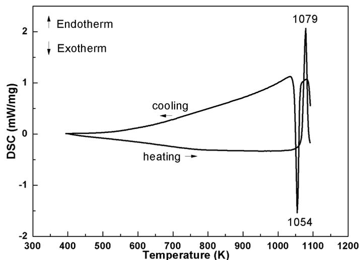
**Figure 4.16** DSC trace of Bi<sub>12</sub>(Bi<sub>0.5</sub>Fe<sub>0.5</sub>)O<sub>19.5</sub>.
