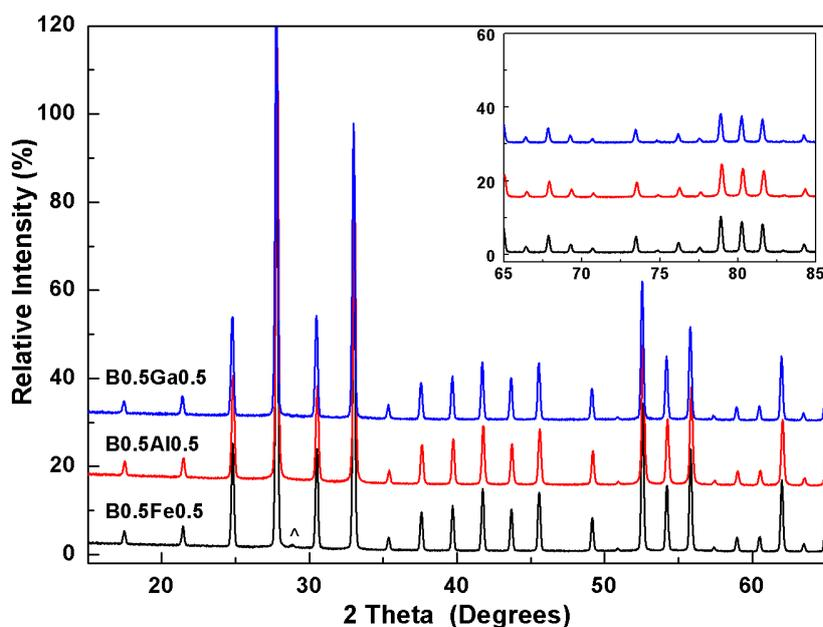
**Figure 5.5** XRPD results of  $Bi_{12}(B_{0.5}Fe_{0.5})O_{19.5}$ ,  $Bi_{12}(B_{0.5}Al_{0.5})O_{19.5}$  and  $Bi_{12}(B_{0.5}Ga_{0.5})O_{19.5}$ . Notation ^ indicates an impurity phase of  $Bi_2Fe_4O_9$  (ICCD card [25-90]).
