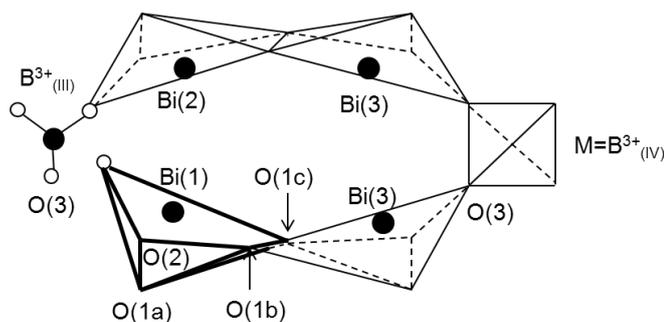
**Figure 5.1** Fragment of the structure showing two different types of boron coordination  $BO(3)_3$  and  $BO(3)_4$  units in the M-sites of  $B^{3+}$  containing sillenites.
