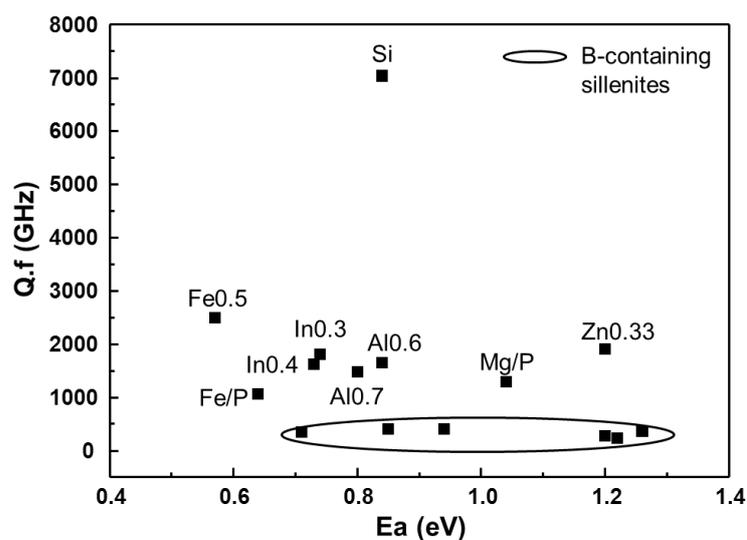
**Figure 7.6** Bulk activation energy ( $E_a$ ) versus quality factor (Q.f) for sillenites.
