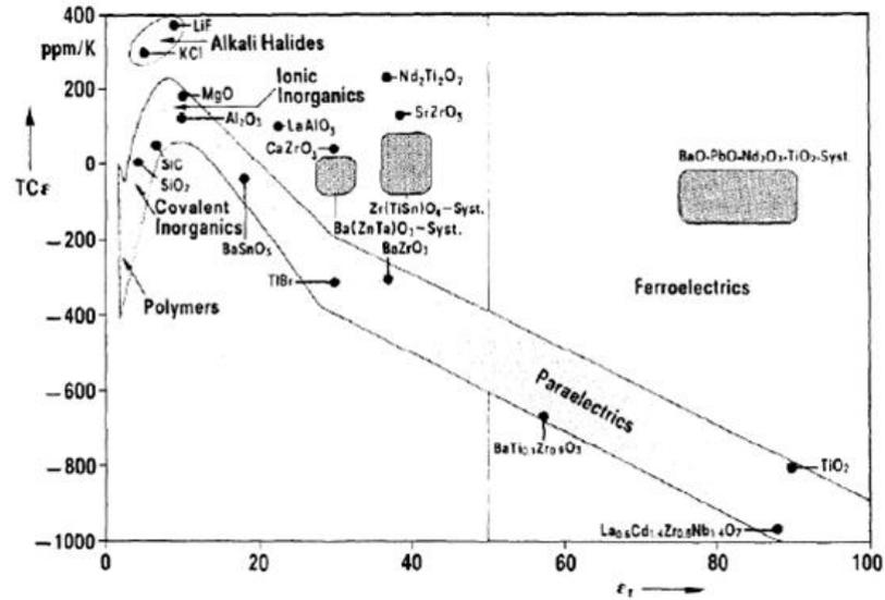
**Figure 1.10** <sup>[65]</sup> Temperature coefficient of permittivity  $\tau_\epsilon$  versus relative permittivity  $\epsilon_r$  for various materials after Harrop.
