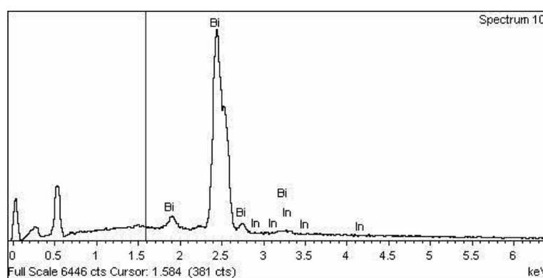
**Figure 4.14** EDS spectrum of  $\text{Bi}_{12}(\text{Bi}_{0.7}\text{In}_{0.3})\text{O}_{19.5}$ .
