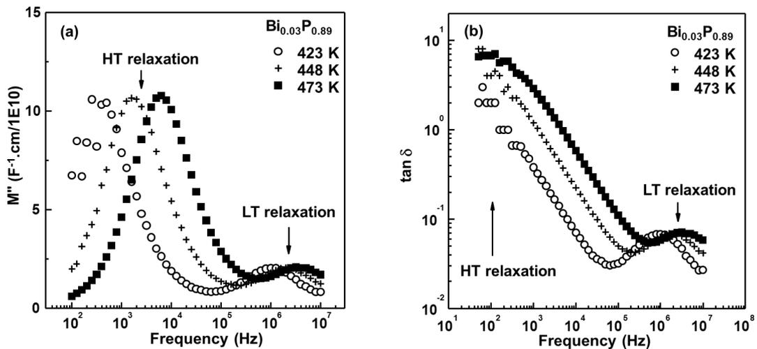
**Figure 6.11** (a)  $M''$  and (b)  $\tan \delta$  spectroscopic plots for  $Bi_{12}(Bi_{0.03}P_{0.89})O_{20.27}$  to show the coexistence of low/high temperature (LT/HT) relaxation phenomenon.
