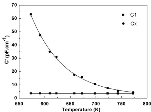
**Figure 3.18** Temperature-dependence of the real capacitance  $C_1$  (■) and  $C_x$  (●) from fitted values.
