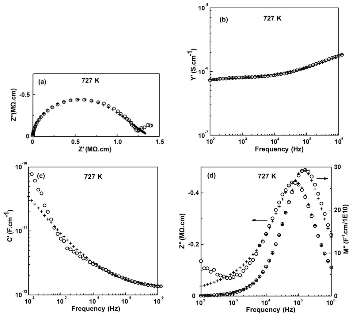
**Figure 9.13** High temperature IS experimental data points ( $\circ$ ) and the fitting results ( $+$ ) to equivalent circuit in Figure 9.10 (a) with (a)  $Z^*$  plot; (b)  $Y'$ , (c)  $C'$ , and (d)  $-Z''/M''$  spectroscopic plots at 727 K for  $\text{Bi}_{12}(\text{Bi}_{0.3}\text{Al}_{0.7})\text{O}_{19.5}$ .
