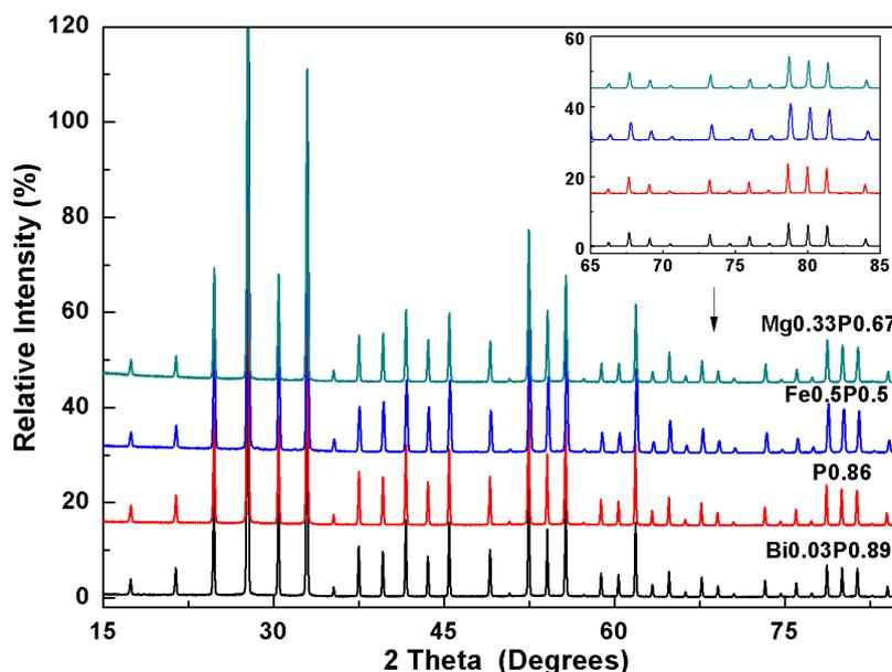
**Figure 6.2** XRPD results of single-phase  $P^{5+}$  containing sillenites  $Bi_{12}(Bi^{3+}_{0.03}P^{5+}_{0.89}\square_{0.08})O_{20.27}$ ,  $Bi_{12}(P^{5+}_{0.86}\square_{0.14})O_{20.15}$ ,  $Bi_{12}(Fe^{3+}_{0.5}P^{5+}_{0.5})O_{20}$  and  $Bi_{12}(Mg^{2+}_{0.33}P^{5+}_{0.67})O_{20}$ .
