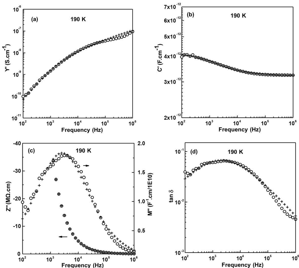
**Figure 9.25** Low temperature IS experimental data points ( $\circ$ ) and the fitting results ( $+$ ) to equivalent circuit shown in Figure 9.10 (b) with (a)  $Y'$ ; (b)  $C'$ , (c)  $-Z''/M''$ , and (d)  $\tan \delta$  spectroscopic plots at 190 K for  $\text{Bi}_{12}(\text{B}_{0.5}\text{P}_{0.5})\text{O}_{19.5}$ .
