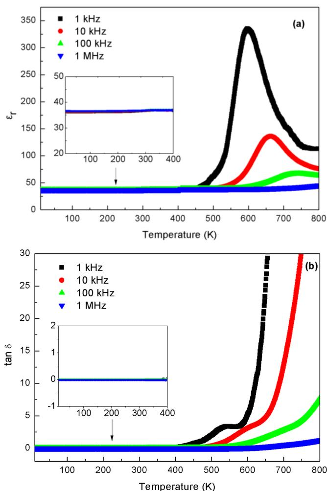
**Figure 3.7** Temperature dependence of (a) permittivity,  $\epsilon_r$ , and (b) dielectric loss,  $\tan \delta$ , of  $\text{Bi}_{12}\text{SiO}_{20}$ . Insets are an expanded view of lower temperature data between 10 and 400 K.
