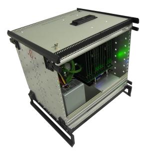
Figure 6.3: University of Leeds 96-channel Ultrasound Array Research Platform (UARP) system. The front panel of the UARP is removed for this photograph.
