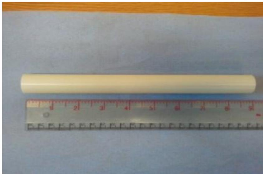
Figure 5.1: The photograph of 8Y-FSZ tube (OD 21mm x ID 16mm x Length 220mm)
