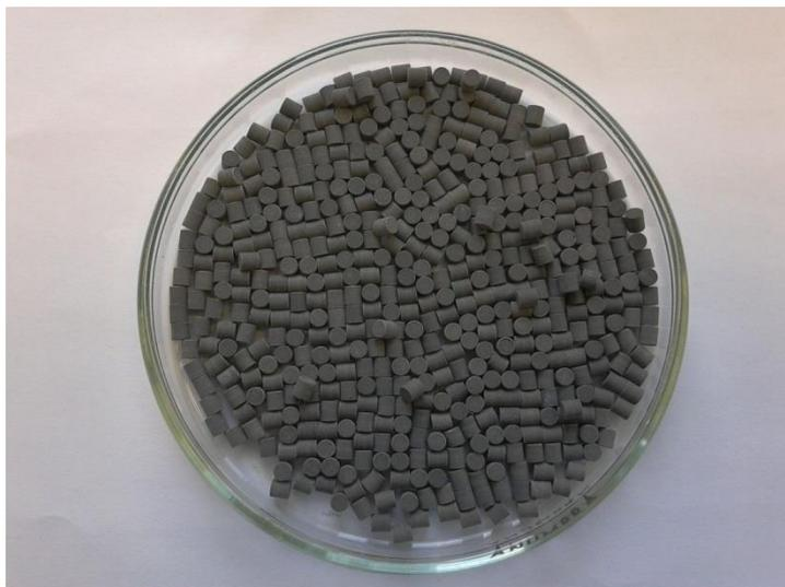
Figure 6.7:  $Pt/Al_2O_3$  catalyst ( $Pt$ , 0.5% on 1/8in alumina pellets, reduced)
