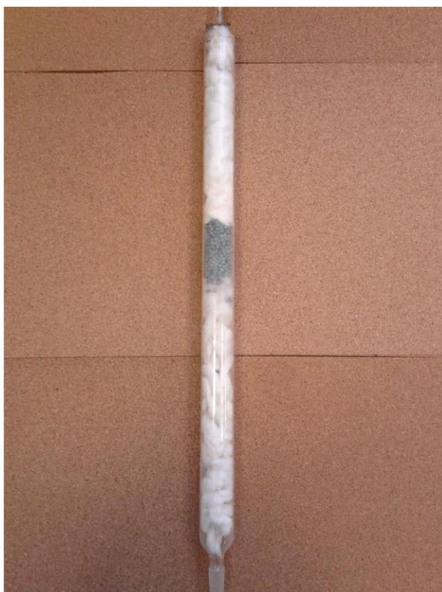
Figure 6.8: Decomposer filled with catalyst and ceramic wool layers
