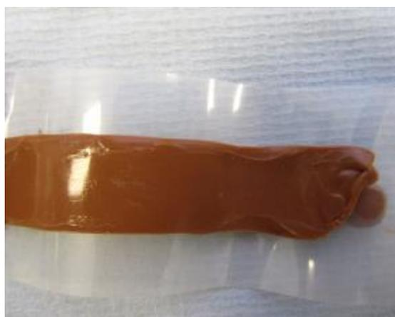
Figure 5.15: Vacuum bag sealant tape
