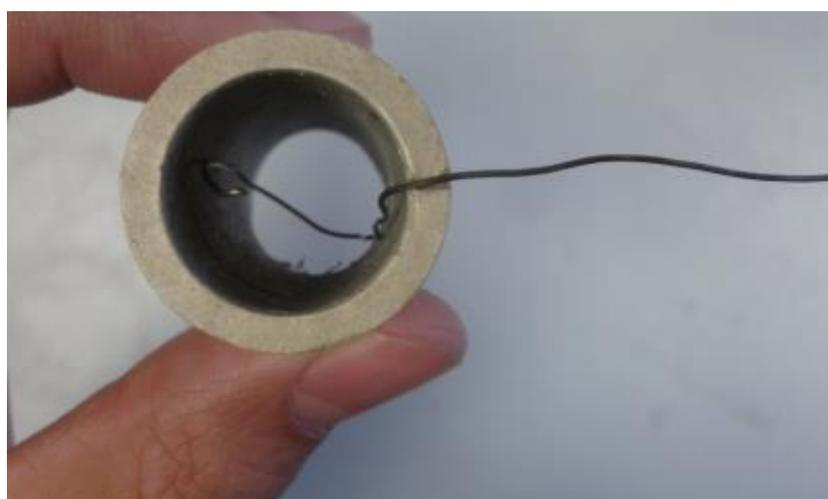
Figure 5.12: *Electrical connection of tube inner electrode surface to power supply*
