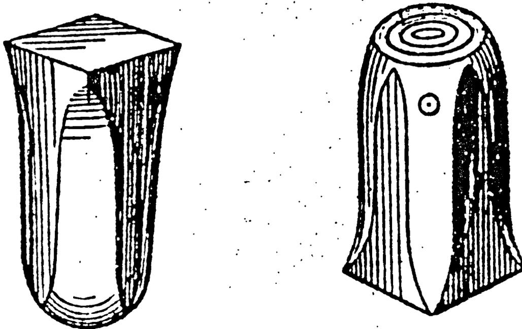
Figure 9.4. Hollow clay pots used in England for vaulting at the end of the eighteenth century.
