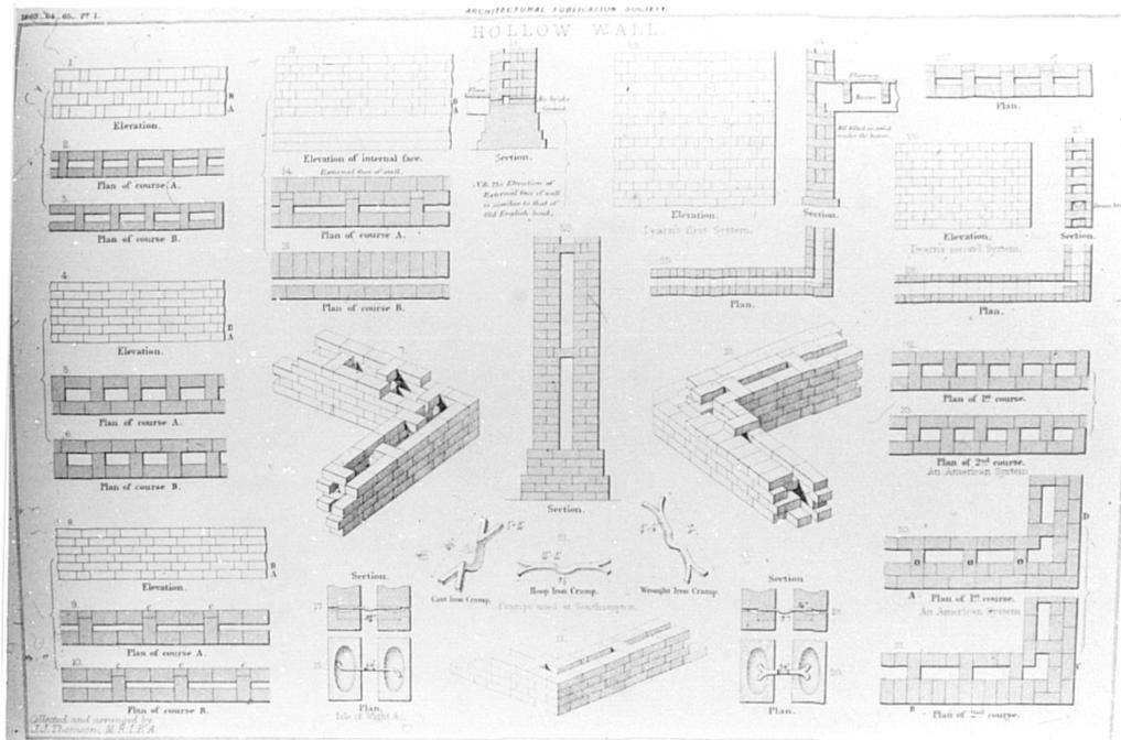
Figure 11.3. Various techniques for constructing hollow walls during the nineteenth century. [From Architectural Publication Society, Illustrations Vol. I (1865)]
