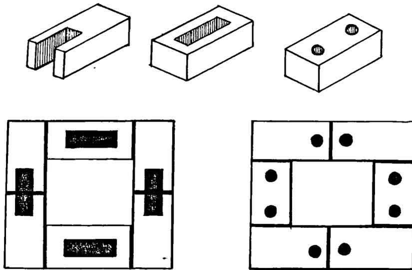
Figure 9.6. Benford Deacon's ventilating hollow bricks, British Patent No. 3664, 1813. [Adapted from The Building News (1858) p. 317]
