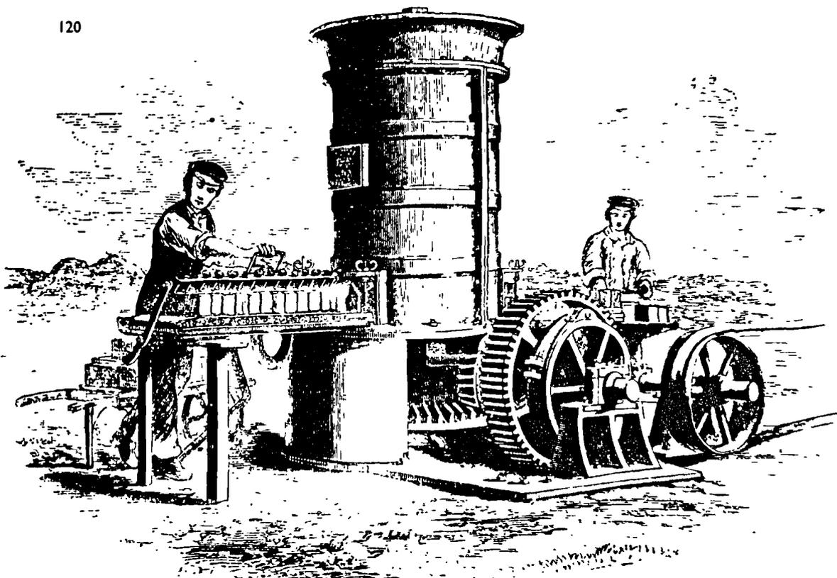
Figure 7.1. Extrusion brickmaking machine attached to a pug mill, Bulmer and Sharp, manufacturer, c. 1860.
