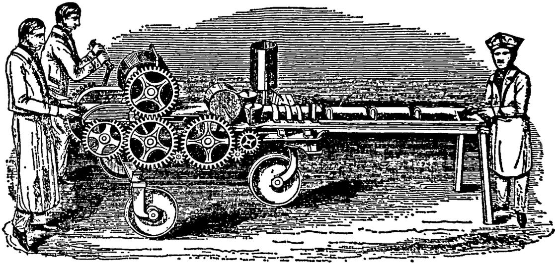
Figure 5.4. Tilemaking machine by the Marquess of Tweeddale, British Patent No. 7253, 1836. [From *The Builder* Vol. 1 1843, p. 195]
