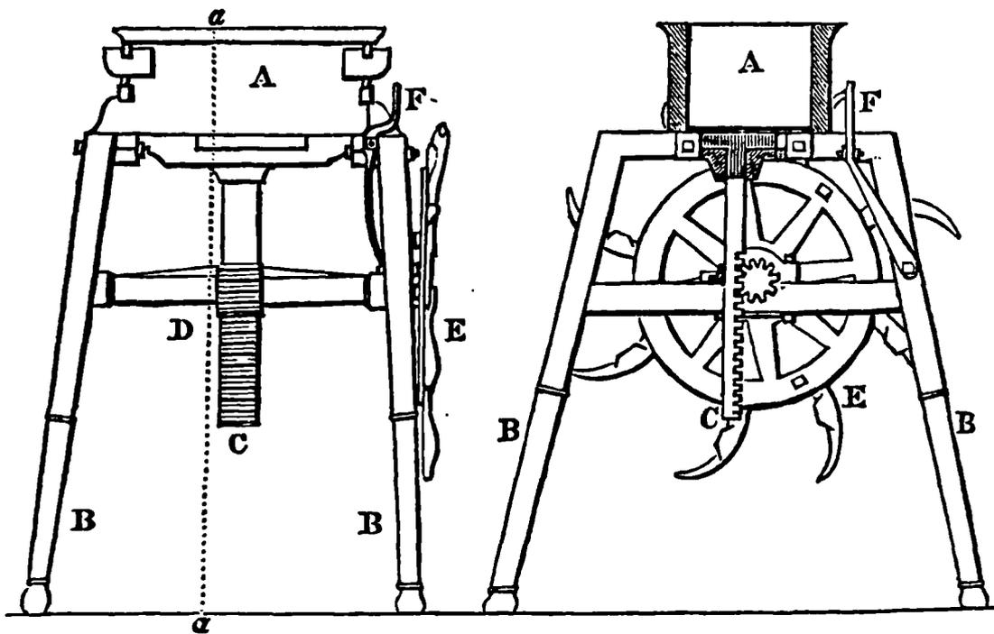
Figure 5.1. Tile-moulding machine invented and manufactured by Robert Beart, c. 1841.
