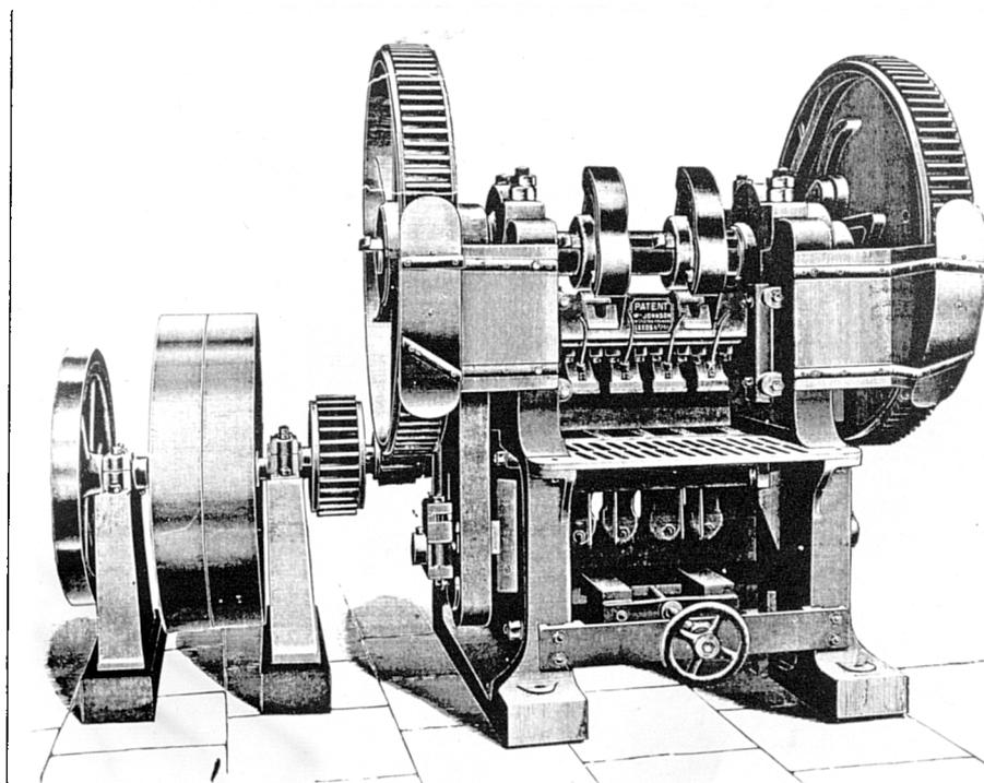
Figure 7.16. Johnson's Patent "Universal" Moulding and Pressing Machine. [From William Johnson, Armley, Leeds trade catalogue, 1894]
