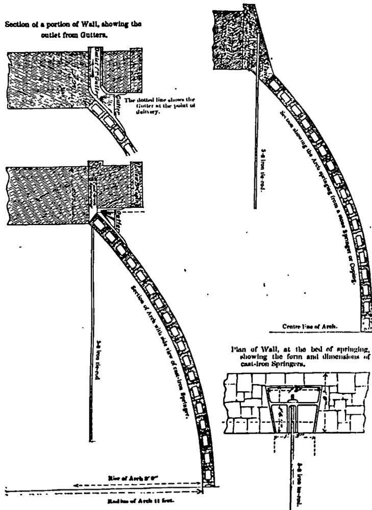
Figure 9.9. Hollow brick roof constructed on the estate of Earl Grey at Howich, c. 1850. [From Journal of the Royal Agricultural Society of England (1854) p. 182]
