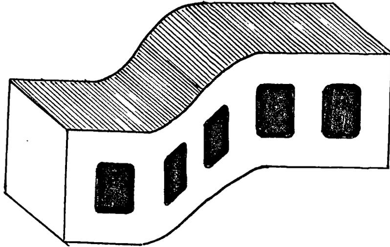
Figure 11.5. Hollow bonding bricks with modified S-curve designed by John Taylor.
