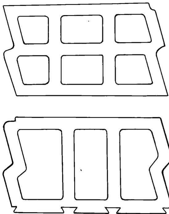
Figure 10.8. Interlocking hollow bricks for fire-proof floors and ceilings patented by J. Bunnett, British Patent No. 1292, 1859. [Adapted from drawing enrolled with patent]
