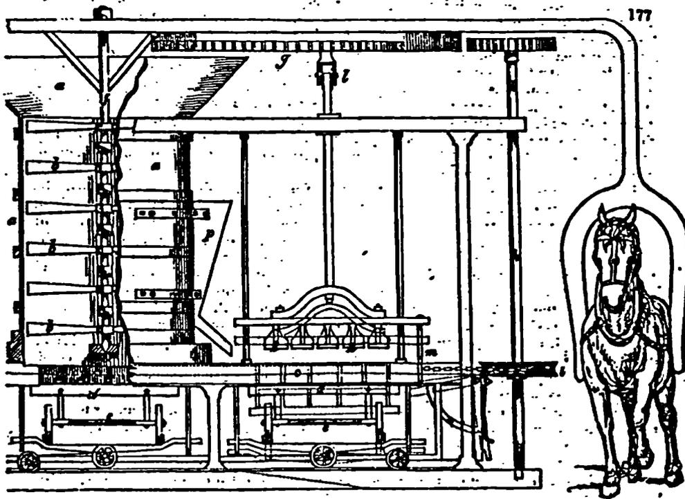
Figure 4.3. Brickmaking machine patented by Thomas Staniford (or Stainford) and George Henry Lyne, British Patent No. 5246, 1825. [From Andrew Ure, A Dictionary of Arts, Manufactures and Mines (1835) p. 186]
