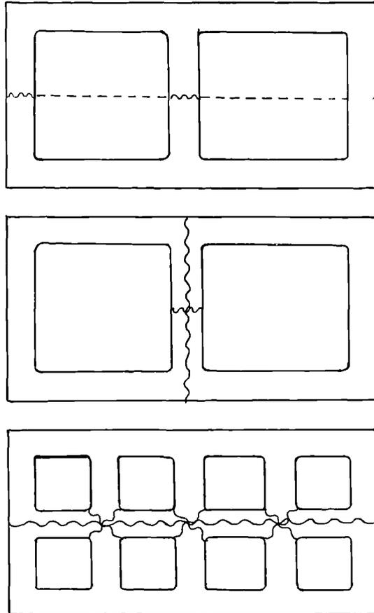
Figure 10.6. Improvements in hollow bricks patented by Jules Henry Borie, British Patent No.13,369, 1850. In previous methods of manufacture (top), the rods holding the perforating cores cut laterally through the outer surfaces of the bricks, thus weakening them. Borie re-arranged the rods so they only cut through the internal divisions of the bricks (centre and bottom).
