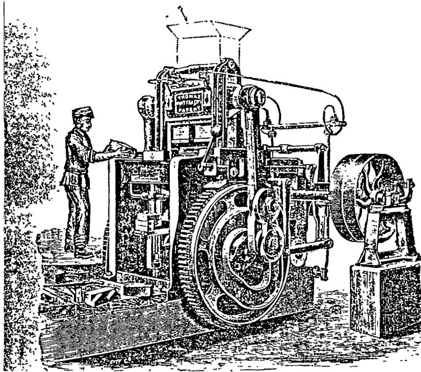
Figure 7.15. Semi-dry brickmaking machine manufactured by Christopher Whittaker and Company, Accrington, c.1890. [From M. Powis Bale, The Building News (1890) p.443]
