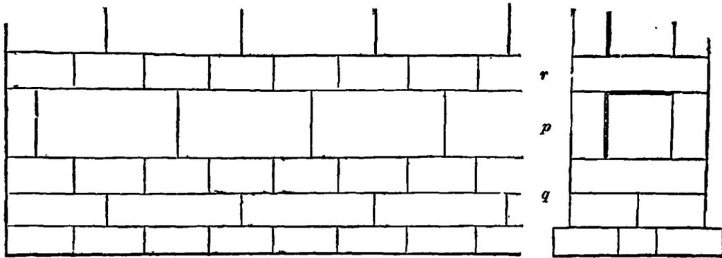
Figure 11.1. Dearn's method of building hollow walls; elevation and section of part of a wall.
