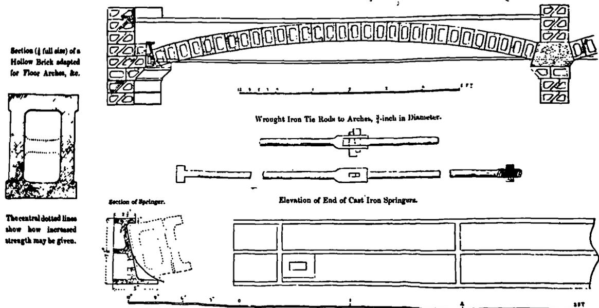
Section (1/2 full size) of a Hollow Brick adapted for Floor Arches, &c.
