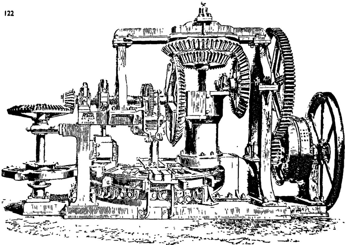
Figure 7.14. Bradley and Craven's semi-dry brick moulding and pressing machine, c. 1862.
