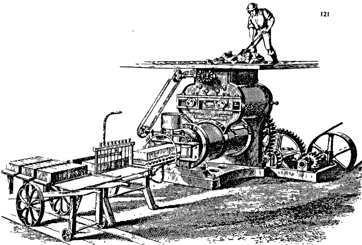
Figure 7.2. Ramp-loaded brickmaking machine by Henry Clayton, c. 1860.
