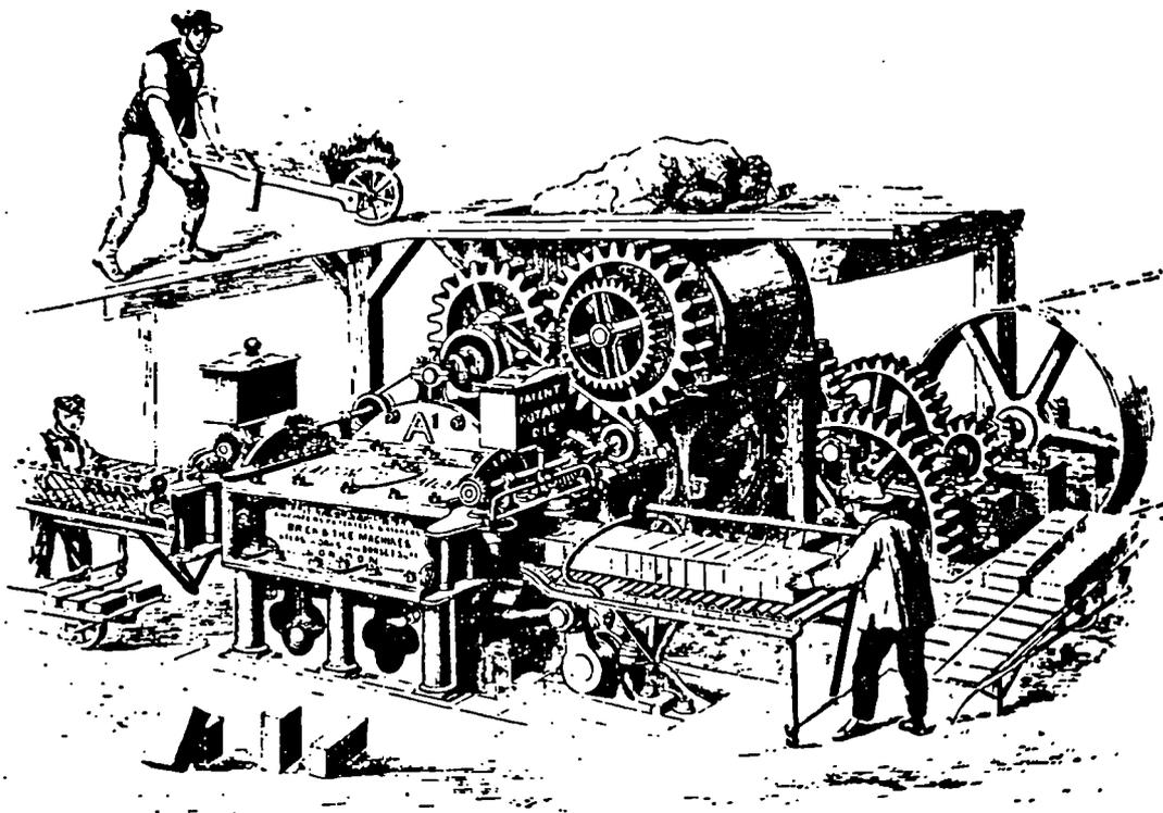
Figure 7.4. Henry Clayton's Universal "A 1" Combined Three-Process Brick Machine.
