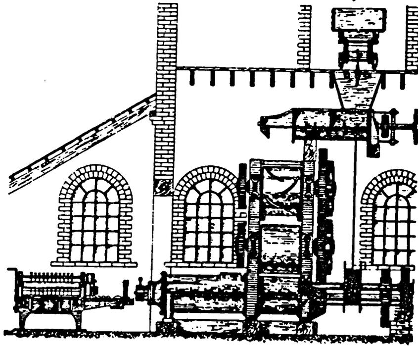
Figure 7.6. Extrusion brickmaking plant with feeder or trough mixer, two sets of crushing rolls, pug mill, die and cutting table. [From Alfred Searle, Modern Brickmaking (1931) p. 139]
