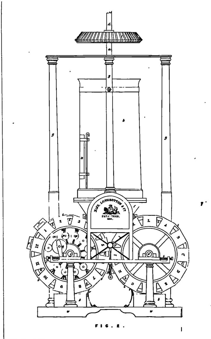
Figure 4.4. Vertical wheel moulding machine, British Patent No. 6257, 1832, John J. Clark, John Nash and John Longbottom. [Drawing enrolled with patent]
