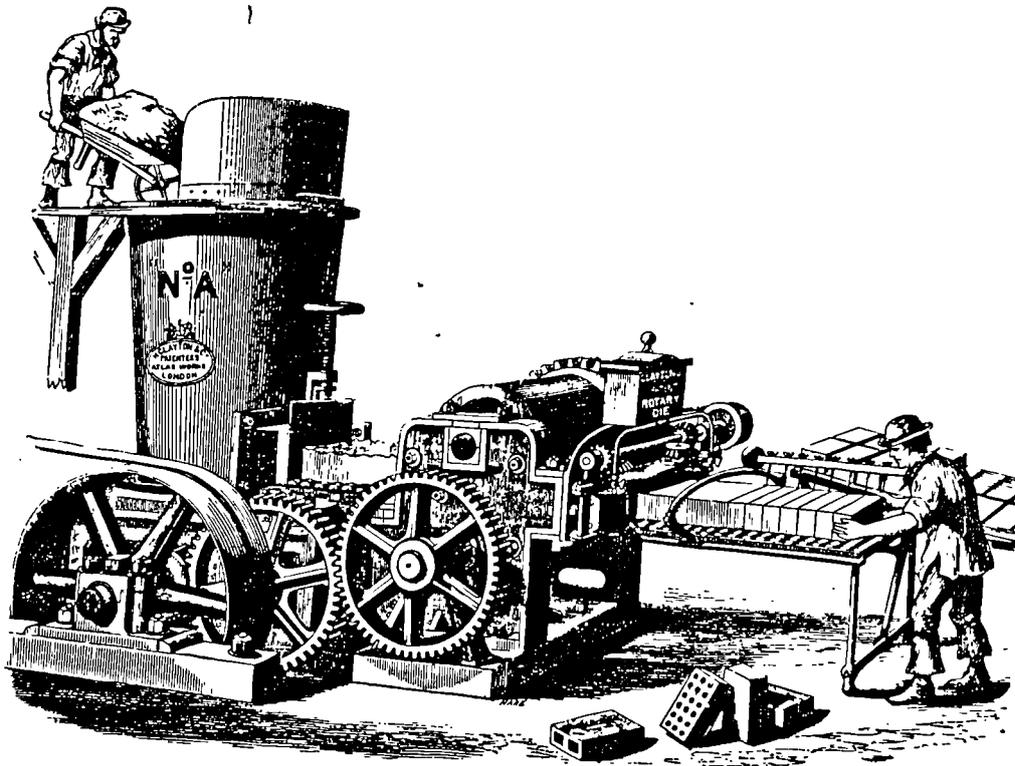
Figure 7.9. Henry Clayton's Combined Two-Process Brick Machine.
