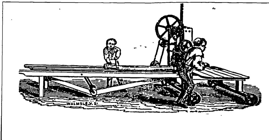
Figure 5.2. Unpatented tilemaking machine by John Hatcher of Benenden, Kent.
