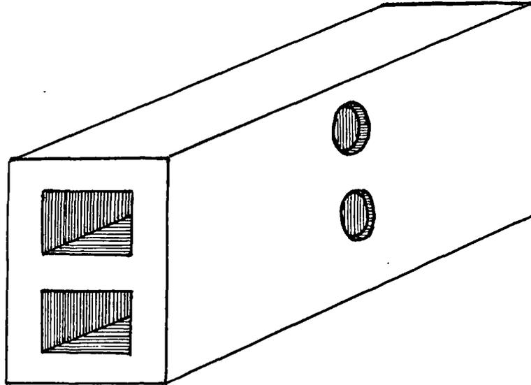
Figure 9.8. Hollow partition bricks patented in France by M. Collas, c.1842.
