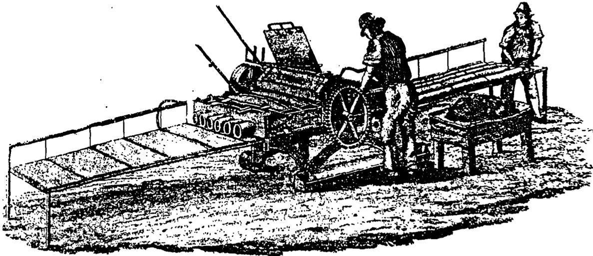
Figure 5.9. Whitehead's prize tilemaking machine, c. 1851.
