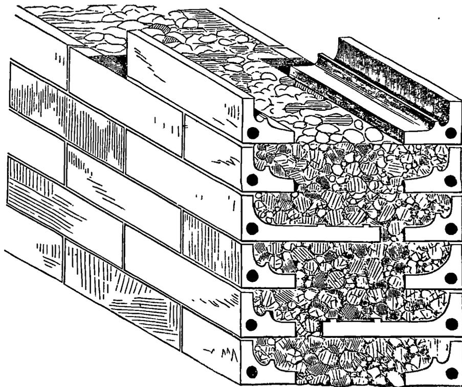
Figure 11.12. John Taylor's perforated facing bricks built into a concrete wall.
