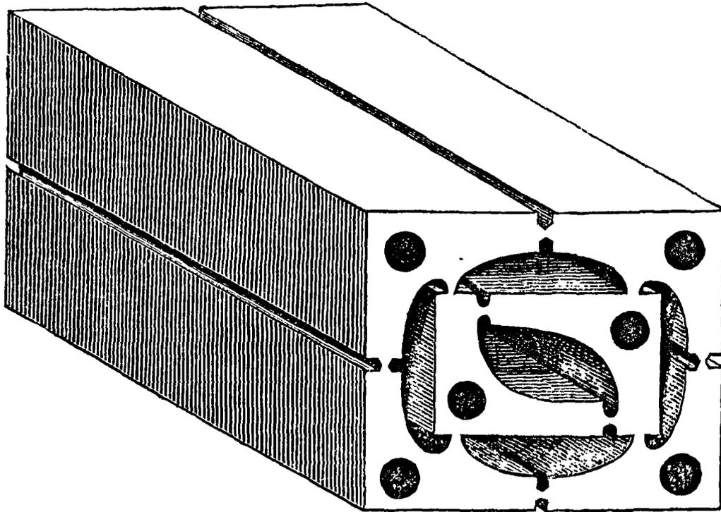
Figure 11.11. John Taylor's perforated facing bricks for bonding in with concrete; machine-extruded in one piece to prevent breakage, 1863.
