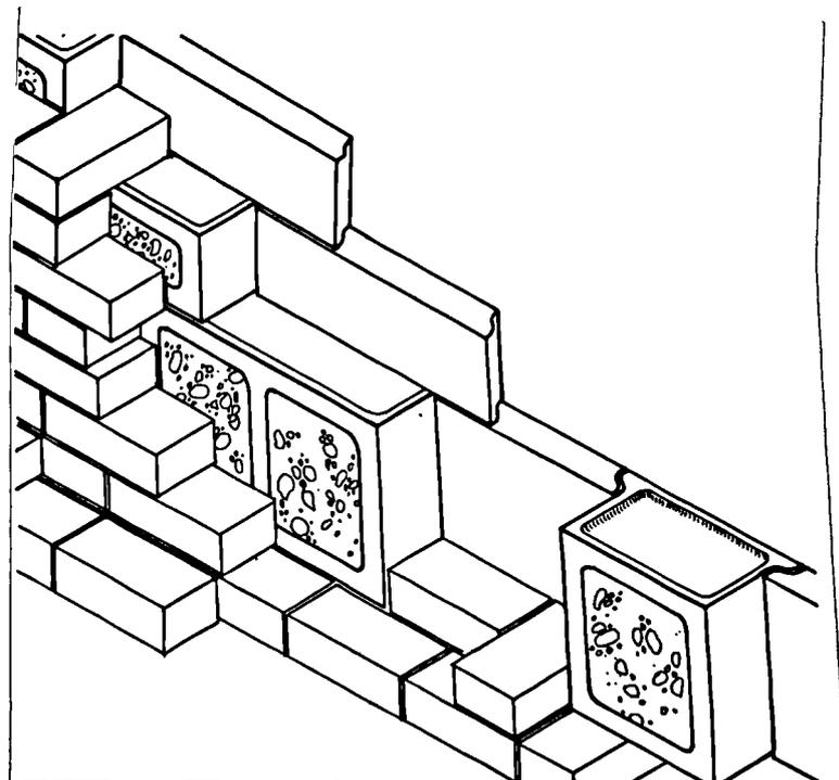
Figure 11.16. Filled terra cotta blocks bonded into the structural brickwork at the Natural History Museum, London, completed 1881. [From John Olley and Caroline Wilson, Architects Journal (1985) p. 41]
