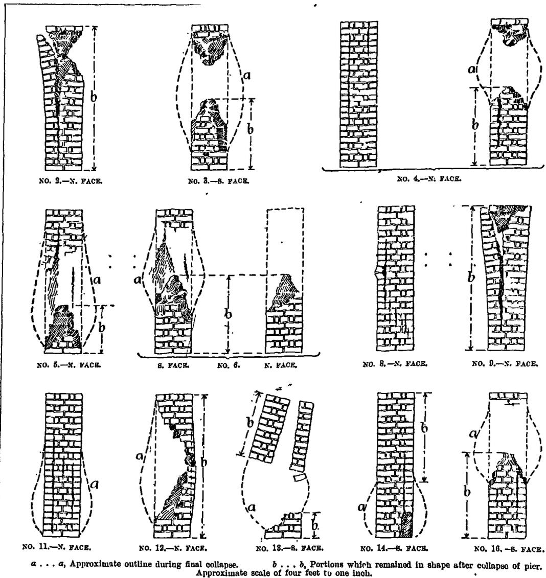
FIG. 13.—DIAGRAMS SHOWING WAYS IN WHICH PIERS FAILED.
