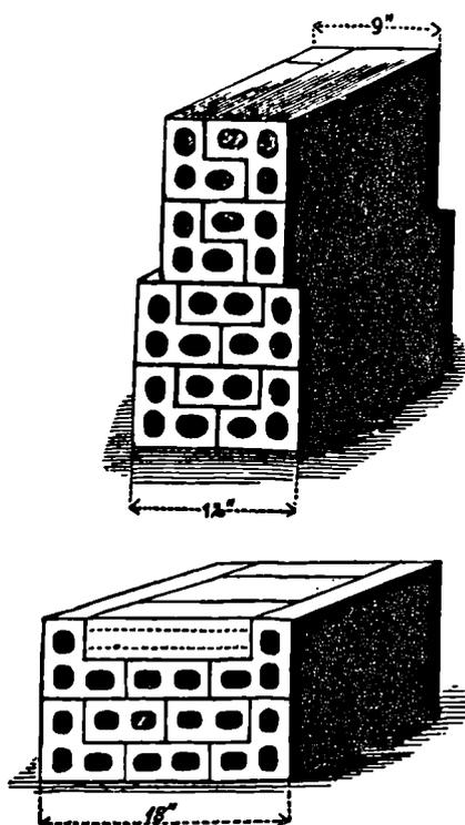
Figure 10.2. Sections of wall built with Henry Roberts' Patent Bonded Hollow Bricks.
