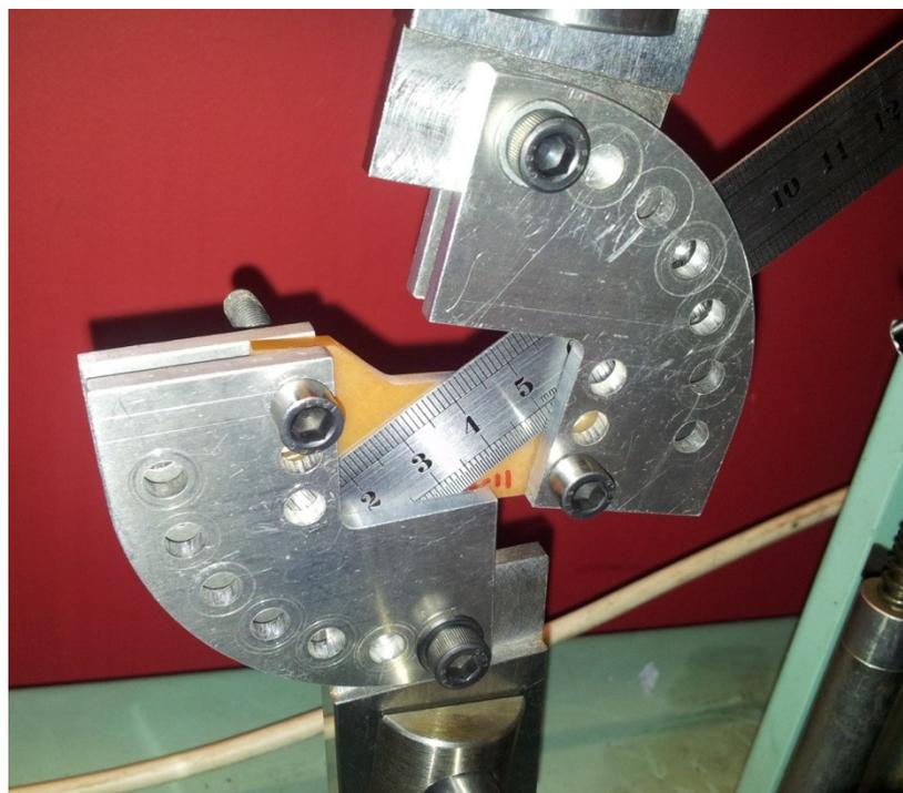
**Figure 4.11 – Steel rule in the plane of a specimen for 2D calibration (note; the specimens were pushed flush with the grip fronts for testing so the focal + calibration planes were kept consistent.)**
