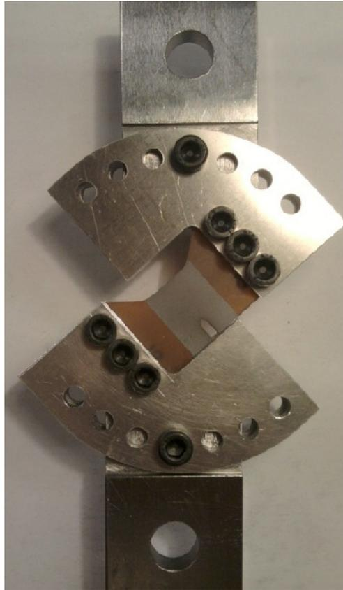
**Figure 6.7 – A painted mixed-mode specimen in the assembled grips at a 45° loading angle.**
