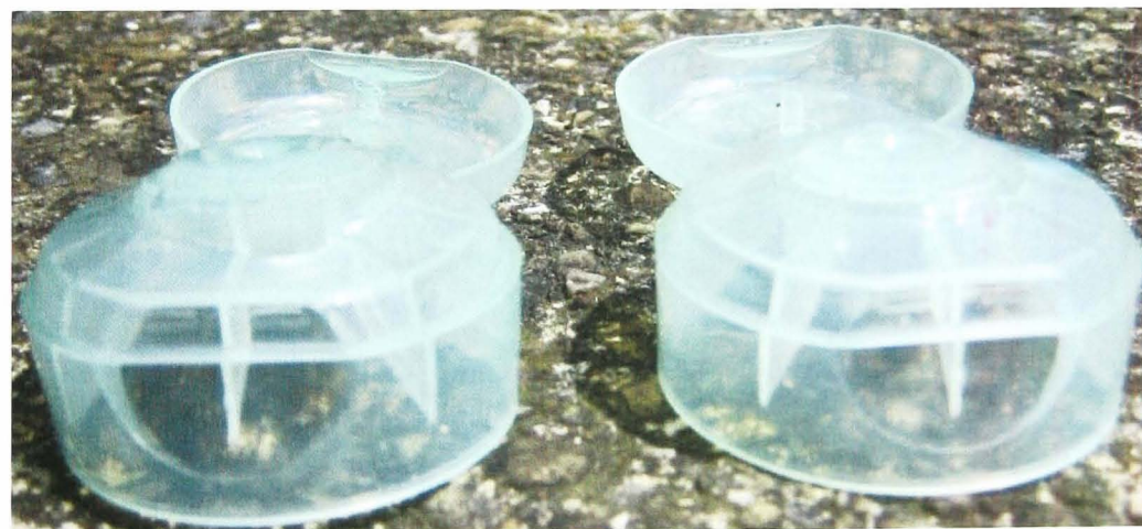
Figure 4-23. Failed Products at 11.3s Cycle Time
