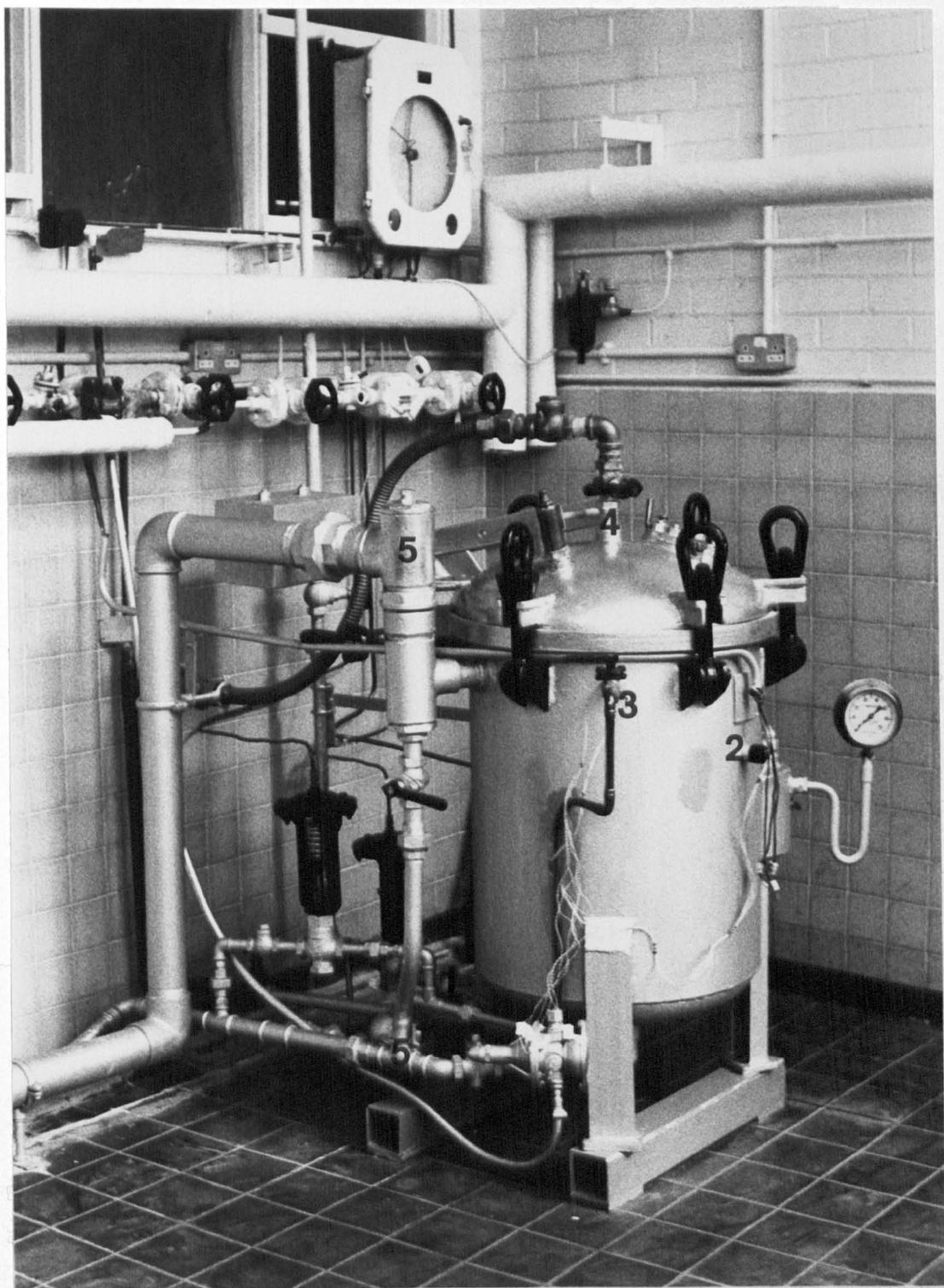
Figure 3.2. Static canning retort. (1) Steam input, (2) compression gland for thermocouple insertion, (3) compressed air line, (4) cold water line, (5) vent and drain.
