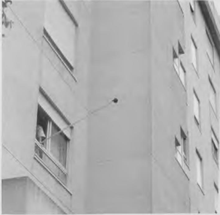
**Figure A4.4: Noise measurement at the apartment façade.**
