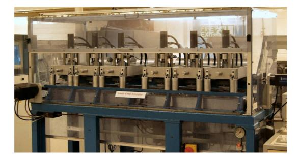
Figure 2.1: Leeds Mark II Physiological Anatomical Six Station Hip Joint Simulator.
