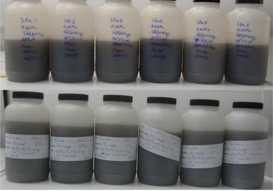
Figure 4.7: Serum colour for all stations at 0.66 million cycles of test (top) and 3 million cycles of test (bottom) under microseparation conditions. Stations 1, 3 and 5 had the cups inclined at 45° and 2, 4 and 6 had the cups inclined at 65°.
