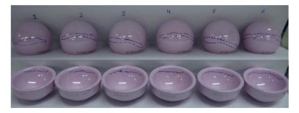
Figure 5.3: Stripe-like wear areas formed on all the femoral heads after introducing microseparation to the gait cycle, with a corresponding wear area near the rim of the acetabular cup.
