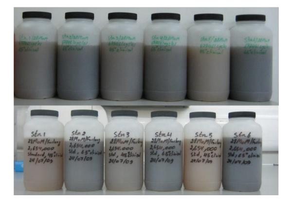
Figure 4.6: Serum colour for all stations at 0.68 million cycles of test (top) and 2.65 million cycles of test (bottom) under standard gait conditions. Stations 1, 3 and 5 had the cups inclined at 45° and 2, 4 and 6 had the cups inclined at 65°.
