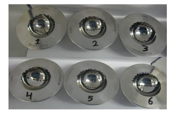
Figure 4.14: Images of the 6 acetabular cups after 6 million cycles of testing. Ink marking show two distinct wear areas; a smooth wear area at the bottom with a rougher wear area adjacent to the rim of the acetabular cup.
