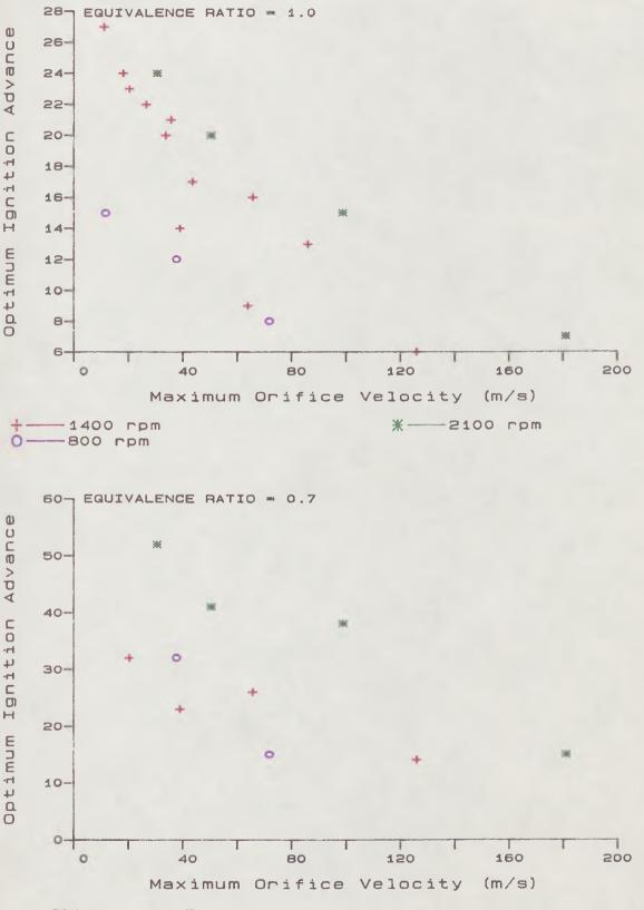
Effect of Maximum Orifice Velocity on Optimum Ignition Advance
