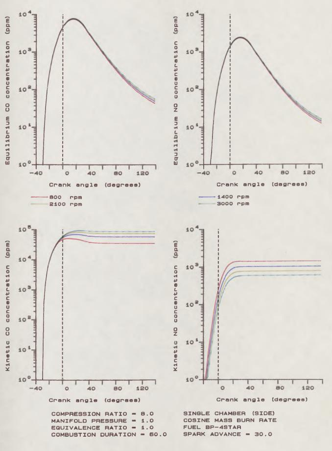
FIG.5.14 Effect of Varying Engine Speed
