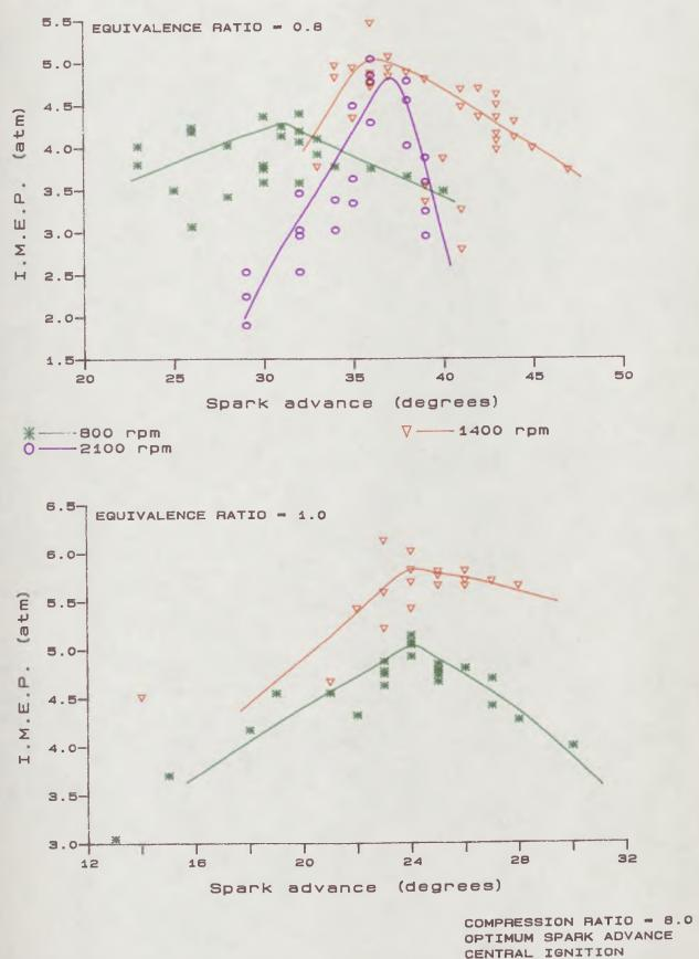
Fig. 4.17 Effect of Engine Speed and Ignition Timing on Power Output
