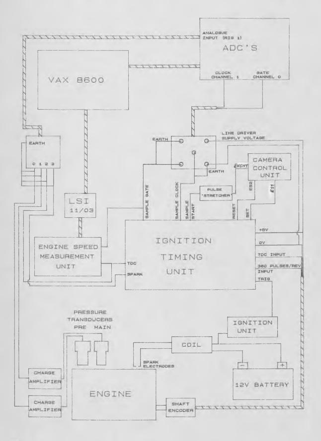
Fig. 3.12 Diagram showing the electronic control and data acquisition system
