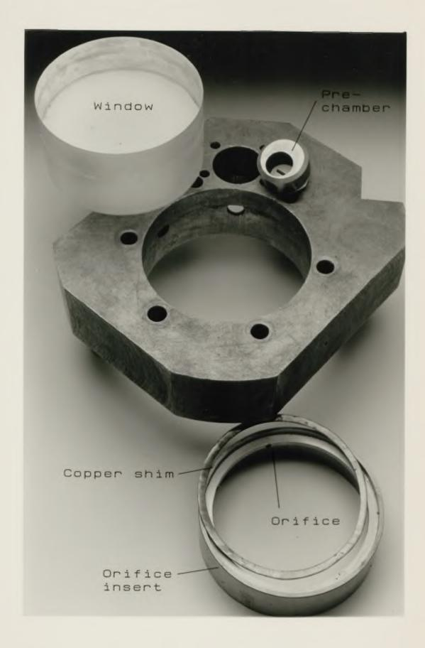
Fig.3.8 The divided chamber cylinder head.
