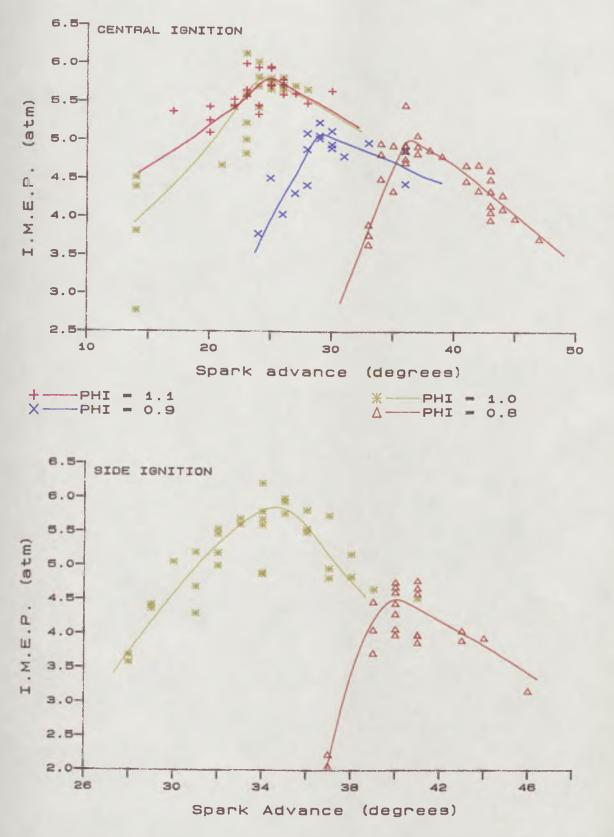
OPTIMUM SPARK ADVANCE ENGINE SPEED = 1400 PPM COMPRESSION RATIO = 8.0
