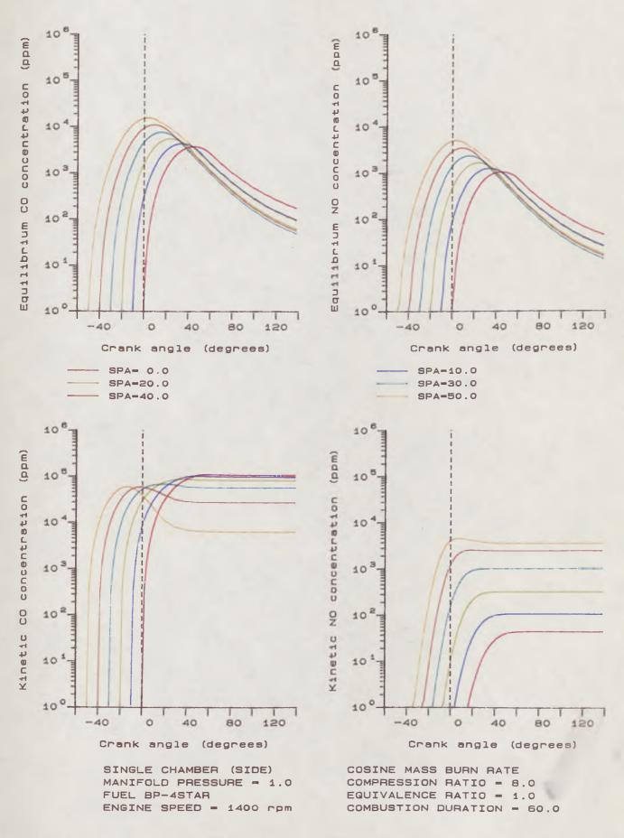
Fig.5.9 Effect of Varying Spark Advance
