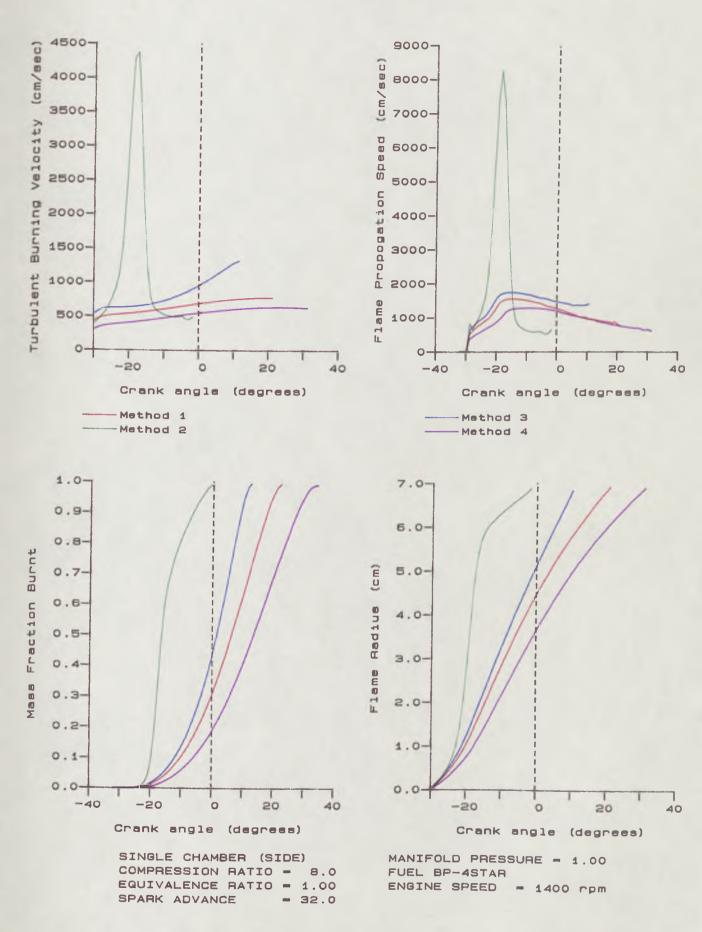
Fig.6.7 Effect of Varying Flame Speed Ratio
