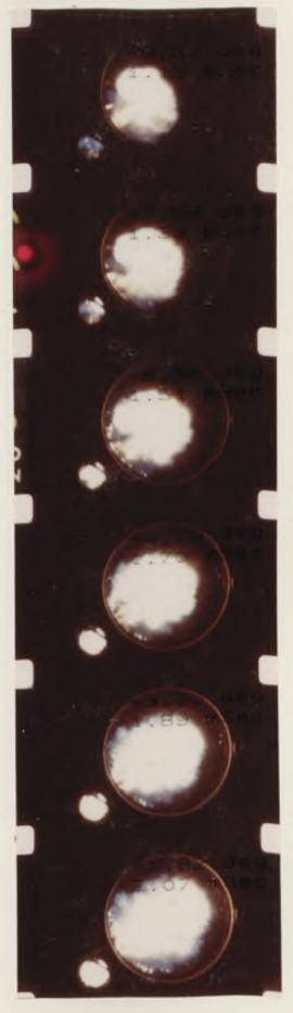
Fig.4.28 Flame propagation photographs (VR = 17%. 10mm x no.5 slotted orifice)
