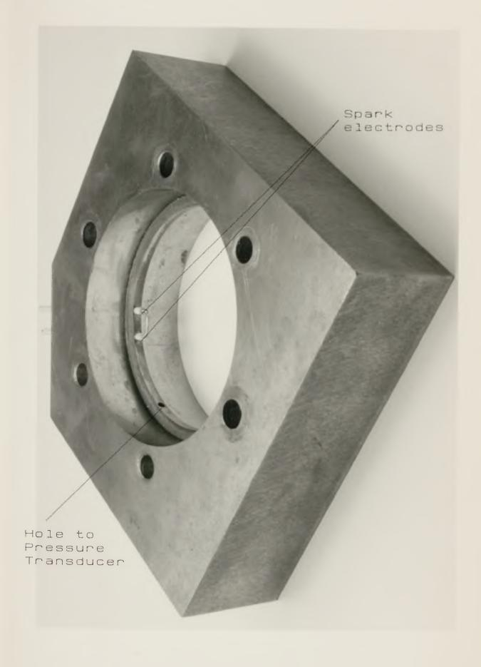
Fig.3.9 The single chamber cylinder head.
