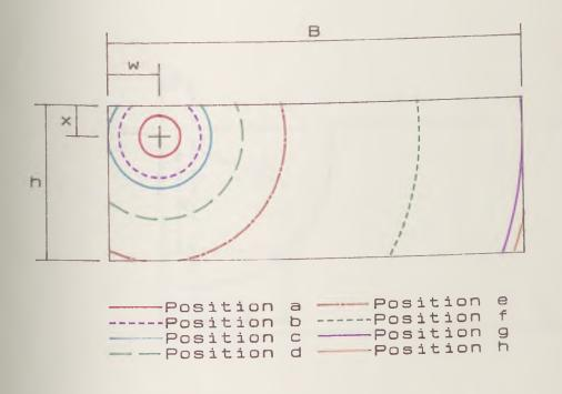
Fig.C.2 Cross section of cylinder showing volume occupied by flame at different radii (side ignition)
