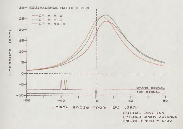
Fig. 4.19 Effect of Compression Ratio on cylinder pressure
