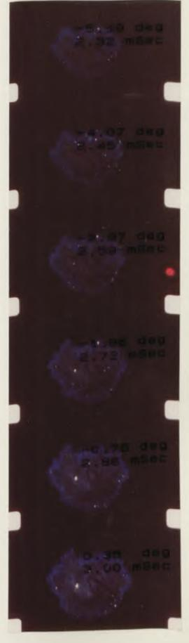
Fig.4.10 Flame propagation photographs (Single chamber, PHI = 1.0) -15.1 deg -5.19 deg 1.09 mSec 2.32 mSec
