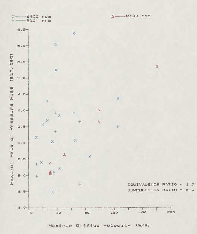
Effect of Maximum Orifice Velocity on Maximum Rate of Pressure Rise in the Pre-Chamber
