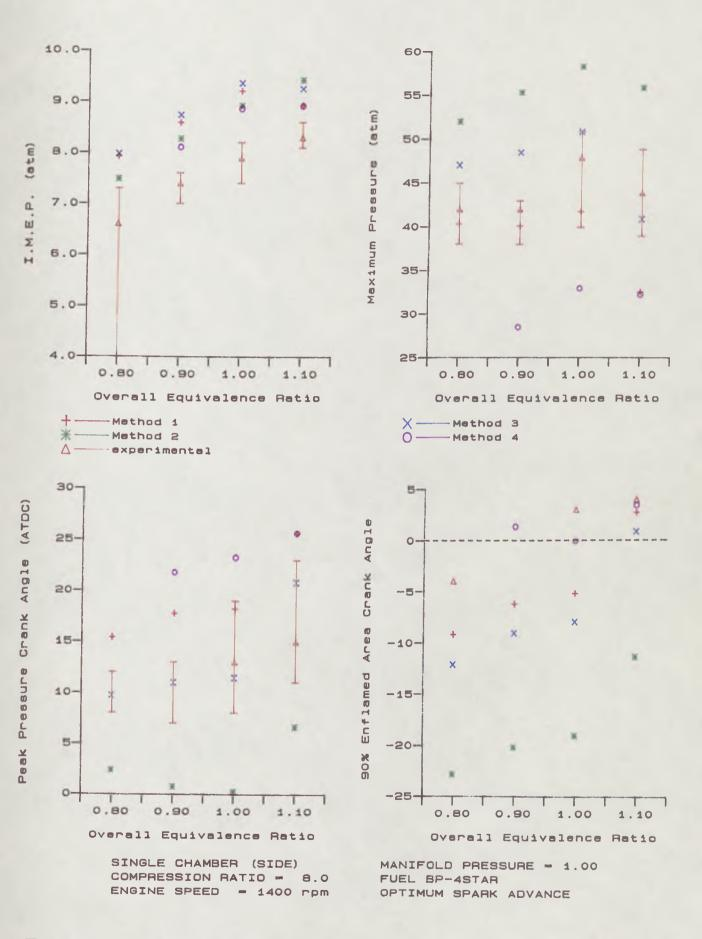
Fig.6.8 Effect of Varying Flame Speed Ratio
