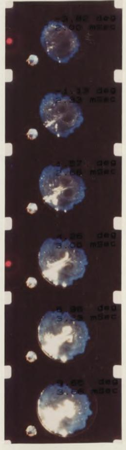
Fig.4.26 Flame propagation photographs (VR = 10%, 2 x no.5 Orifices)
