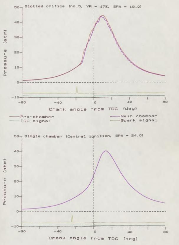
ENGINE SPEED = 1400 Ppm EQUIVALENCE RATIO = 1.0 COMPRESSION RATIO = 8.0
