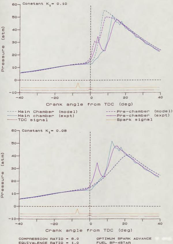
EQUIVALENCE RATIO = 1.0 ENGINE SPEED = 1400 ppm ORIFICE DIAMETER = 5 mm FUEL BP-4STAR VOLUME RATIO = 25%
