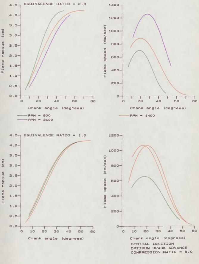
Fig. 4.18 Effect of Engine Speed on flame propogation rate
