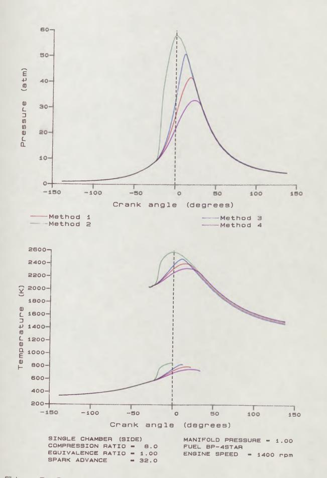
Fig.6.6 Effect of Varying Flame Speed Ratio
