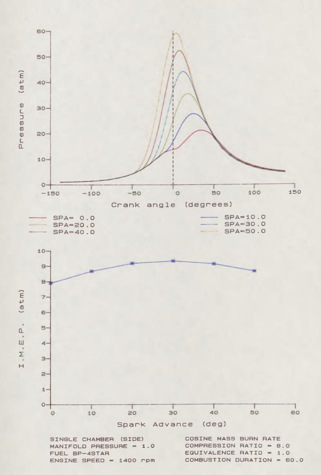
Fig.5.8 Effect of Varying Spark Advance
