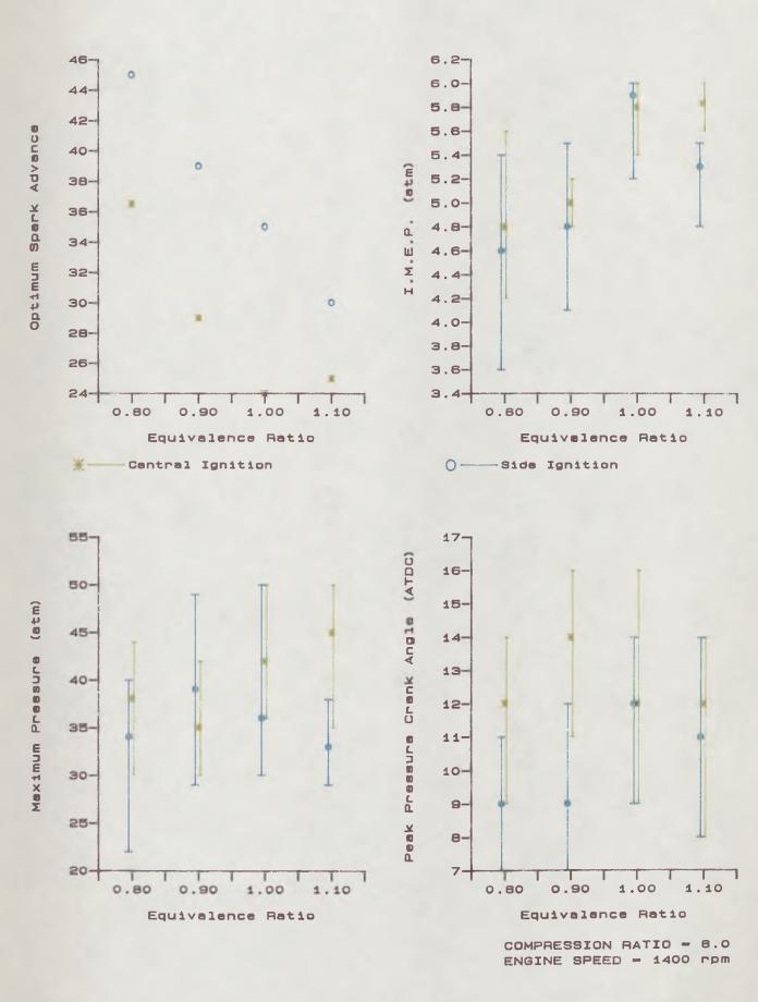
Fig.4.16 Effect Of Spark Plug location
