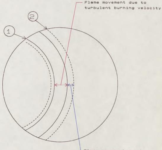
Flame movement due to expansion of burnt charge
