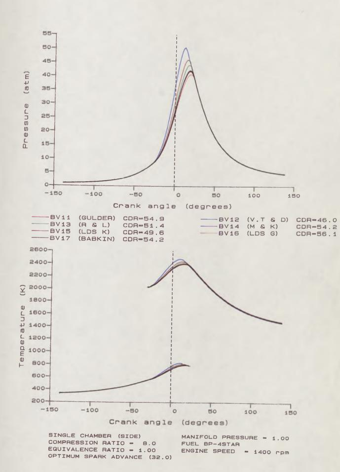
Fig.6.4 Effect of Laminar Burning Velocity
