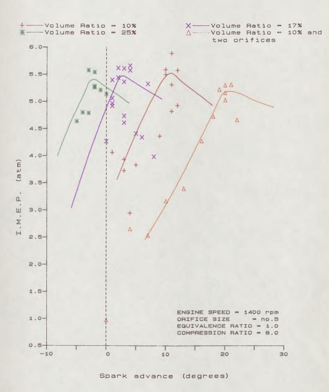
Effect of Volume Ratio on Optimum Ignition Timing
