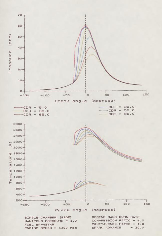
Fig.5.10 Effect of varying combustion duration
