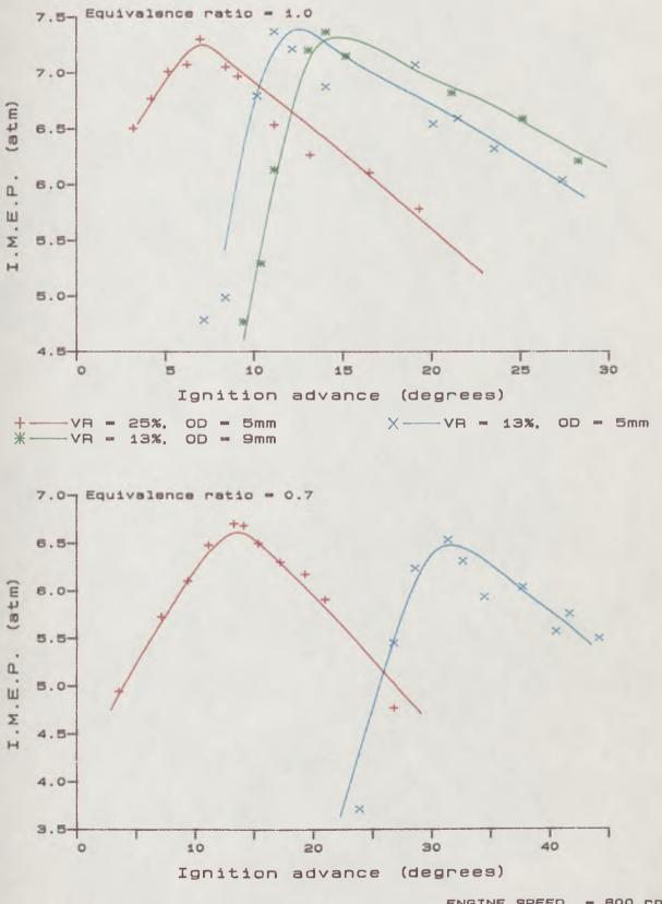
ENGINE SPEED = 800 rpm COMPRESSION RATIC = 8.0
