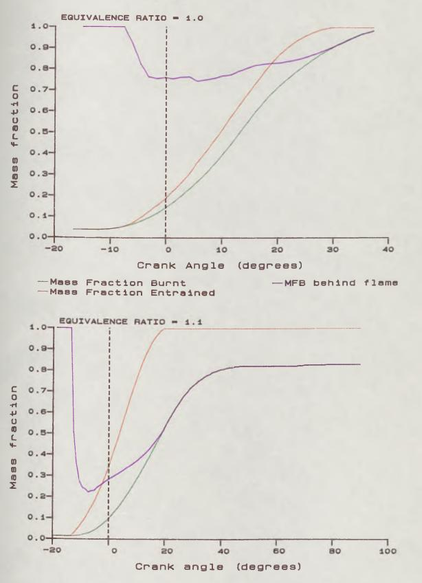
CENTRAL IGNITION COMPRESSION RATIO= 8.0 ENGINE SPEED = 1400
