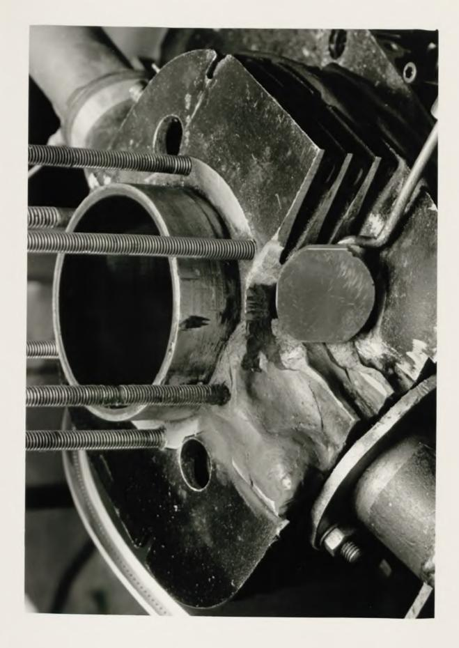
Fig.3.6 Modifications to the cylinder barrel
