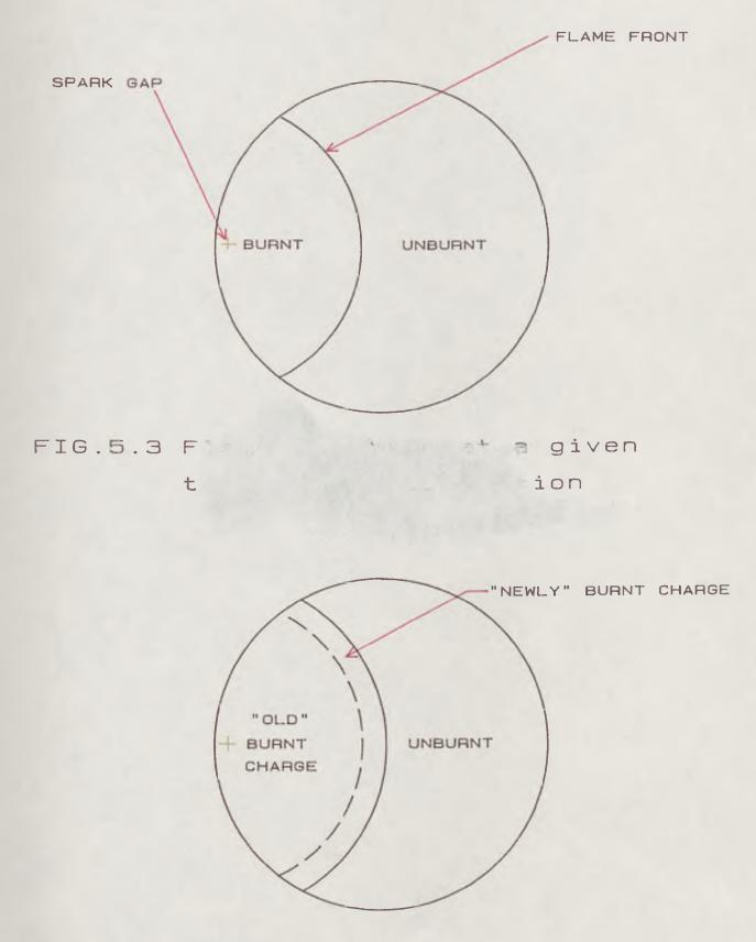
FIG.5.4 Flame position at a later time showing newly entrained charge
