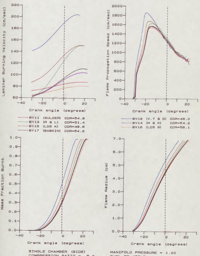
SINGLE CHAMBER (SIDE) COMPRESSION RATIO = 8.0 EQUIVALENCE RATIO = 1.00 OPTIMUM SPARK ADVANCE (32.0) MANIFOLD PRESSURE = 1.00 FUEL BP-4STAR ENGINE SPEED = 1400 rpm
