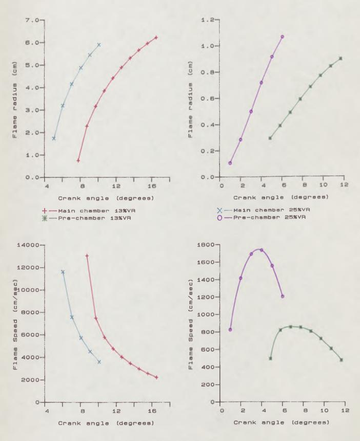
Comparison of flame propagation rates with varying volume ratio.
