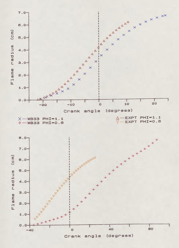
Fig.5.16 Comparison of Experimental And Predicted Flame Radii
