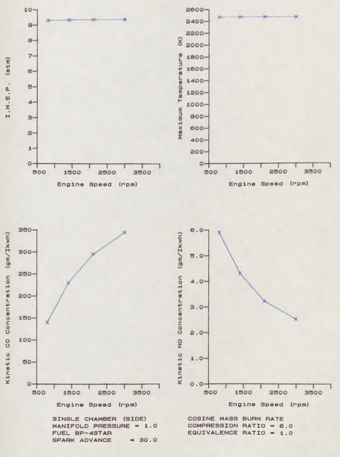
Fig.5.15 Effect of Varying Engine Speed
