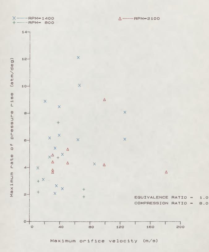
Effect of Maximum Orifice Velocity on Maximum Rate of Pressure Rise in the Main Chamber
