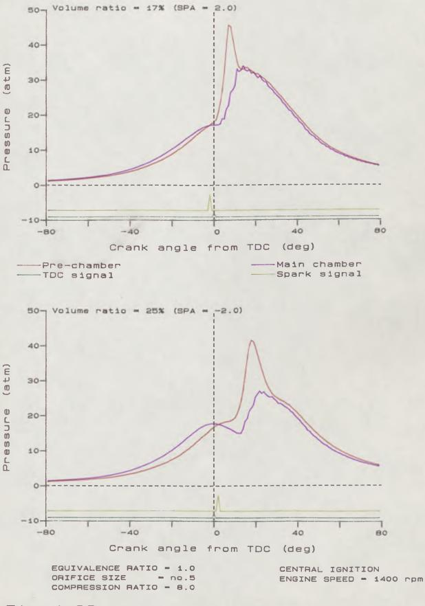
Effect of Volume ratio on Cylinder pressure
