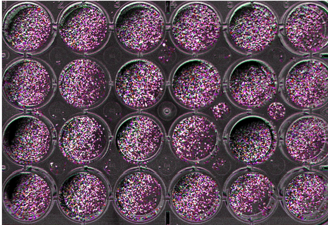
Figure 4.5: The spread of signal across a 24 well microplate. This time-to-colour merge picture was generated from frames 877-882 of the “Salt test” video (Supplementary Material). Grey scale shows lack of movement, colour indicates movement. Overall, the spread of movement looks even across the plate. Note: dark patches within the wells are due to light reflection and high density salt patches; movement colour outside of the wells is due to salt escaping from the wells.
