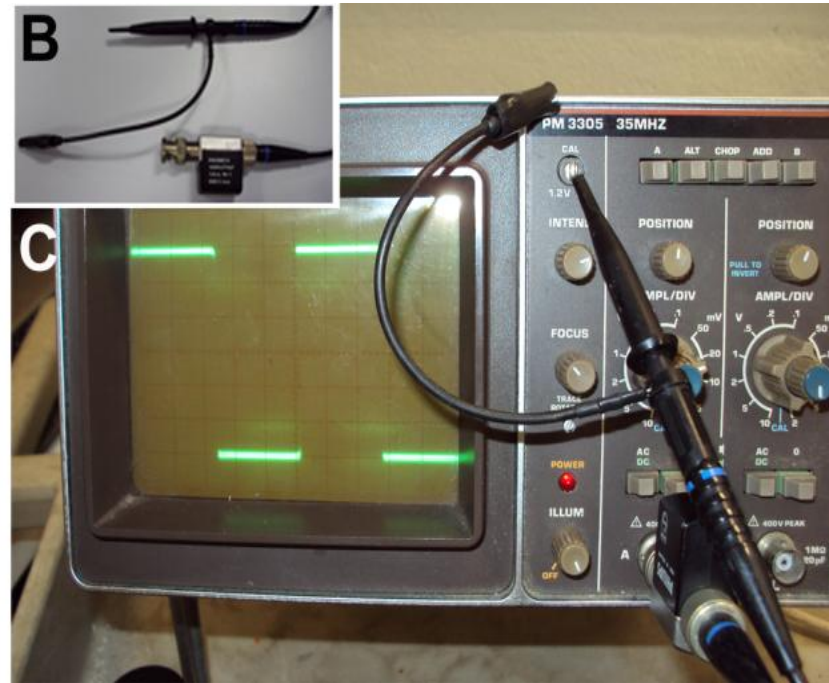
Figure 2.5: Calibration of the oscilloscope. The oscilloscope was adjusted using a trimmer and measuring pin (B), which was attached to oscilloscope (C). Adjustments were made to ensure correct compensation (A).
