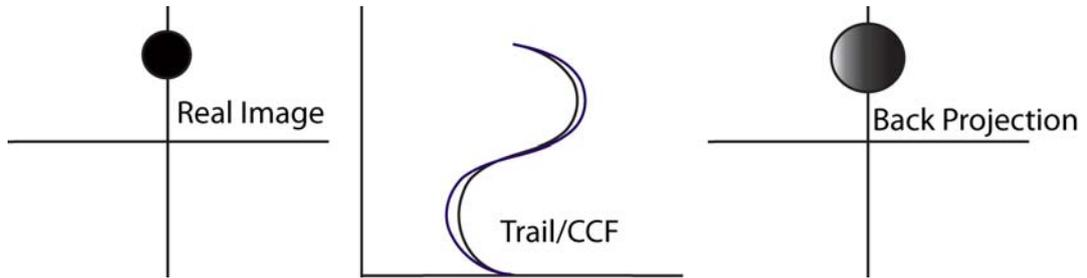
Figure 3.8: Left: An emission site in a real image  $(0, K_y)$ . Centre: The resulting trail from a point in the emission site (black), together with a sinusoid of similar velocity (blue). Right: A back projection of the trail without filtering. The image is blurred due to contamination with similar sinusoids.
