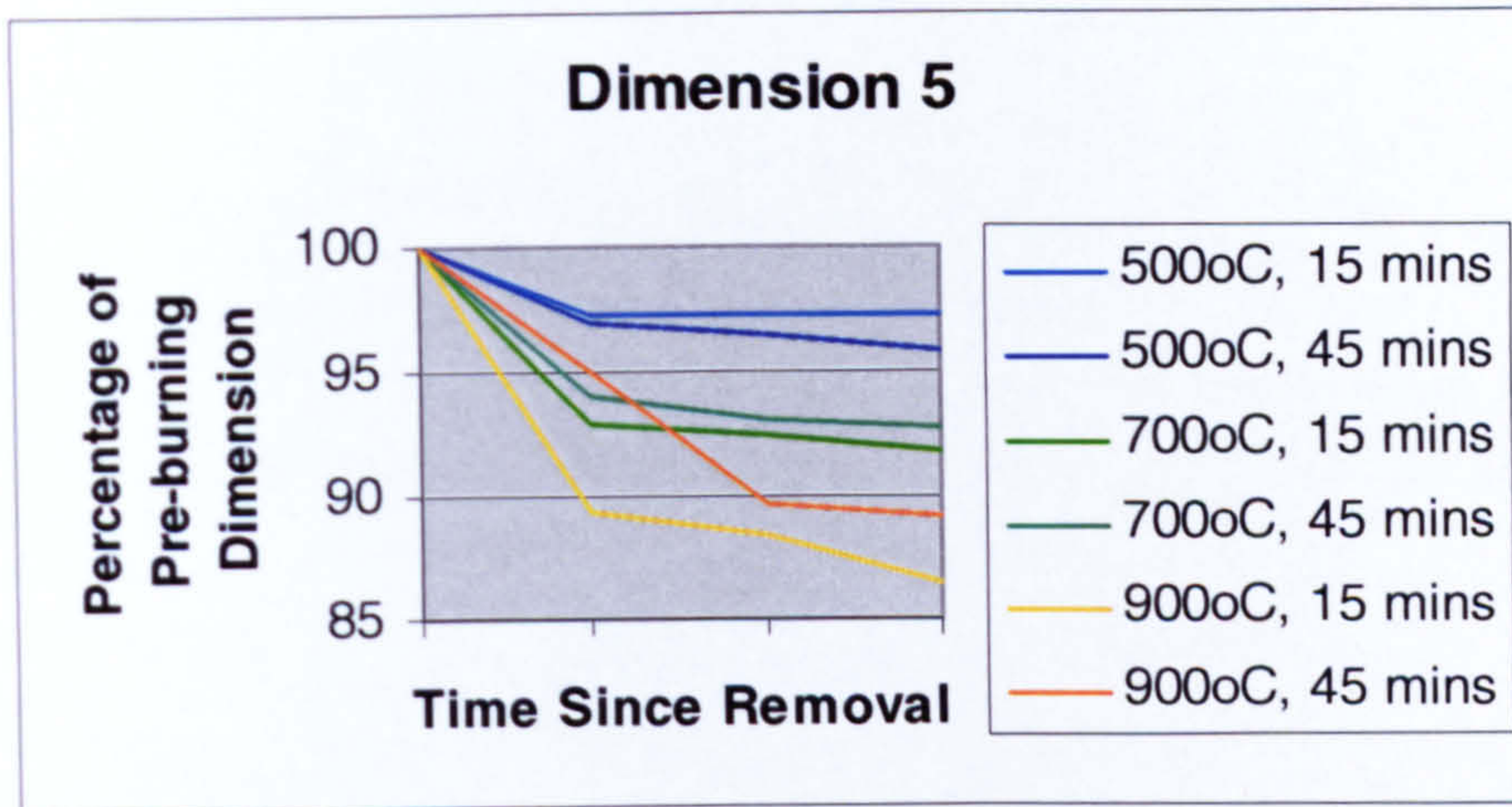
Figure 9.5 Heat-induced dimensional change in experimentally-burned bone
