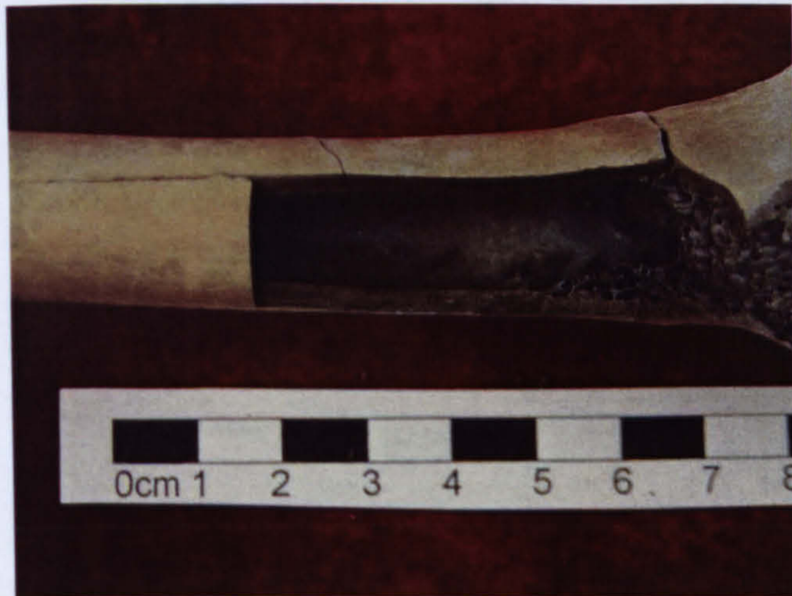
Figure 5.21 Variations in Colour in Sample 3-0005-01 [500°C for 45 minutes]
