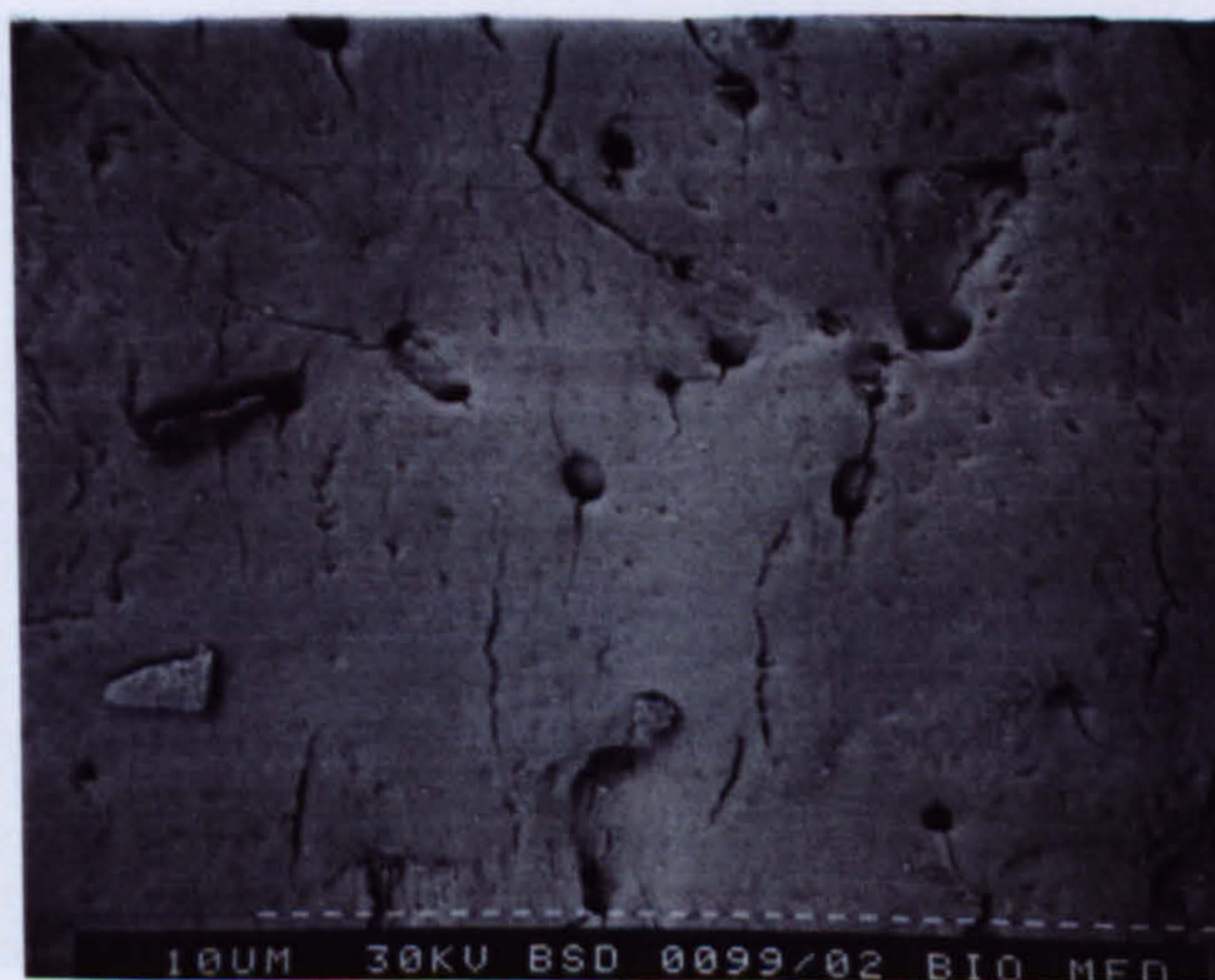
Figure 6.18 SEM image, sample 3-2-7, outer surface (upper), inner surface (lower) [500°C for 15 minutes]
