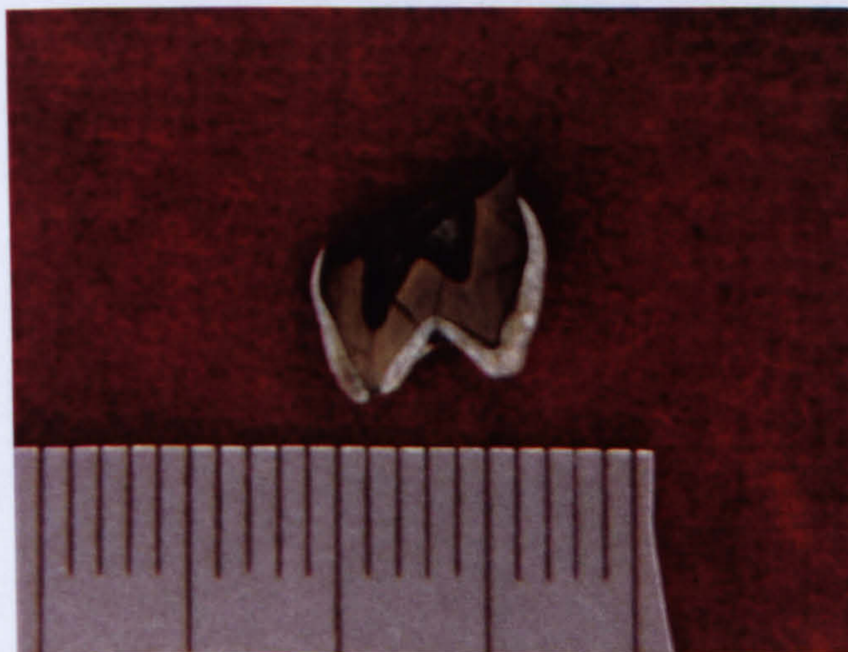
Figure 5.22 Variations in Colour in Sample 4-0001-04 [500°C for 15 minutes]
