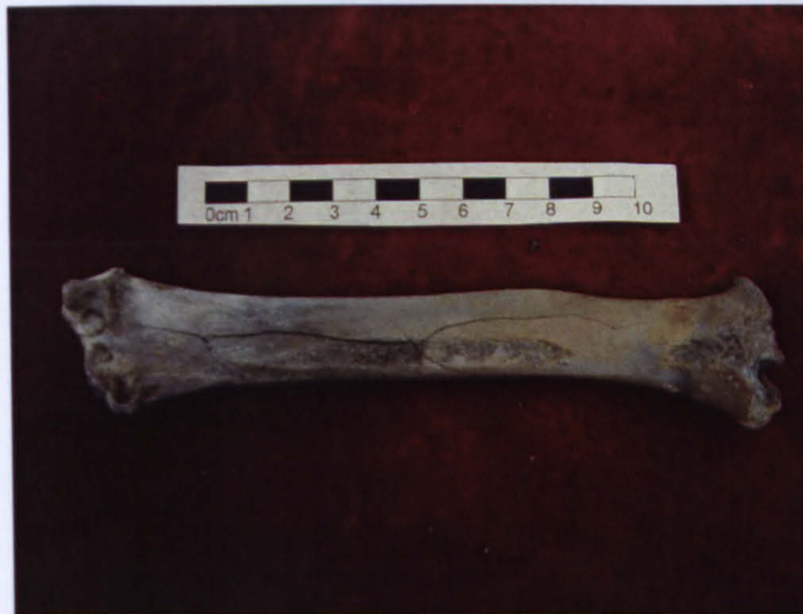
Figure 5.19 Multiple Colours on Sample 3-0005-08 [500°C for 45 minutes]
