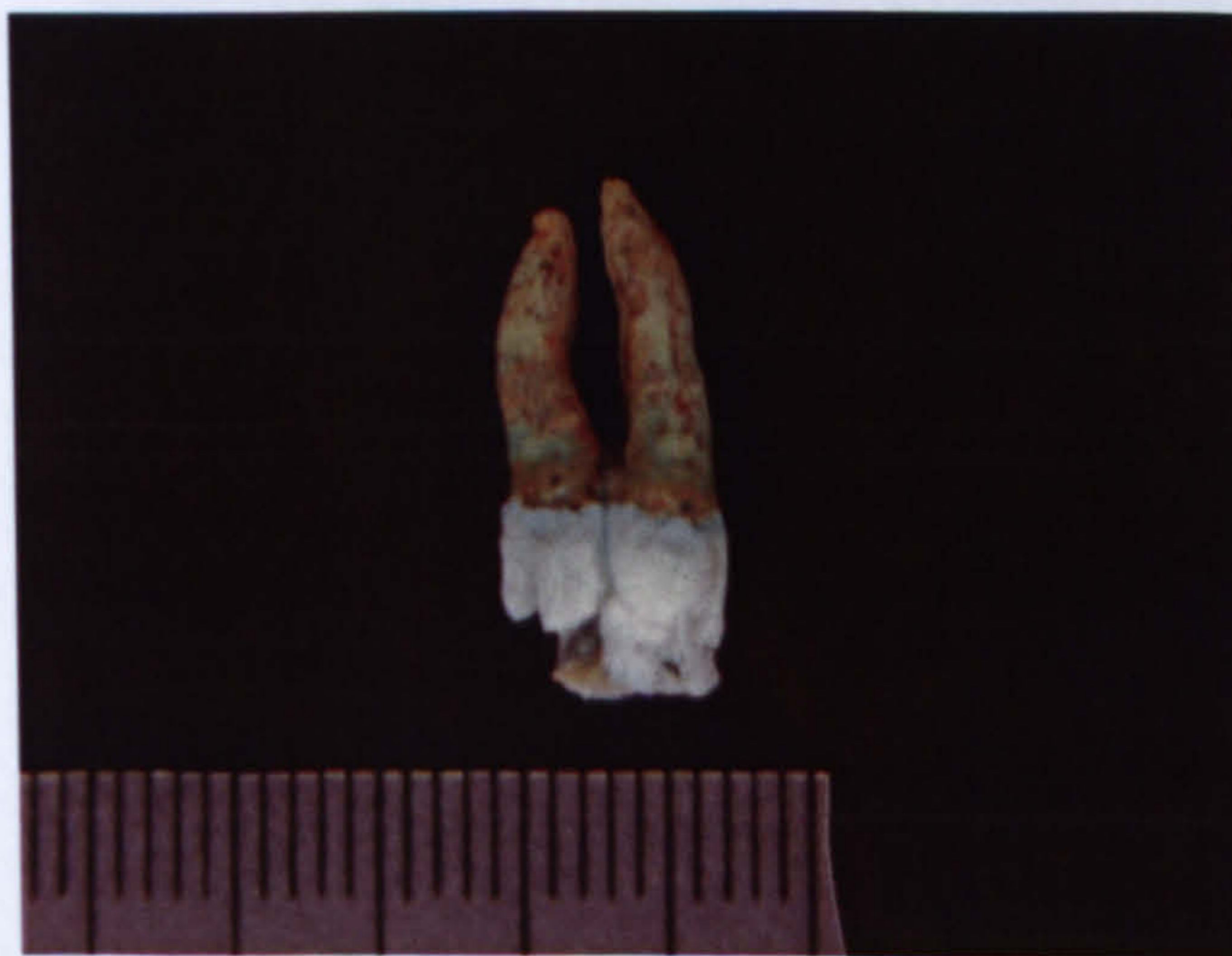
Figure 5.20 Multiple Colours on Sample 2-0005-01 [900°C for 15 minutes]
