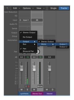
\* The number of output options depends on the number of outputs of your audio interface. Find out which output on the audio interface the speaker is connected to, then select the output number in Logic accordingly.
