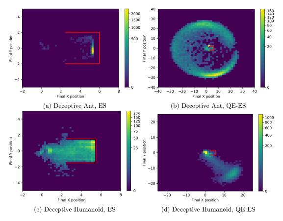
Figure 4.8: 2D histogram of the final positions of the population from the last generation for the Deceptive Ant and Deceptive Humanoid tasks. The red lines represent the walls of the trap, which makes the problem deceptive. For both environments, ES ends up trapped, (a) and (c), while QE-ES is able to overcome the local optimum, (b) and (d). Please note the change in scale.
