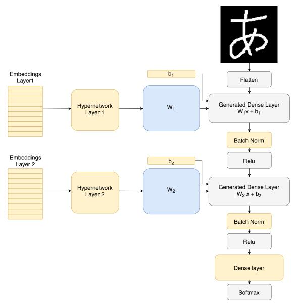
Figure 6.4: The indirect architecture used in the experiments. The yellow boxes are learned parameters, the blue boxes are generated parameters and the grey boxes are functions. The direct encoding uses the same architecture, but the two dense layers are represented directly.
