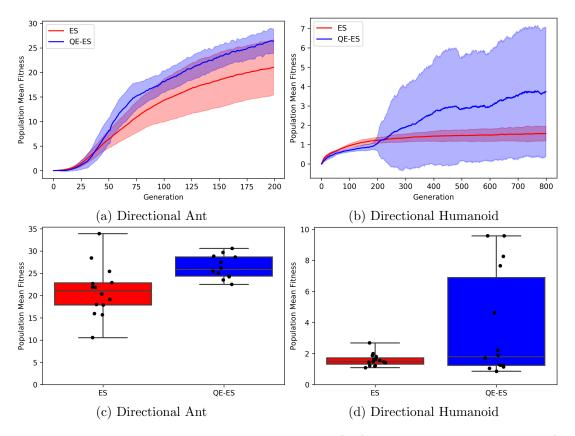
Figure 4.6: Mean fitness for the Directional Ant (a,c) and Directional Humanoid (b,d) tasks, where evolvability and fitness are not aligned. In (a), both algorithms are able to find good policies, but QE-ES receives higher fitness on average. In the more difficult task (b), ES fails to learn to walk and turn in the right direction at the same time, while QE-ES is able to make progress.
