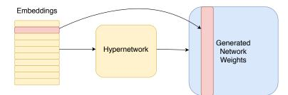
Figure 6.2: Hypernetworks: Each embedding is transformed into a chunk of weights by the Hypernetwork [6]. Yellow blocks represent the learned parameters, the blue block represents the generated weights, and the red blocks show an example of how a single embedding is transformed into a chunk of generated weights. See Fig. 6.4 on how a Hypernetwork can be used as part of a larger model
