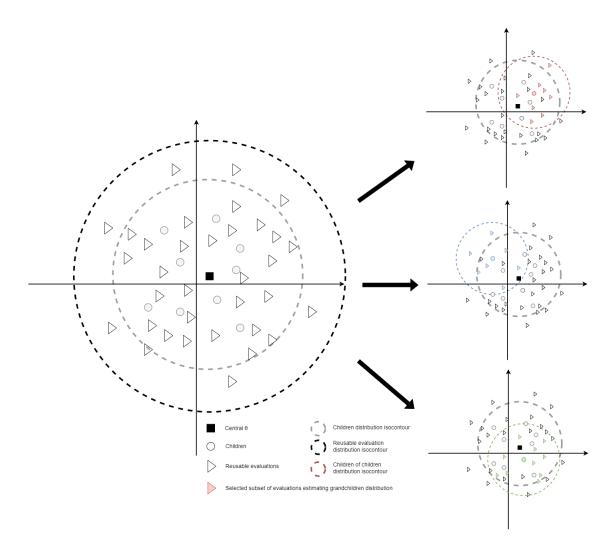
Figure 4.2: This figure illustrates how Resampling EE-ES reuses evaluations multiple times to estimate the evolvability of each child. Because the same evaluations are reused multiple times, Resampling EE-ES can get away with c\*n evaluations, (*n* is the population size, *c* is a constant not dependent on population size), instead of the  $n^2$  evaluations of the normal EE-ES (4.1).
