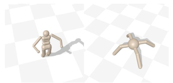
Figure 5.2: The robots from the brax humanoid (left) and ant (right) environments. Fitness is the distance walked by these robots, while the behaviour descriptors are the x and y coordinates of the final position of the robots at the end of the simulation.
