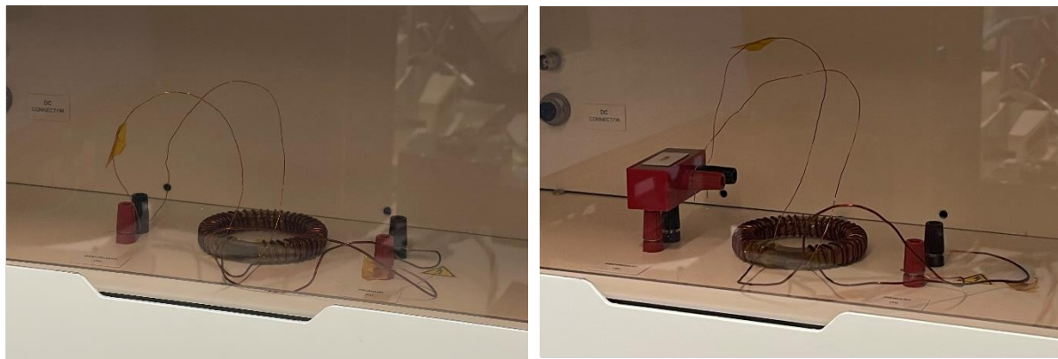
a. Directly connected (low induced V_2 )
