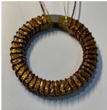
Figure 6.3 Toroid sample construction steps
