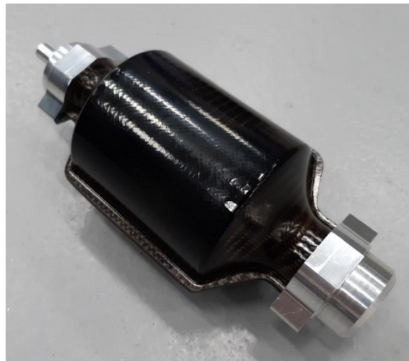
Figure 6.16 Novel hollow carbon-fibre shaft and hub
