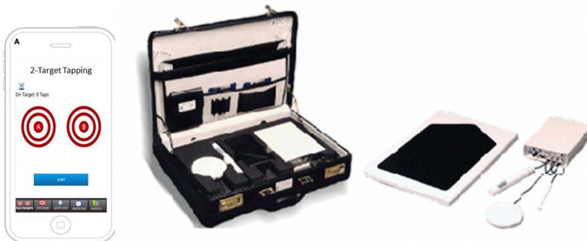
**Figure 2.1.** Two surface contact methods to record finger tapping. The left side of the figure shows smartphone screen targets [20], the right side shows equipment that includes a touch recording plate (the white circle) [17].
