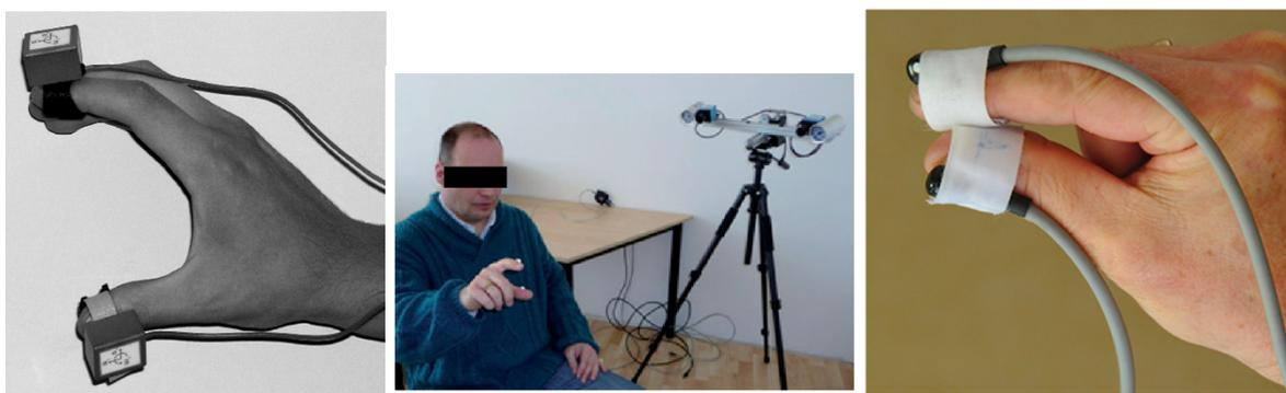
**Figure 2.2.** Wearable devices to record finger tapping. Left to right: systems based on gyroscopes [27], infrared cameras [37], and electromagnetic sensors [44].
