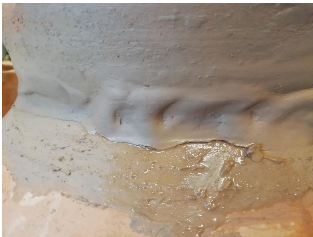
Figure 45. Distillate / condensing vapour penetrating through the clay seal between the still head and body during the 2000 ml run with the Gandhāra apparatus configuration.
