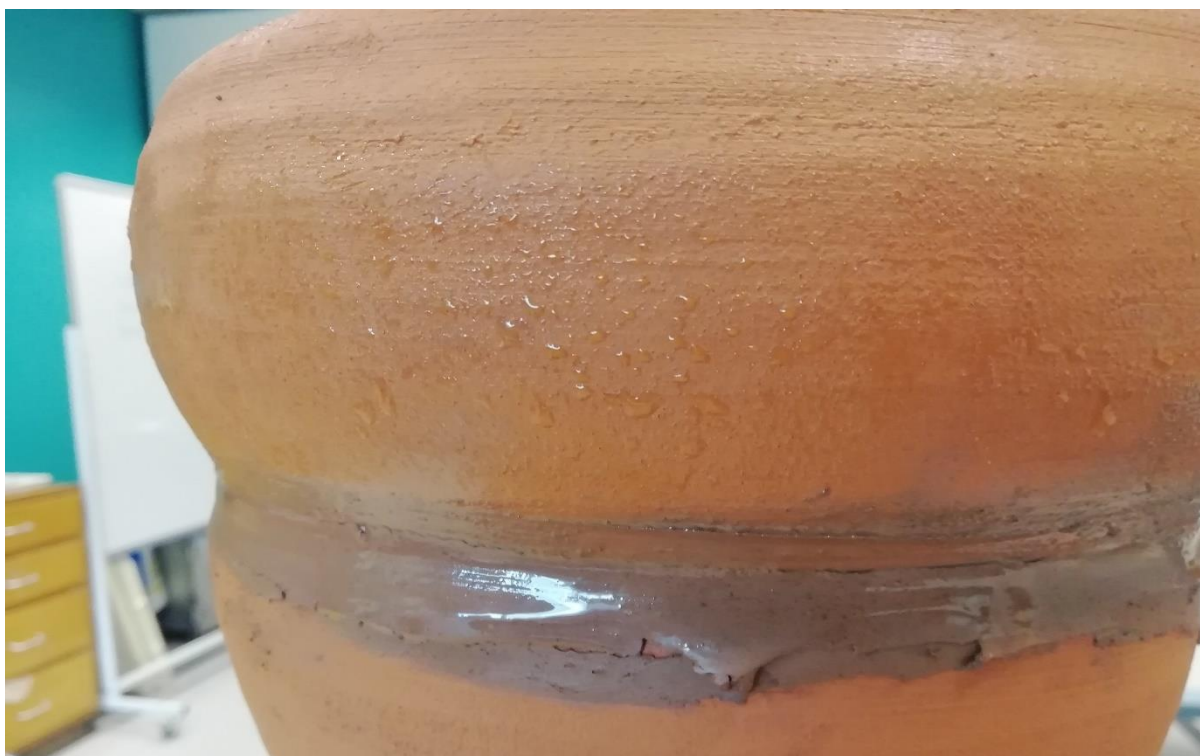
Figure 61. External 'sweating' noted on the condenser exterior.
