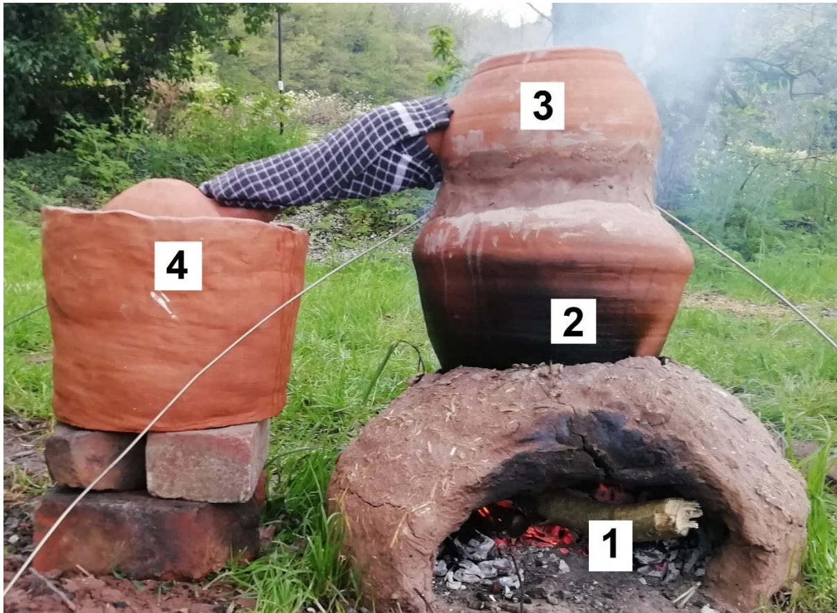
Figure 46. Location of thermocouples on reconstructed Gandhāra apparatus: 1. Heat source (within hearth); 2. Distilland (inside still body, below level of liquid and not touching ceramic interior); 3. Still head (interior); 4. Receiver (interior). The use of the hearth instead of a hotplate as employed in the preliminary experimental studies (see Chapter 5) allows for a greater surface area of the still body to be heated.
