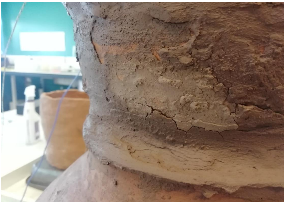
Figure 40. Slip layer applied over seals between body and condenser as an intervention to help maintain optimal distilling conditions (photograph by the author).
