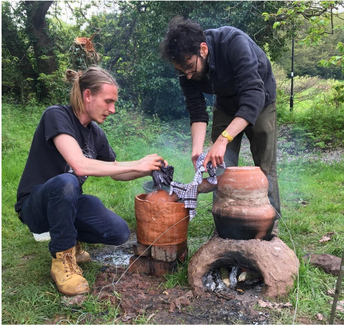
Figure 50. The complete reconstructed Gandhāra still in operation using a clay hearth to heat the distilland and cloths being changed along the condensing tube (photograph by Matthew J. Lester).
