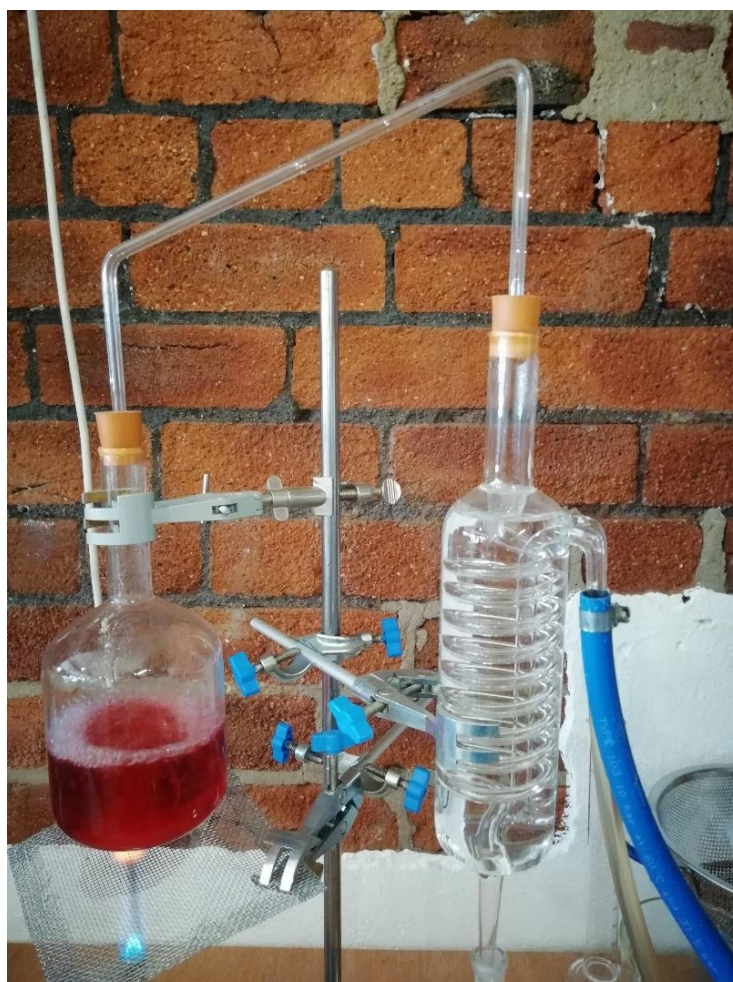
Figure 4. A modern laboratory Thorpe still apparatus in use for alcohol by volume (ABV) analysis (right); the ethanol in the alcoholic red solution is vapourised, travels through the glass adapting pipe (moving from a hotter to colder atmosphere) and is then condensed in the cooler atmosphere maintained in the glass condenser before collecting into a receiving vessel below (photograph by the author).
