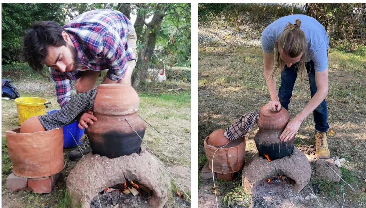
Figure 53. Repairing seams between the apparatus components using clay and clay slip to maintain a pressurised atmosphere in the still (photographs by the author and Matthew J. Lester).
